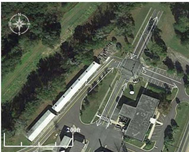
The four-leg intersection at the TERL (Figure 4-1) has six approaching lanes and four departing lanes and is located on level terrain. Turning lanes were not be utilized throughout the testing to simplify the phasing patterns. There was no lane-changing occurring once a vehicle arrival is detected and no pedestrians were assumed to be present in the vicinity of the intersection. A total of six vehicles were used
