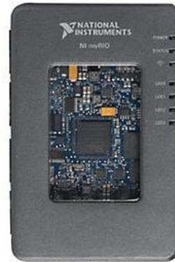
**Figure 3-13 National Instruments (NI) myRIO-1900 to replace the previous hardware**
