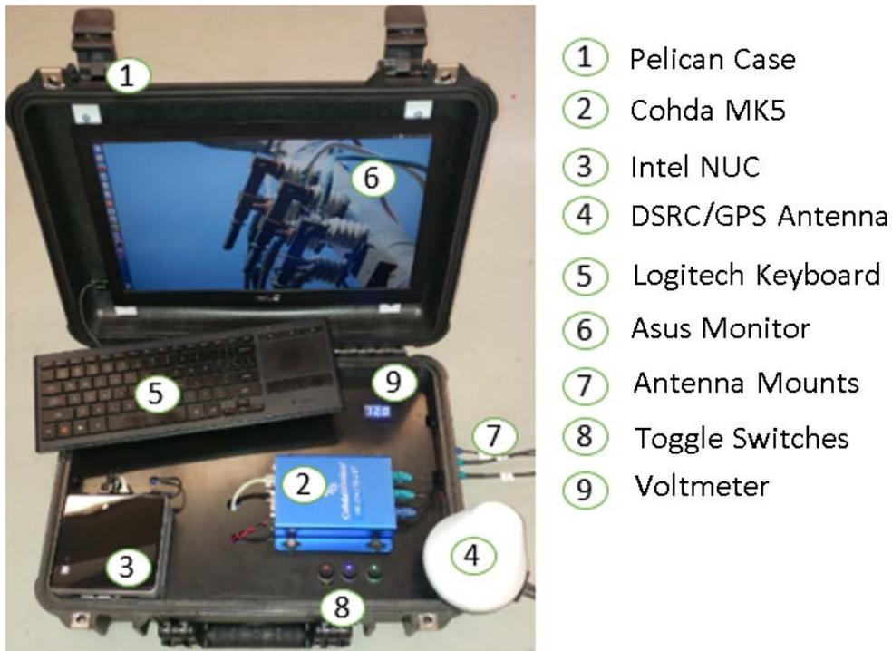
**Figure 3-8 Connected vehicle suitcase**
