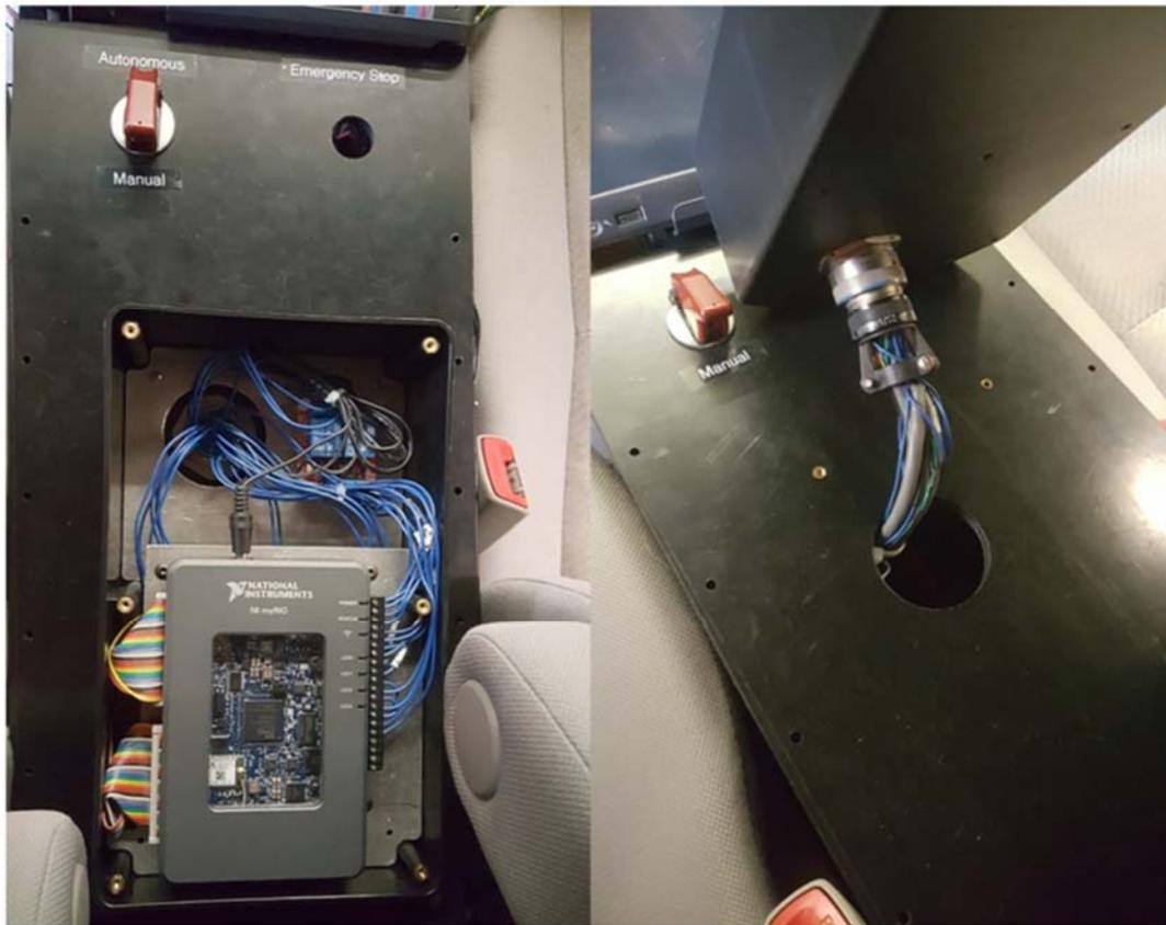
**Figure 3-16 (Left) Top view of the cover plate. (Right) View of the bottom of the box**
