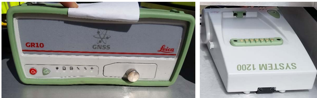
Figure 3-9. GNSS receivers: GR10 (left) and GRX1200 (right).
