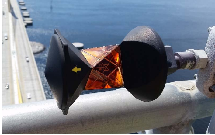
Figure 3-12. Prism on the North Tower.
