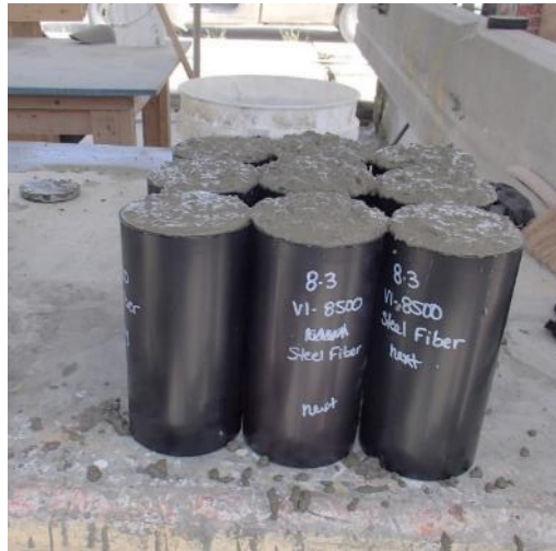
Figure C-3 Cylinders for testing of compressive strength
