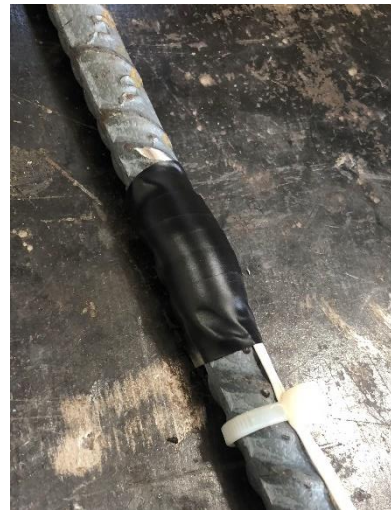
Figure 4-32 IS strain gage prior to reinforcement installation
