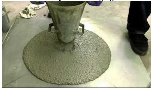
Figure A-1 Test setup for ASTM C1611-11
