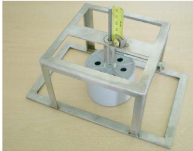
Figure A-5 Test setup and penetration apparatus (ASTM C1712-14)
