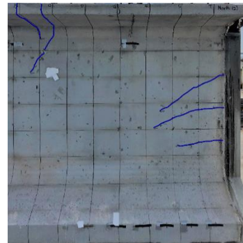
Figure 5-40 End region cracking after prestress transfer for SH-30 specimen: (a) analytical and (b) experimental.
