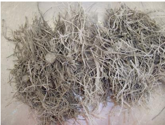
Figure 2-14 Fiber clumping during mixing (Macrosynthetic fiber with length 2.3 in. (58 mm) at volume of 0.7%)
