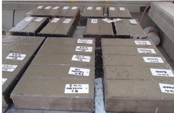
Figure C-2 Beam molds and cast specimens
