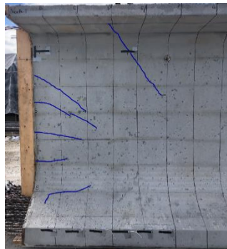
Figure 5-40 End region cracking after prestress transfer for SH-30 specimen: (a) analytical and (b) experimental.
