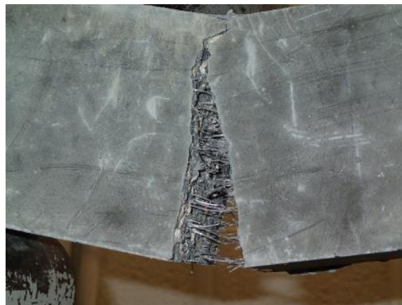
Figure 3-12 ARS test specimens cracked surface
