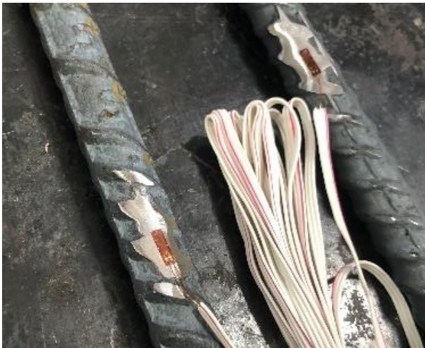
Figure 4-32 IS strain gage prior to reinforcement installation
