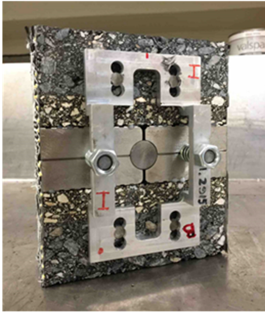
(b) Assembled CSIC specimen
