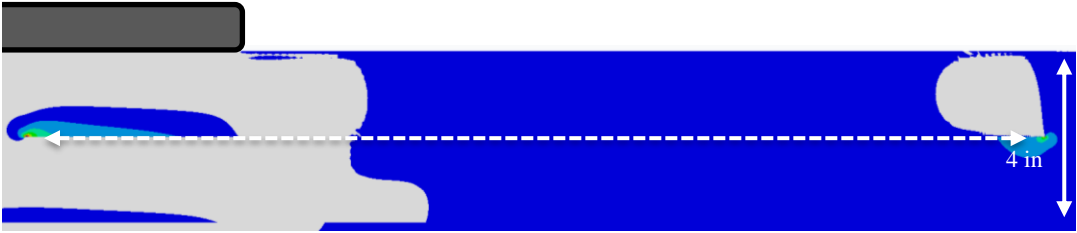
c. Load center moved 12 in from wheelpath center
