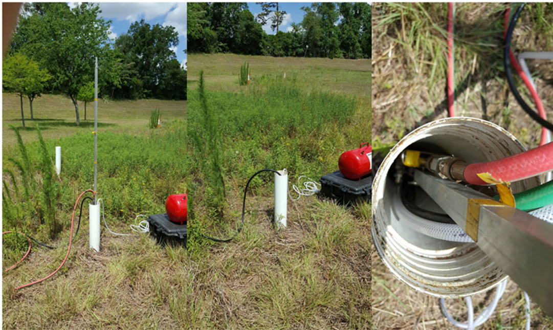
Figure 4-17 Setup of low-frequency solenoid source and 3D geophone string at Newberry site
