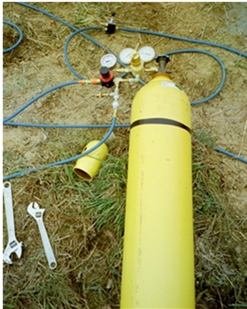
Figure 2-8 High-Pressure Air Cylinder for Powering Pneumatic Solenoid SH Source
