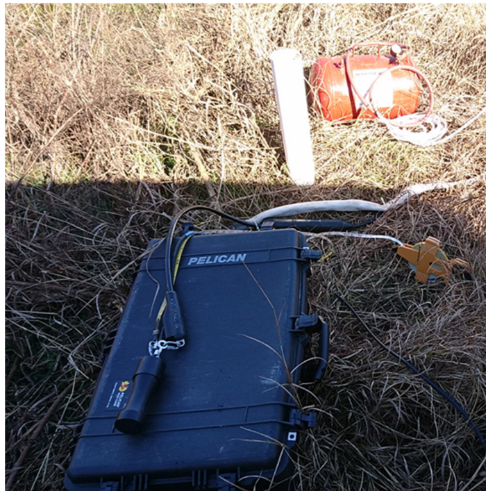
Figure 4-21 Barrel stove source coupled to end of 3D geophone string
