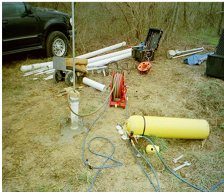
Figure 2-9 Double Hose System for Pneumatic Solenoid SH Source
