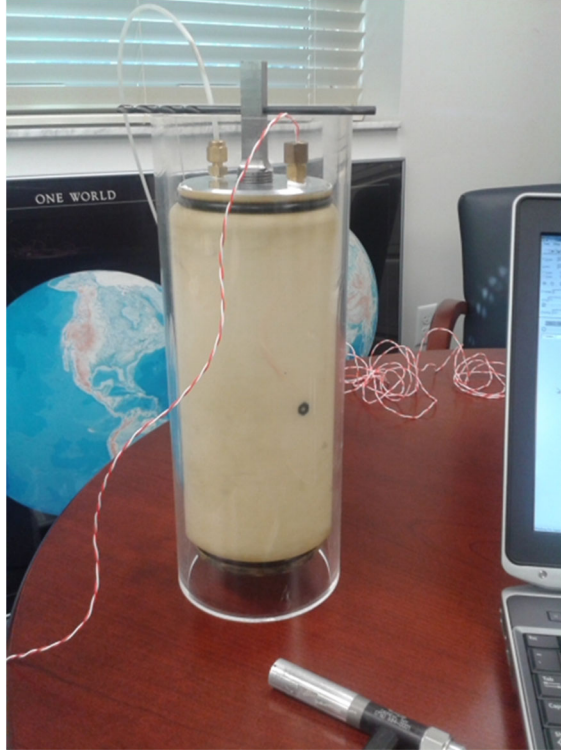
Figure 2-12 Kalinski-Type Bladder Shown Inflated Inside an Acrylic Tube
