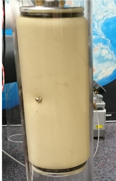
Figure 2-14 Stud and Washer System for Contacting Accelerometer to Borehole Wall
