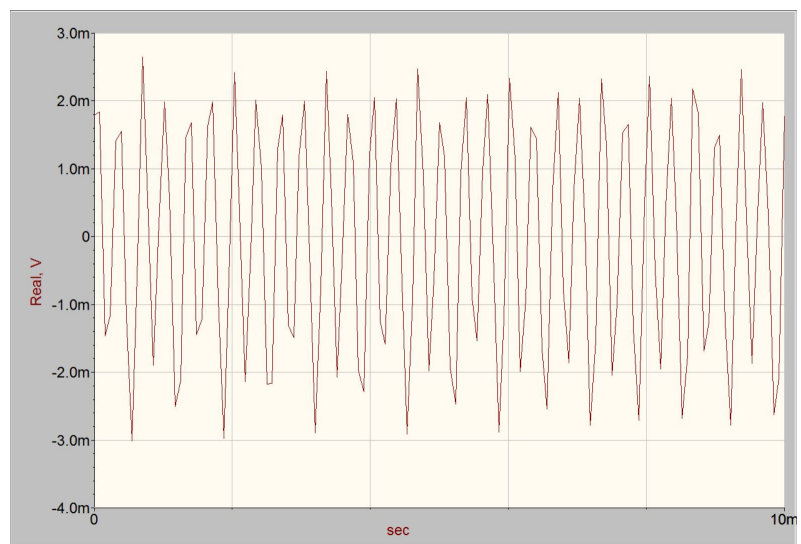
Figure 4-22 Demonstration of barrel stave source vibration in cased borehole
