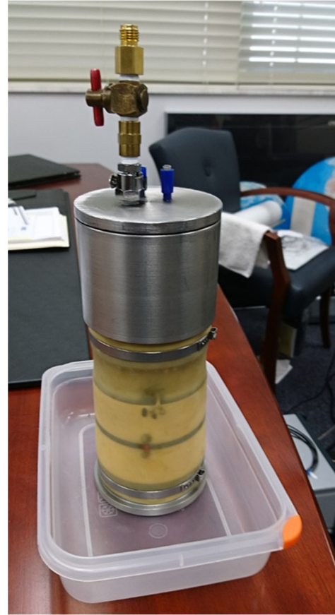
Figure 2-5 Inflatable Canister for Coupling Piezocylinders with Borehole Wall
