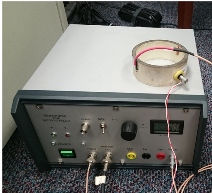
Figure 2-3 Piezoelectric Cylinders and Second Trial of Piezocylinder Amplifier
