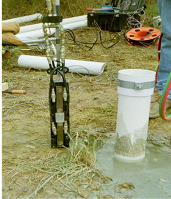
Figure 2-7 Pneumatic Solenoid SH Source
