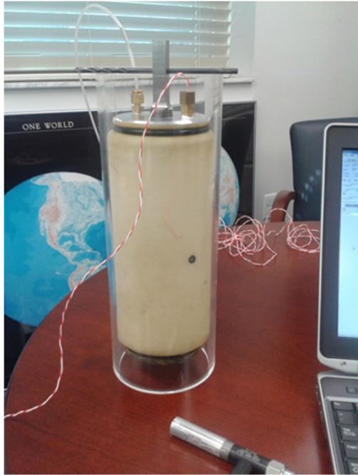
Figure 4-1 Demonstration of borehole receiver coupling system in acrylic tube
