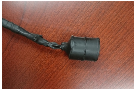
Figure 2-1 Schematic of Thill (1978) Borehole Transducer
