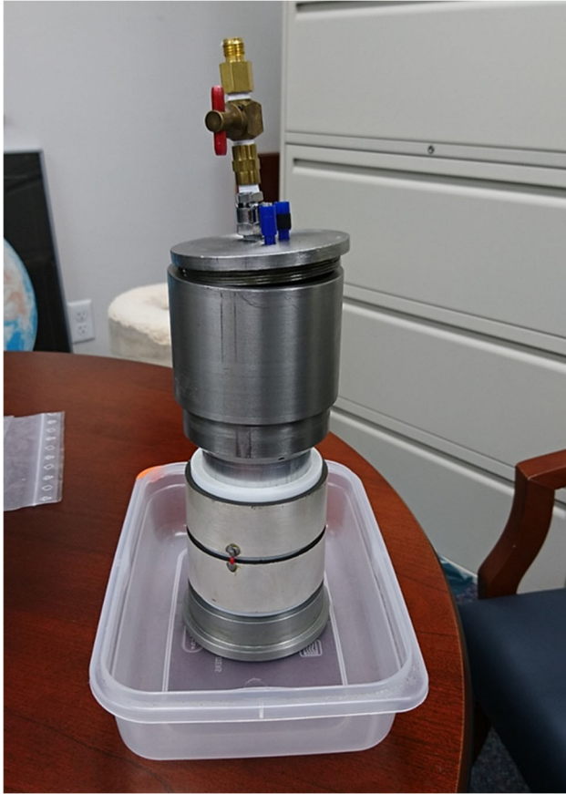
Figure 2-5 Inflatable Canister for Coupling Piezocylinders with Borehole Wall
