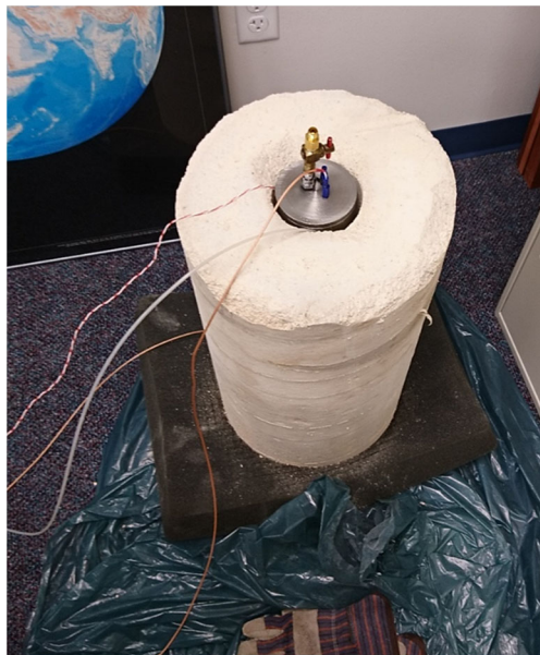
Figure 4-7 Demonstration of inflatable canister/piezocylinder with receiver coupling system in synthetic limerock cylinder
