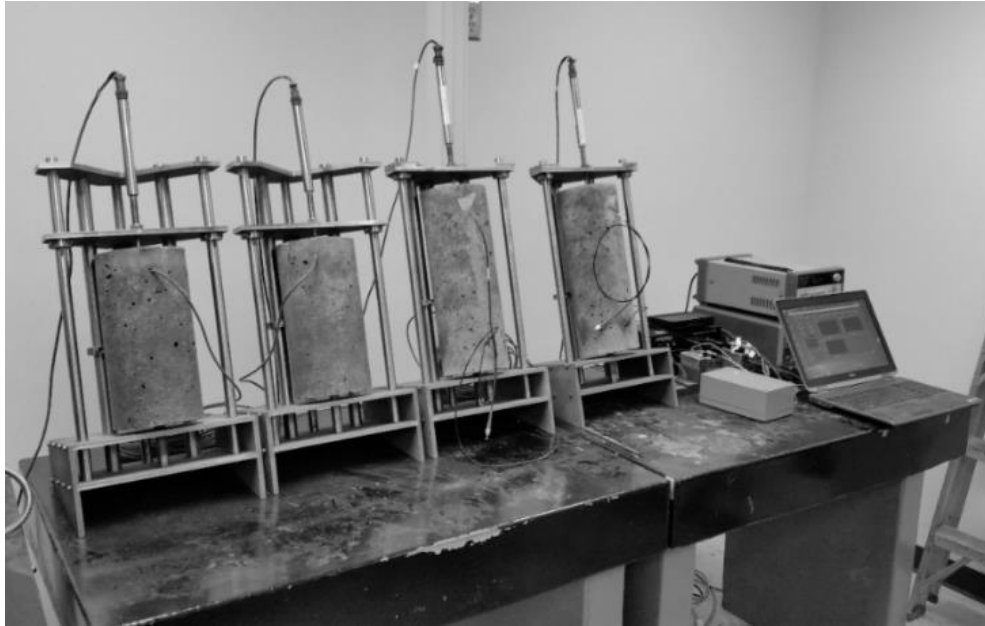
Figure 7-7. Setup for free shrinkage measurement using a LVDT
