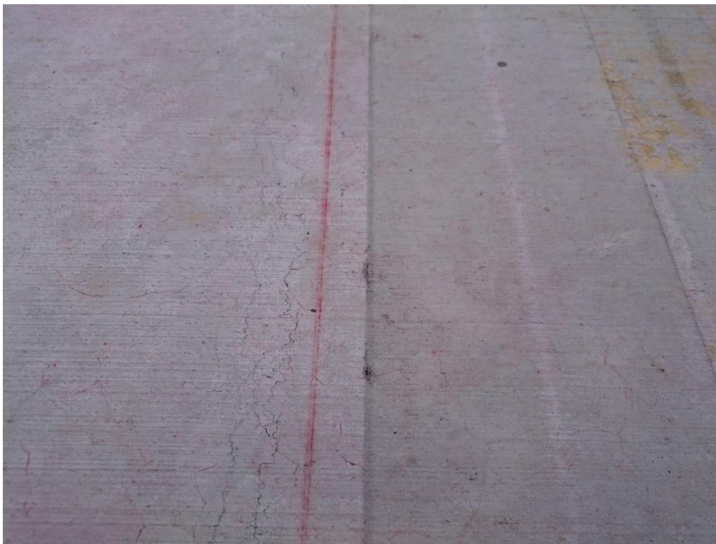
Figure 8-7. Surface of standard-mix slab after HVS loading
