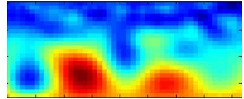
The highly variable top of a limestone layer appears red and orange in this "snapshot" of an underground section, 40 ft wide and 18 ft deep.
