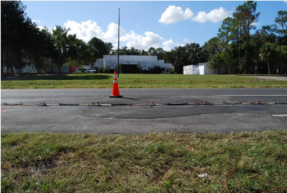
Figure 6.1 US 441 Site: (a) land-streamer and propelled energy generator source, b) repaired sinkhole location
