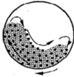
Figure 6-2 Aggregate and Steel Balls Interaction Mechanism in MD Apparatus (Masad et al., 2009)
