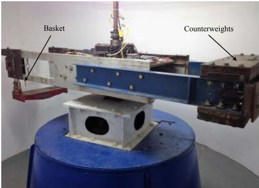
Figure 2.2.1 Geotechnical centrifuge at the University of Florida, Gainesville
