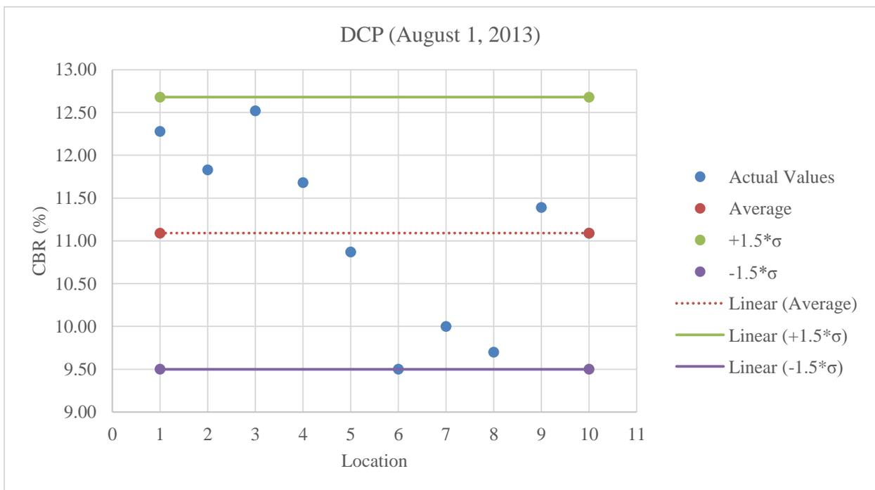
Figure C.46: Plot of DCP values for stabilized subgrade at optimum moisture content
