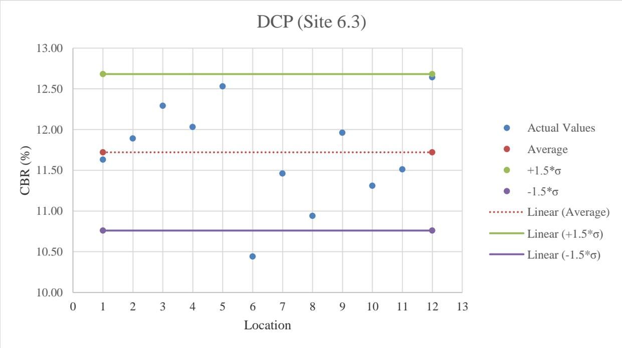
**Figure E.64:** DCP testing results on A-3 material
