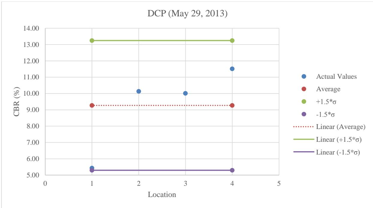
Figure B.21: DCP testing on A-2-4 below optimum moisture content
