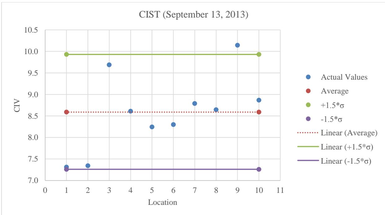
**Figure C.54:** Plot of CIST values for stabilized subgrade below optimum moisture content
