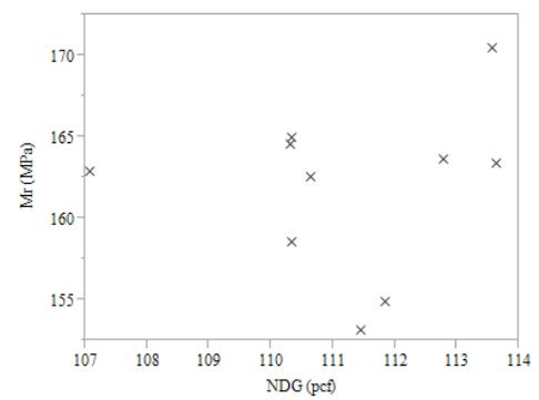
**Figure F.5:** Scatterplot of laboratory resilient modulus vs. NDG measurements (pcf)
