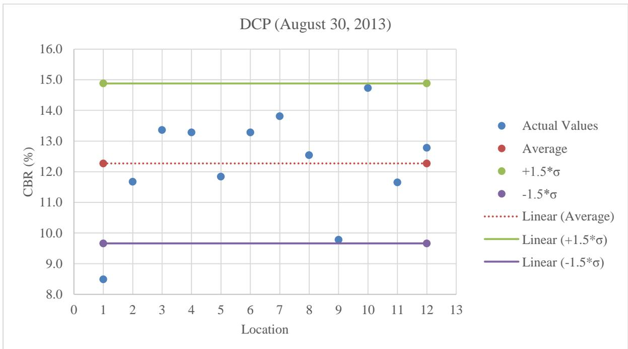
Figure C.10: Plot of DCP values for A-3 at 7% less than optimum moisture content
