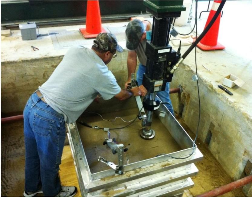
**Figure 3.18:** Photograph of 6-in. diameter PLT in test box placed in east test pit
