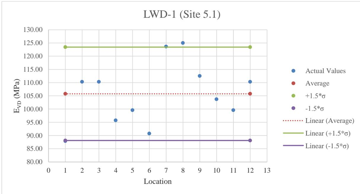
Figure E.41: LWD-1 testing results on limerock material
