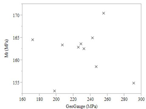
**Figure F.4:** Scatterplot of laboratory resilient modulus vs. GeoGauge measurements (MPa)
