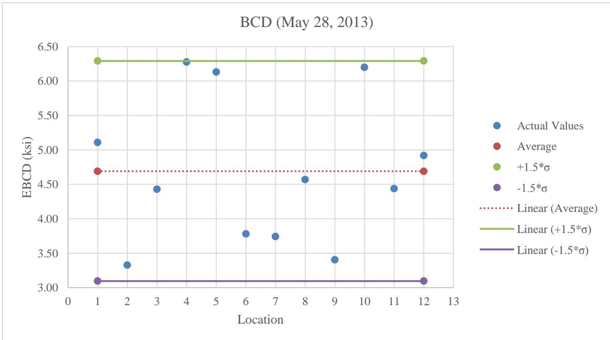
Figure B.6: BCD testing on stabilized subgrade above optimum moisture content
