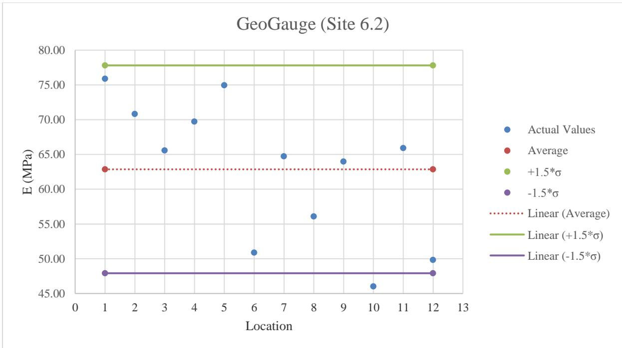
**Figure E.59:** GeoGauge testing results on A-3 material
