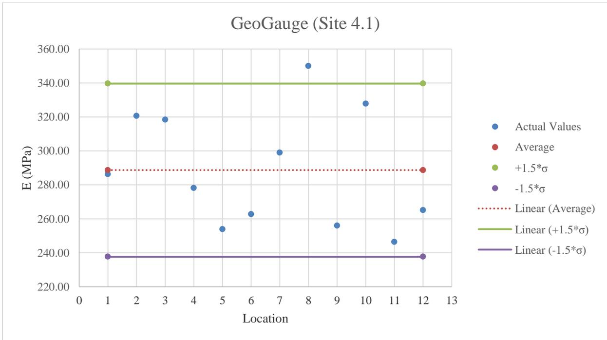
**Figure E.31:** GeoGauge testing results on stabilized subgrade
