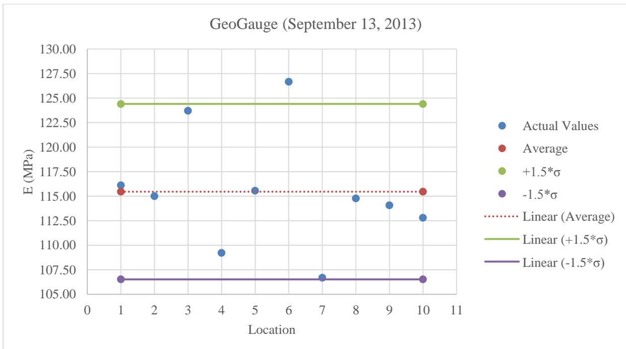
Figure C.52: Plot of GeoGauge values for stabilized subgrade below optimum moisture content
