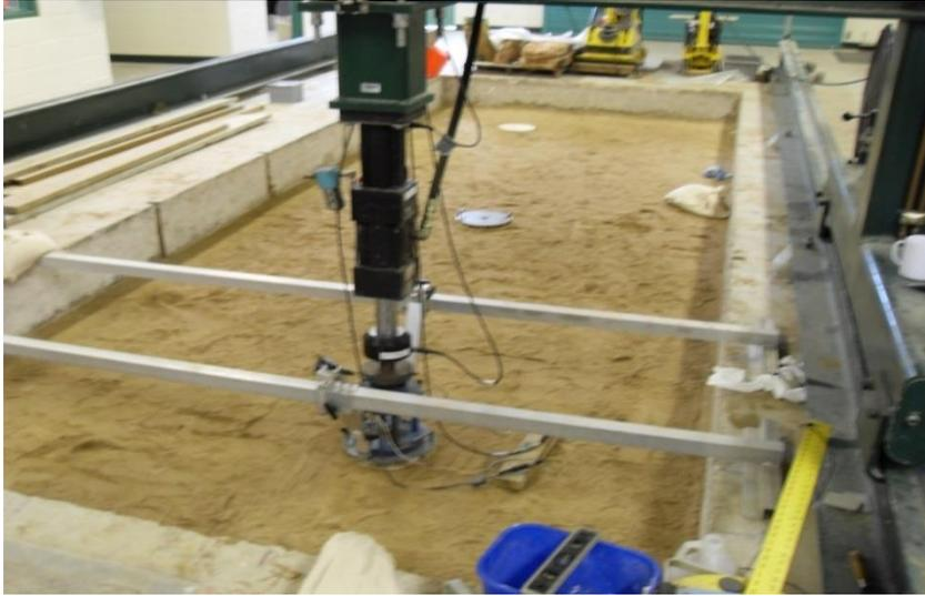
**Figure 3.16:** Photograph of east test pit and 12-in. static PLT
