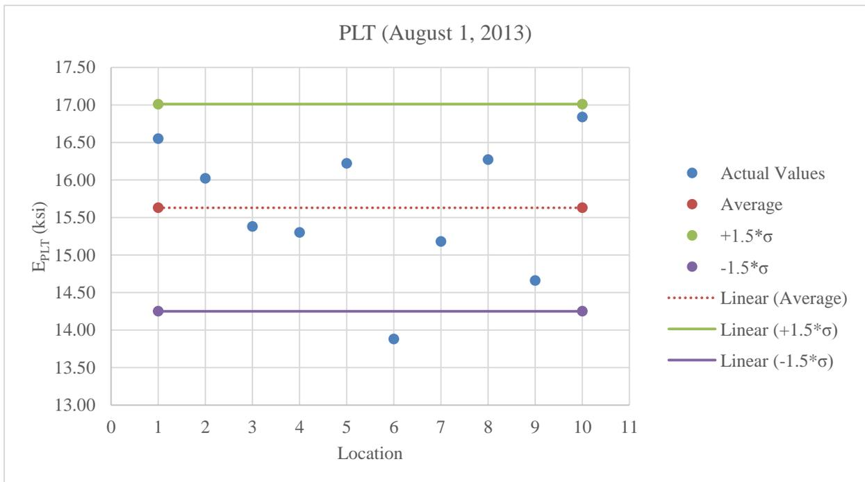
**Figure C.50:** Plot of PLT values for stabilized subgrade at optimum moisture content
