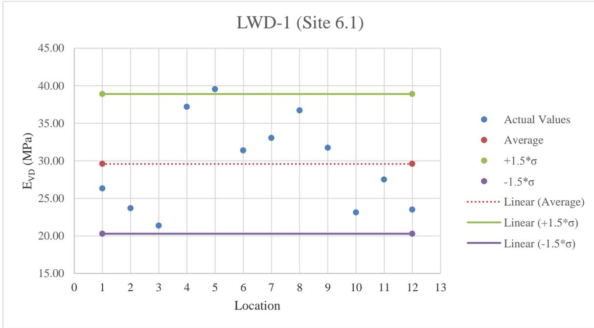
Figure E.53: LWD-1 testing results on A-3 material
