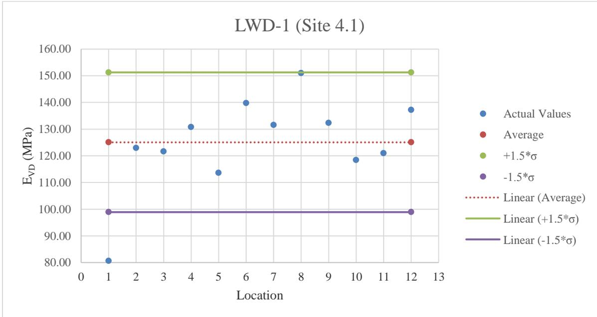
Figure E.29: LWD-1 testing results on stabilized subgrade
