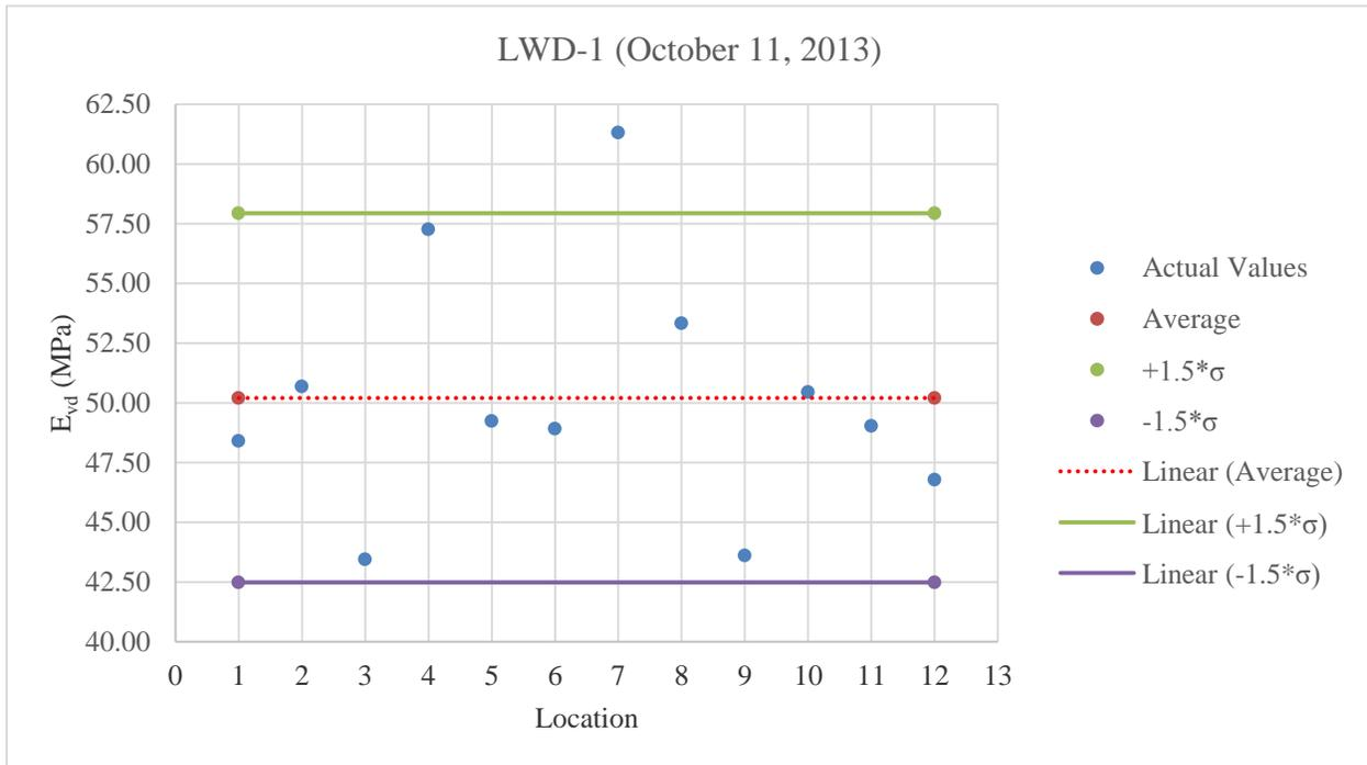
Figure C.15: Plot of LWD-1 values for A-2-4 low fines at optimum moisture content
