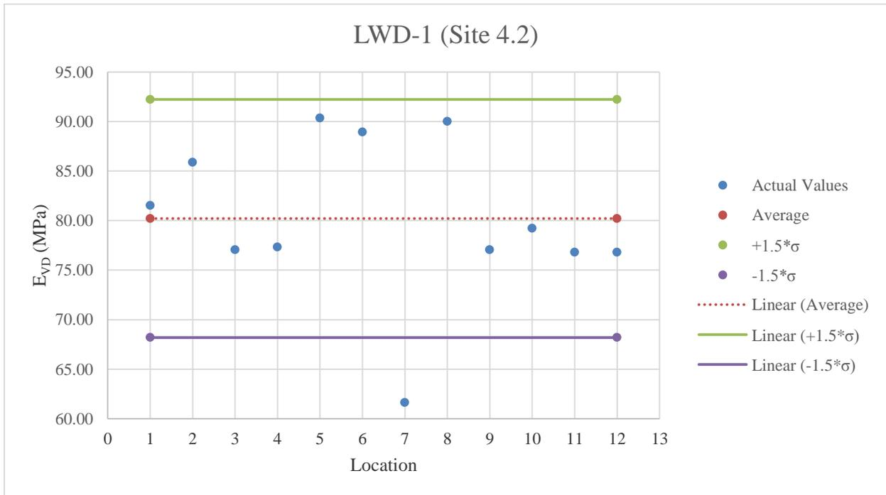
**Figure E.34:** LWD-1 testing results on stabilized subgrade
