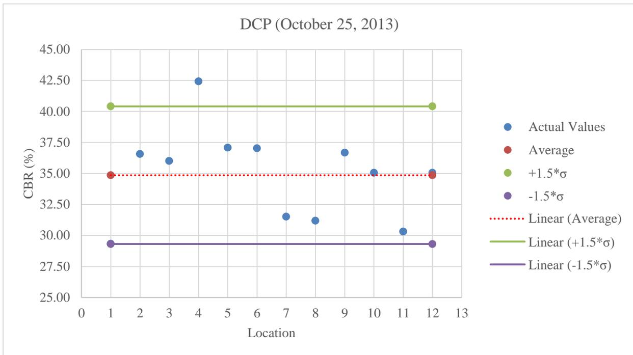
**Figure C.25:** Plot of DCP values for A-2-4 low fines at 6% less than optimum moisture content
