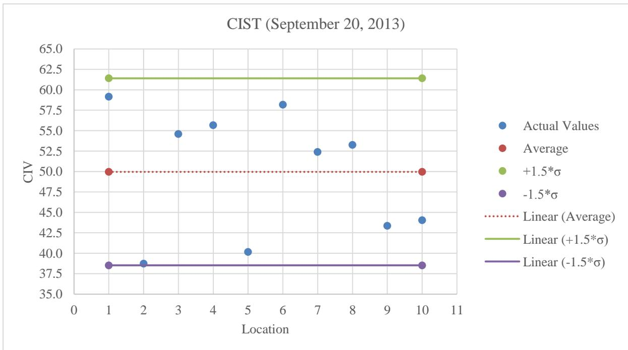
**Figure C.40:** Plot of CIST values for limerock at 3% less than optimum moisture content
