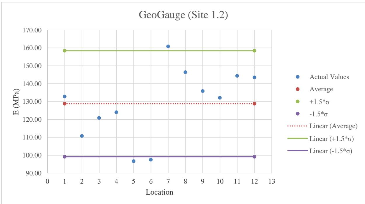
**Figure E.6:** GeoGauge testing results on GAB material
