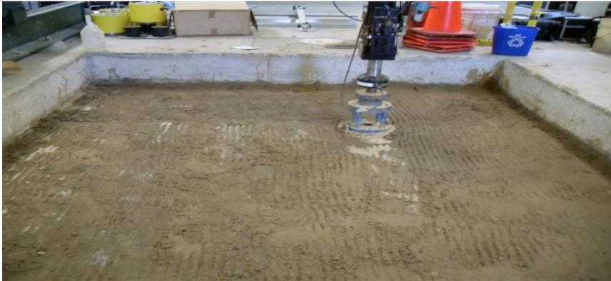
**Figure 3.17:** Photograph of east test pit and static PLT
