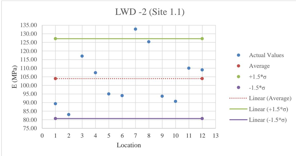
Figure E.1: LWD-2 testing results on GAB material
