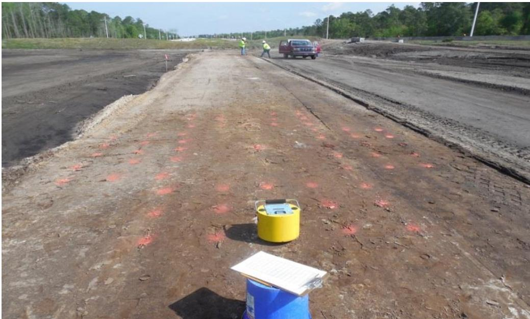
**Figure 5.17:** Project Site #3 SR-9B - Photograph of layout, typical at three stations (GeoGauge shown)
