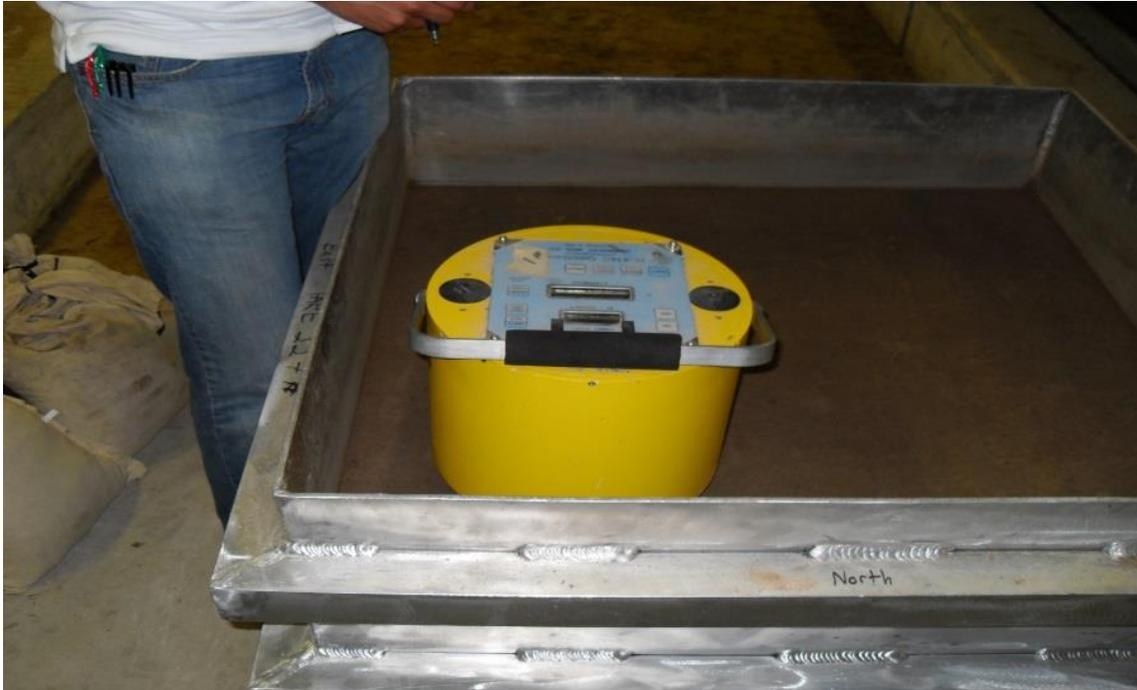
**Figure 3.9:** Photograph of GeoGauge in test box
