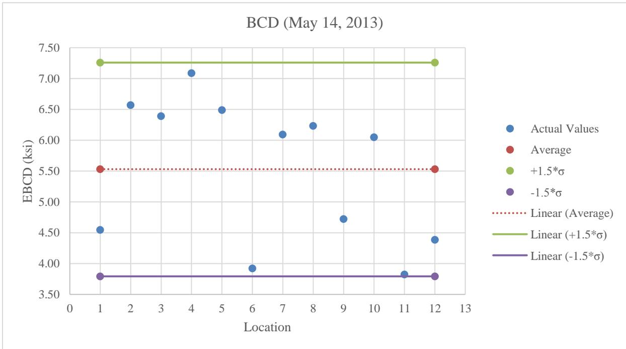
**Figure B.4:** BCD testing on stabilized subgrade at optimum moisture content
