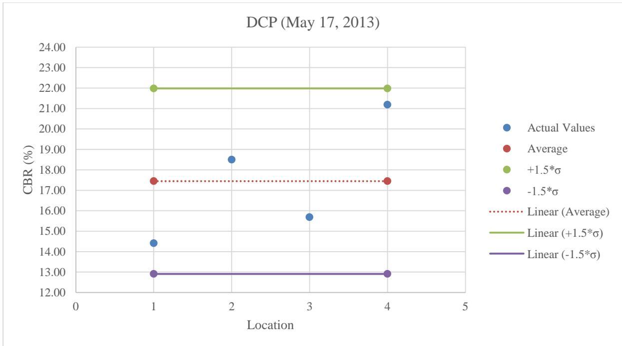
**Figure B.19:** DCP testing on stabilized subgrade below optimum moisture content
