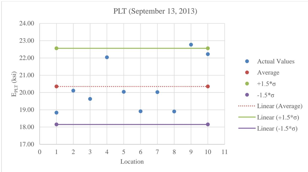
**Figure C.57:** Plot of PLT values for stabilized subgrade below optimum moisture content
