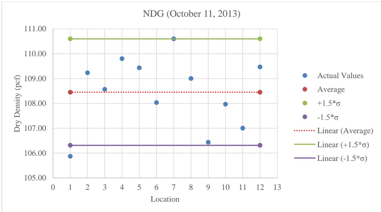
Figure C.19: Plot of NDG values for A-2-4 low fines at optimum moisture content
