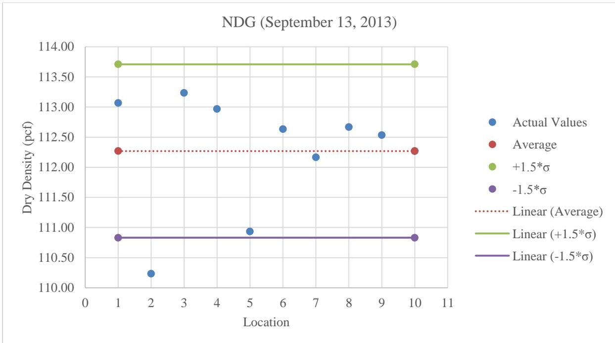
**Figure C.55:** Plot of NDG values for stabilized subgrade below optimum moisture content
