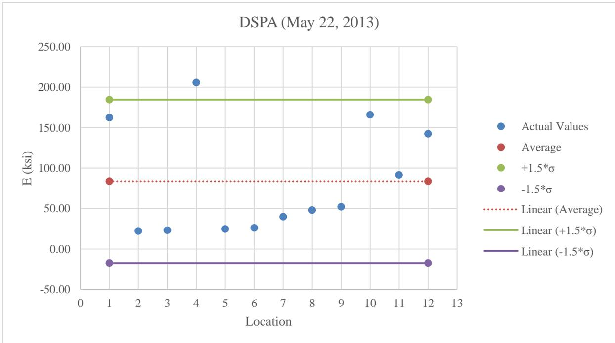
**Figure B.14:** DSPA testing on stabilized subgrade above optimum moisture content
