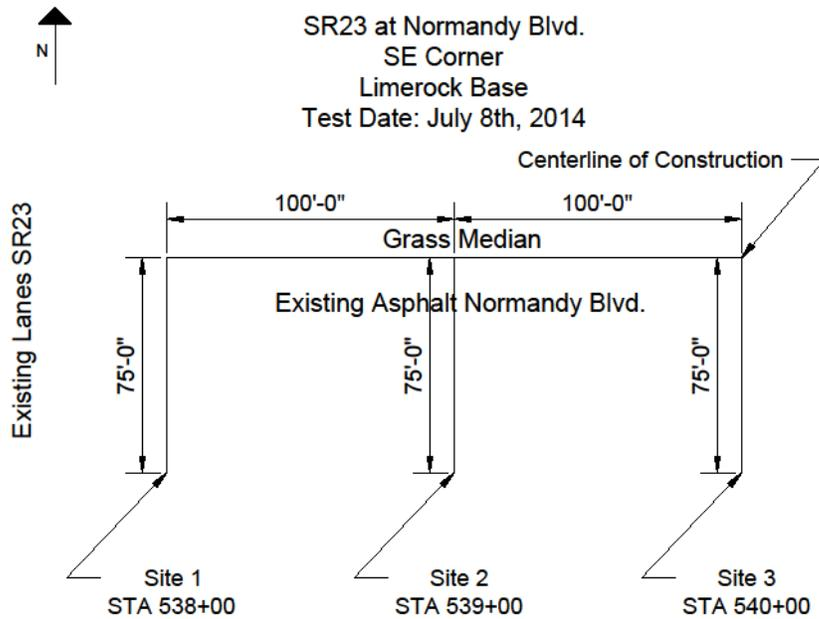
**Figure 5.32:** Project Site #5 SR-23 limerock base - Test site location sketch
