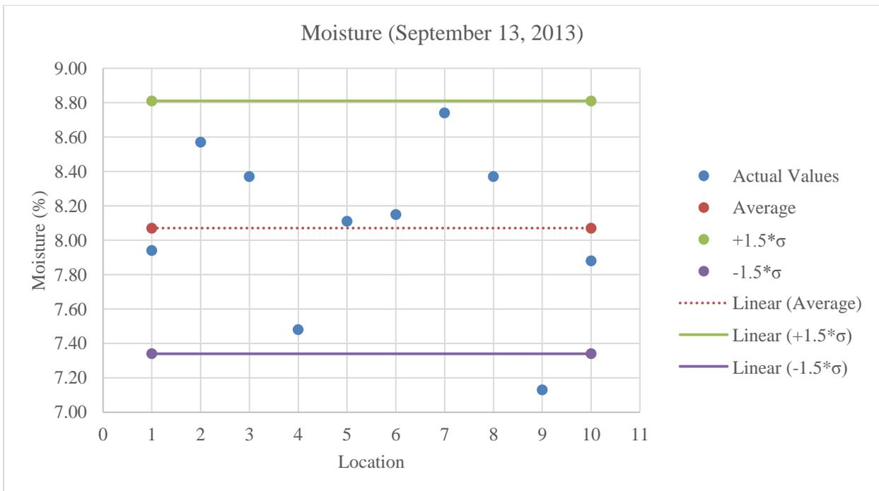
**Figure C.56:** Plot of moisture values for stabilized subgrade
