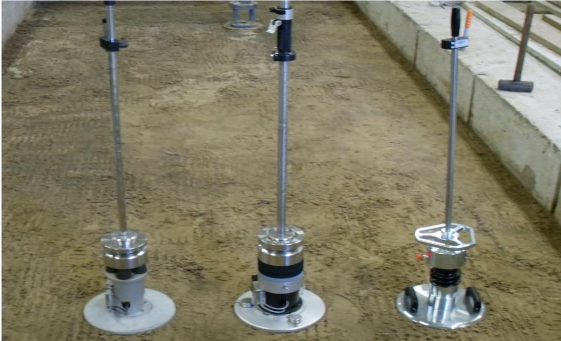
**Figure 3.5:** Photograph of LWD devices in east test pit
