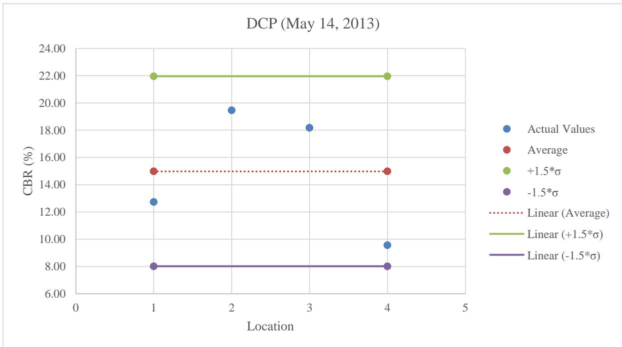
Figure B.18: DCP testing on stabilized subgrade at optimum moisture content
