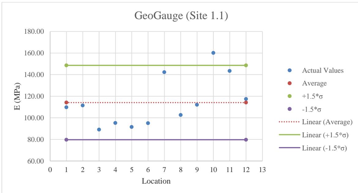
Figure E.2: GeoGauge testing results on GAB material
