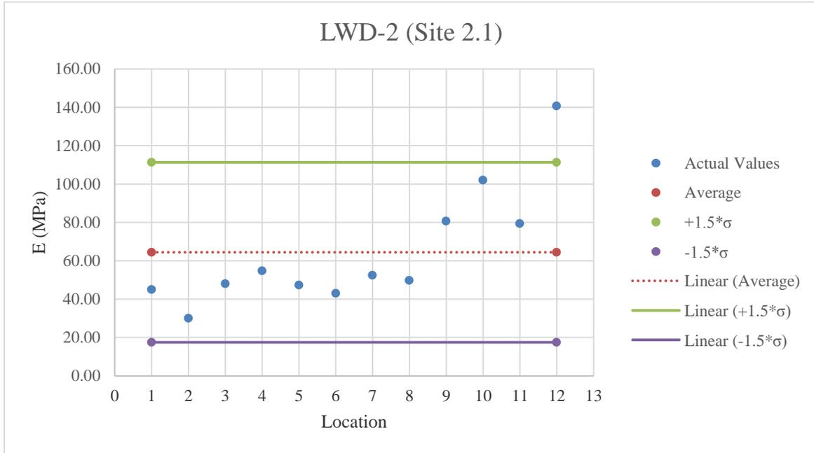
Figure E.13: LWD-2 testing results on A-2-4 material
