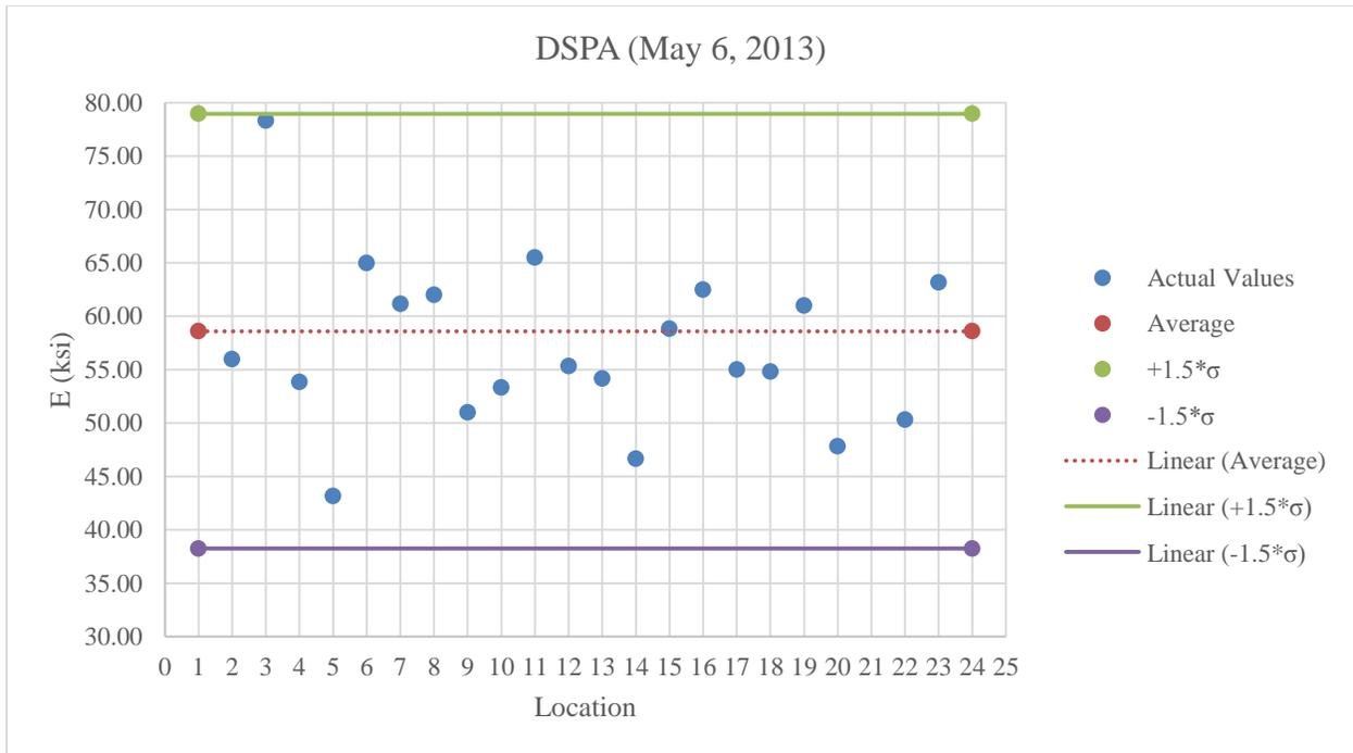
**Figure B.11:** DSPA testing on A-2-4 below optimum moisture content
