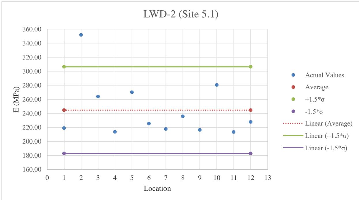
Figure E.42: LWD-2 testing results on limerock material
