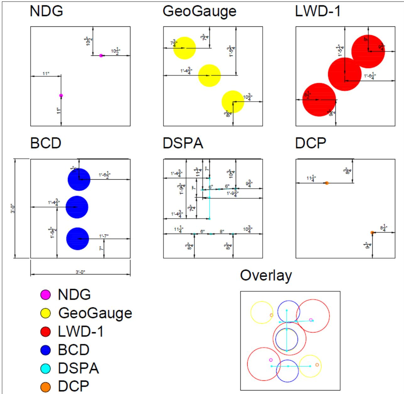
**Figure 3.10:** Testing device orientation in the test box
