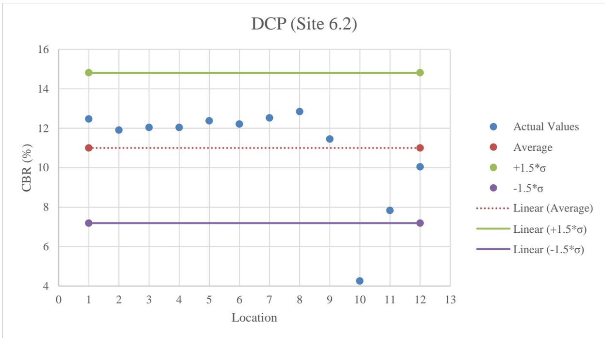
**Figure E.60:** DCP testing results on A-3 material
