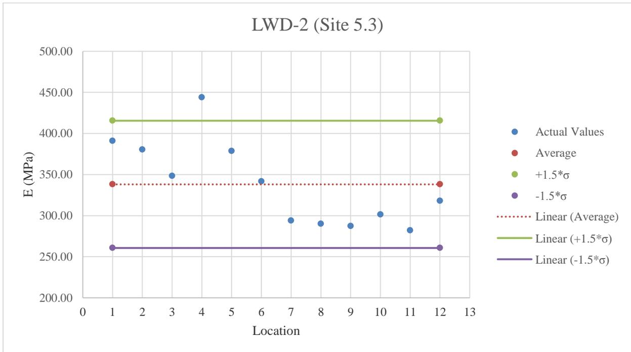
**Figure E.50:** LWD-2 testing results on limerock material
