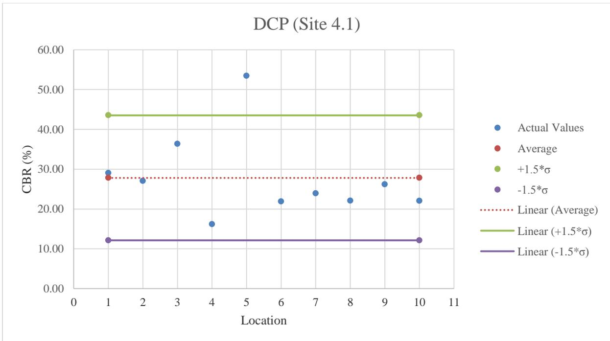
**Figure E.32:** DCP testing results on stabilized subgrade
