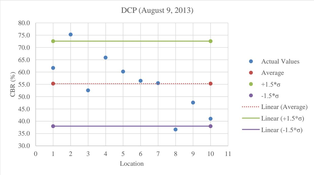
Figure C.32: Plot of DCP values for limerock at optimum moisture content
