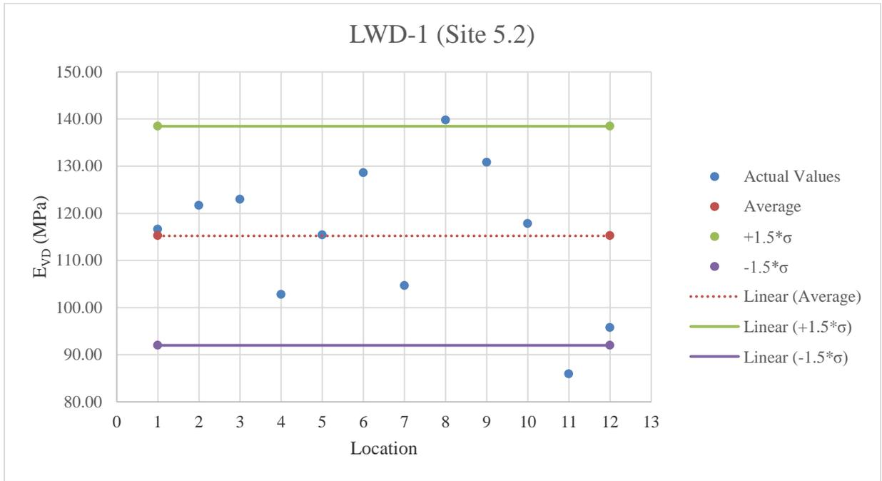
**Figure E.45:** LWD-1 testing results on limerock material
