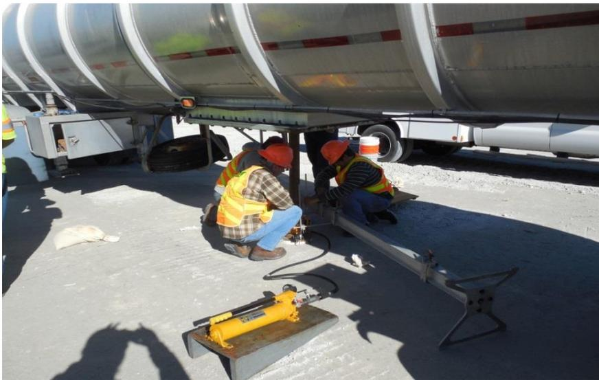
**Figure 5.7:** Project Site #1 I-95 - Photograph of 12-in. diameter static PLT
