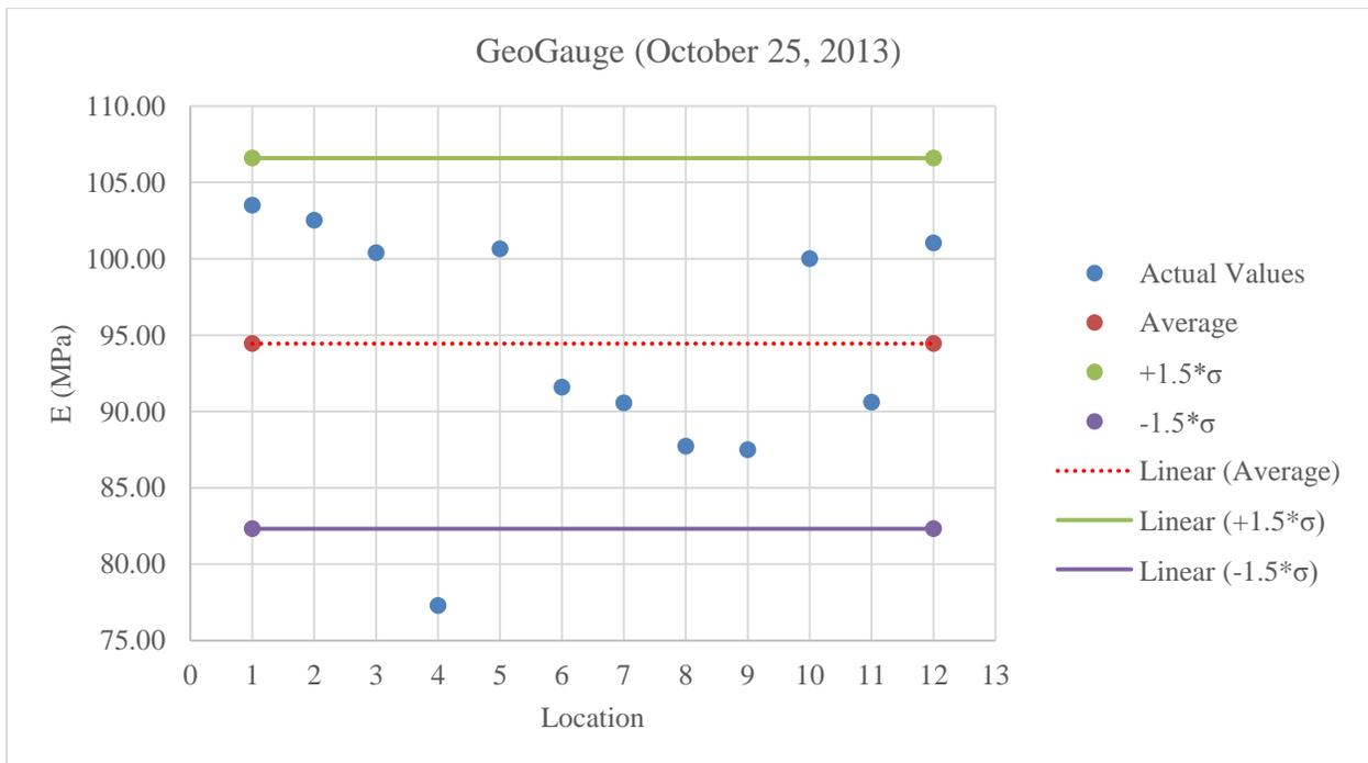
**Figure C.24:** Plot of GeoGauge values for A-2-4 low fines at 6% less than optimum moisture content
