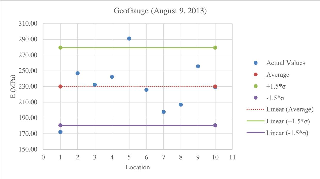
Figure C.31: Plot of GeoGauge values for limerock at optimum moisture content
