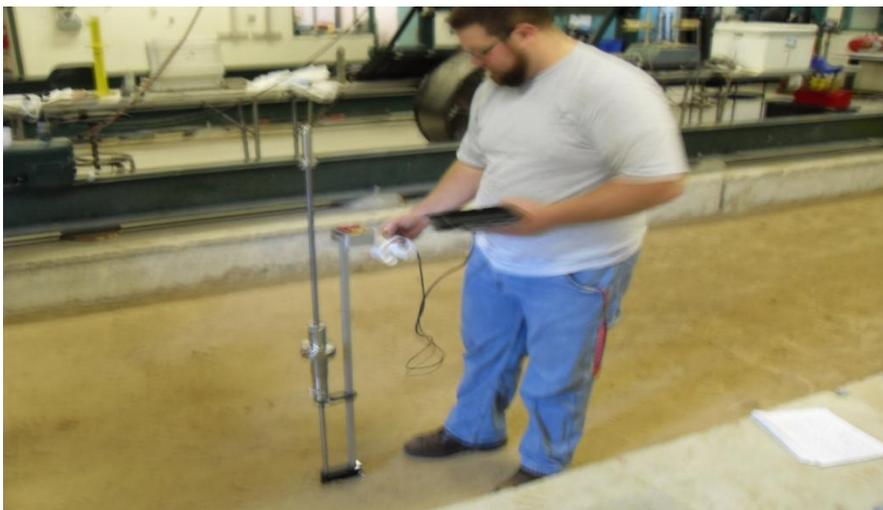
**Figure 3.15:** Photograph of east test pit and DCP
