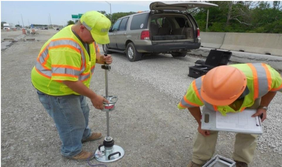
**Figure 7.2:** Photograph of INDOT LWD deflection measurement on #53 aggregate base
