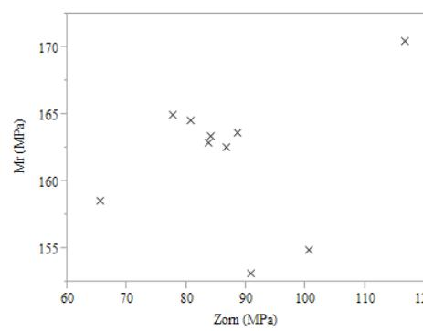
**Figure F.7:** Scatterplot of laboratory resilient modulus vs. LWD-1 measurements (MPa)
