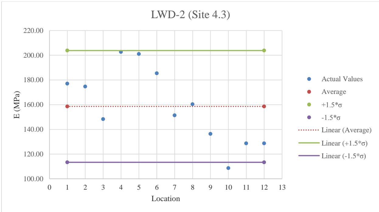
**Figure E.39:** LWD-2 testing results on stabilized subgrade
