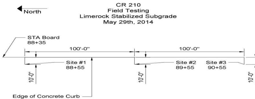
**Figure 5.29:** Project Site #4 CR-210 - Test location sketch
