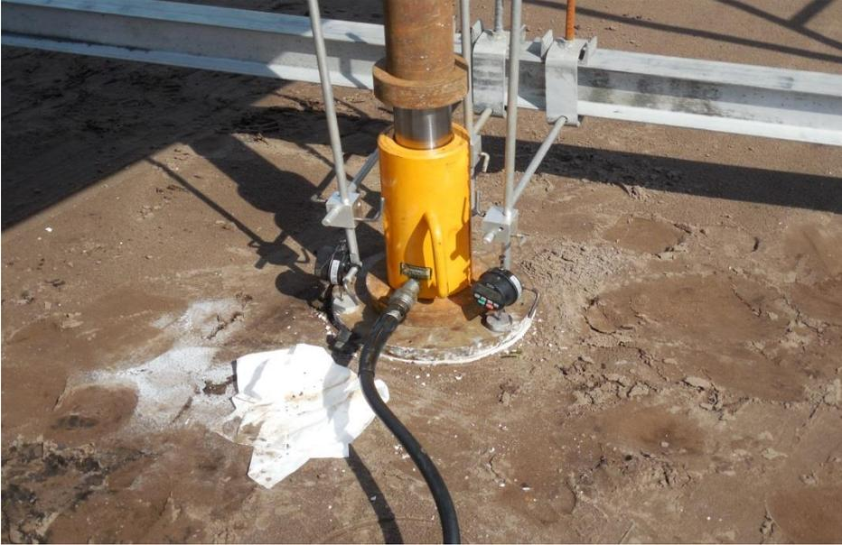
**Figure 5.36:** Project Site #6 SR-23 A-3 embankment - Photograph of PLT
