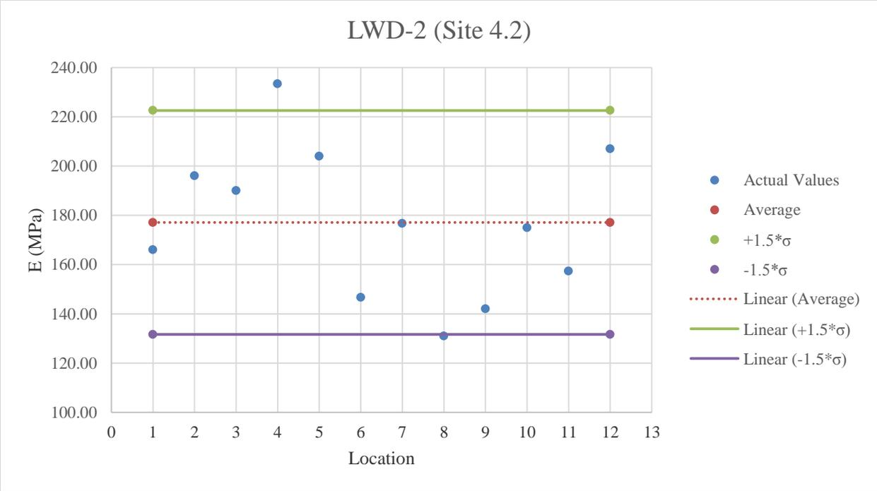
**Figure E.35:** LWD-2 testing results on stabilized subgrade
