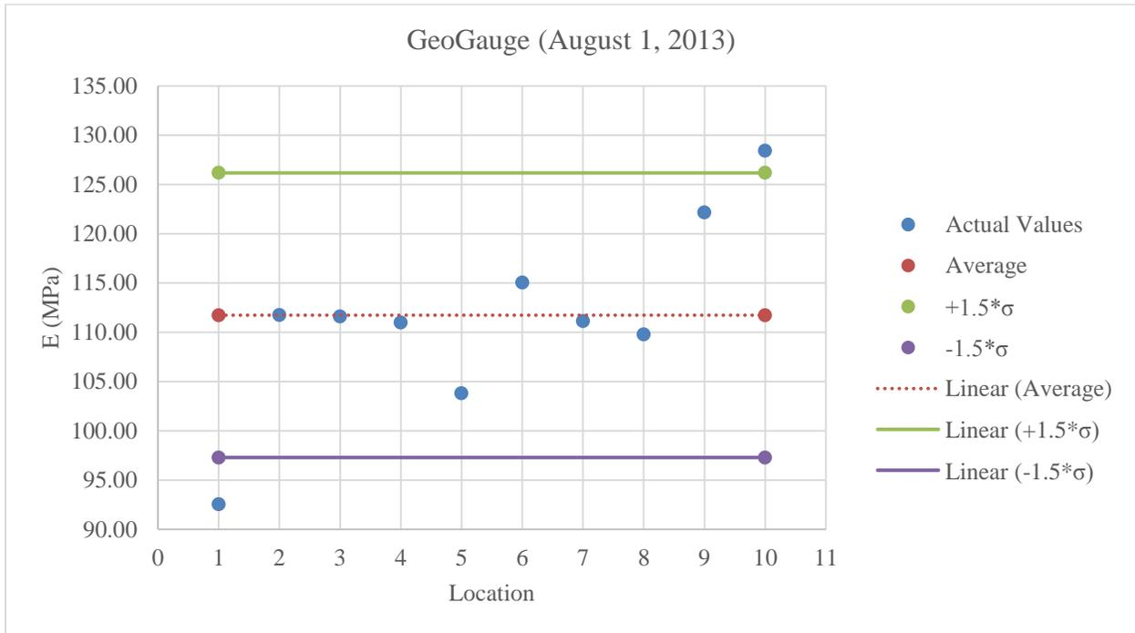
Figure C.45: Plot of GeoGauge values for stabilized subgrade at optimum moisture content
