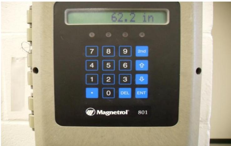
**Figure 3.12:** Photograph of east test pit Magnetrol water level control system
