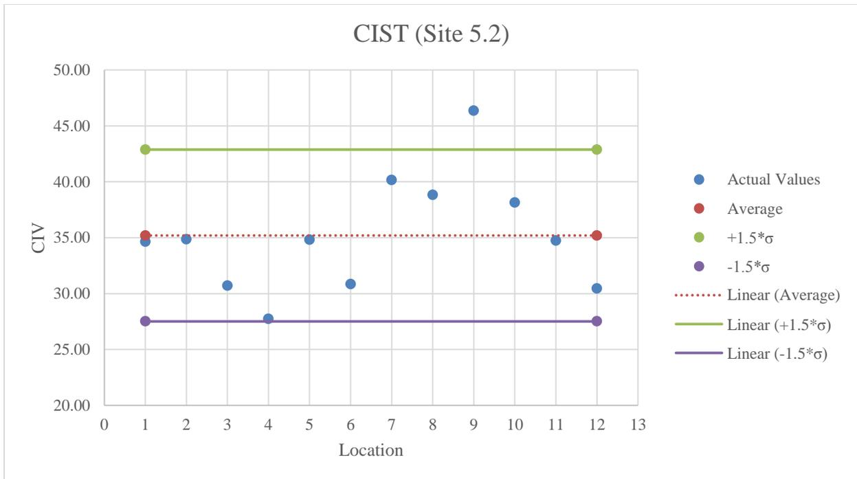
**Figure E.48:** CIST testing results on limerock material
