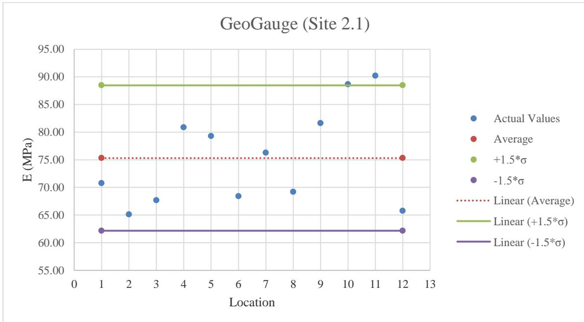
Figure E.14: GeoGauge testing results on A-2-4 material
