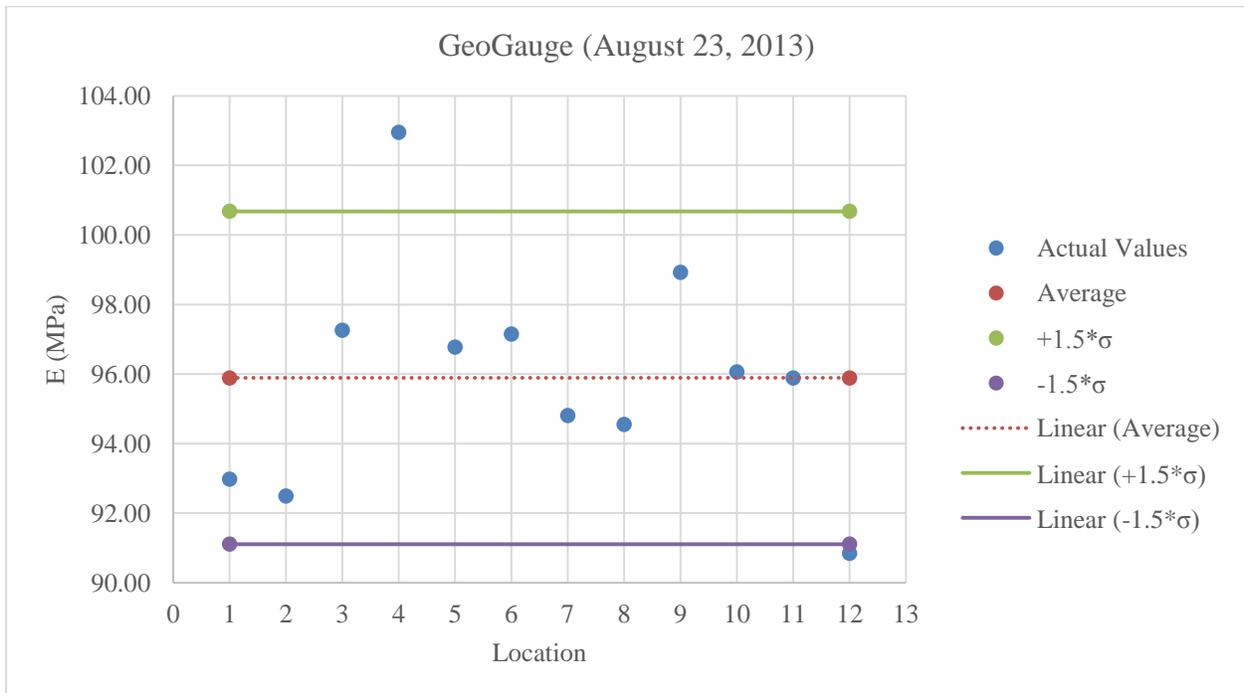
**Figure C.2:** Plot of GeoGauge values for A-3 at optimum moisture content
