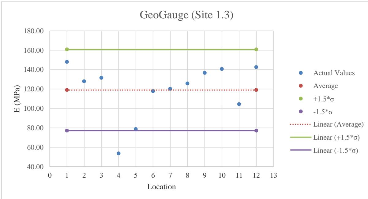
**Figure E.10:** GeoGauge testing results on GAB material
