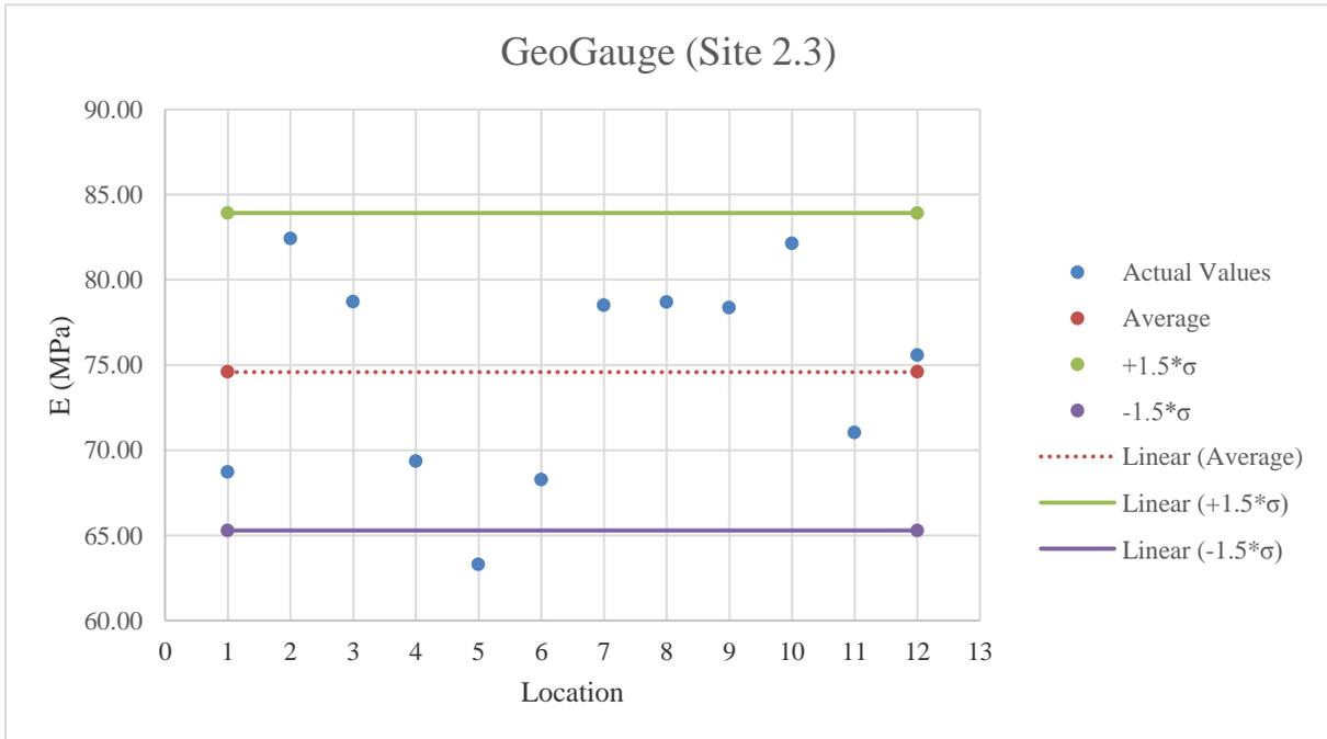
**Figure E.20:** GeoGauge testing results on A-2-4 material
