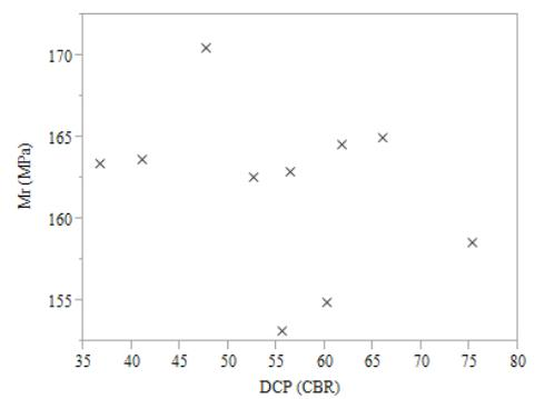
**Figure F.2:** Scatterplot of laboratory resilient modulus vs. DCP measurements (CBR)
