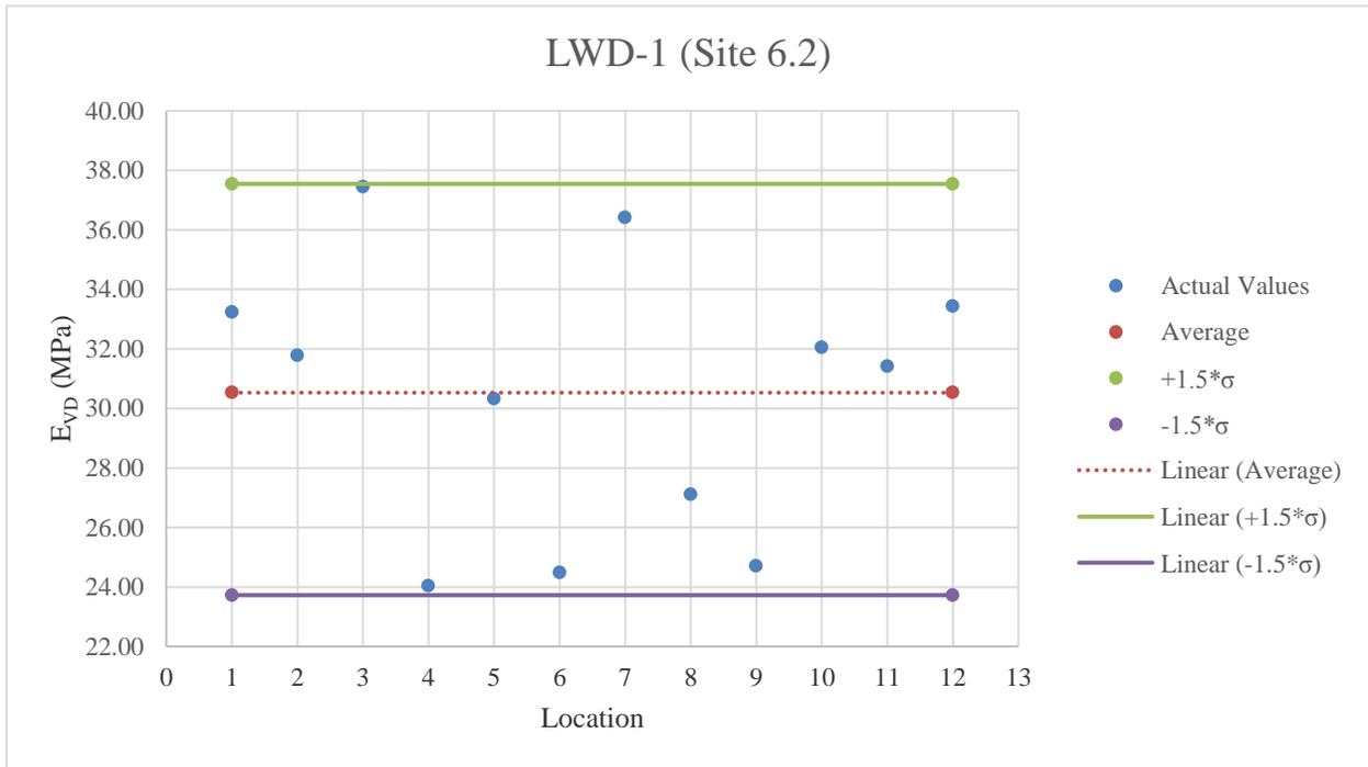
**Figure E.57:** LWD-1 testing results on A-3 material
