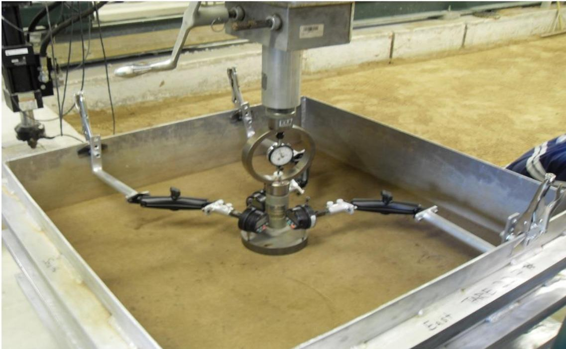
**Figure 3.8:** Photograph of mini-PLT in test box with modified clamping devices
