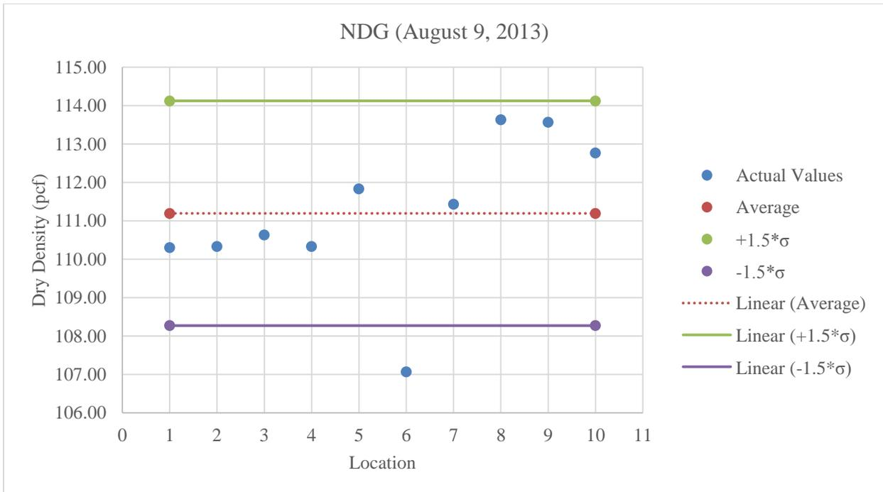
**Figure C.34:** Plot of NDG values for limerock at optimum moisture content
