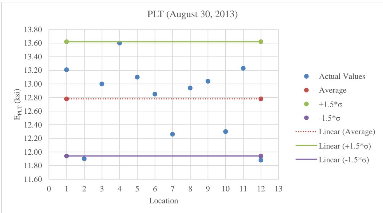
Figure C.14: Plot of PLT values for A-3 at 7% less than optimum moisture content
