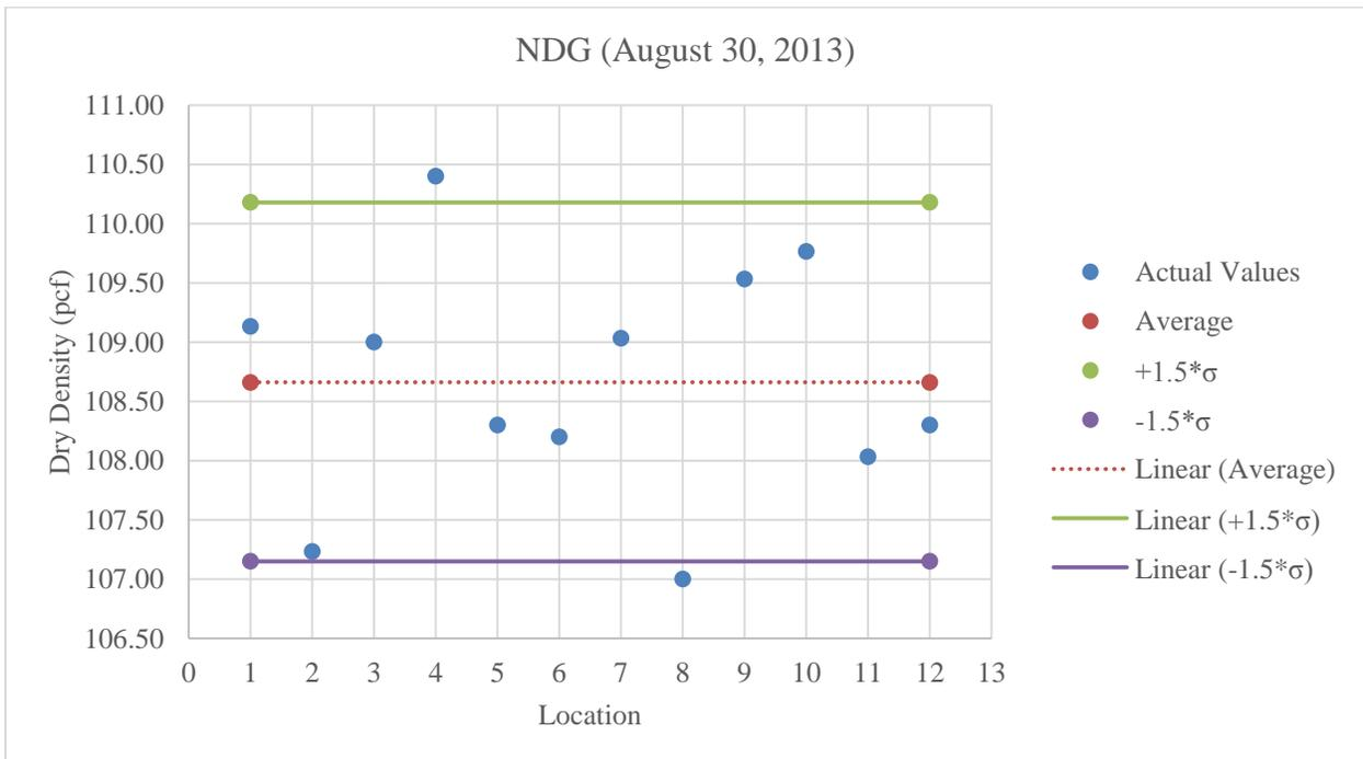
**Figure C.12:** Plot of NDG values for A-3 at 7% less than optimum moisture content
