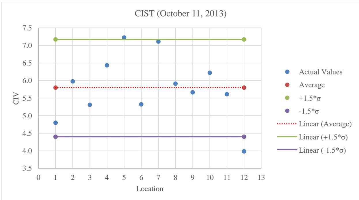
**Figure C.18:** Plot of CIST values for A-2-4 low fines at optimum moisture content
