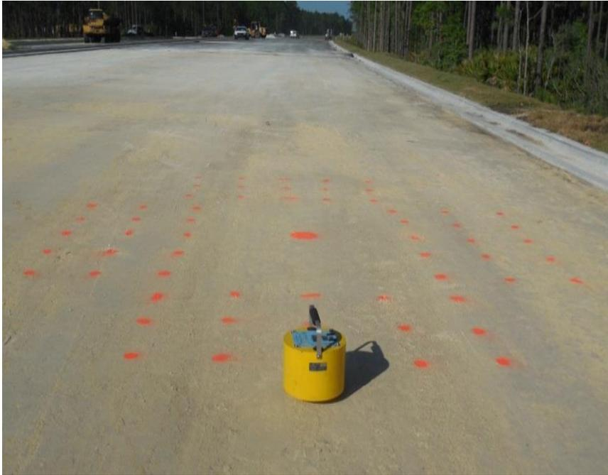
**Figure 5.25:** Project Site #4 CR-210 - Photograph of 12 test locations per device (GeoGauge shown)
