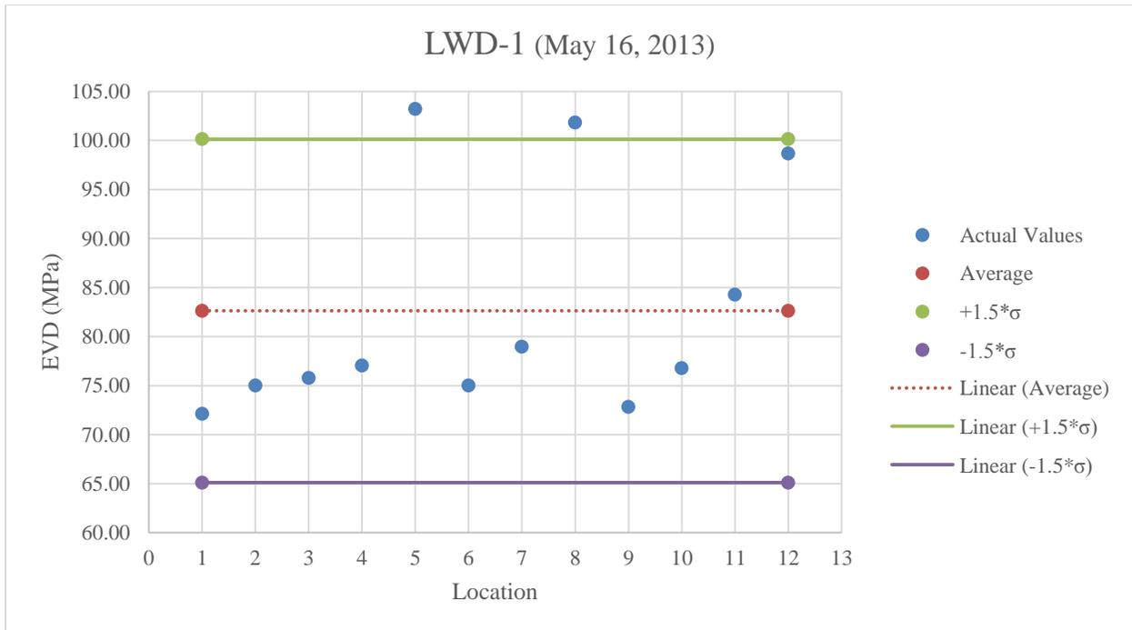
**Figure B.33:** LWD-1 testing on stabilized subgrade below optimum moisture content
