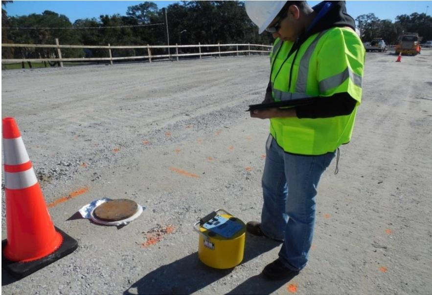
**Figure 5.4:** Project Site #1 I-95 - Photograph of GeoGauge and plate load testing
