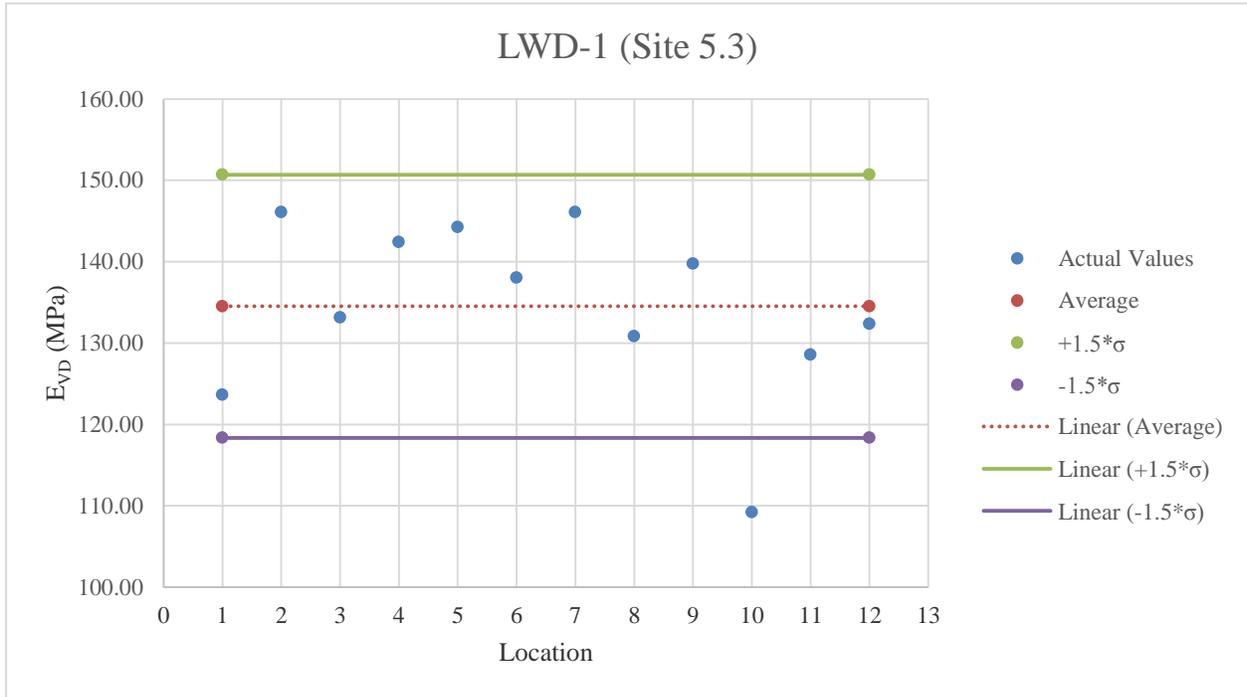
**Figure E.49:** LWD-1 testing results on limerock material
