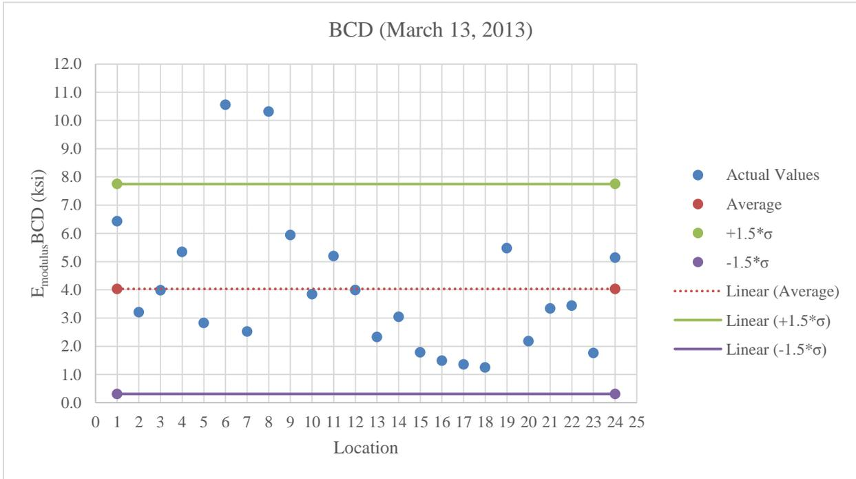
**Figure B.1:** BCD testing on A-3 at optimum moisture content (In kilopounds per square inch, *ksi*)
