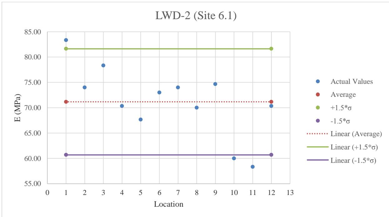
Figure E.54: LWD-2 testing results on A-3 material
