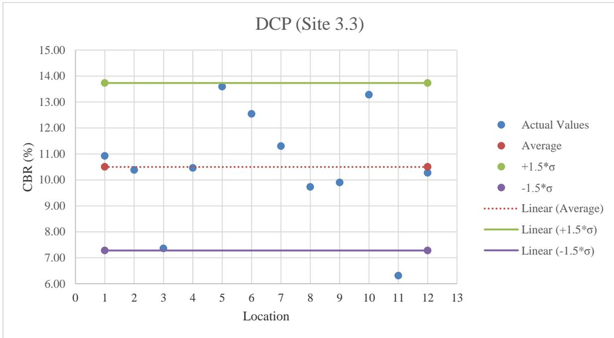
Figure E.27: DCP testing results on A-3 material
