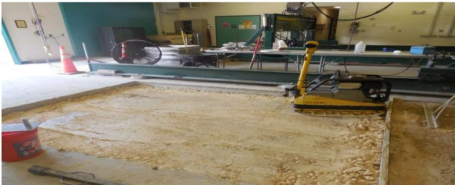
**Figure 4.1:** Photograph of east test pit south limerock base compaction
