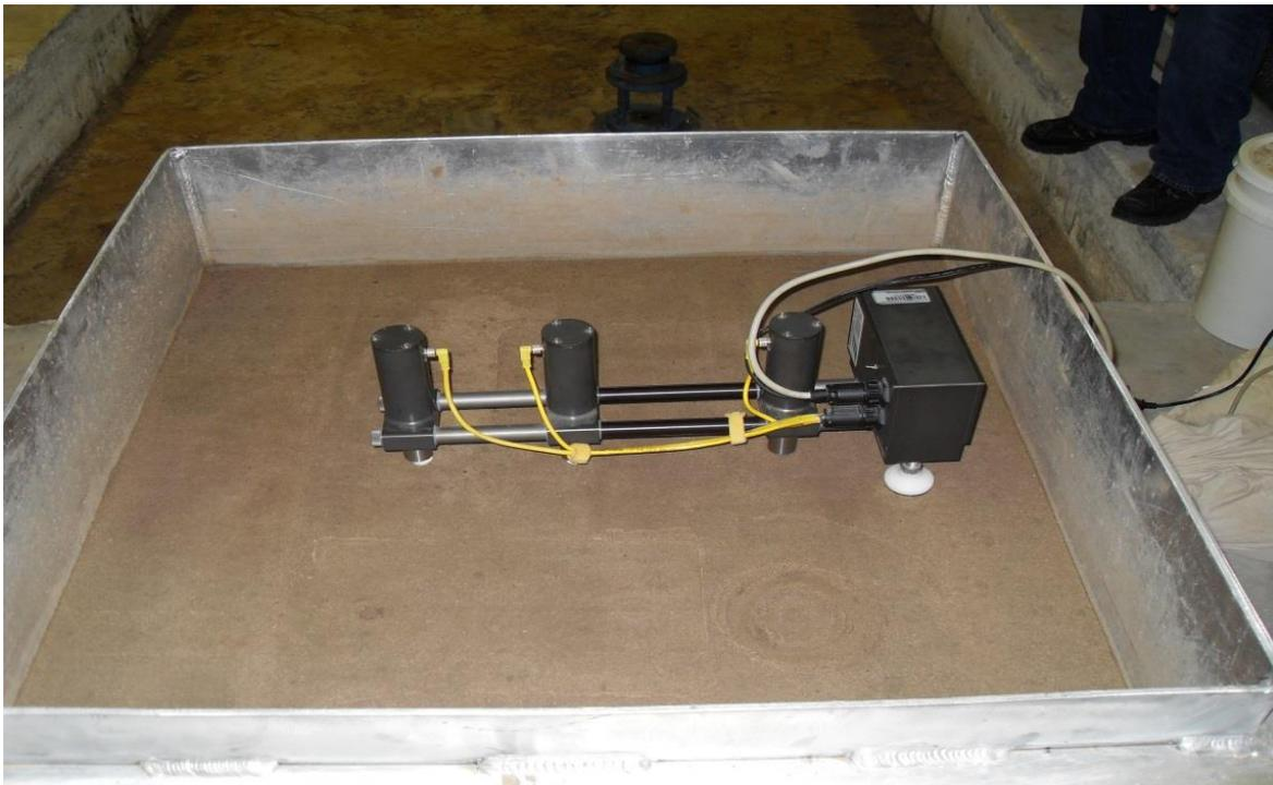
**Figure 3.6:** Photograph of DSPA in test box upper lift
