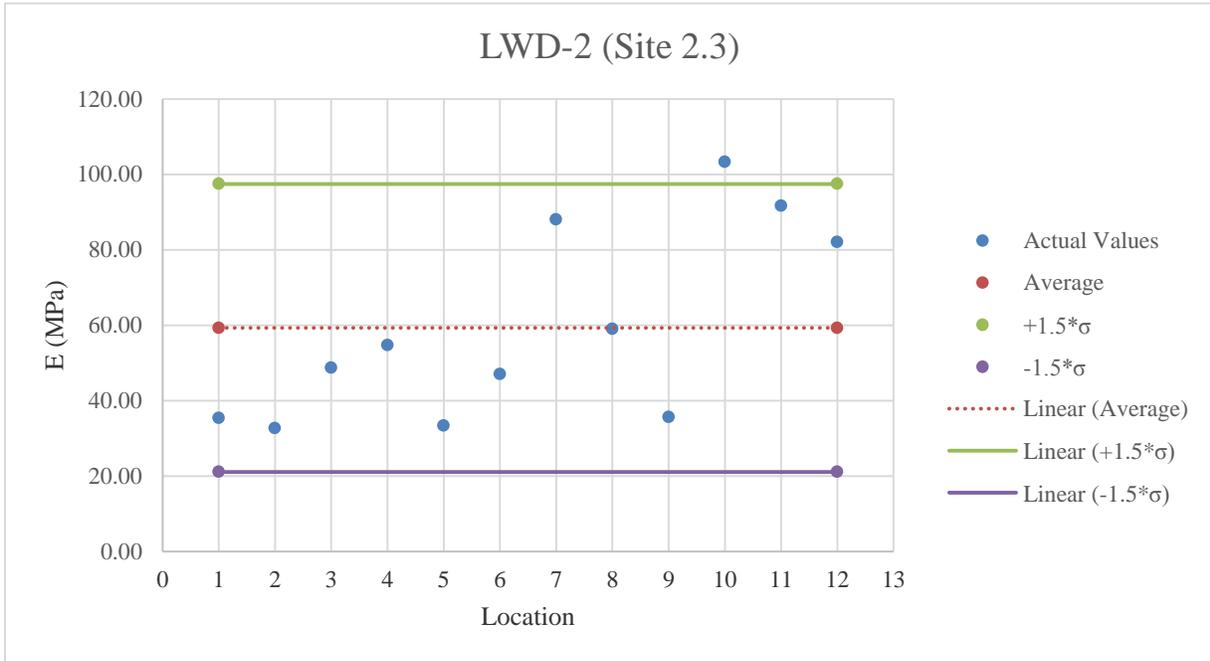
**Figure E.19:** LWD-2 testing results on A-2-4 material
