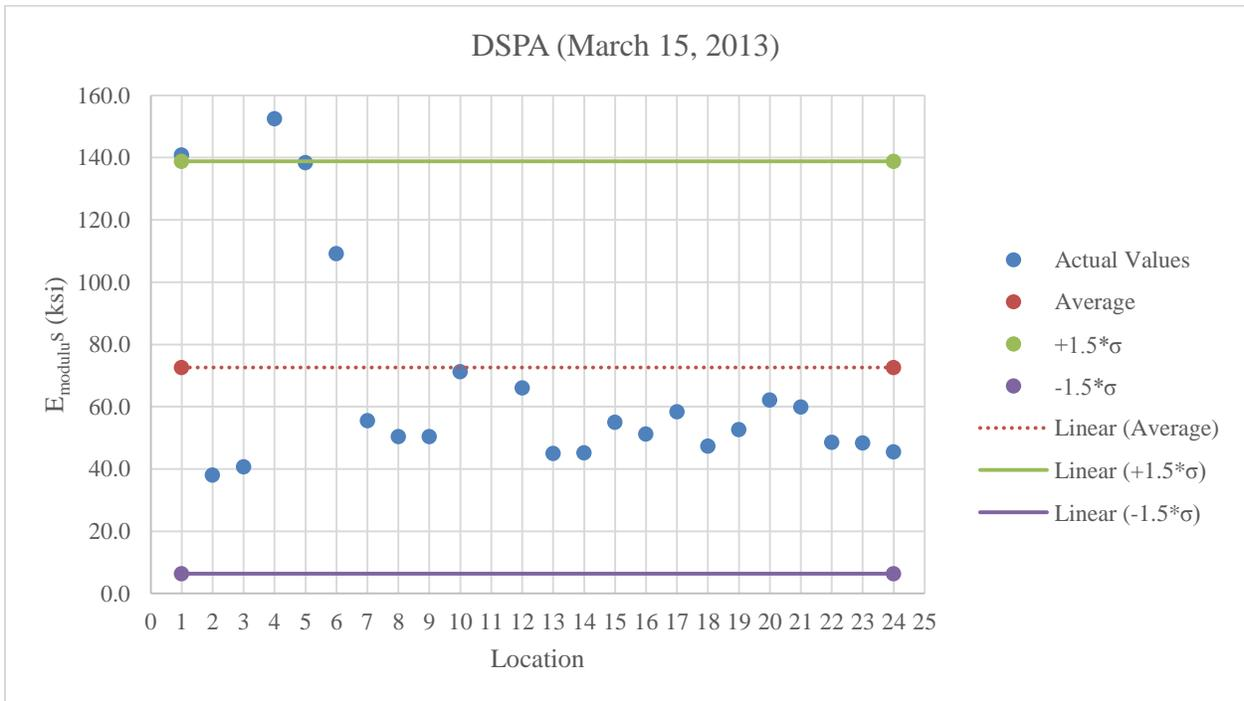
**Figure B.8:** DSPA testing on A-3 at optimum moisture content
