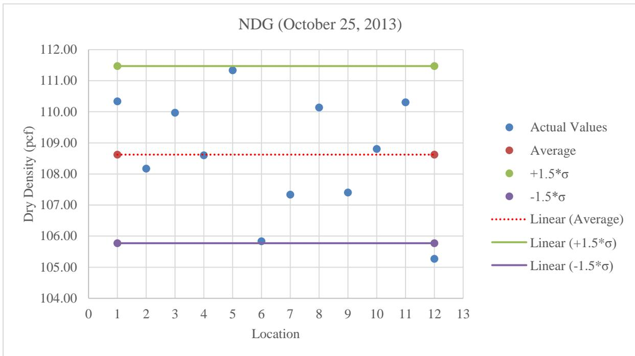
**Figure C.27:** Plot of NDG values for A-2-4 low fines at 6% less than optimum moisture content
