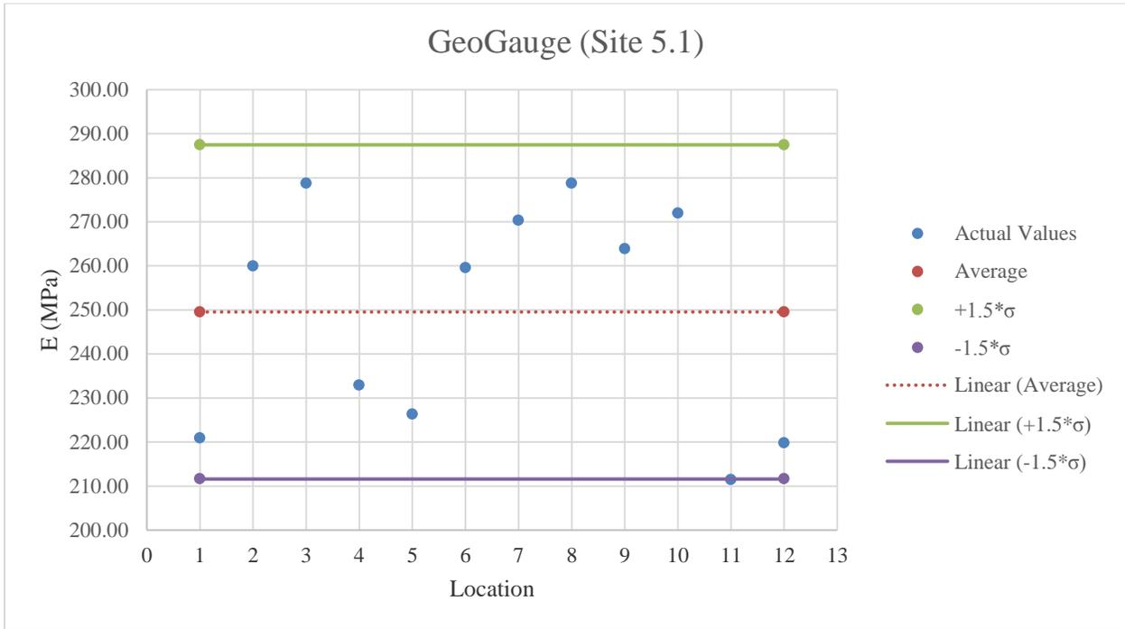
**Figure E.43:** GeoGauge testing results on limerock material
