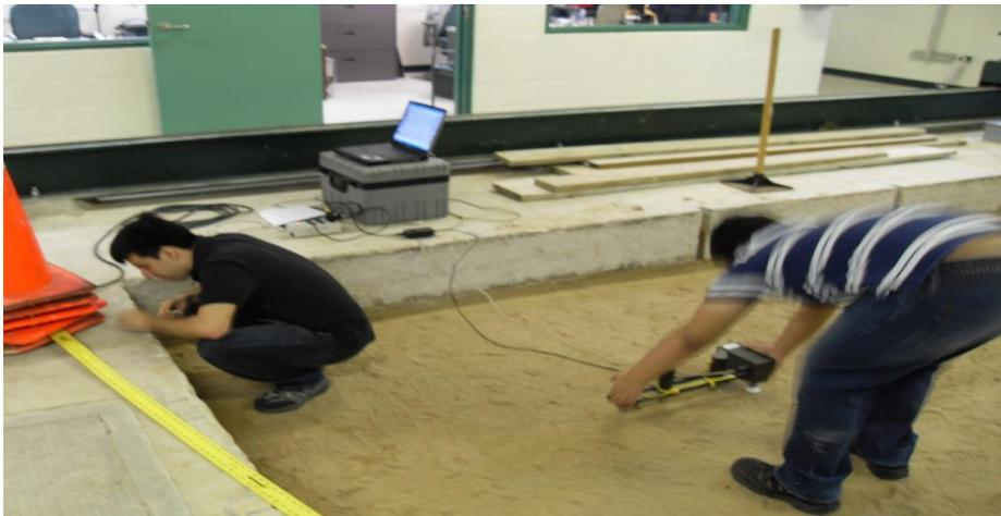
**Figure 3.14:** Photograph of east test pit layout and DSPA
