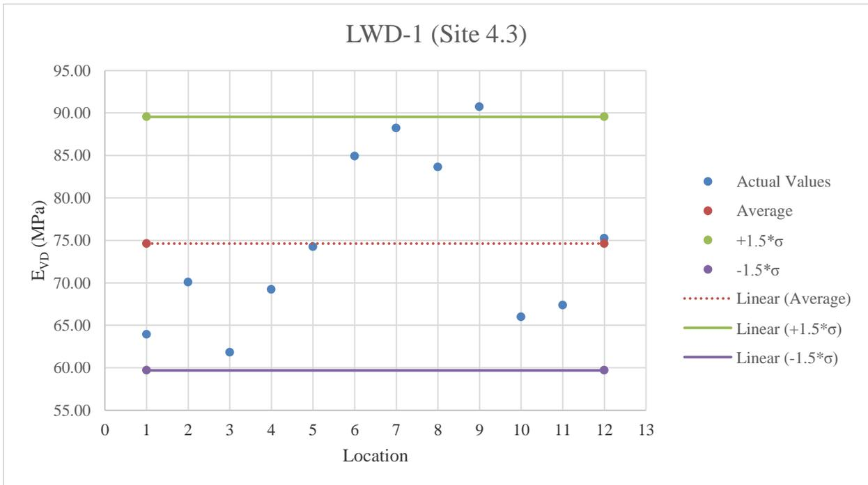
**Figure E.38:** LWD-1 testing results on stabilized subgrade
