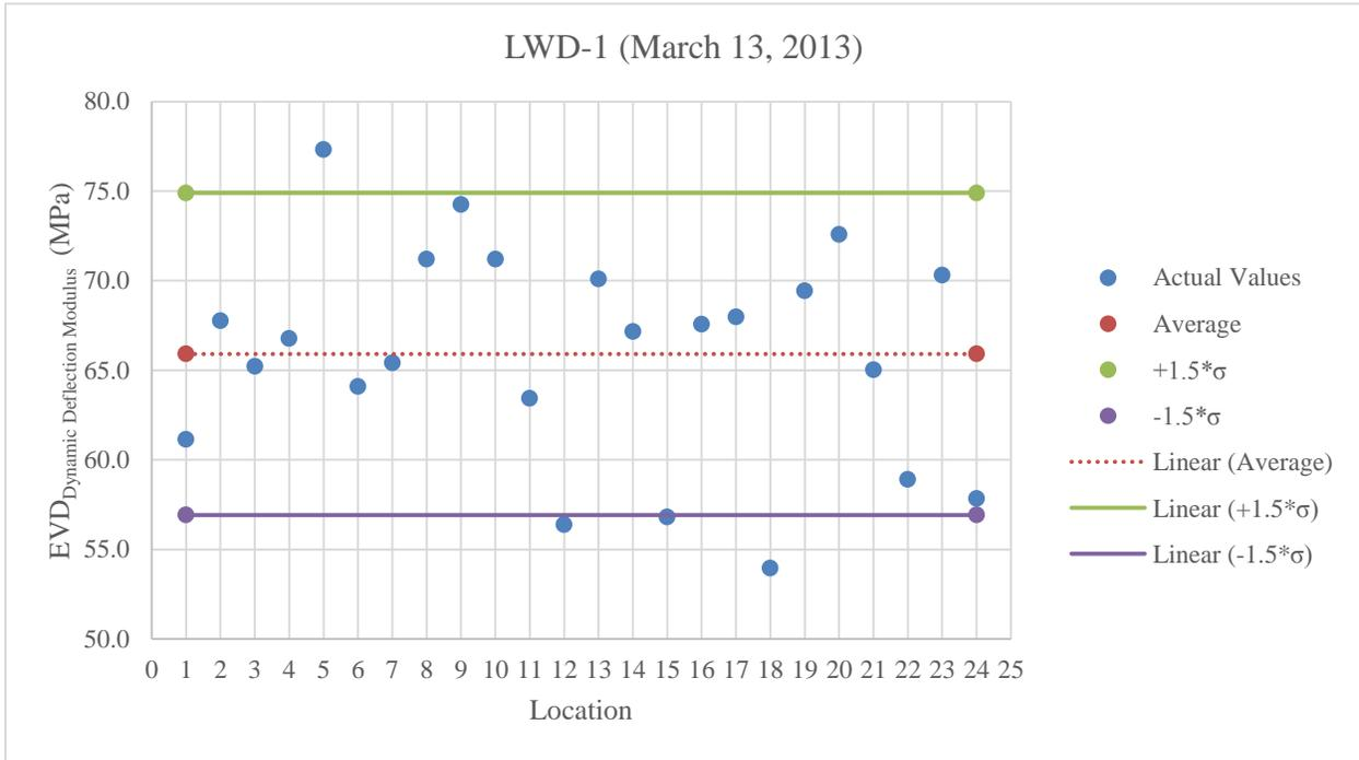
**Figure B.29:** LWD-1 testing on A-3 at optimum moisture content
