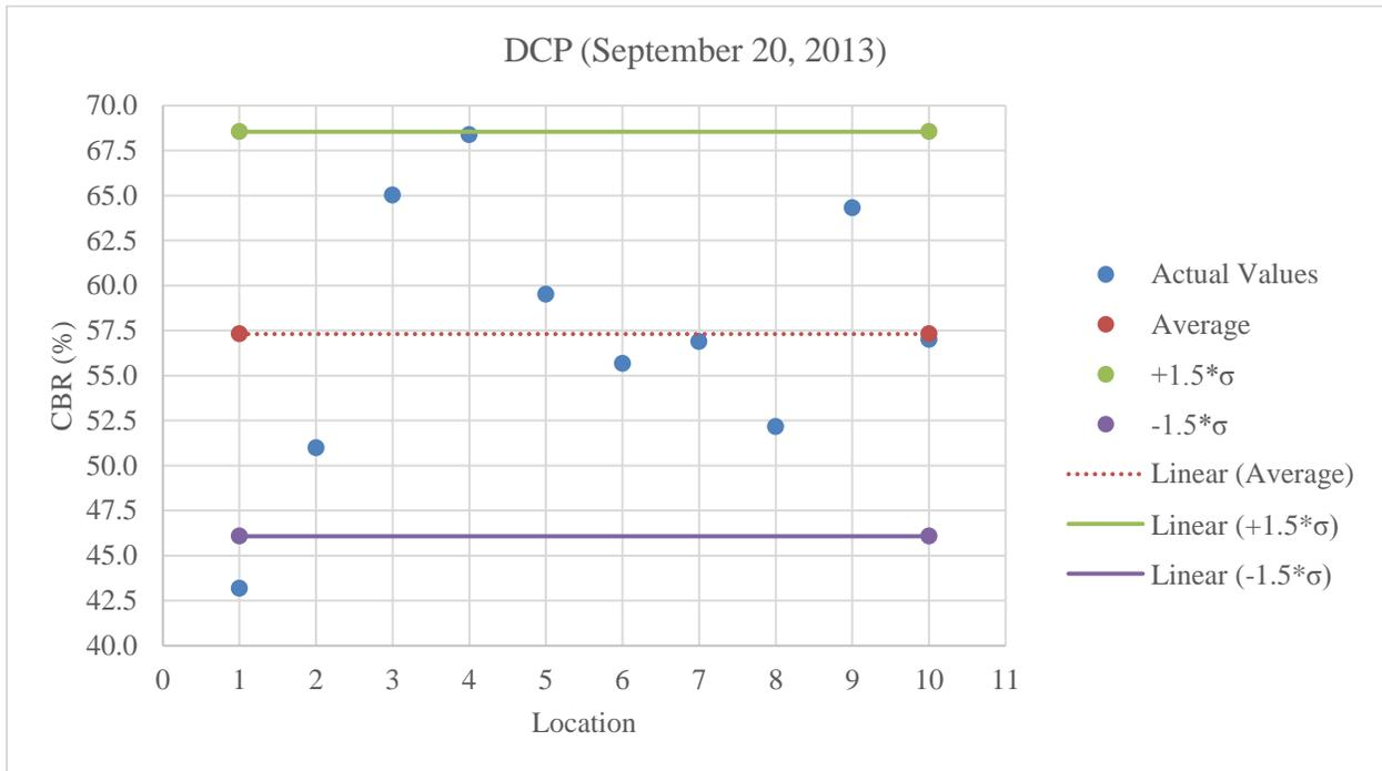
**Figure C.39:** Plot of DCP values for limerock at 3% less than optimum moisture content
