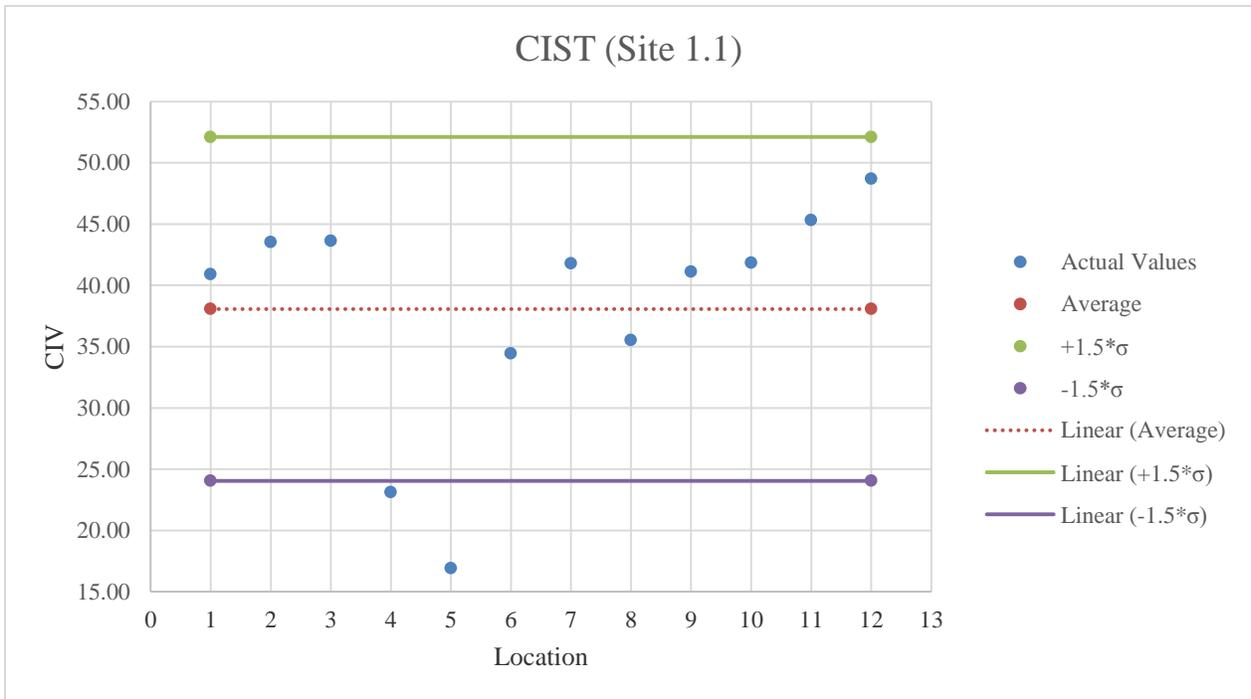
**Figure E.4:** CIST testing results on GAB material
