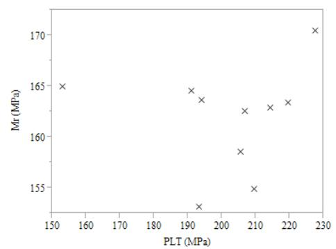
**Figure F.6:** Scatterplot of laboratory resilient modulus vs. PLT measurements (MPa)
