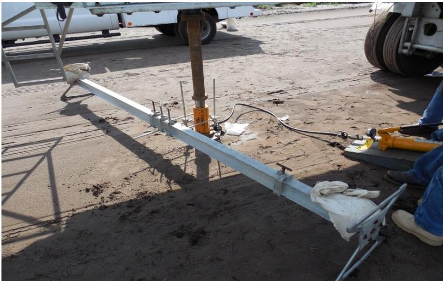
**Figure 5.35:** Project Site #6 SR-23 A-3 embankment - Photograph of PLT
