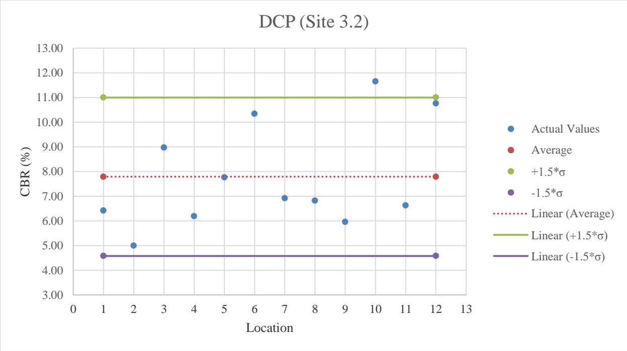
**Figure E.25:** DCP testing results on A-3 material
