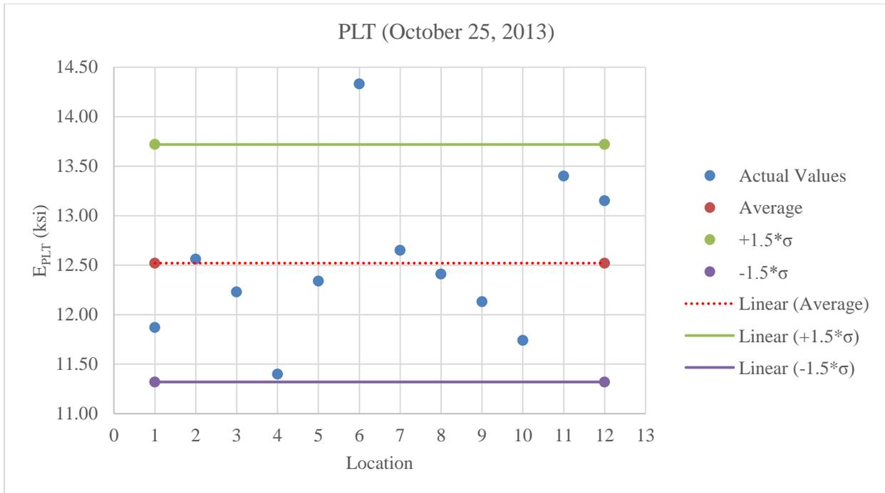
**Figure C.29:** Plot of PLT values for A-2-4 low fines at 6% less than optimum moisture content
