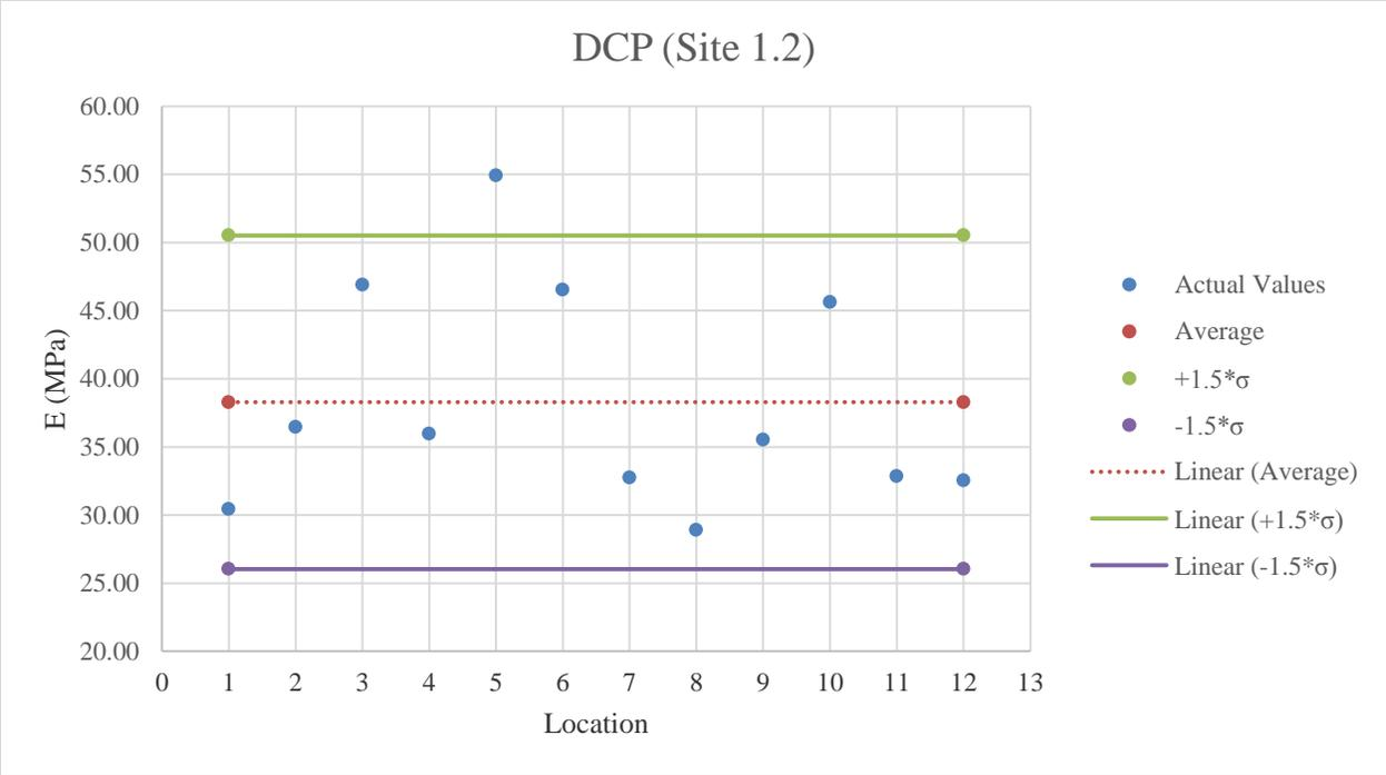
**Figure E.7:** DCP testing results on GAB material
