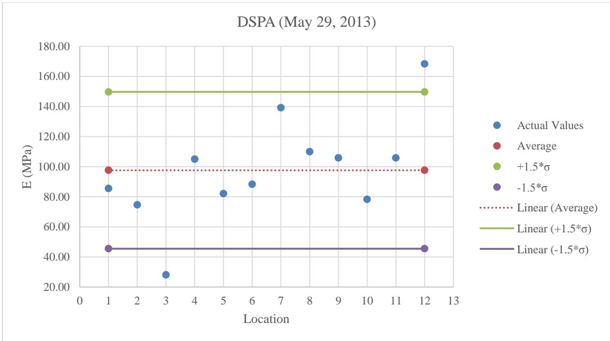
**Figure B.15:** DSPA testing on A-2-4 below optimum moisture content
