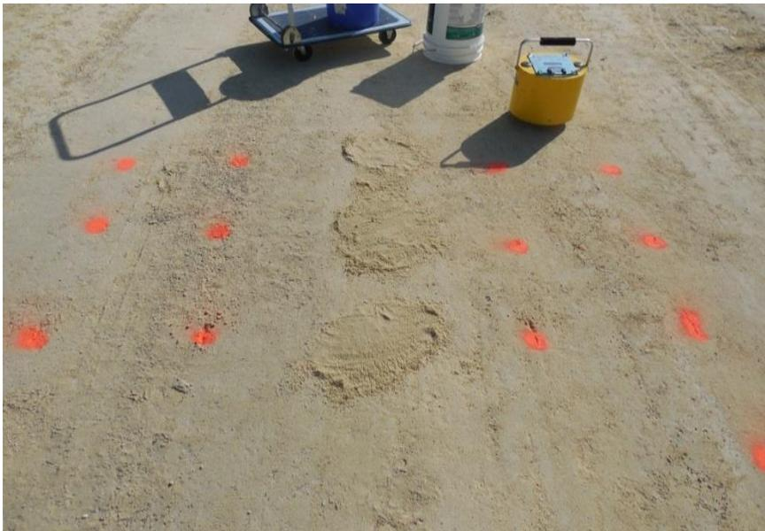
**Figure 5.26:** Project Site #4 CR-210 - Photograph of damp, fine sand used for bedding for GeoGauge due to the irregular surface of the limerock
