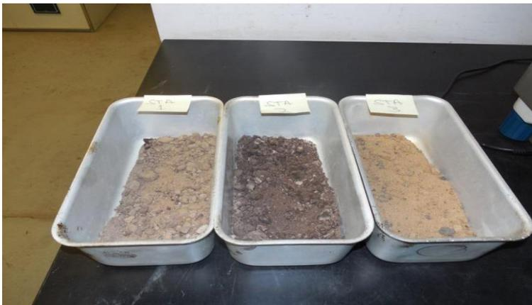
**Figure 5.21:** Project Site #3 SR-9B - Photograph of oven-dried samples (From left to right: north, center, and south. Note different colors.)
