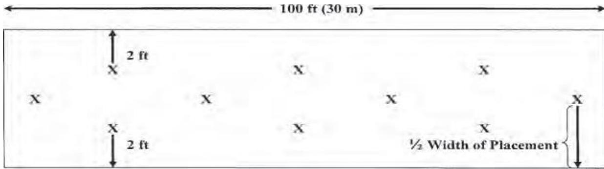
**Figure 7.1:** INDOT LWD test pad for maximum allowable deflection determination
