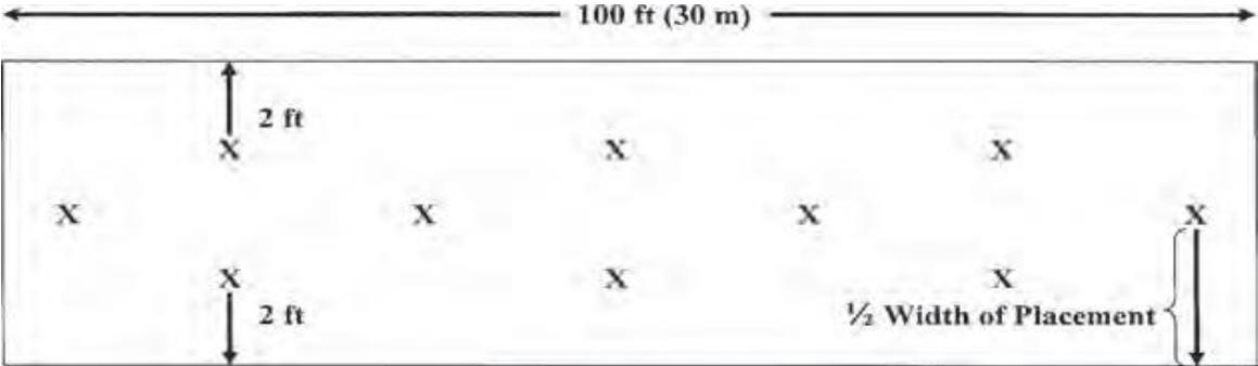
**Figure 8.1:** INDOT test section for LWD (for reference as DCP test section)
