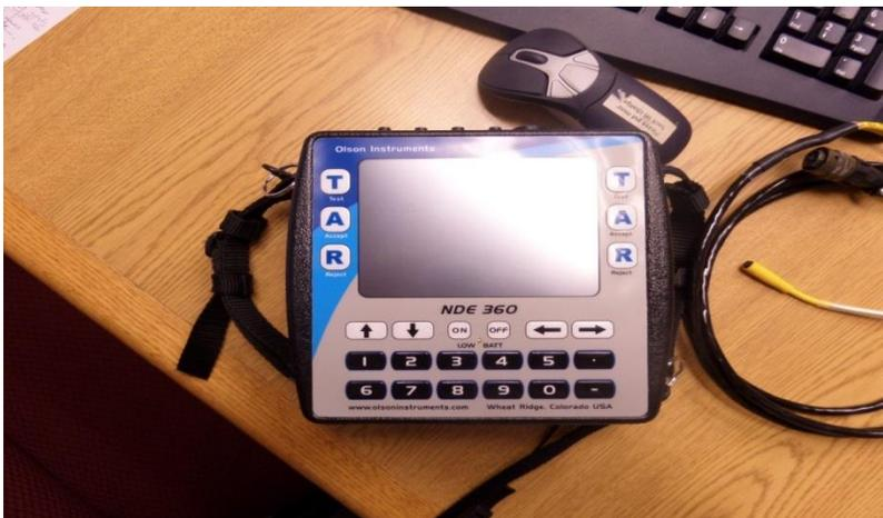
**Figure 7.10:** Photograph of Olson prototype LWD data collector
