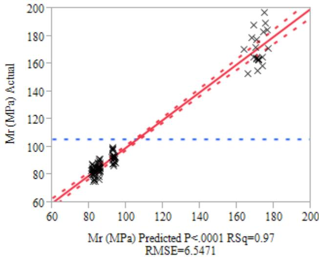
The Actual by Predicted Plot shows the actual (observed)  $M_R$  values against the predicted  $M_R$  values. As the predicted values come closer to the actual values, the points on the scatterplot fall closer around the red line.
