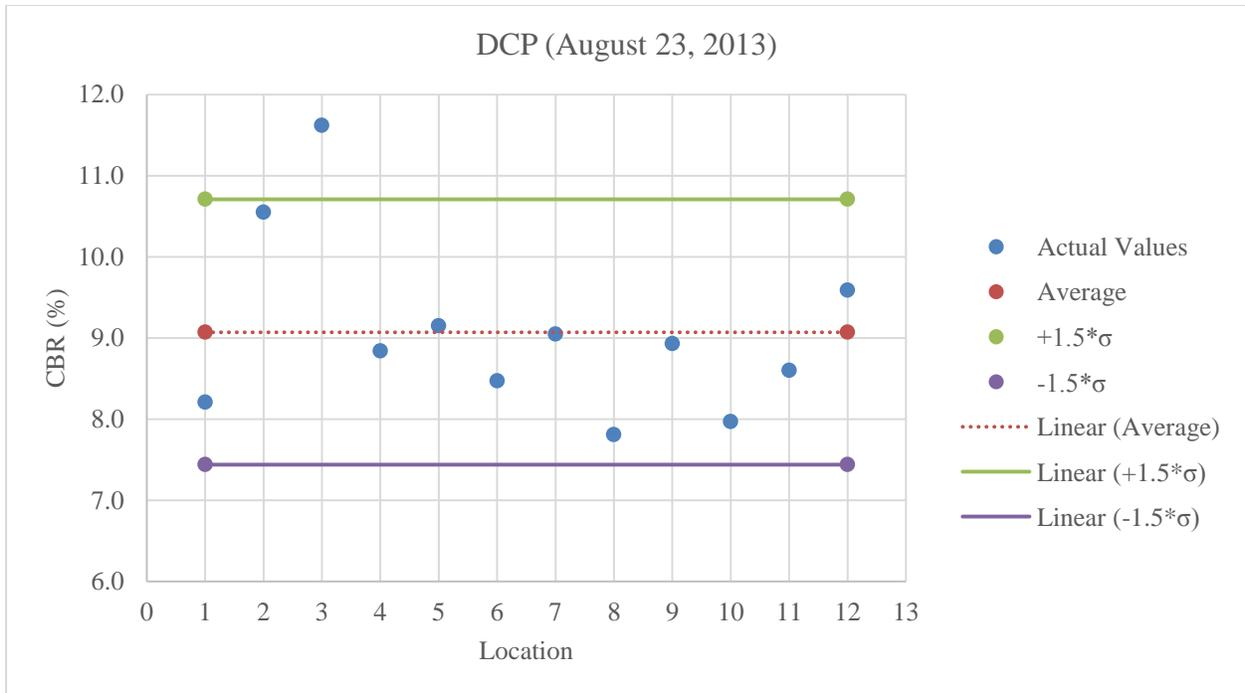
**Figure C.3:** Plot of DCP values for A-3 at optimum moisture content
