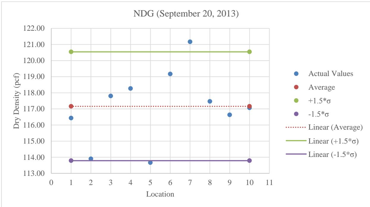
**Figure C.41:** Plot of NDG values for limerock at 3% less than optimum moisture content
