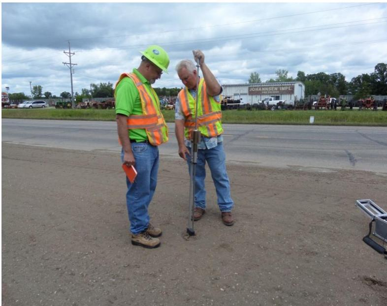
**Figure 7.6:** Photograph of Mn/DOT DCP on Class 5 aggregate base
