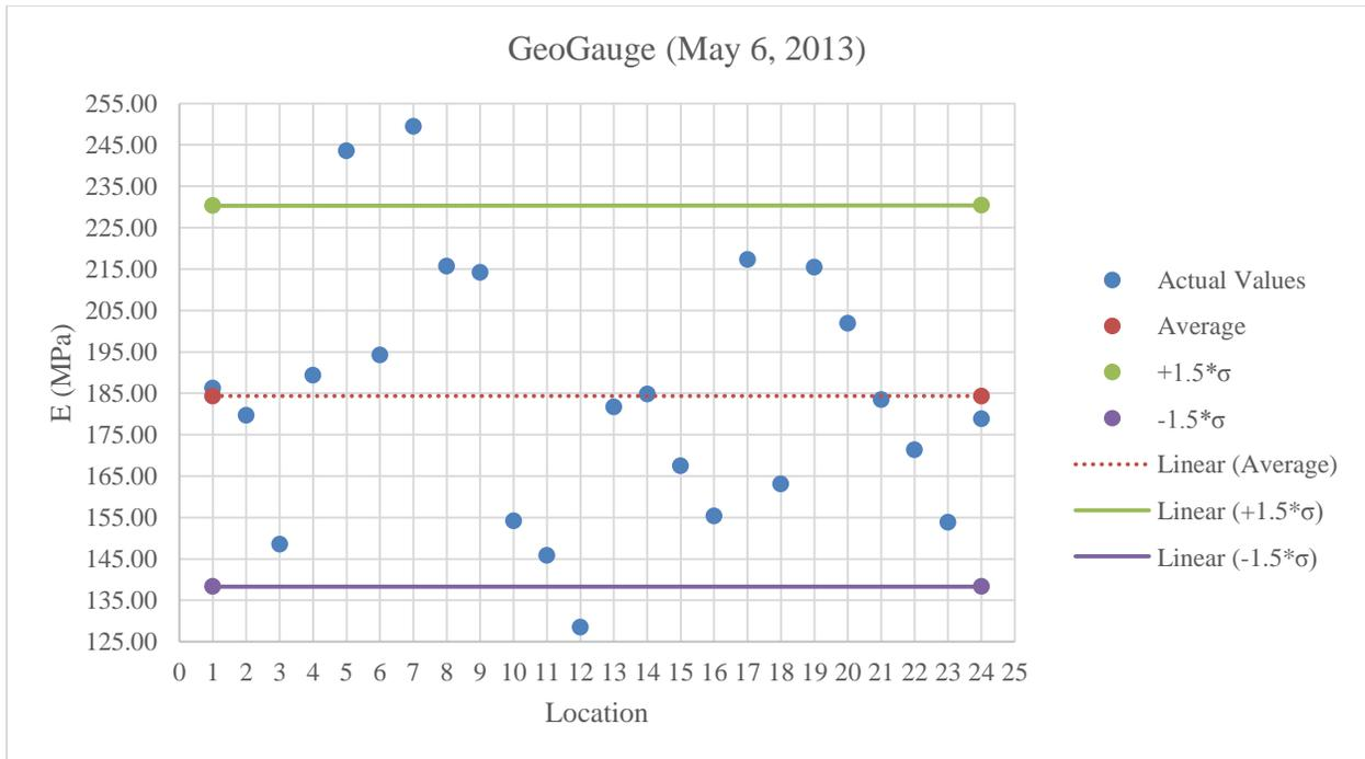
**Figure B.25:** GeoGauge testing on A-2-4 below optimum moisture content
