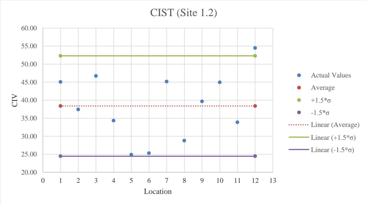
**Figure E.8:** CIST testing results on GAB material
