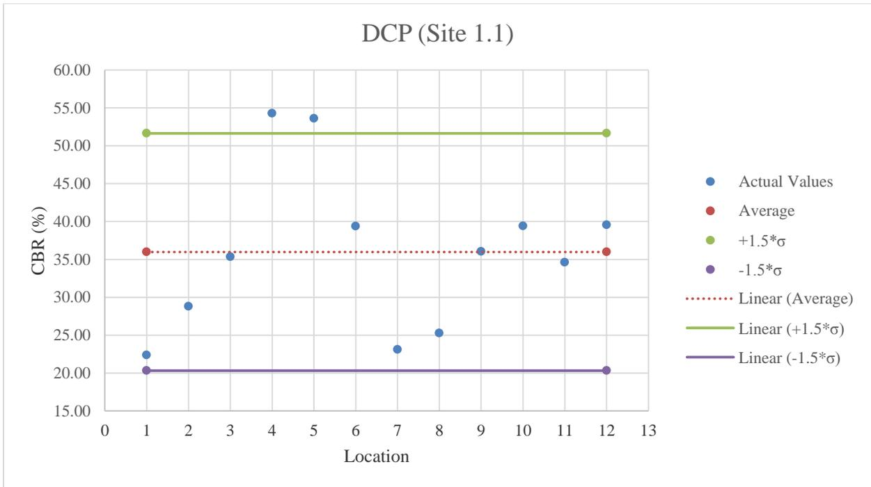
**Figure E.3:** DCP testing results on GAB material
