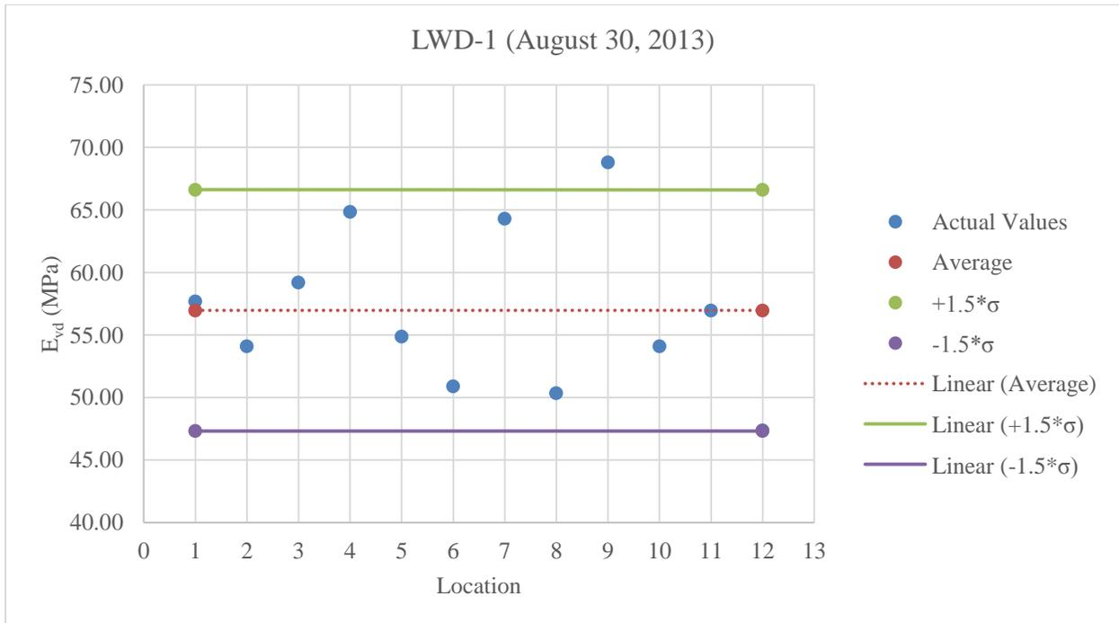
**Figure C.8:** Plot of LWD-1 values for A-3 at 7% less than optimum moisture content
