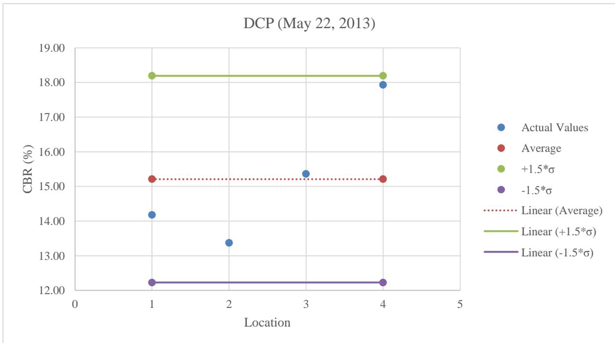
**Figure B.20:** DCP testing on stabilized subgrade above optimum moisture content
