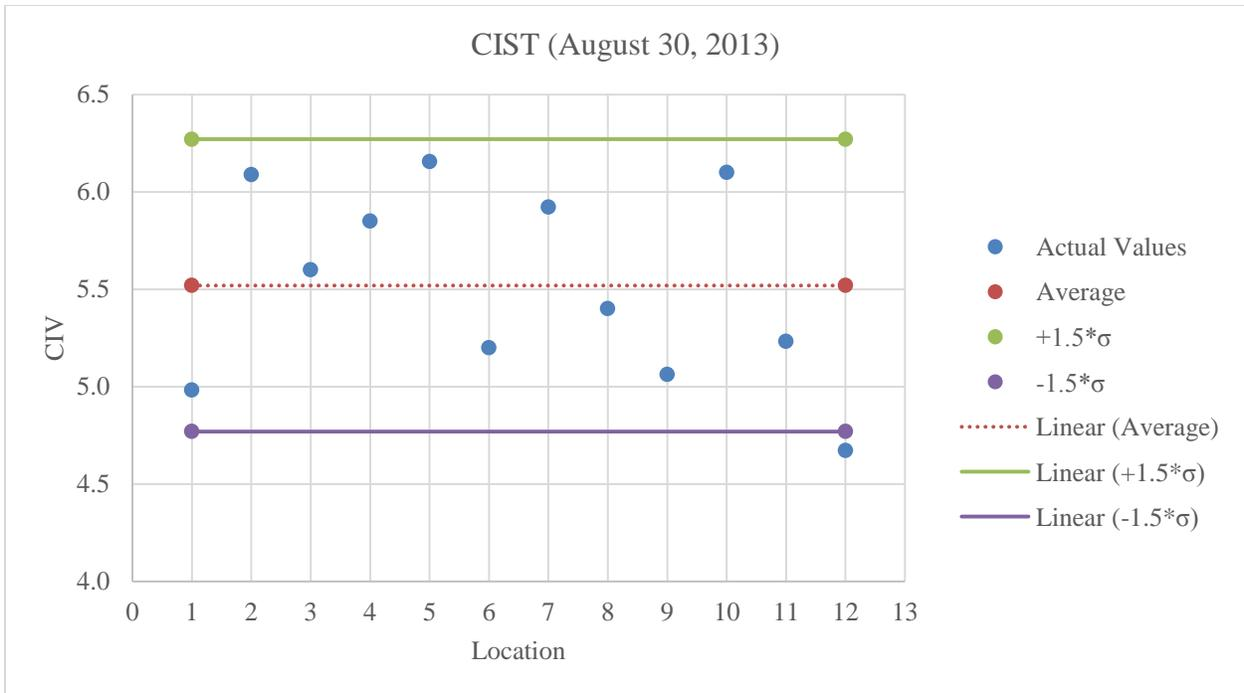
**Figure C.11:** Plot of CIST values for A-3 at 7% less than optimum moisture content
