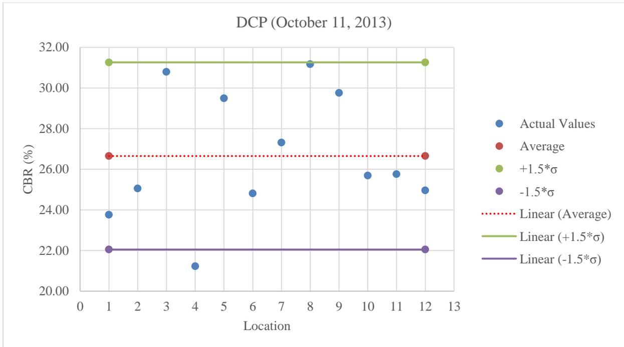
**Figure C.17:** Plot of DCP values for A-2-4 low fines at optimum moisture content
