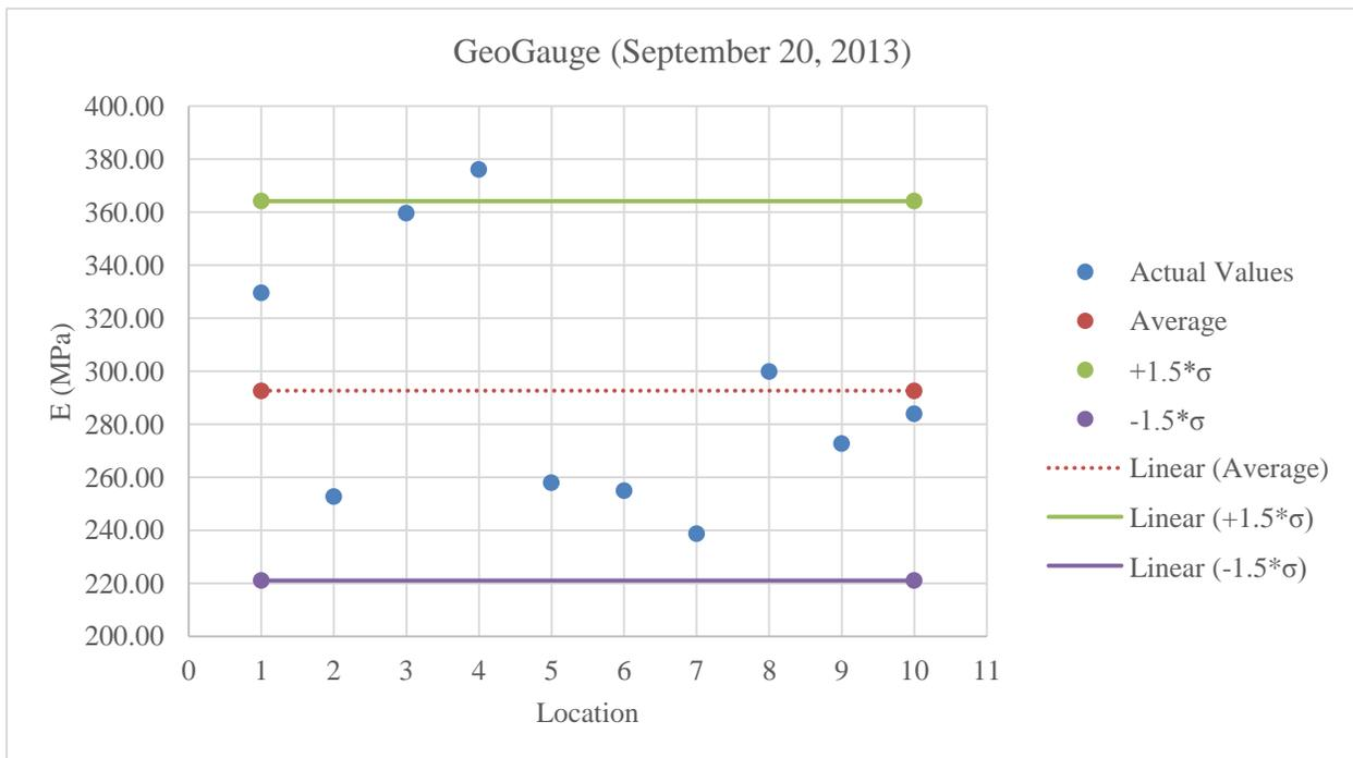
Figure C.38: Plot of GeoGauge values for limerock at 3% less than optimum moisture content
