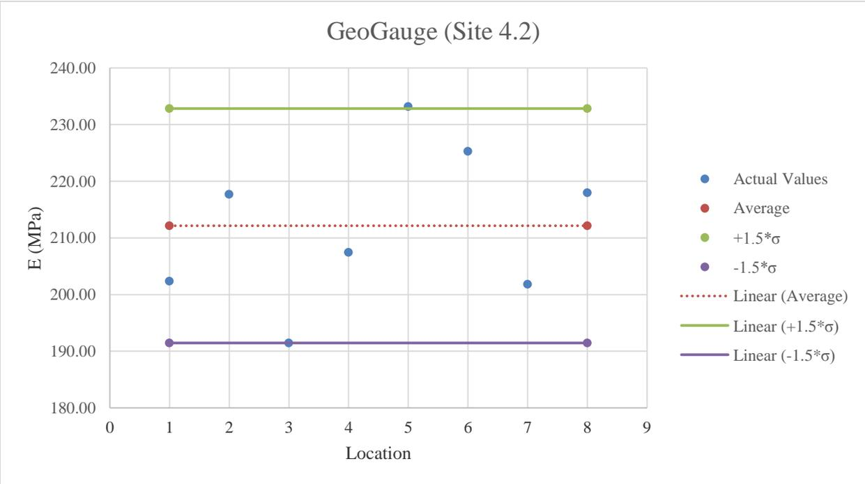
**Figure E.36:** GeoGauge testing results on stabilized subgrade
