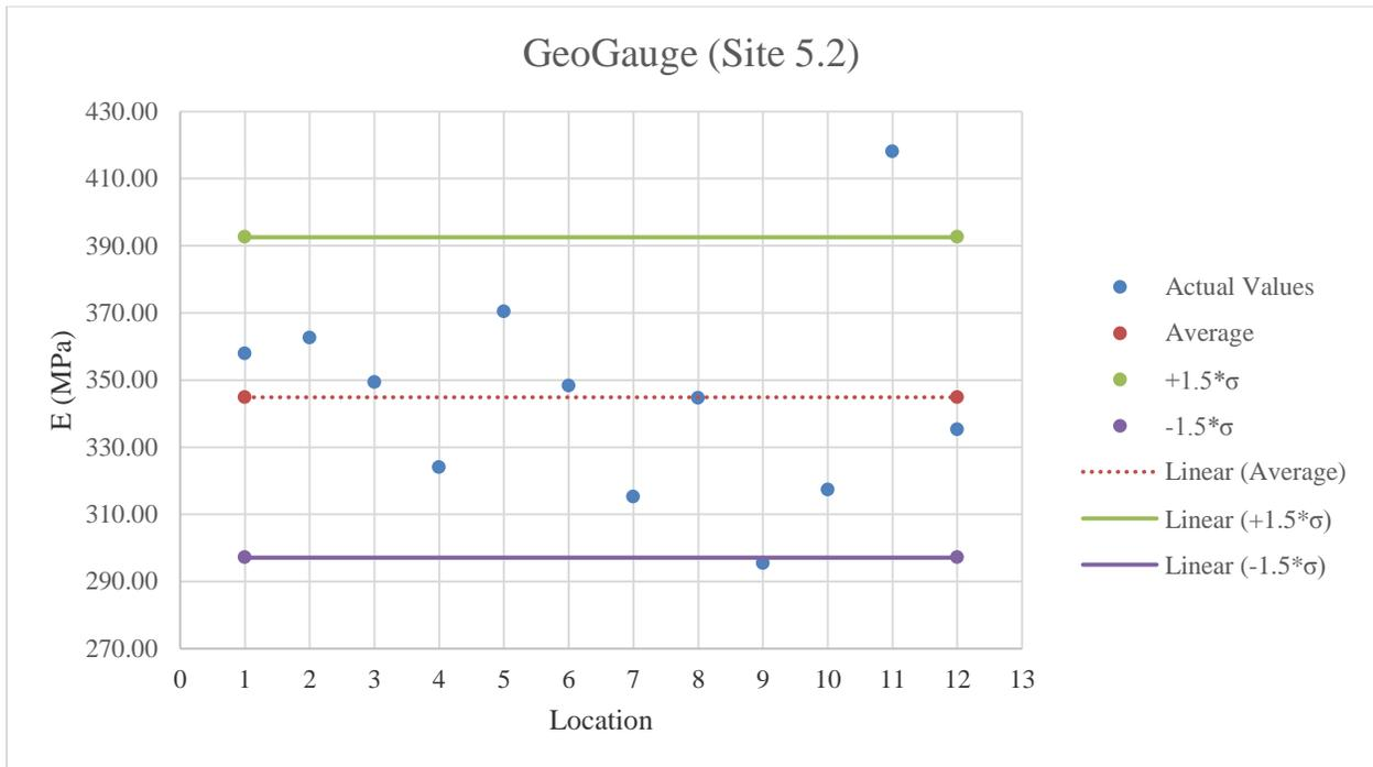
**Figure E.47:** GeoGauge testing results on limerock material
