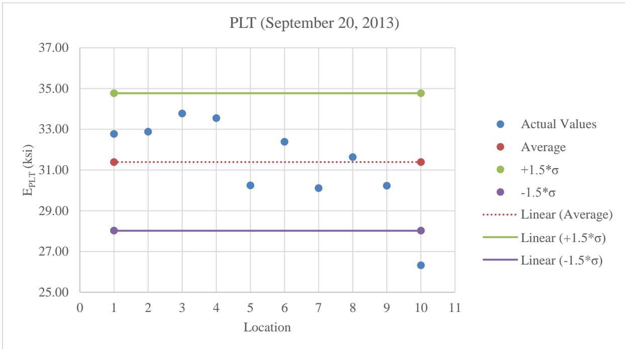
**Figure C.43:** Plot of PLT vales for limerock at 3% less than optimum moisture content
