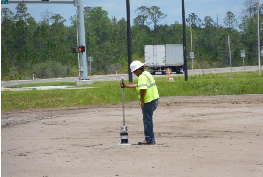
**Figure 5.34:** Project Site #6 SR-23 A-3 embankment - Photograph of LWD-2 test
