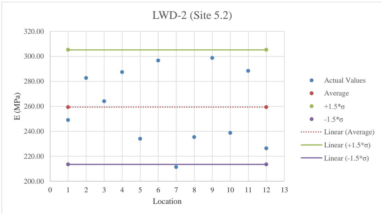
**Figure E.46:** LWD-2 testing results on limerock material
