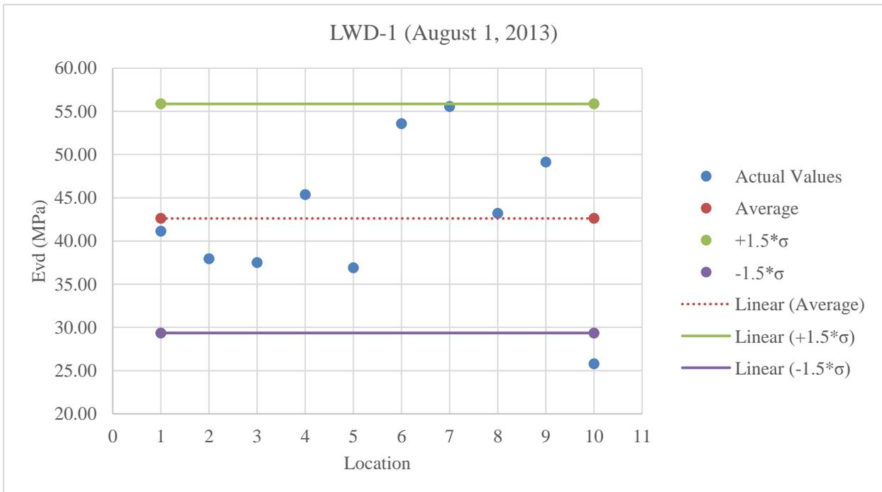
**Figure C.44:** Plot of LWD-1 values for stabilized subgrade at optimum moisture content
