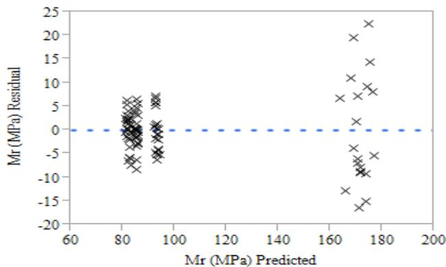
The Residual by Predicted Plot shows the residuals plotted against the predicted values of laboratory  $M_R$ . Residual values scattered randomly about zero are desired.
