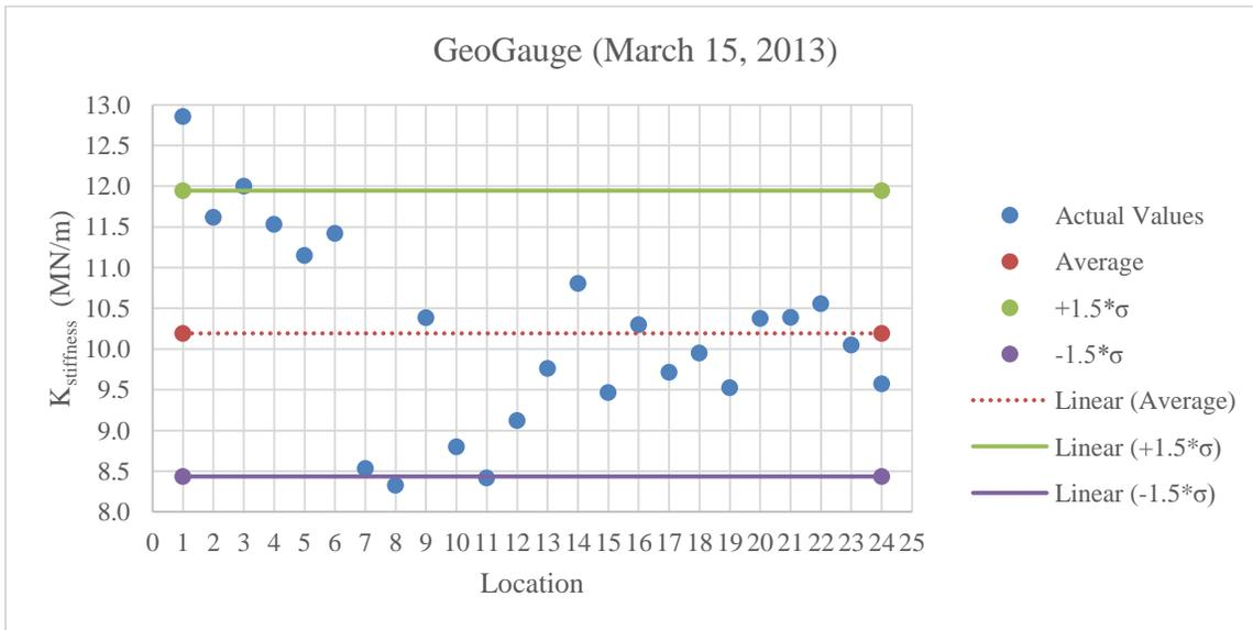
Figure B.22: GeoGauge testing on A-3 at optimum moisture content
