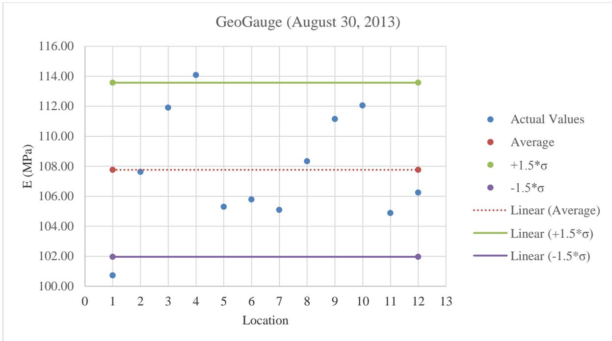
Figure C.9: Plot of GeoGauge values for A-3 at 7% less than optimum moisture content
