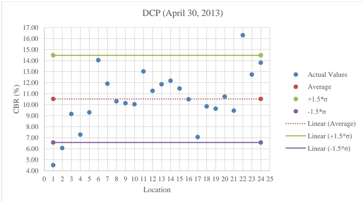
Figure B.17: DCP testing on A-2-4 at optimum moisture content
