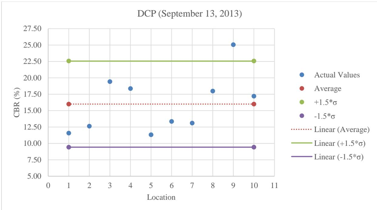
**Figure C.53:** Plot of DCP values for stabilized subgrade below optimum moisture content
