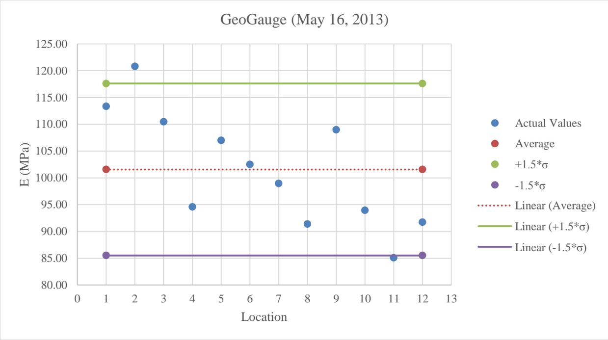
**Figure B.27:** GeoGauge testing on stabilized subgrade below optimum moisture content
