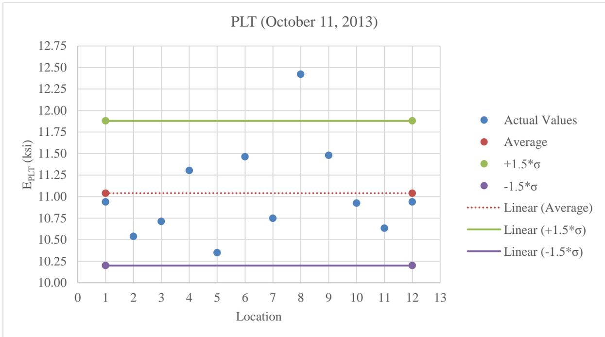
**Figure C.21:** Plot of PLT values for A-2-4 low fines at optimum moisture content
