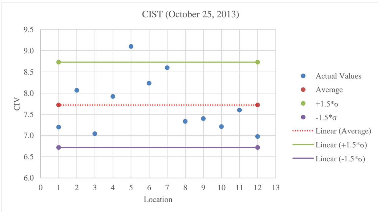
**Figure C.26:** Plot of CIST values for A-2-4 low fines at 6% less than optimum moisture content
