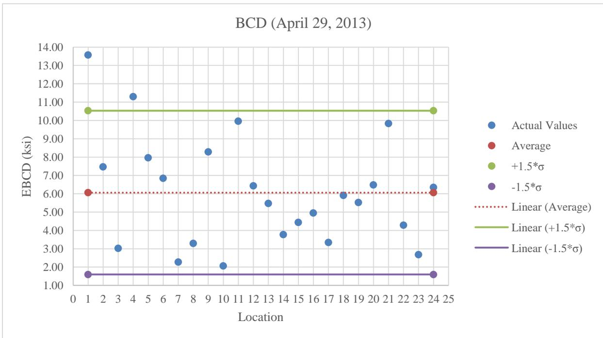
**Figure B.2:** BCD testing on A-2-4 at optimum moisture content
