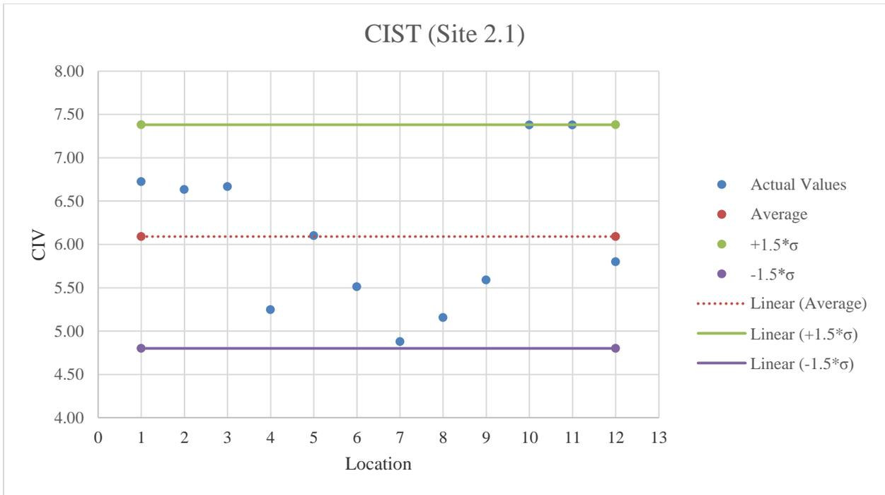
**Figure E.15:** CIST testing results on A-2-4 material
