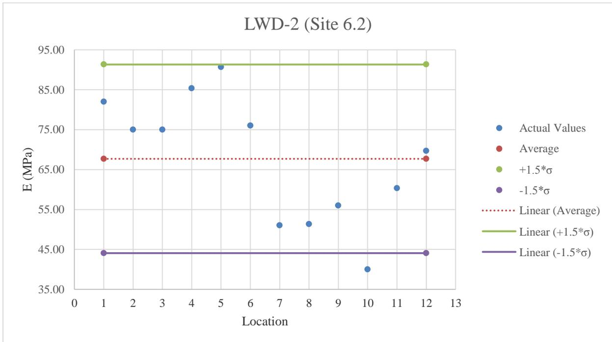
**Figure E.58:** LWD-2 testing results on A-3 material
