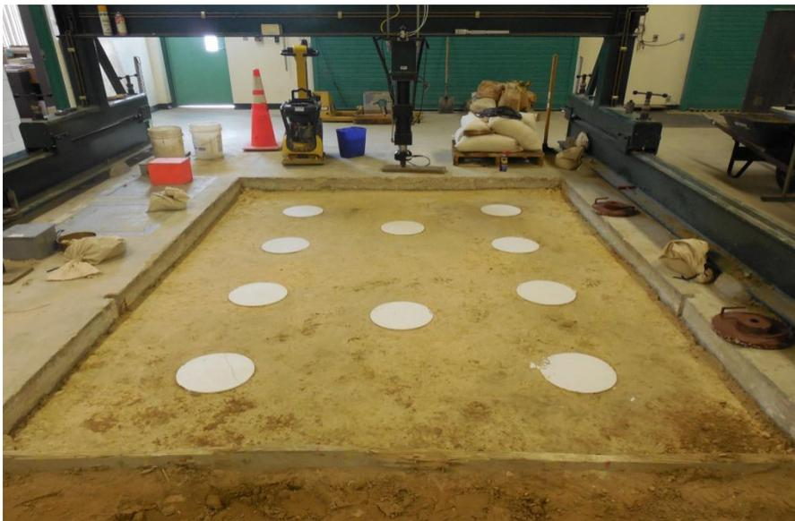
**Figure 4.4:** Photograph of east test pit limerock base ten PLT locations per half pit
