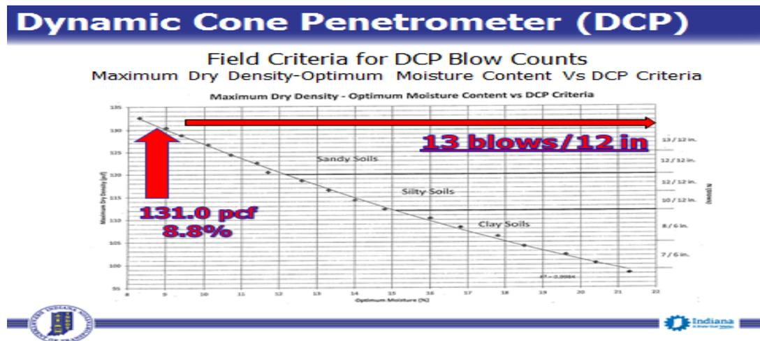
**Figure 7.4:** INDOT field criteria for DCP blow counts
