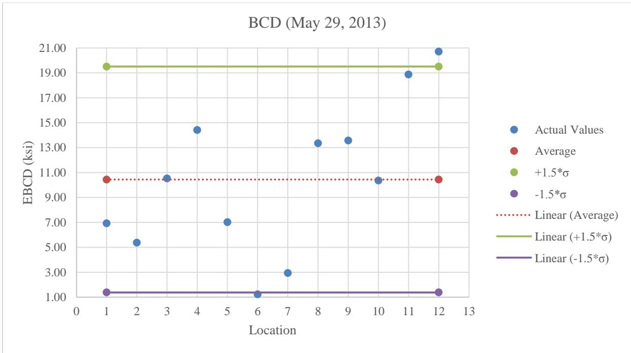
**Figure B.7:** BCD testing on A-2-4 below optimum moisture content
