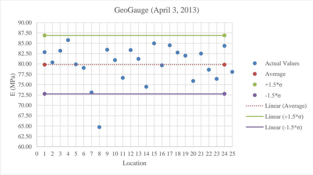
Figure B.23: GeoGauge testing on A-3 below optimum moisture content
