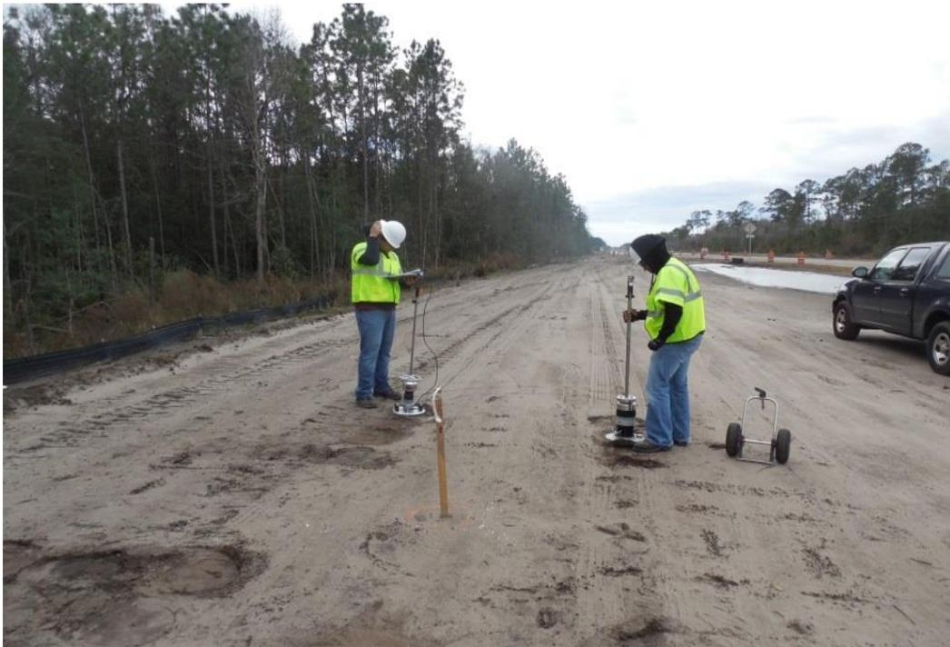
**Figure 5.11:** Project Site #2 US-301 - Photograph of LWDs by two different manufacturers
