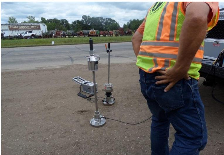
**Figure 7.8:** Photograph of Mn/DOT LWDs on Class 5 aggregate base
