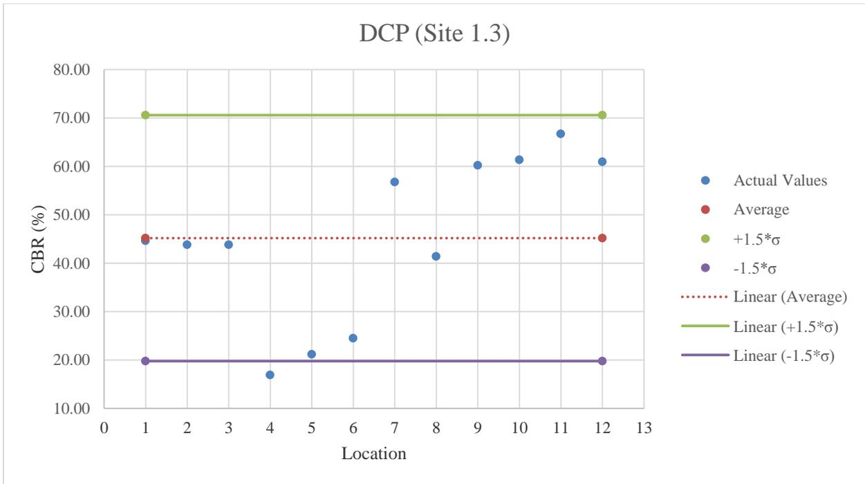
**Figure E.11:** DCP testing results on GAB material
