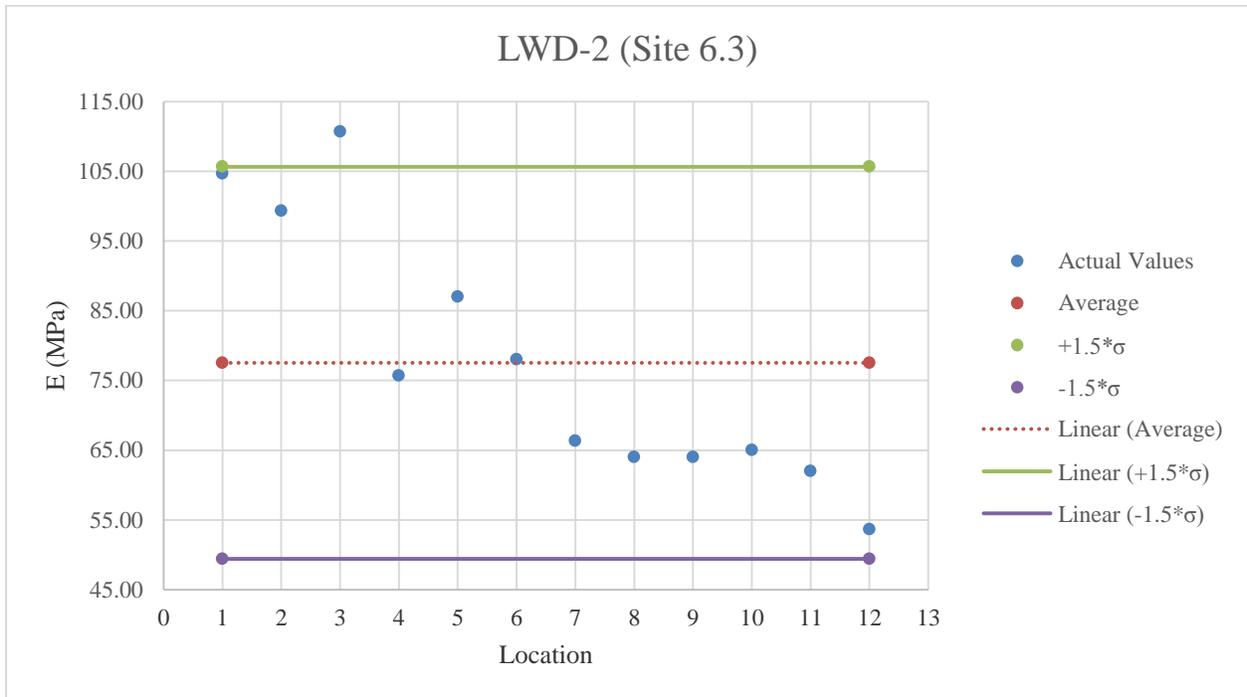
**Figure E.62:** LWD-2 testing results on A-3 material
