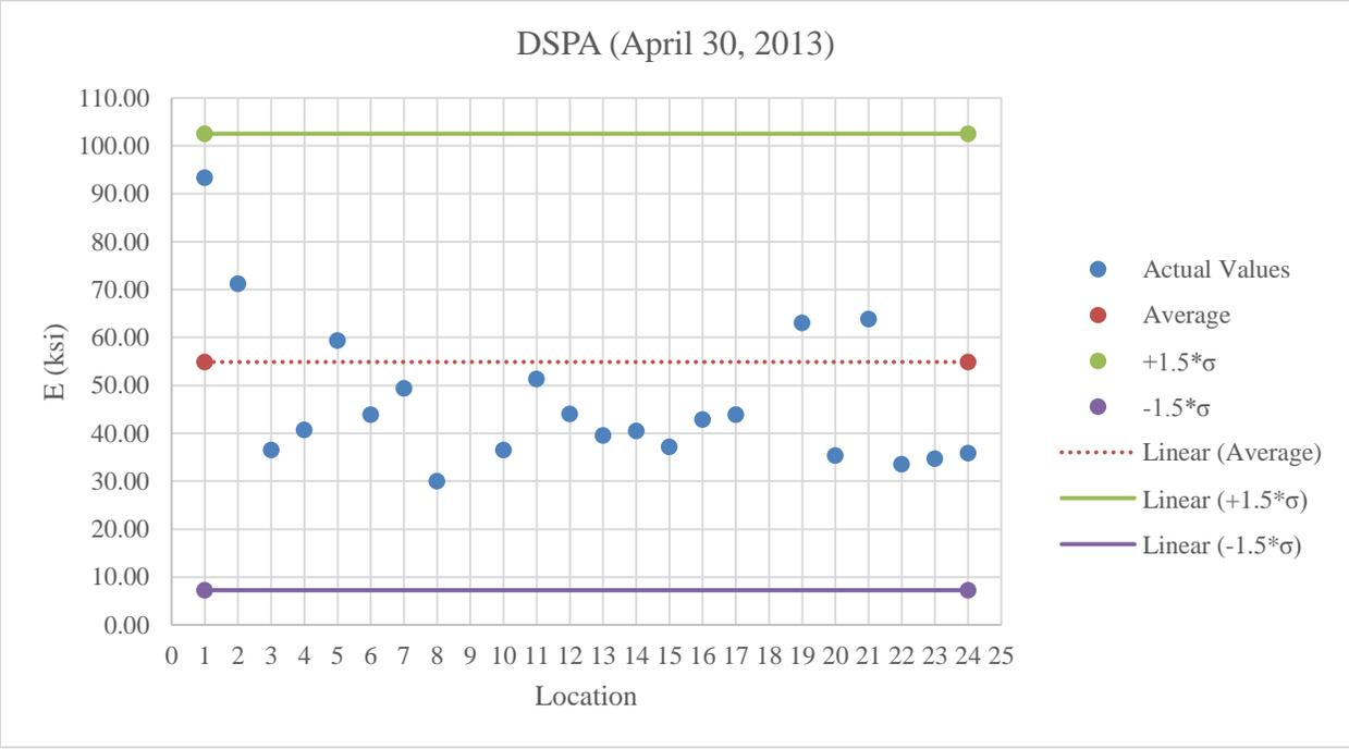
Figure B.10: DSPA testing on A-2-4 at optimum moisture content
