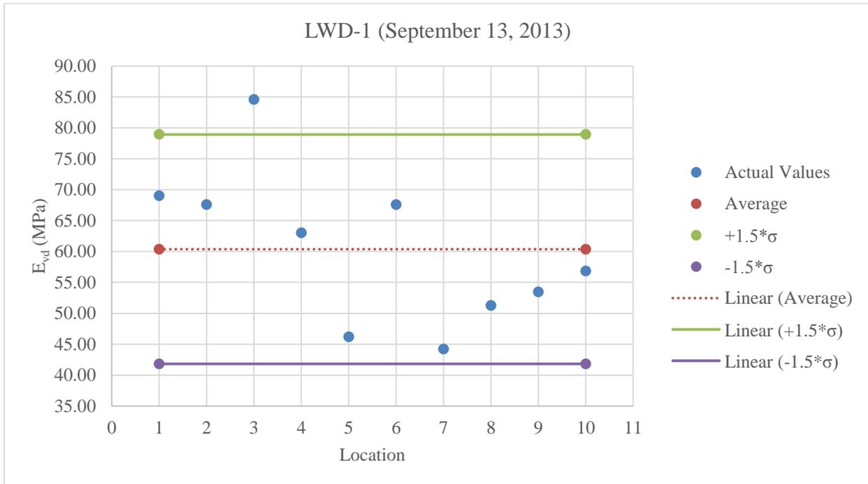
Figure C.51: Plot of LWD-1 values for stabilized subgrade below optimum moisture content
