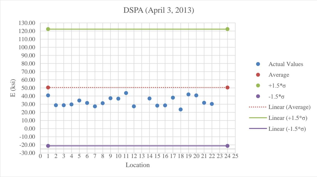
Figure B.9: DSPA testing on A-3 below optimum moisture content
