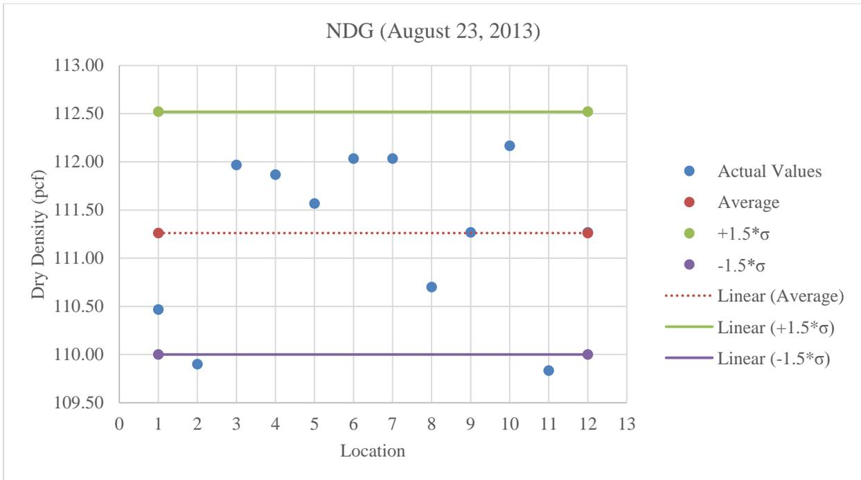
**Figure C.5:** Plot of NDG values for A-3 at optimum moisture content
