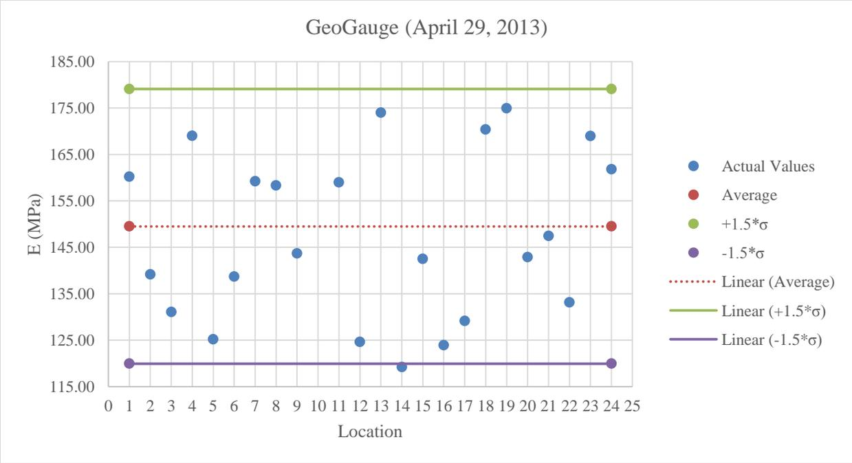
Figure B.24: GeoGauge testing on A-2-4 at optimum moisture content
