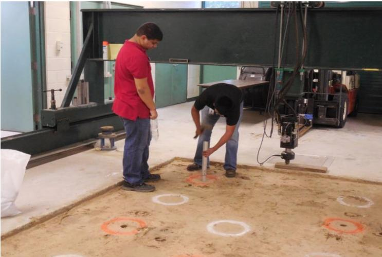
**Figure 4.6:** Photograph of east test pit limerock base ten moisture samples
