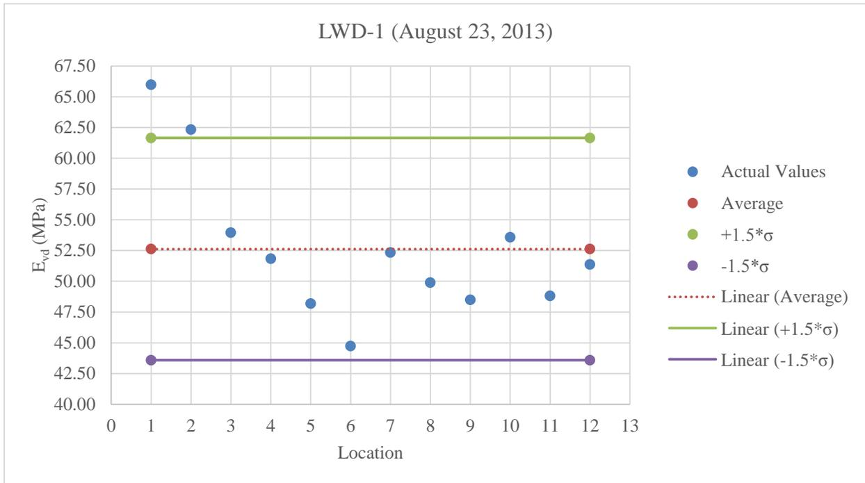
**Figure C.1:** Plot of LWD-1 values for A-3 at optimum moisture content
