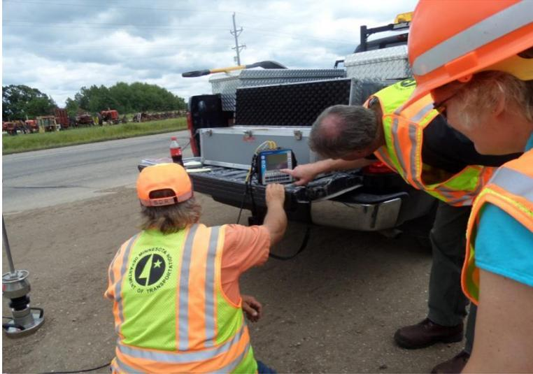
**Figure 7.9:** Photograph of Olson prototype LWD on Class 5 aggregate base
