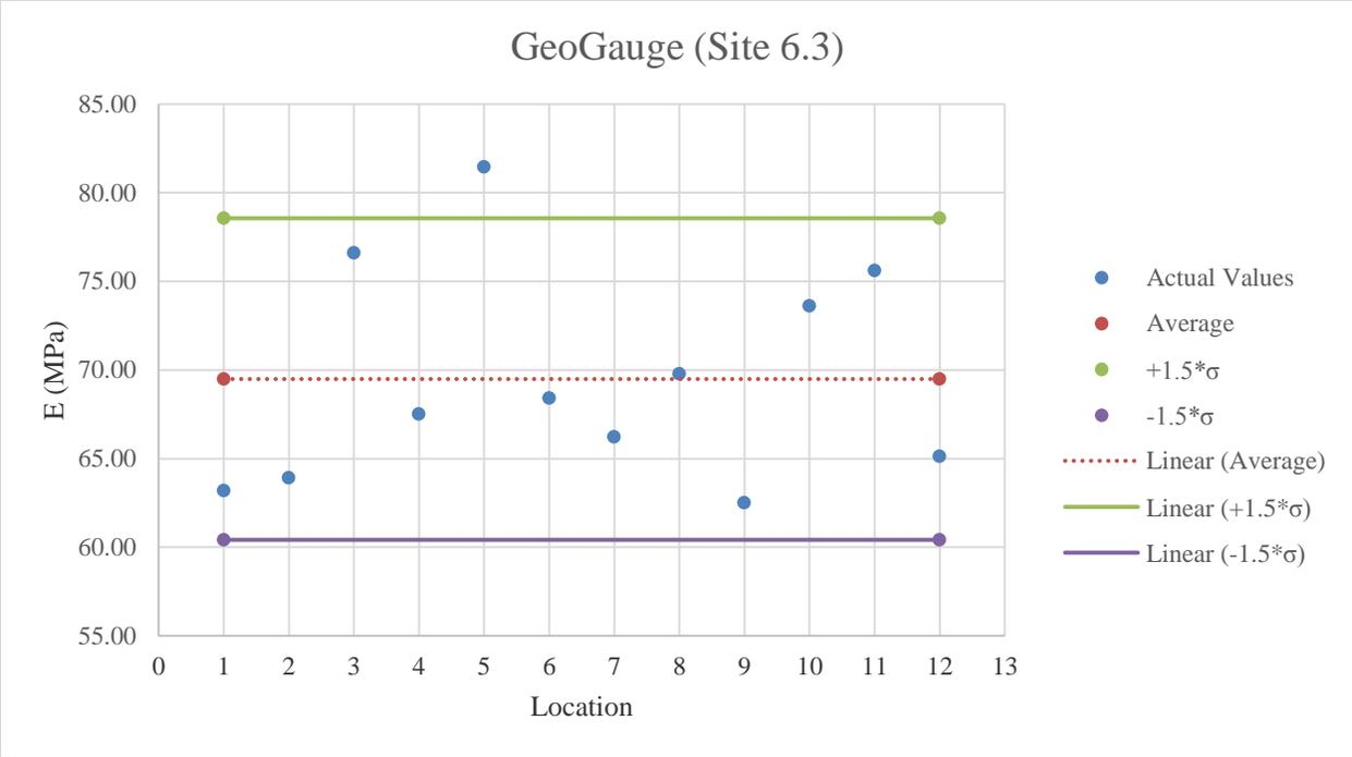
**Figure E.63:** GeoGauge testing results on A-3 material
