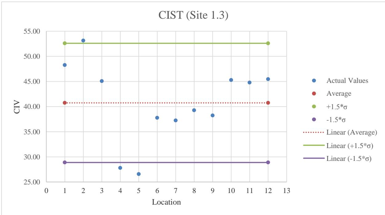
**Figure E.12:** CIST testing results on GAB material
