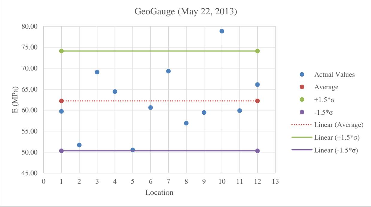
**Figure B.28:** GeoGauge testing on stabilized subgrade above optimum moisture content
