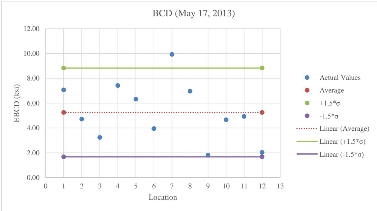
Figure B.5: BCD testing on stabilized subgrade below optimum moisture content
