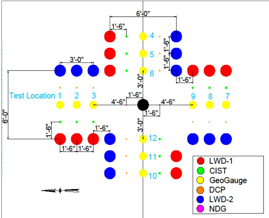
**Figure 5.1:** Orientation of each test site, typical three places
