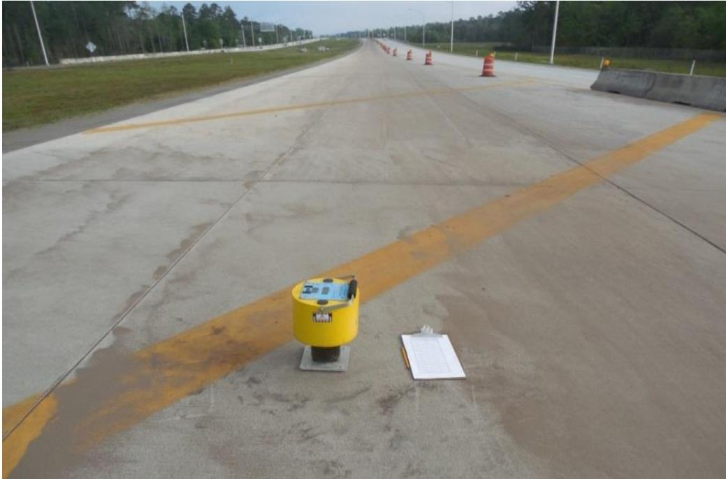
**Figure 5.16:** Project Site #3 SR-9B - Photograph of GeoGauge calibration check
