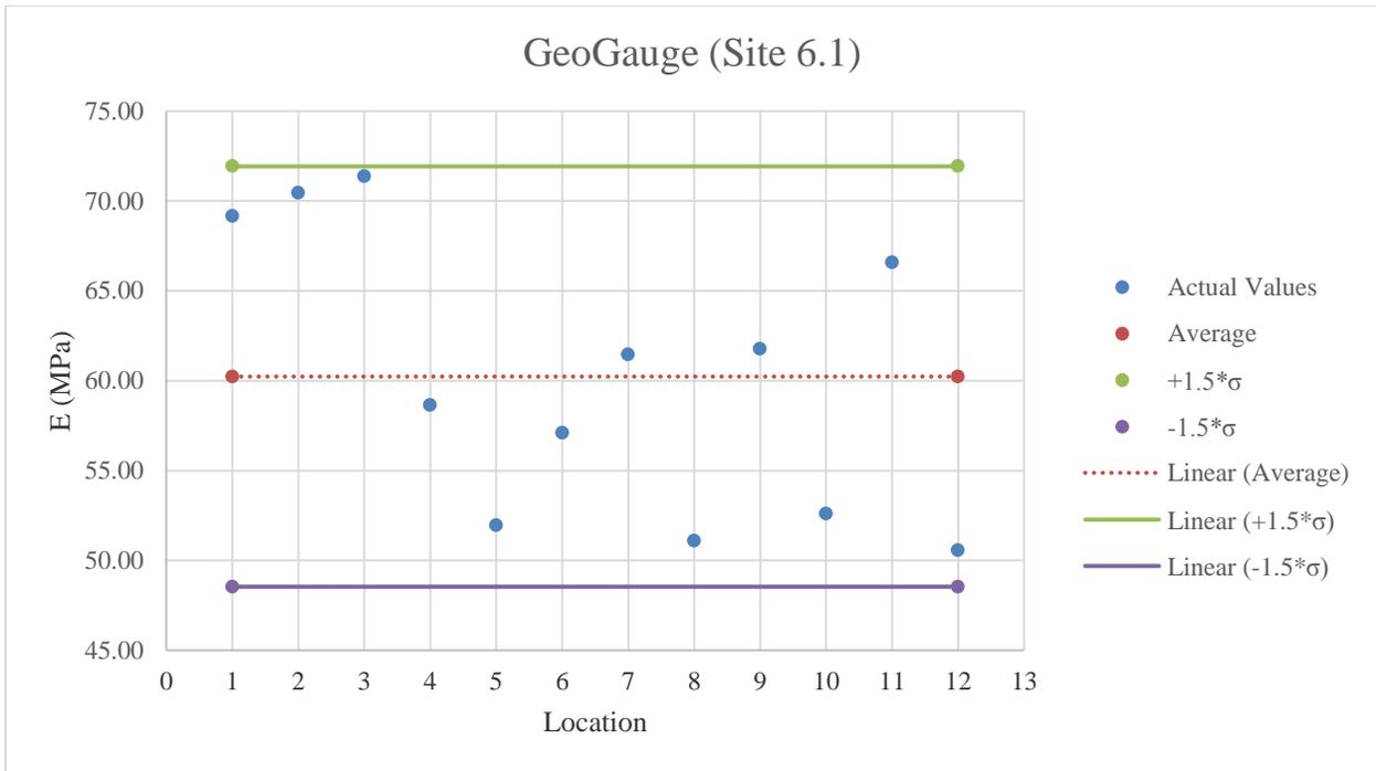
**Figure E.55:** GeoGauge testing results on A-3 material
