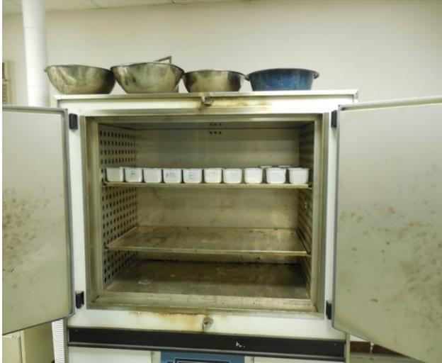
**Figure 4.7:** Photograph of oven drying for moisture content determination
