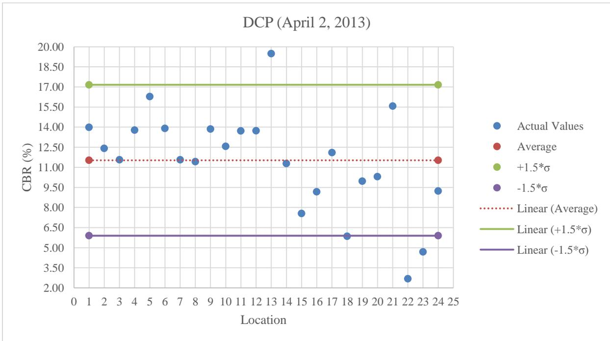
**Figure B.16:** DCP testing on A-3 below optimum moisture content
