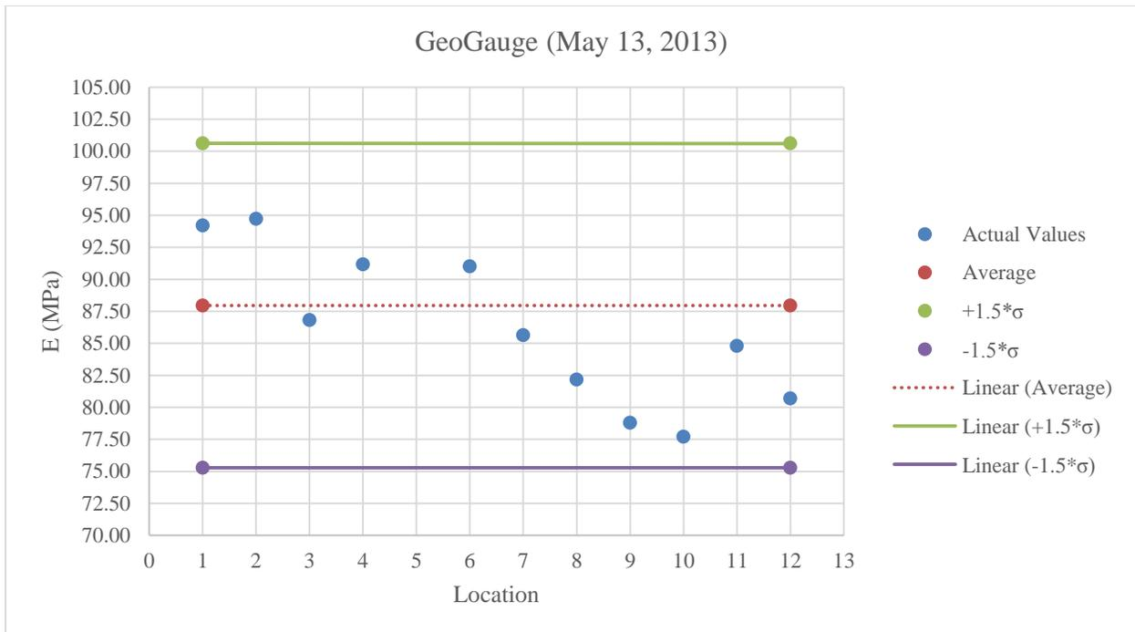
**Figure B.26:** GeoGauge testing on stabilized subgrade at optimum moisture content
