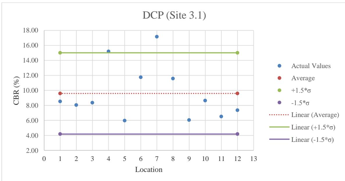
**Figure E.22:** DCP testing results on A-3 material
