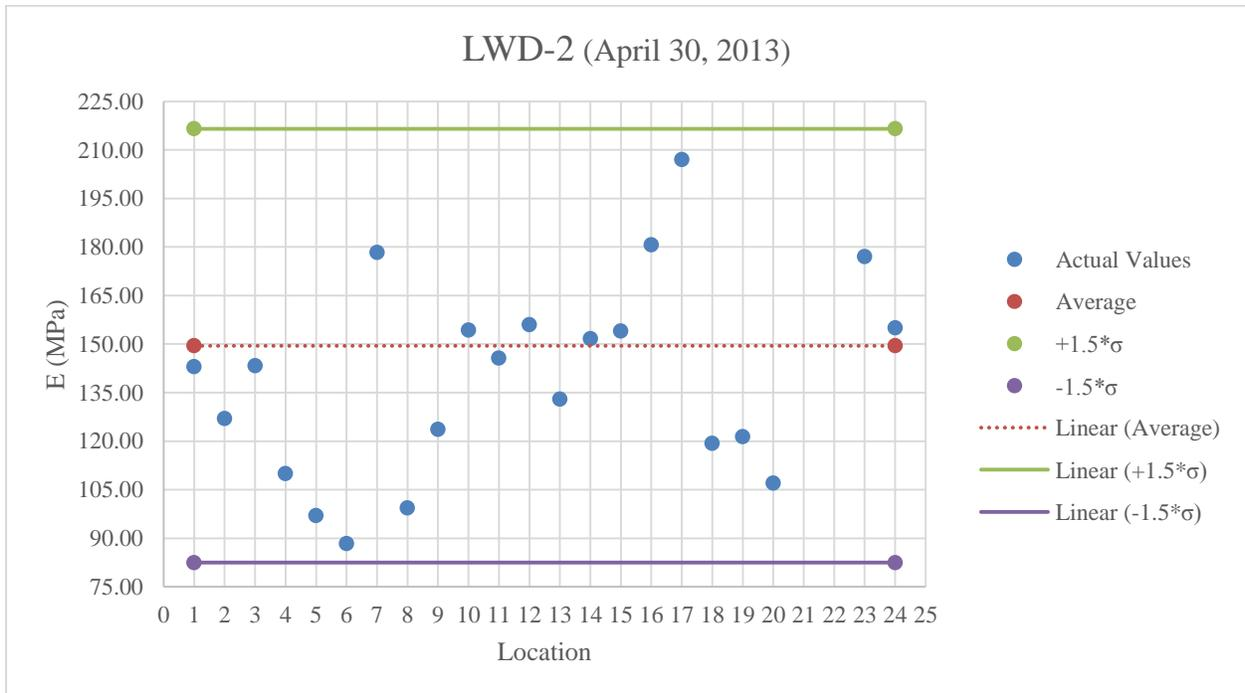
**Figure B.36:** LWD-2 testing on A-2-4 at optimum moisture content
