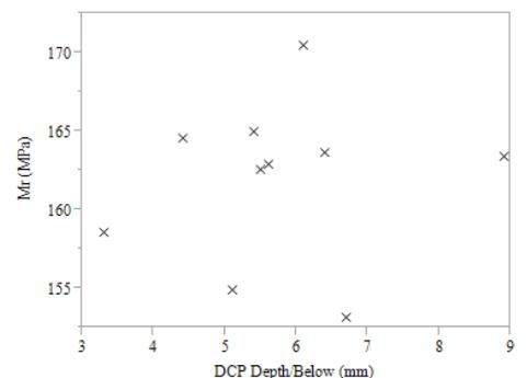
**Figure F.3:** Scatterplot of laboratory resilient modulus vs. DCP (depth per blow) measurements (mm)
