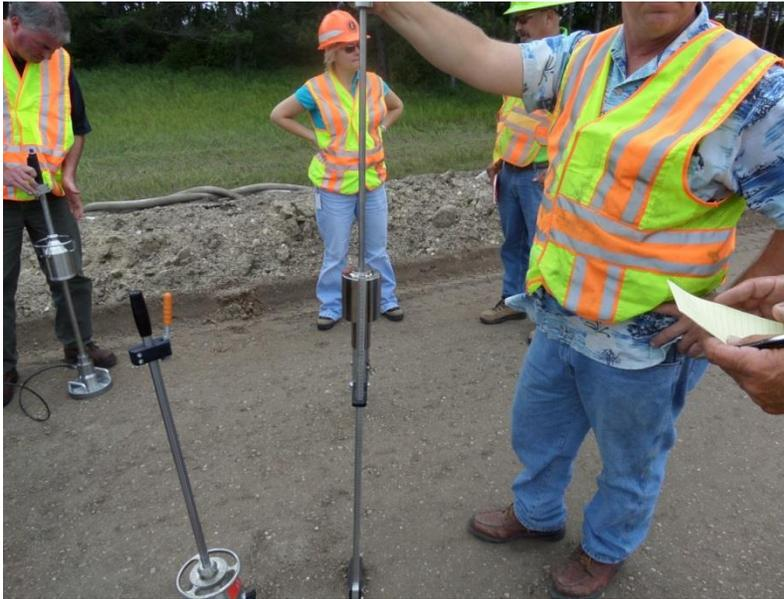
**Figure 7.7:** Photograph of Mn/DOT LWDs and DCP on Class 5 aggregate base
