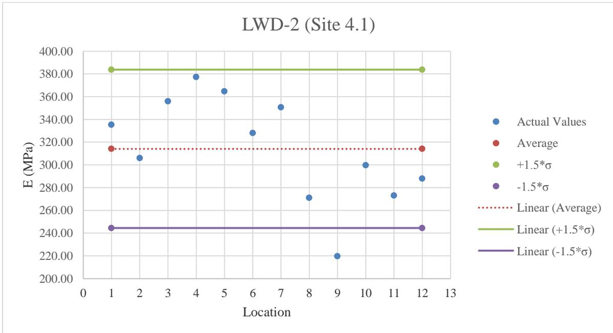
Figure E.30: LWD-2 testing results on stabilized subgrade
