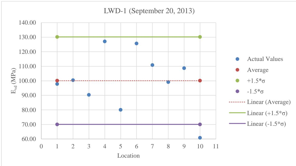
Figure C.37: Plot of LWD-1 values for limerock at 3% less than optimum moisture content
