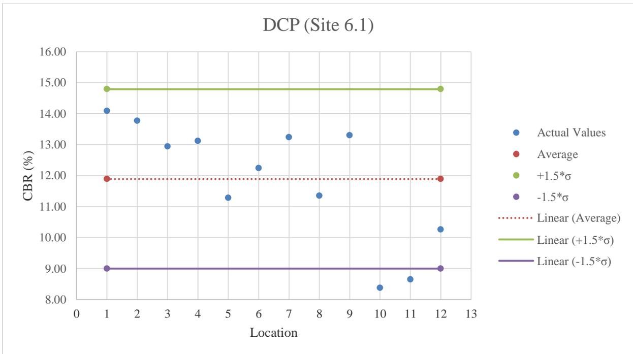
**Figure E.56:** DCP testing results on A-3 material
