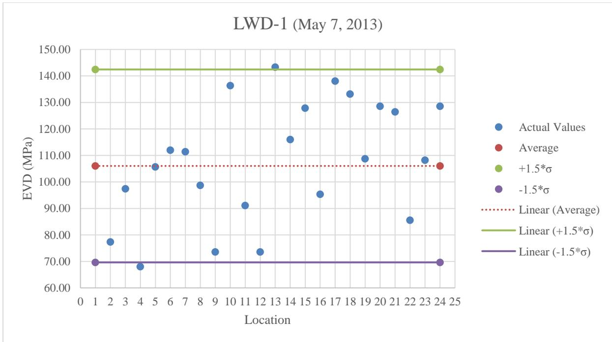
**Figure B.31:** LWD-1 testing on A-2-4 below optimum moisture content
