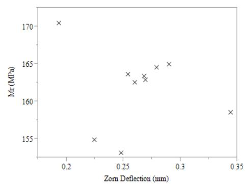
**Figure F.8:** Scatterplot of lab resilient modulus vs. LWD-1 deflection measurements (mm)
