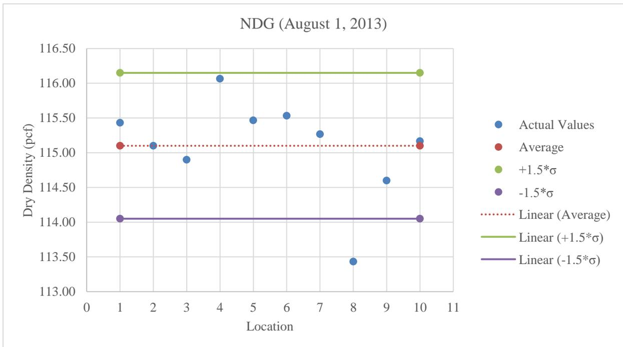
**Figure C.48:** Plot of NDG values for stabilized subgrade at optimum moisture content
