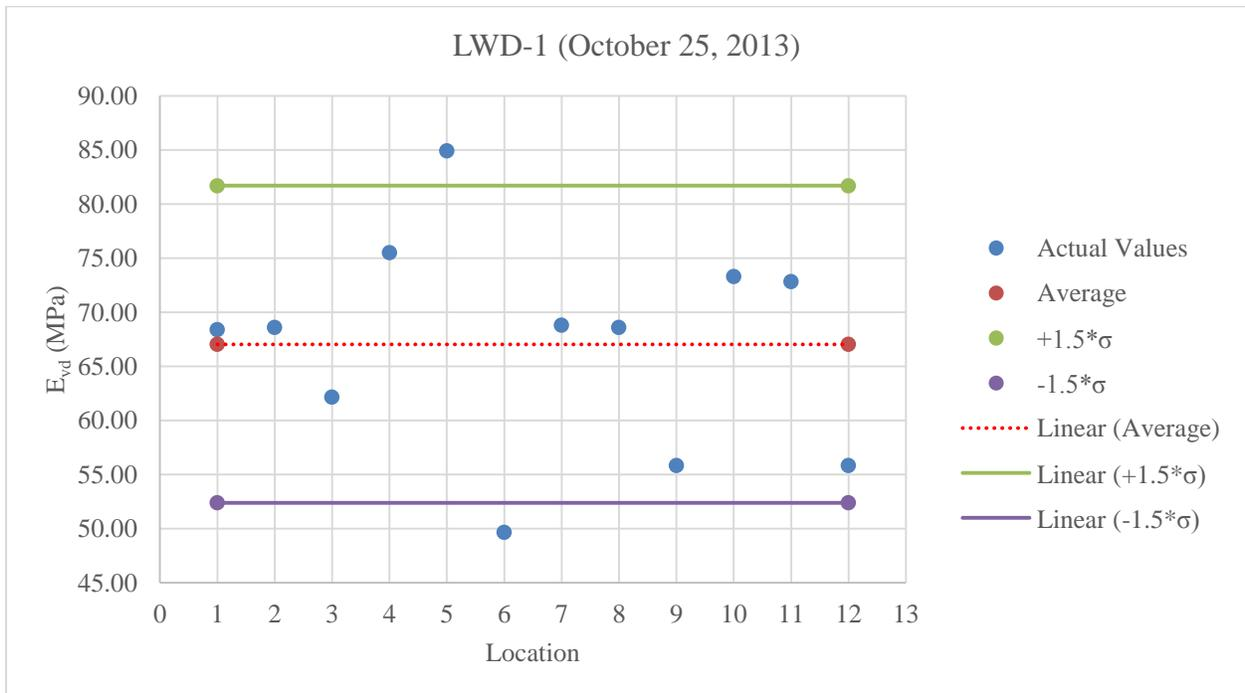
**Figure C.22:** Plot of LWD-1 values for A-2-4 low fines at 6% less than optimum moisture content
