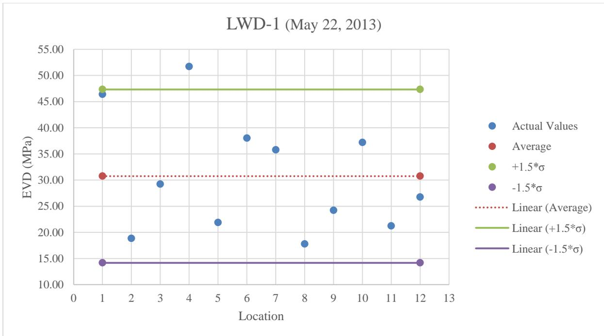
**Figure B.34:** LWD-1 testing on stabilized subgrade above optimum moisture content
