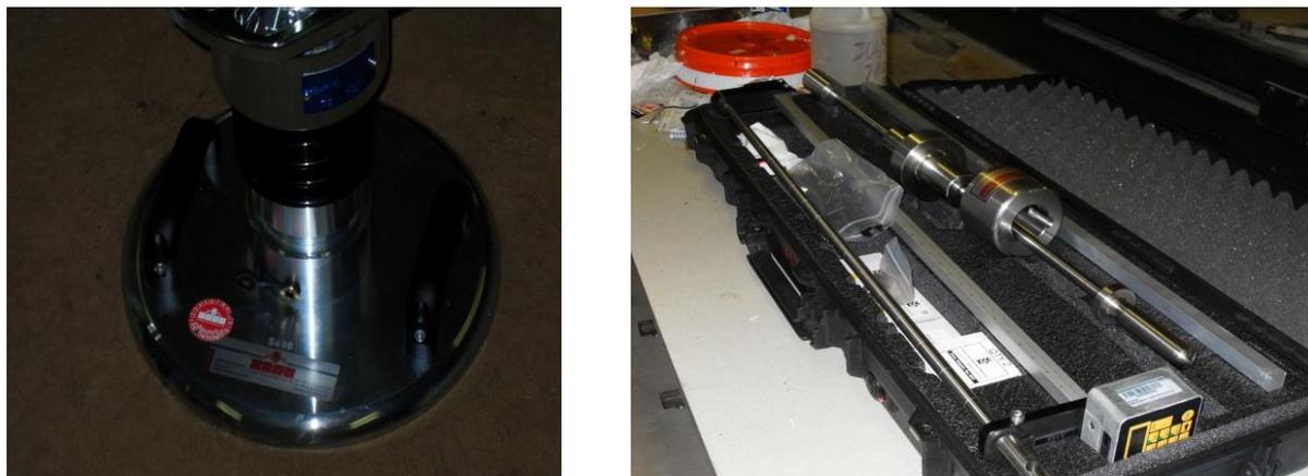
**Figure 3.1:** Photographs of testing equipment purchased (LWD-1, left; DCP, right)
