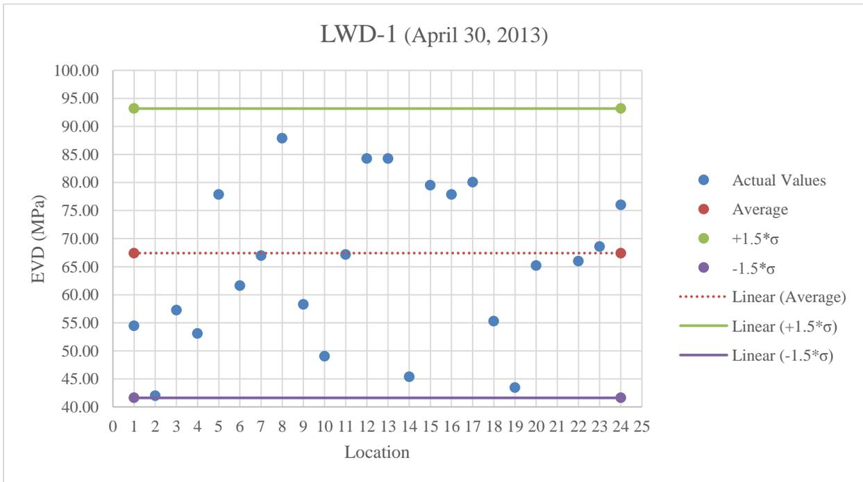
**Figure B.30:** LWD-1 testing on A-2-4 at optimum moisture content
