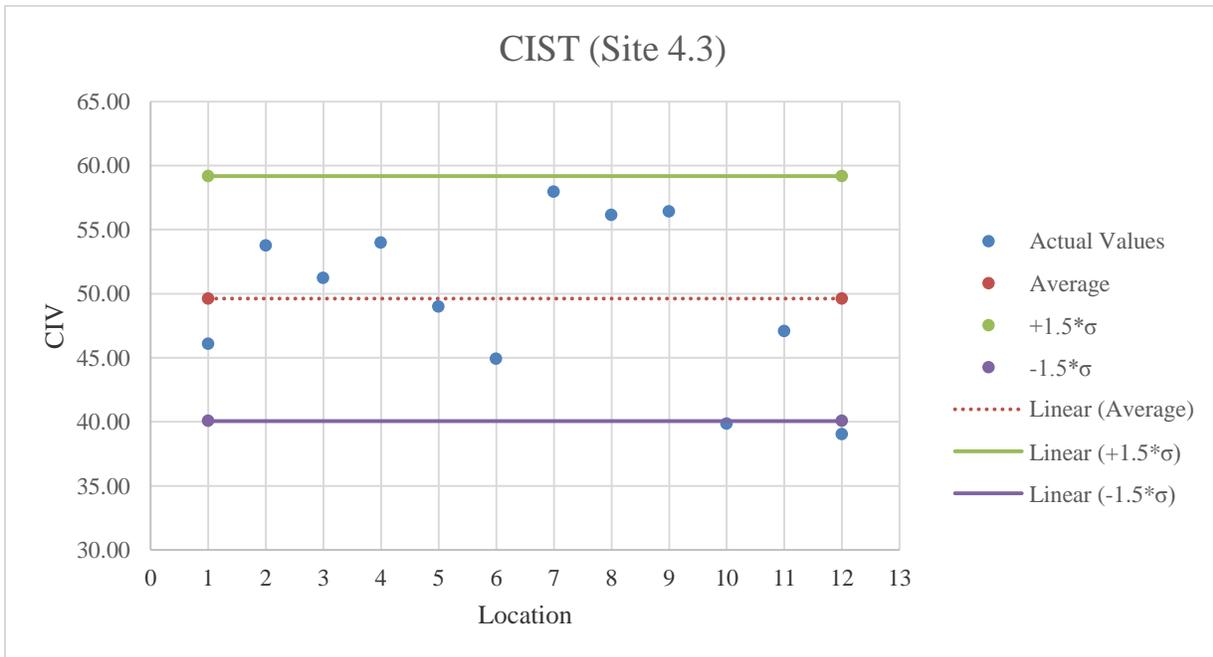
**Figure E.40:** CIST testing results on stabilized subgrade
