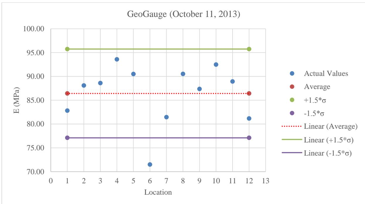
Figure C.16: Plot of GeoGauge values for A-2-4 low fines at optimum moisture content
