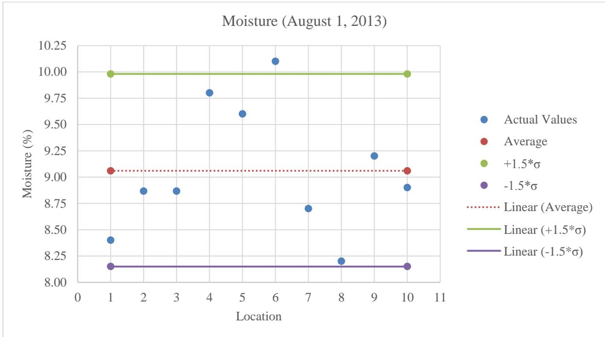
**Figure C.49:** Plot of moisture values for stabilized subgrade
