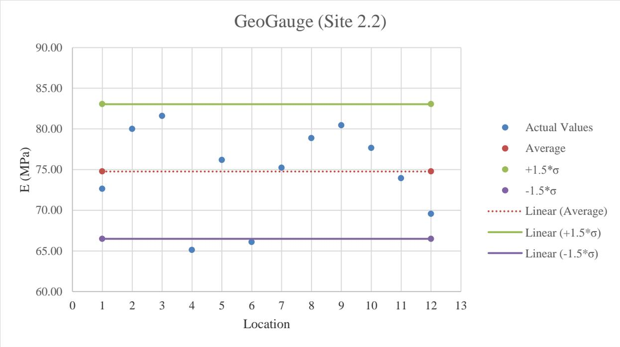
**Figure E.17:** GeoGauge testing results on A-2-4 material
