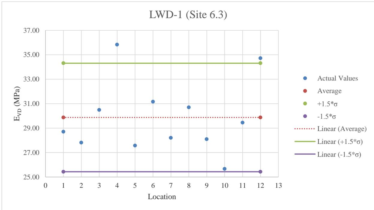
**Figure E.61:** LWD-1 testing results on A-3 material
