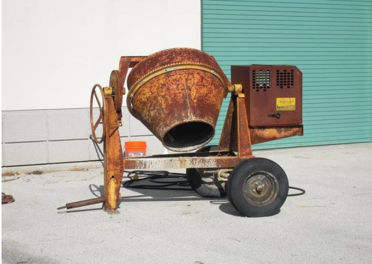
**Figure 3.3:** Photograph of mixer used to achieve target moisture contents
