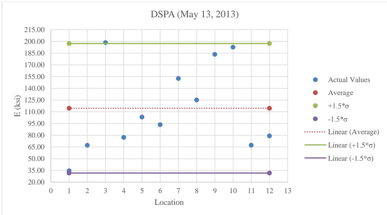
**Figure B.12:** DSPA testing on stabilized subgrade at optimum moisture content
