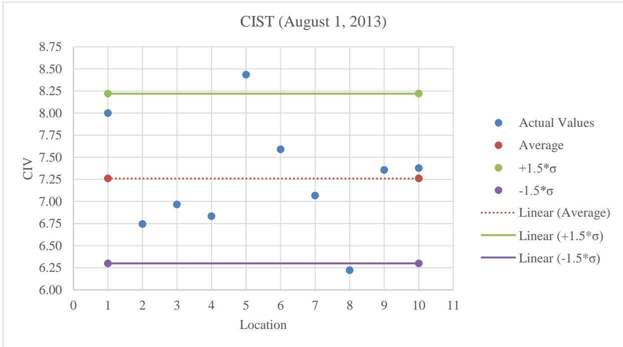
**Figure C.47:** Plot of CIST values for stabilized subgrade at optimum moisture content
