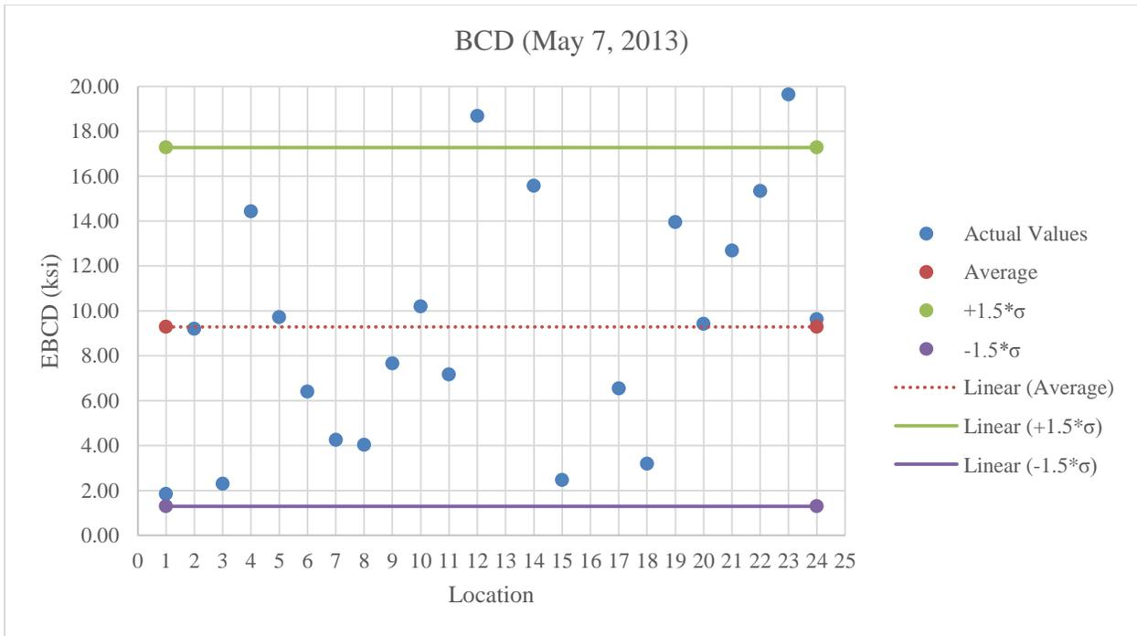
**Figure B.3:** BCD testing on A-2-4 below optimum moisture content
