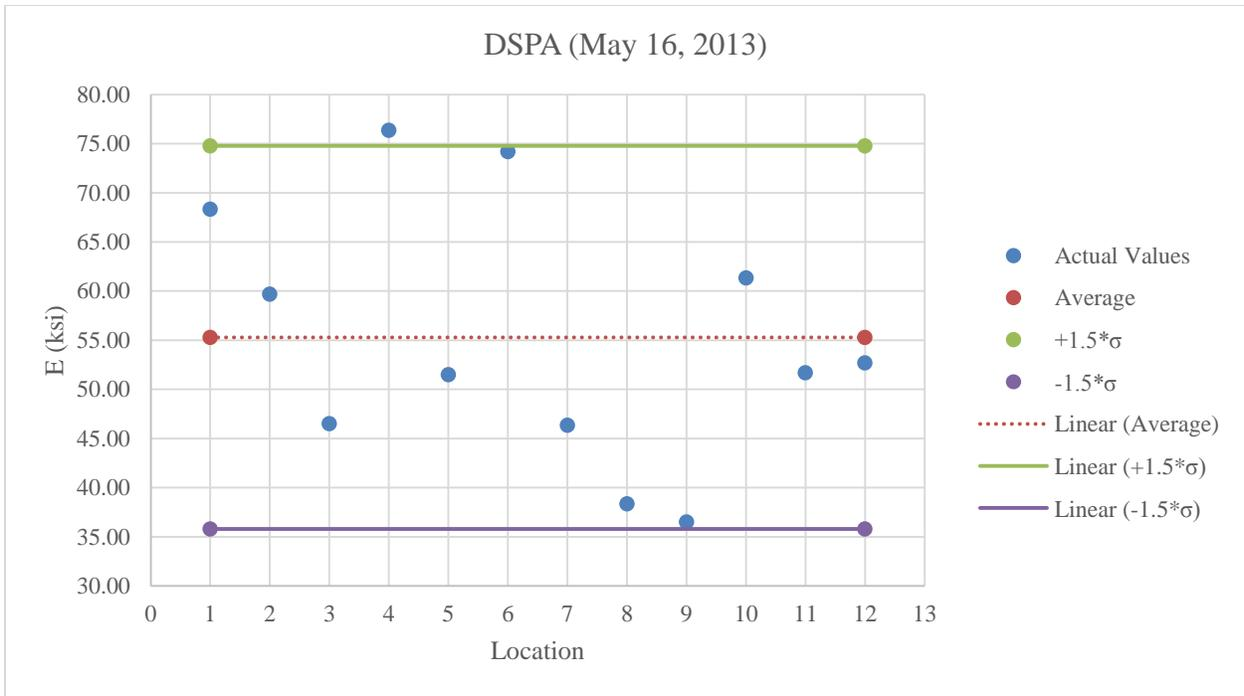
**Figure B.13:** DSPA testing on stabilized subgrade below optimum moisture content
