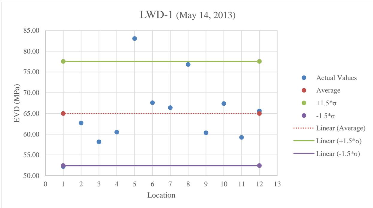
**Figure B.32:** LWD-1 testing on stabilized subgrade at optimum moisture content
