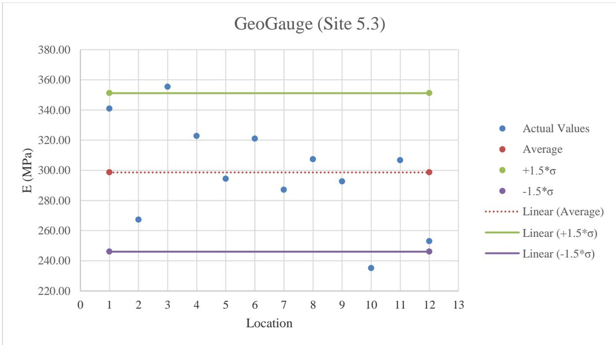
**Figure E.51:** GeoGauge testing results on limerock material
