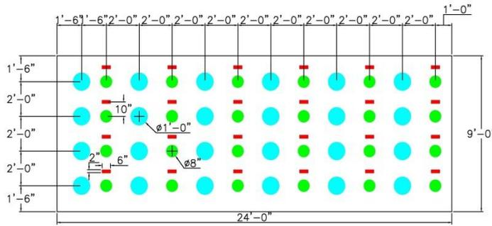
**Figure 3-13.1: Test Pit with LWD-1, BCD, and DCP**
