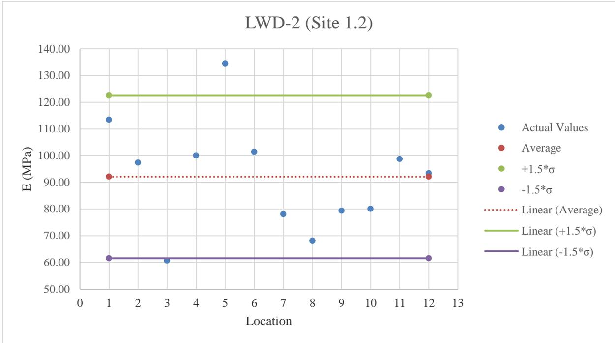
**Figure E.5:** LWD-2 testing results on GAB material
