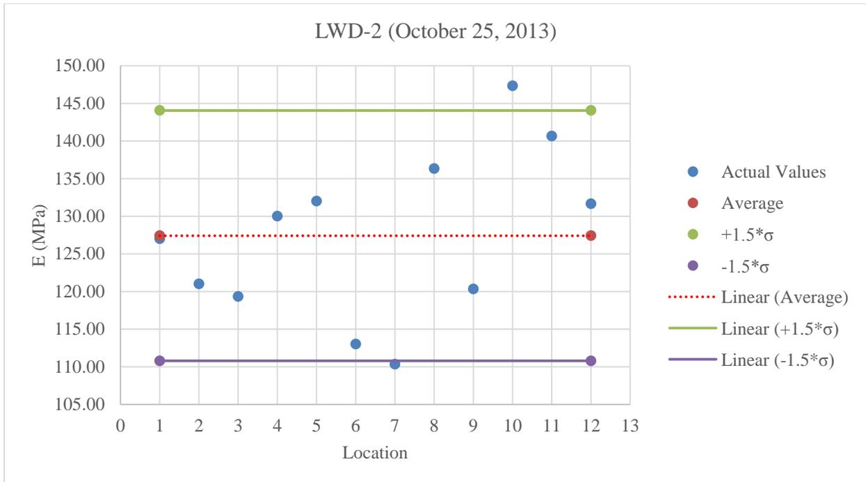
**Figure C.23:** Plot of LWD-2 values for A-2-4 low fines at 6% less than optimum moisture content
