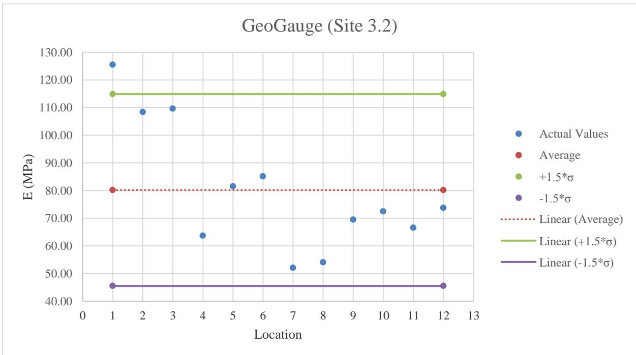
**Figure E.24:** GeoGauge testing results on A-3 material
