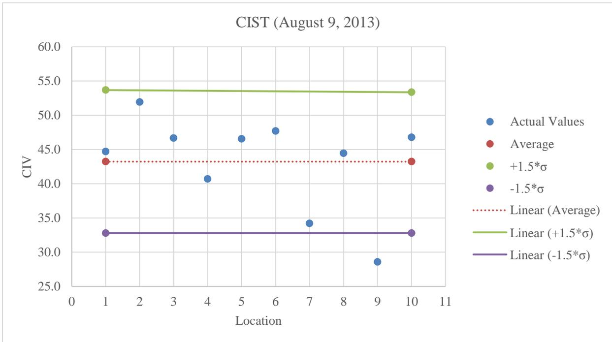
**Figure C.33:** Plot of CIST values for limerock at optimum moisture content
