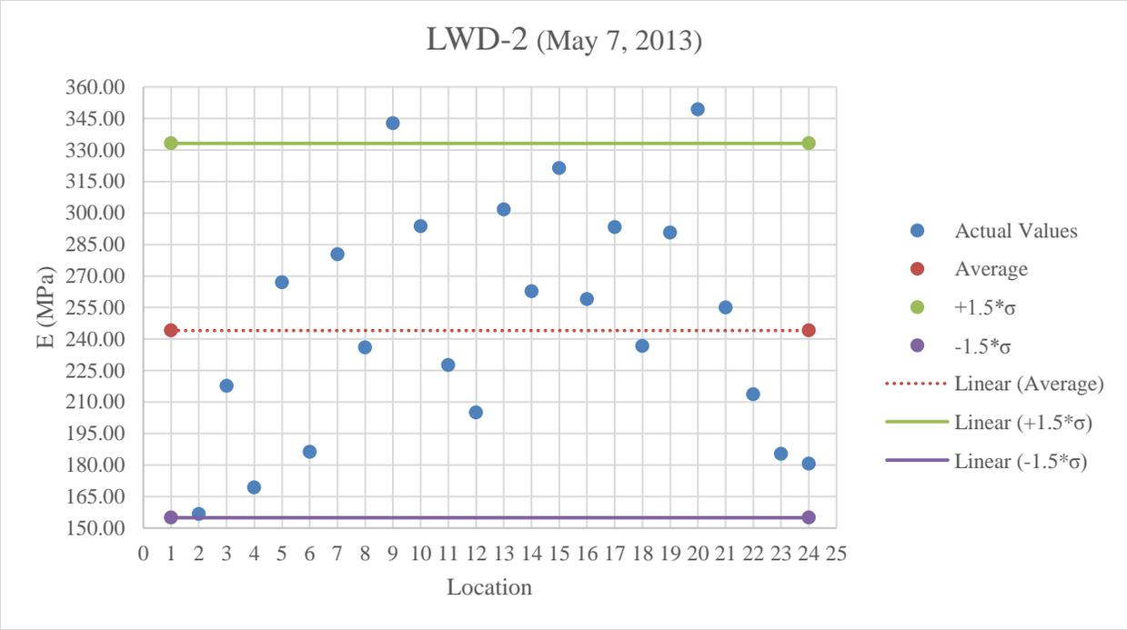
**Figure B.37:** LWD-2 testing on A-2-4 below optimum moisture content
