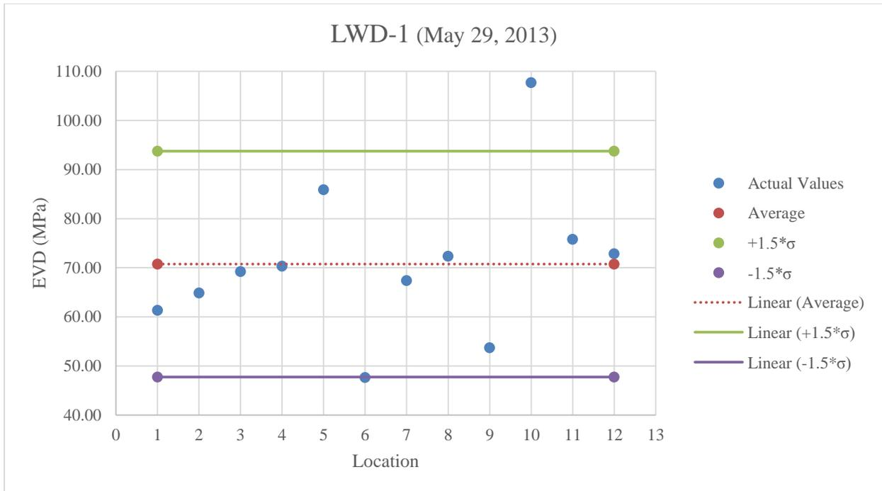
**Figure B.35:** LWD-1 testing on A-2-4 below optimum moisture content
