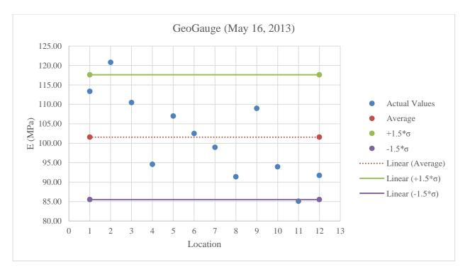
Figure B.27: GeoGauge testing on stabilized subgrade below optimum moisture content
