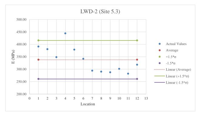
Figure E.50: LWD-2 testing results on limerock material
