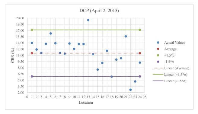
Figure B.16: DCP testing on A-3 below optimum moisture content
