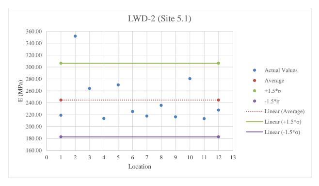
Figure E.42: LWD-2 testing results on limerock material
