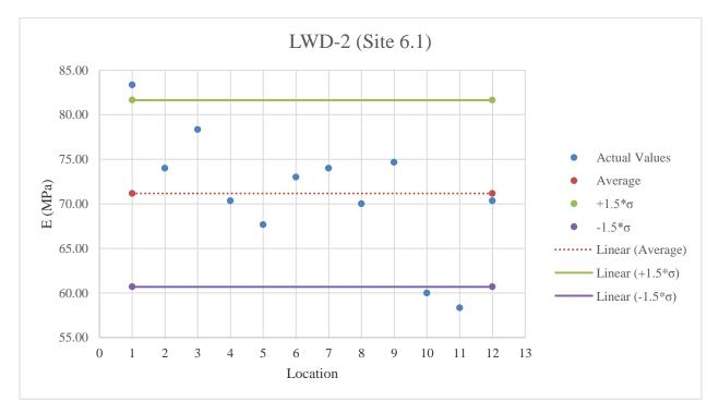
Figure E.54: LWD-2 testing results on A-3 material
