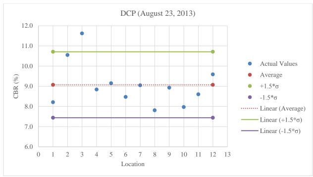
Figure C.3: Plot of DCP values for A-3 at optimum moisture content
