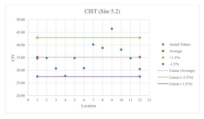
Figure E.48: CIST testing results on limerock material
