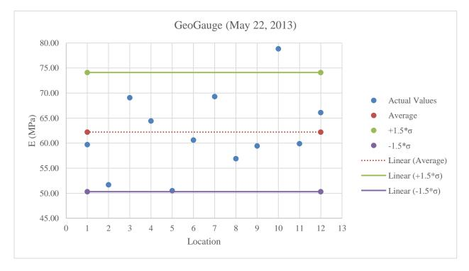
Figure B.28: GeoGauge testing on stabilized subgrade above optimum moisture content
