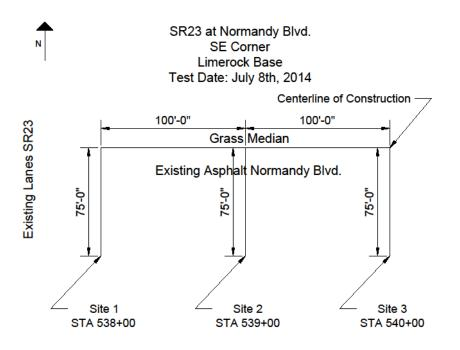
Figure 5.32: Project Site #5 SR-23 limerock base - Test site location sketch
