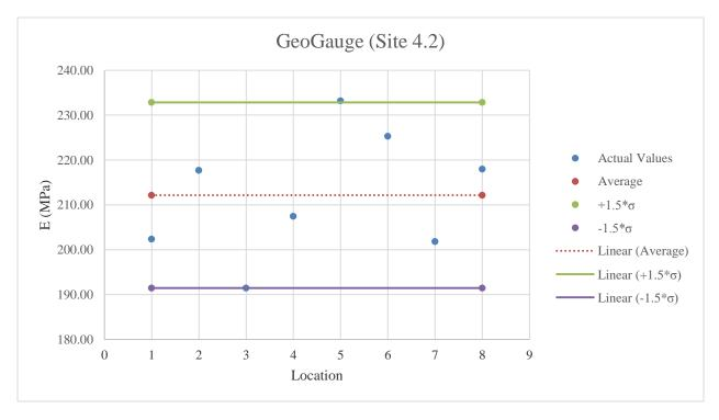
Figure E.36: GeoGauge testing results on stabilized subgrade
