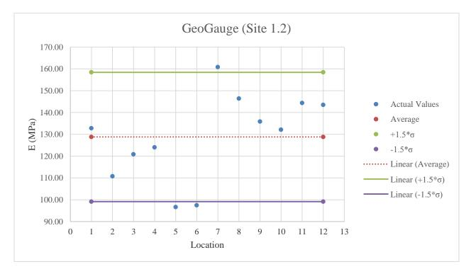
Figure E.6: GeoGauge testing results on GAB material
