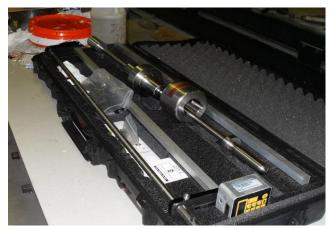
**Figure 3.1:** Photographs of testing equipment purchased (LWD-1, left; DCP, right)
