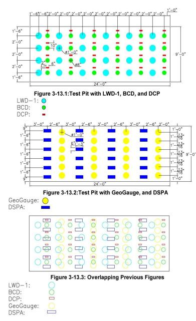
Figure 3.13: Plan of Phase I testing locations in the test pit
