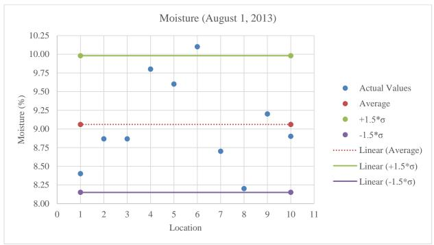
Figure C.49: Plot of moisture values for stabilized subgrade
