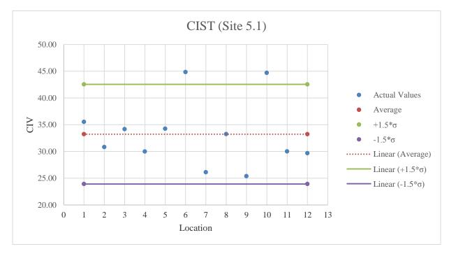
Figure E.44: CIST testing results on limerock material
