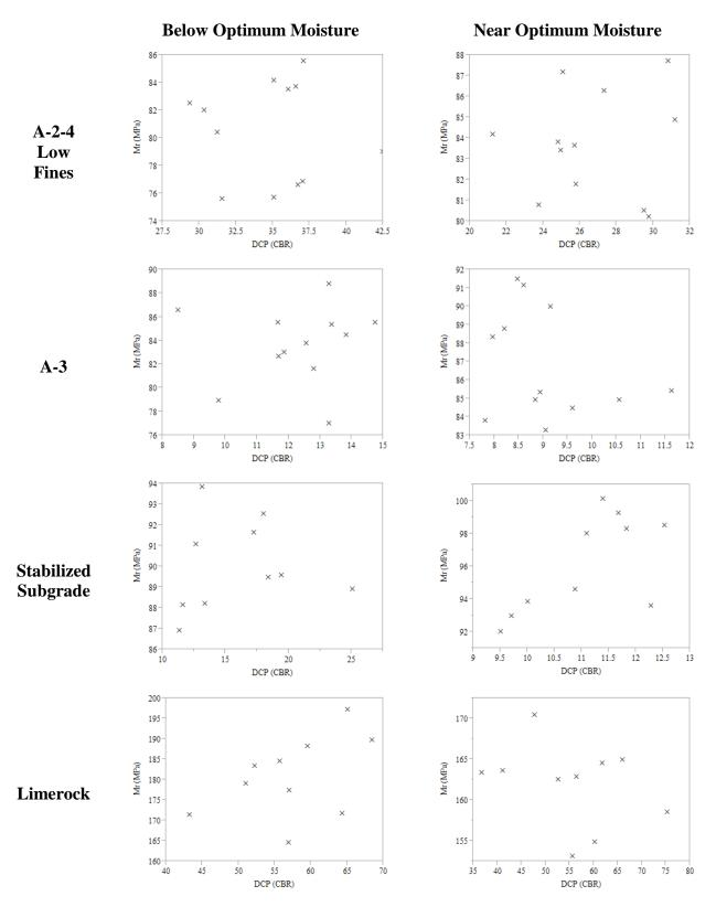
**Figure F.2:** Scatterplot of laboratory resilient modulus vs. DCP measurements (CBR) (See Section F.1.4 for discussion)
