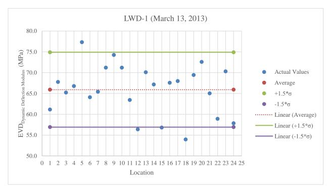
Figure B.29: LWD-1 testing on A-3 at optimum moisture content
