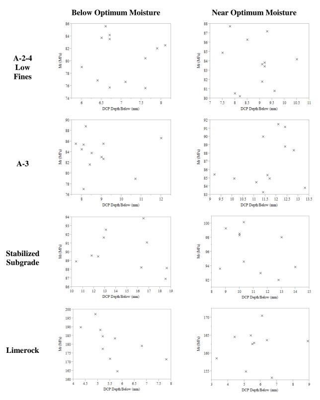
Figure F.3: Scatterplot of laboratory resilient modulus vs. DCP (depth per blow) measurements (mm)
