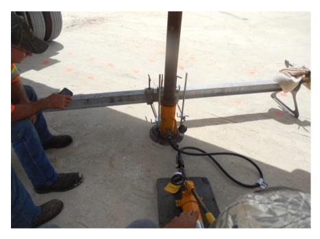
**Figure 5.27:** Project Site #4 CR-210 - Photograph of PLT equipment Two nuclear densities and moistures are run at each of the three sites.
