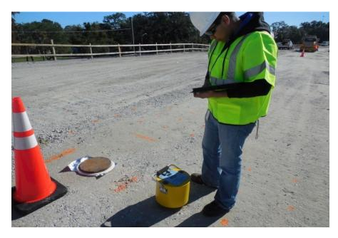
Figure 5.4: Project Site #1 I-95 - Photograph of GeoGauge and plate load testing
