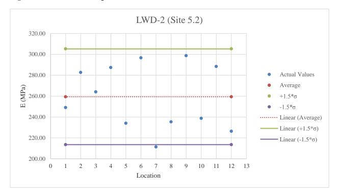
Figure E.46: LWD-2 testing results on limerock material
