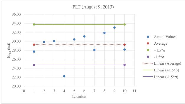
Figure C.36: Plot of PLT values for limerock at optimum moisture content
