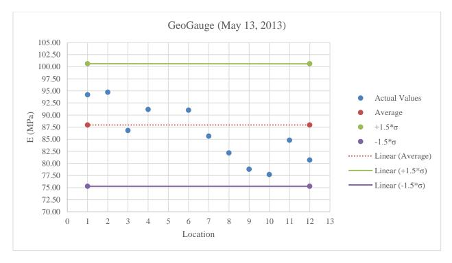
Figure B.26: GeoGauge testing on stabilized subgrade at optimum moisture content
