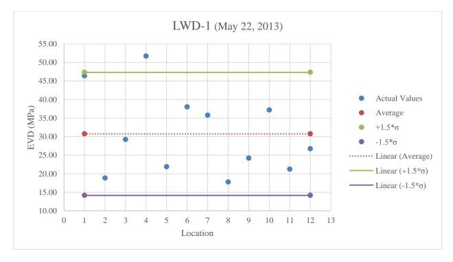
Figure B.34: LWD-1 testing on stabilized subgrade above optimum moisture content
