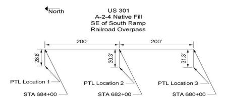
Figure 5.13: Project Site #2 US-301 - East service road test site location sketch
