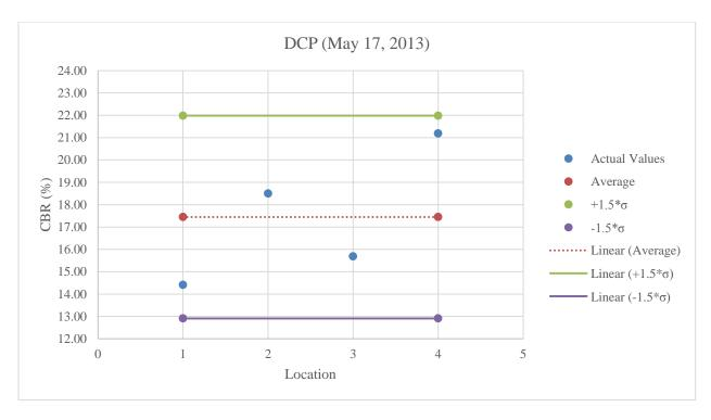
Figure B.19: DCP testing on stabilized subgrade below optimum moisture content
