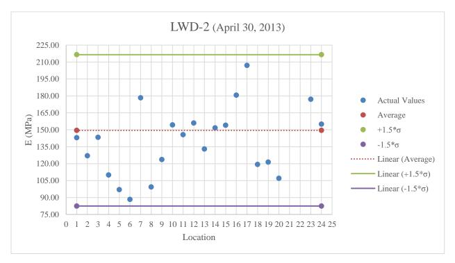
Figure B.36: LWD-2 testing on A-2-4 at optimum moisture content
