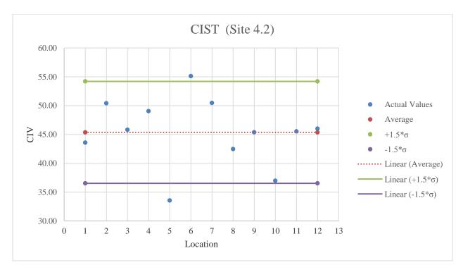
Figure E.37: CIST testing results on stabilized subgrade
