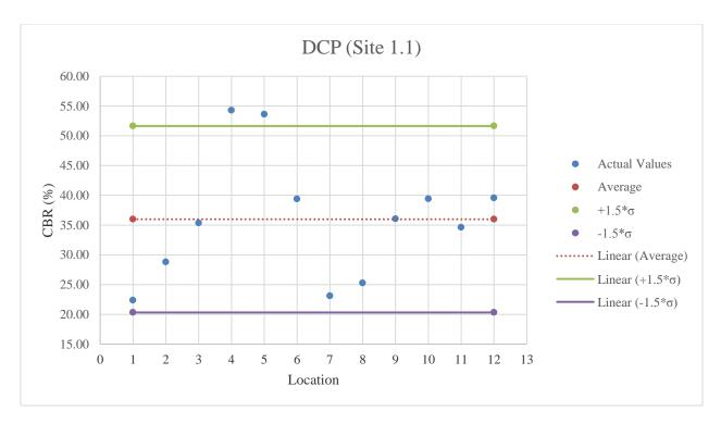
Figure E.3: DCP testing results on GAB material
