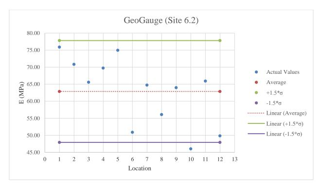
Figure E.59: GeoGauge testing results on A-3 material
