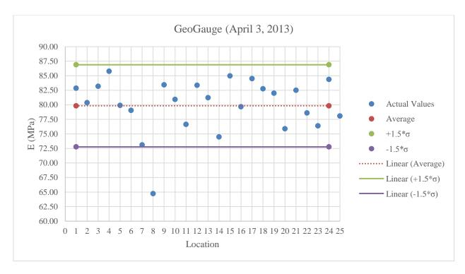
Figure B.23: GeoGauge testing on A-3 below optimum moisture content
