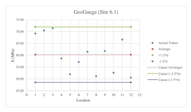
Figure E.55: GeoGauge testing results on A-3 material
