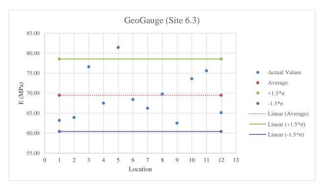
Figure E.63: GeoGauge testing results on A-3 material
