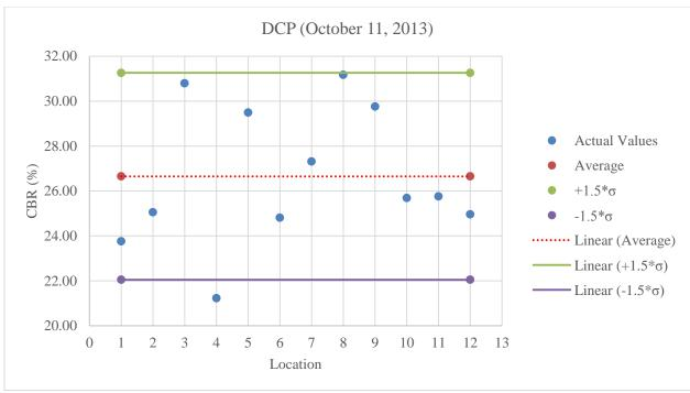
Figure C.17: Plot of DCP values for A-2-4 low fines at optimum moisture content
