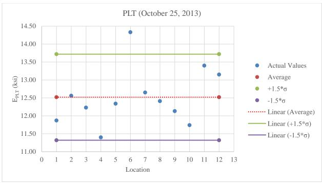
Figure C.29: Plot of PLT values for A-2-4 low fines at 6% less than optimum moisture content
