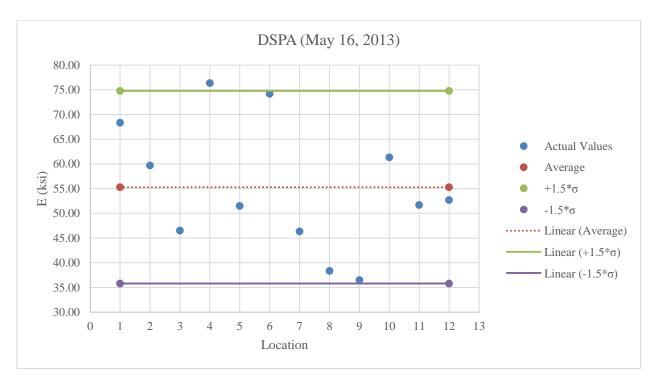
Figure B.13: DSPA testing on stabilized subgrade below optimum moisture content
