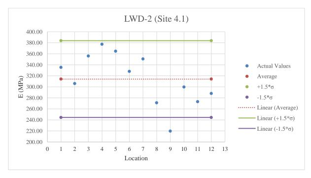
Figure E.30: LWD-2 testing results on stabilized subgrade
