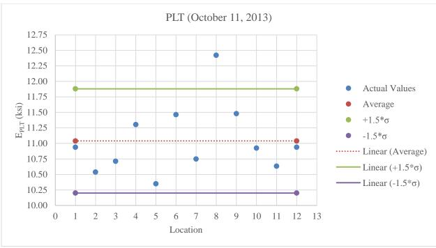
Figure C.21: Plot of PLT values for A-2-4 low fines at optimum moisture content
