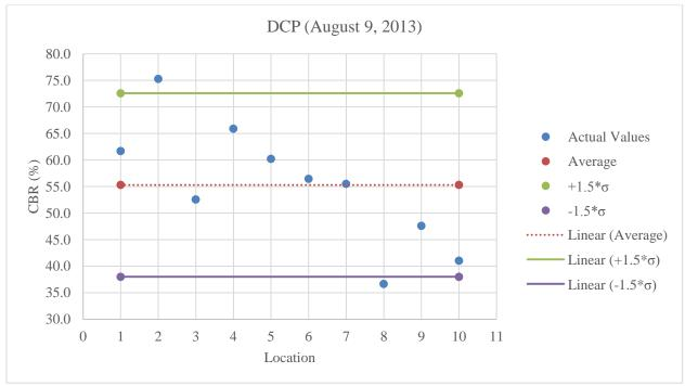
Figure C.32: Plot of DCP values for limerock at optimum moisture content
