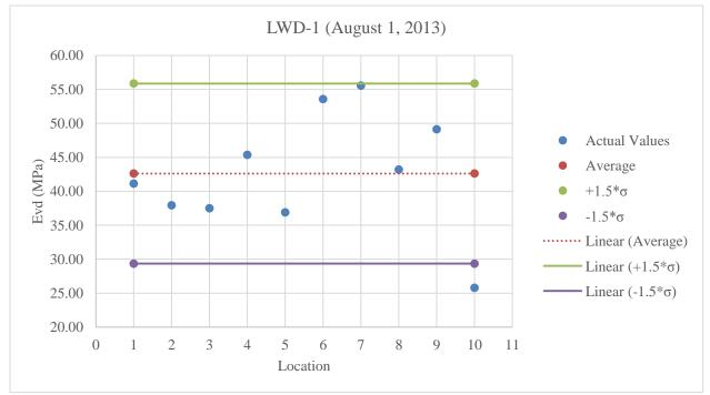
C.7 Results for Devices with Stabilized Subgrade Material at Optimum Moisture Content
