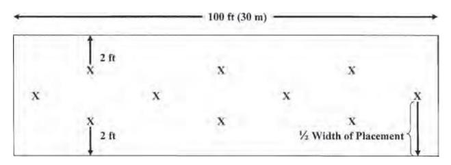
optimum moisture content. Ten LWD tests will be performed on the test section at the following approximate locations:
