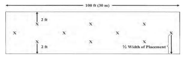
Figure 8.1: INDOT test section for LWD (for reference as DCP test section)
