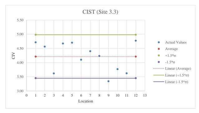
Figure E.28: CIST testing results on A-3 material
