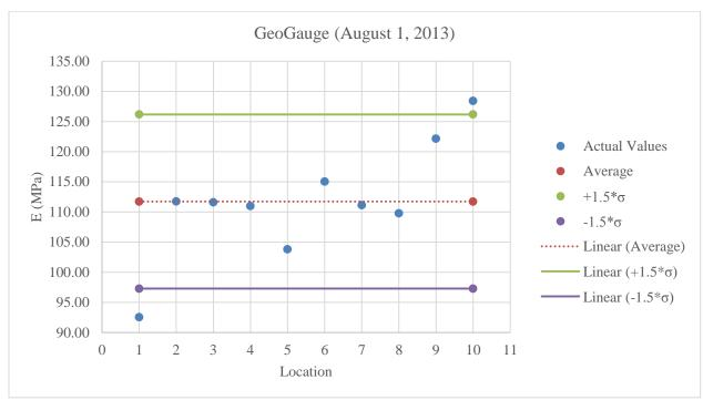
Figure C.45: Plot of GeoGauge values for stabilized subgrade at optimum moisture content
