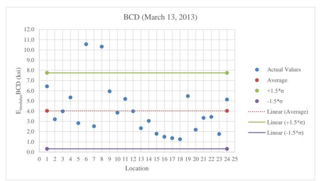
**Figure B.1:** BCD testing on A-3 at optimum moisture content (In kilopounds per square inch, *ksi*)
