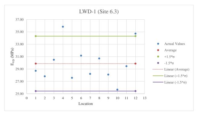
Figure E.61: LWD-1 testing results on A-3 material
