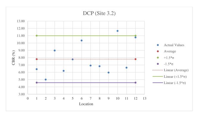
Figure E.25: DCP testing results on A-3 material
