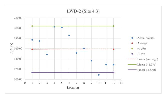
Figure E.39: LWD-2 testing results on stabilized subgrade
