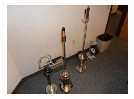
**Figure 7.5:** Photograph of LWDs (From left to right: Modified Prima 100, Zorn Model ZF 2000, and Olson Prototype)
