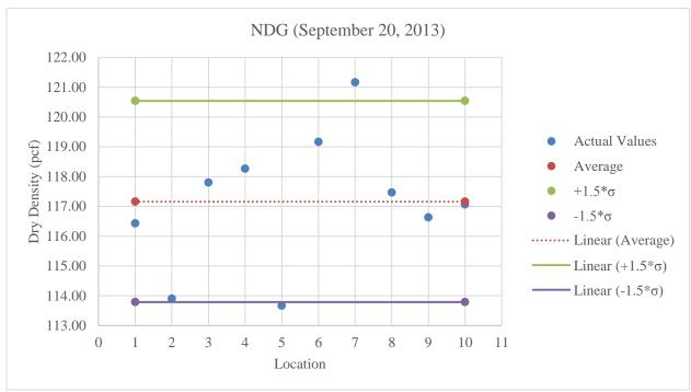
Figure C.41: Plot of NDG values for limerock at 3% less than optimum moisture content
