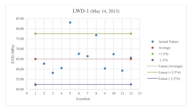
Figure B.32: LWD-1 testing on stabilized subgrade at optimum moisture content
