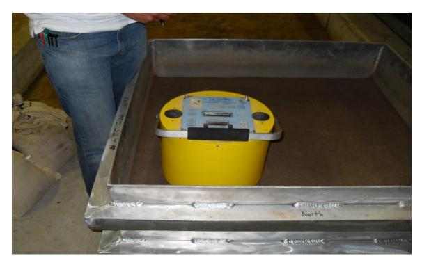
Figure 3.9: Photograph of GeoGauge in test box
