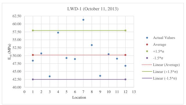
C.3 Results for Devices with A-2-4 Low Fines Material at Optimum Moisture Content
