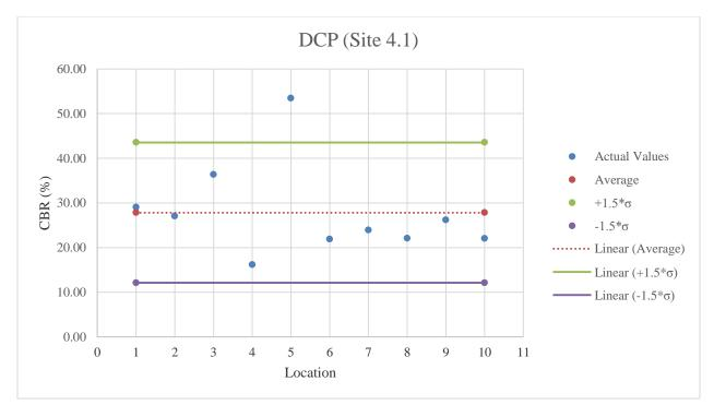
Figure E.32: DCP testing results on stabilized subgrade
