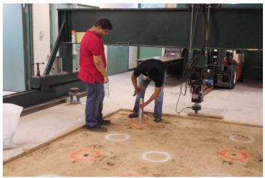
**Figure 4.6:** Photograph of east test pit limerock base ten moisture samples (One per each SSTS location)
