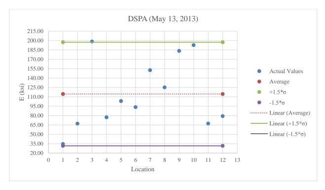
Figure B.12: DSPA testing on stabilized subgrade at optimum moisture content
