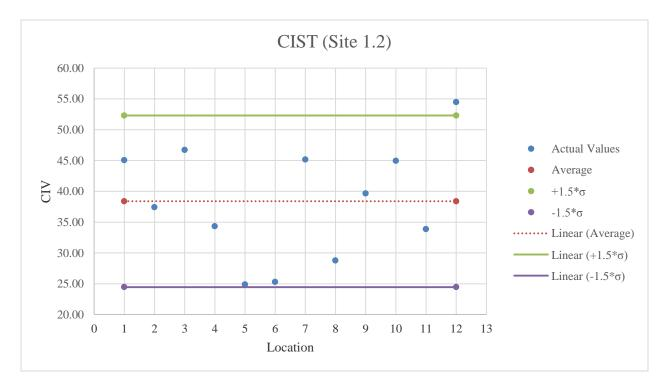
Figure E.8: CIST testing results on GAB material
