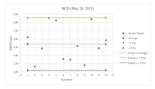
Figure B.6: BCD testing on stabilized subgrade above optimum moisture content
