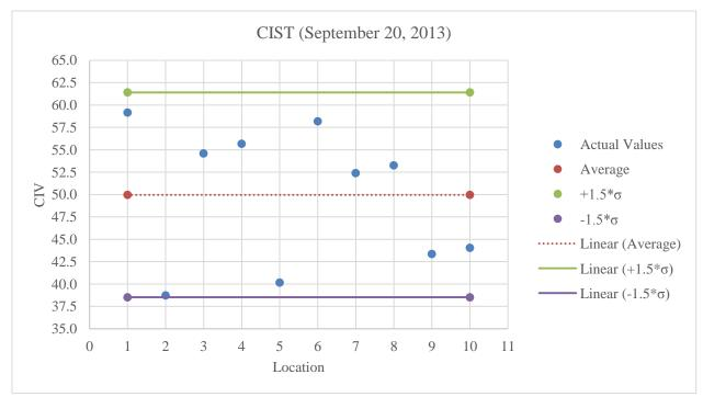
Figure C.40: Plot of CIST values for limerock at 3% less than optimum moisture content
