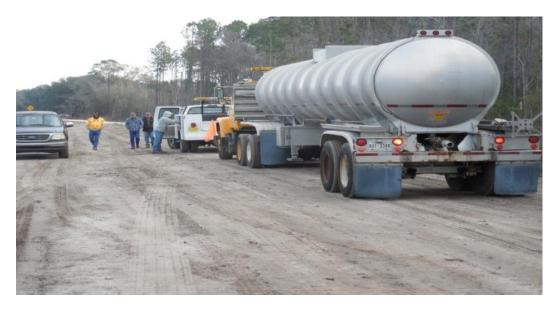
Figure 5.10: Project Site #2 US-301 - Photograph of PLT tanker used for ballast
