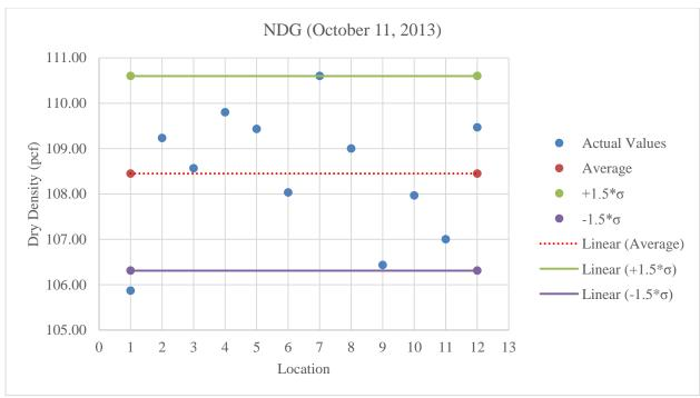
Figure C.19: Plot of NDG values for A-2-4 low fines at optimum moisture content
