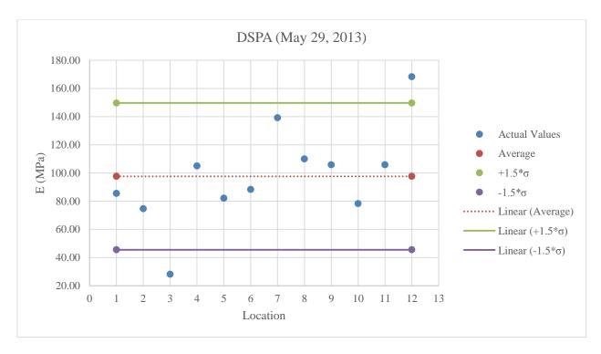
Figure B.15: DSPA testing on A-2-4 below optimum moisture content
