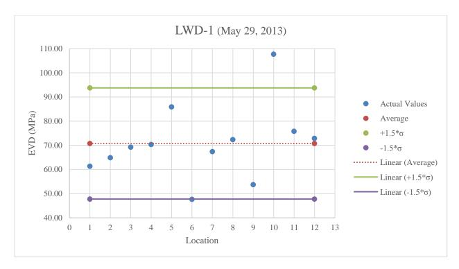
Figure B.35: LWD-1 testing on A-2-4 below optimum moisture content
