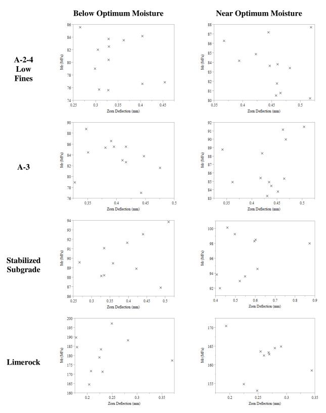
Figure F.8: Scatterplot of lab resilient modulus vs. LWD-1 deflection measurements (mm) (See Section 1.4 for discussion)
