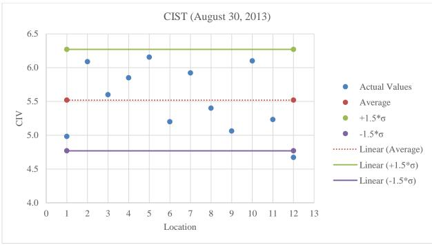
Figure C.11: Plot of CIST values for A-3 at 7% less than optimum moisture content
