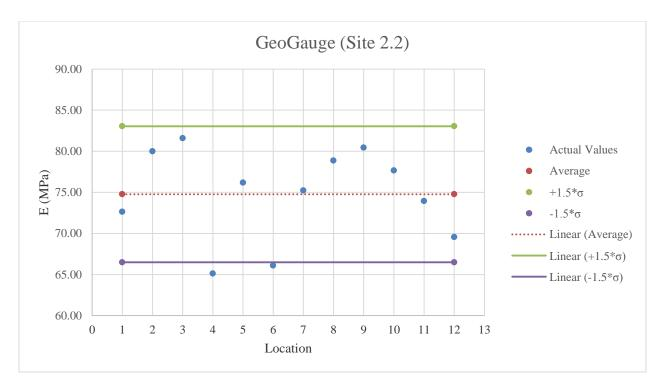
Figure E.17: GeoGauge testing results on A-2-4 material
