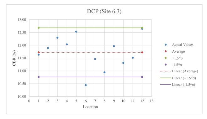
Figure E.64: DCP testing results on A-3 material
