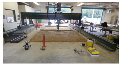
**Figure 4.3:** Photograph of east test pit looking south (Test equipment from left: DCP [in case], LWD-1, CIST, NDG, GeoGauge)
