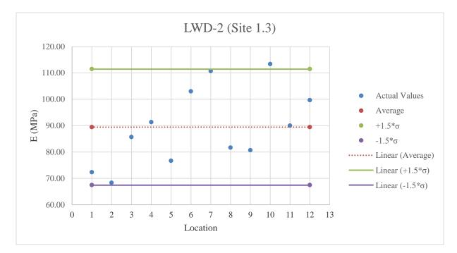
Figure E.9: LWD-2 testing results on GAB material
