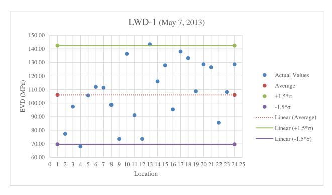
Figure B.31: LWD-1 testing on A-2-4 below optimum moisture content
