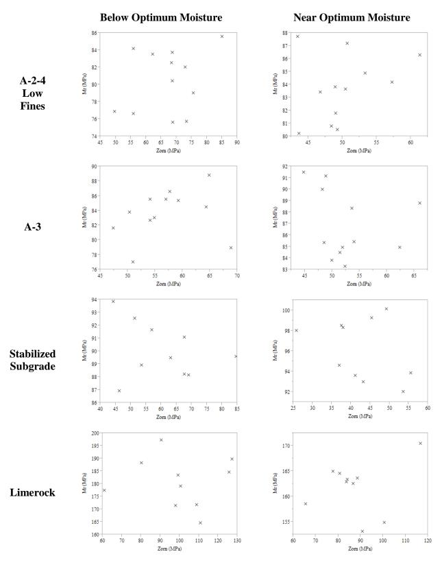
**Figure F.7:** Scatterplot of laboratory resilient modulus vs. LWD-1 measurements (MPa) (See Section F.1.4 for discussion)
