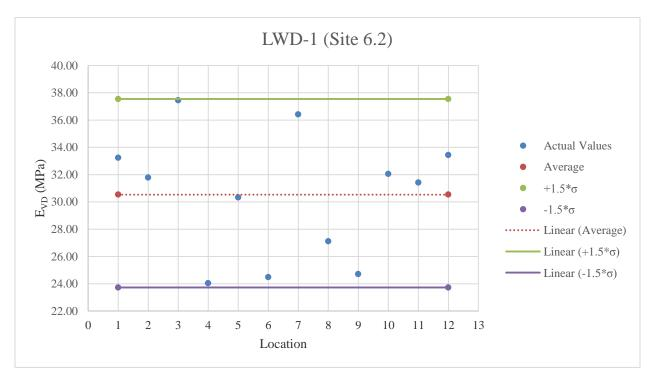
Figure E.57: LWD-1 testing results on A-3 material
