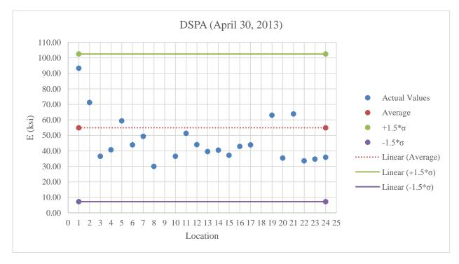
Figure B.10: DSPA testing on A-2-4 at optimum moisture content
