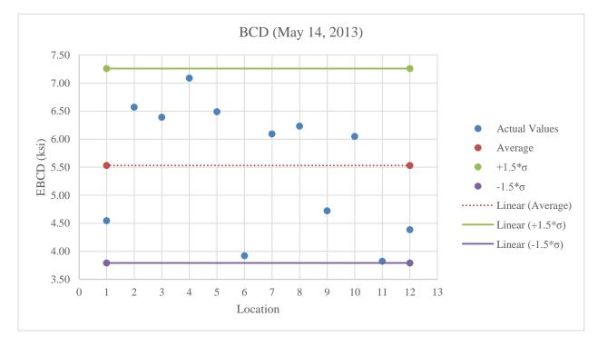
Figure B.4: BCD testing on stabilized subgrade at optimum moisture content
