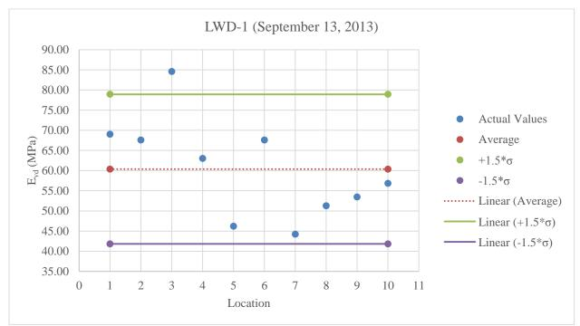
C.8 Results for Devices with Stabilized Subgrade Material below Optimum Moisture Content
