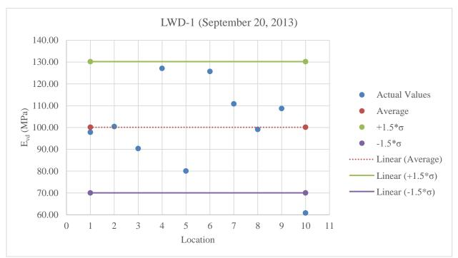
C.6 Results for Devices with Limerock Material below Optimum Moisture Content
