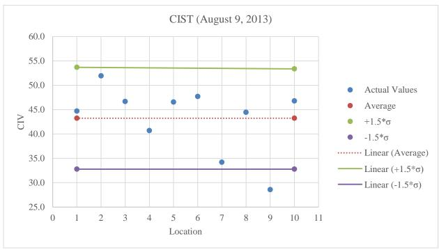
Figure C.33: Plot of CIST values for limerock at optimum moisture content
