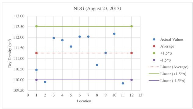
Figure C.5: Plot of NDG values for A-3 at optimum moisture content
