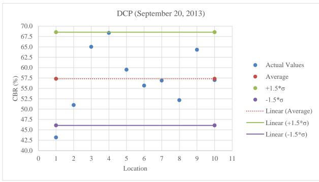
Figure C.39: Plot of DCP values for limerock at 3% less than optimum moisture content
