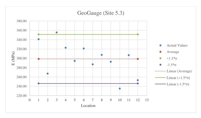
Figure E.51: GeoGauge testing results on limerock material
