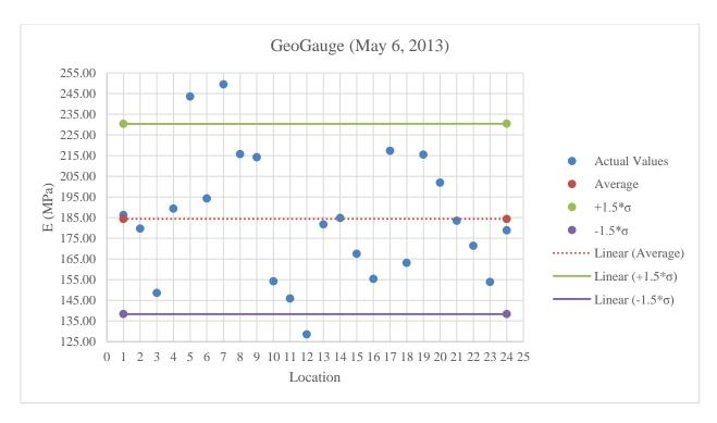
Figure B.25: GeoGauge testing on A-2-4 below optimum moisture content
