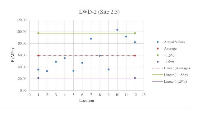
Figure E.19: LWD-2 testing results on A-2-4 material
