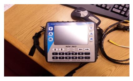
Figure 7.10: Photograph of Olson prototype LWD data collector
