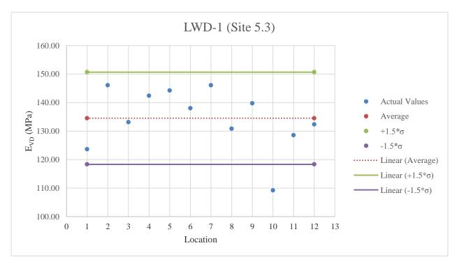
Figure E.49: LWD-1 testing results on limerock material
