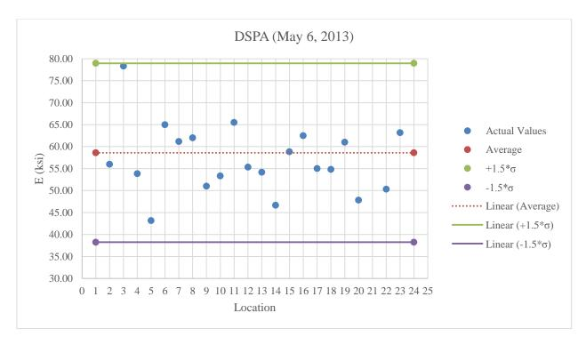
Figure B.11: DSPA testing on A-2-4 below optimum moisture content
