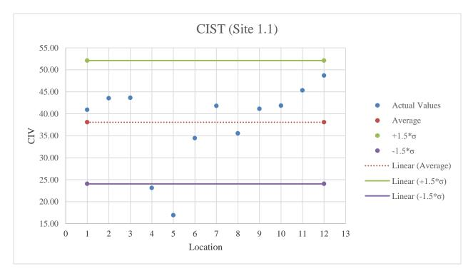
Figure E.4: CIST testing results on GAB material
