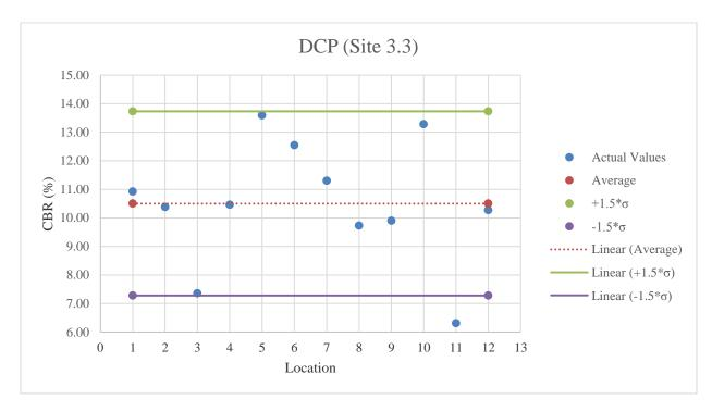
Figure E.27: DCP testing results on A-3 material
