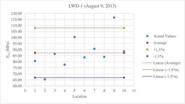
C.5 Results for Devices with Limerock Material at Optimum Moisture Content
