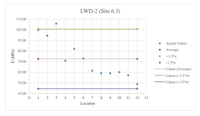
Figure E.62: LWD-2 testing results on A-3 material
