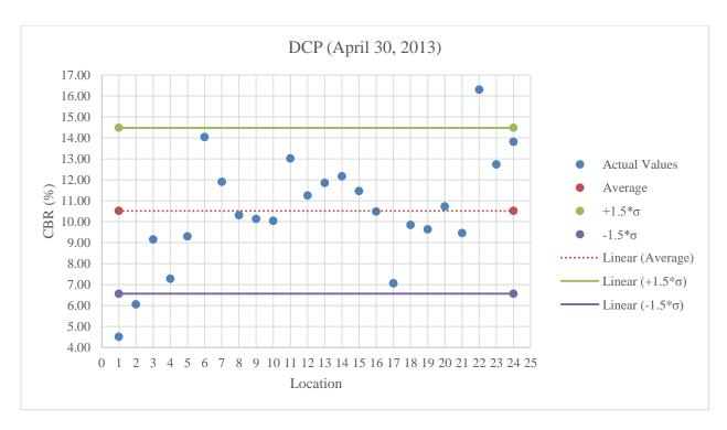
Figure B.17: DCP testing on A-2-4 at optimum moisture content
