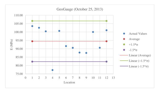
Figure C.24: Plot of GeoGauge values for A-2-4 low fines at 6% less than optimum moisture content
