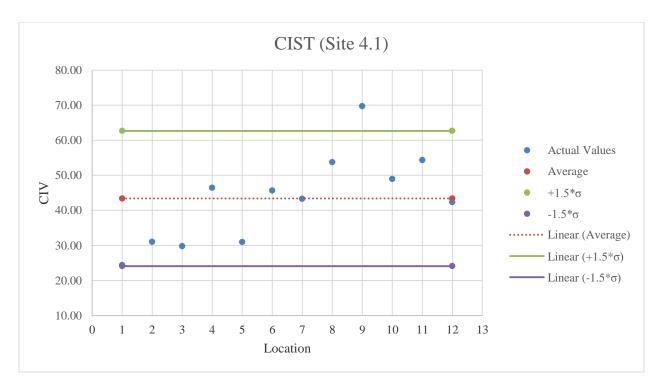
Figure E.33: CIST testing results on stabilized subgrade
