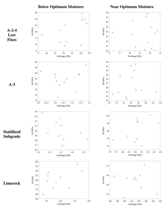
Figure F.4: Scatterplot of laboratory resilient modulus vs. GeoGauge measurements (MPa)
