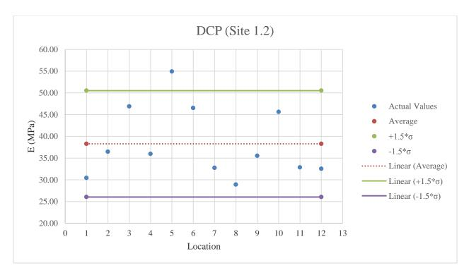
Figure E.7: DCP testing results on GAB material
