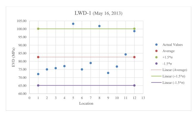
Figure B.33: LWD-1 testing on stabilized subgrade below optimum moisture content
