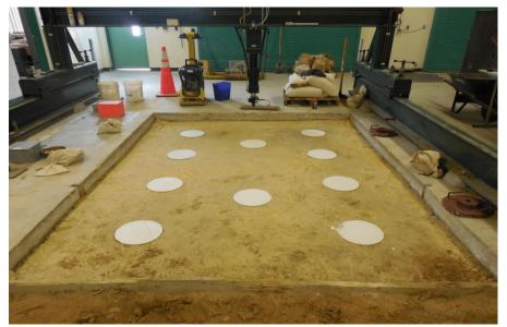
Figure 4.4: Photograph of east test pit limerock base ten PLT locations per half pit
