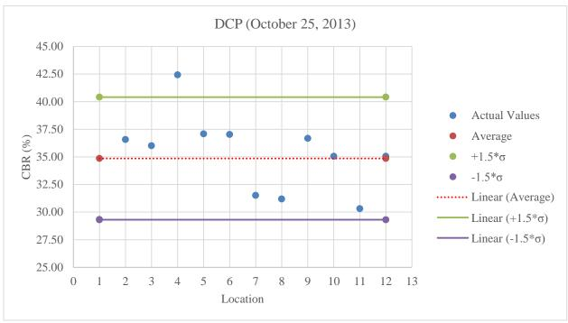
Figure C.25: Plot of DCP values for A-2-4 low fines at 6% less than optimum moisture content
