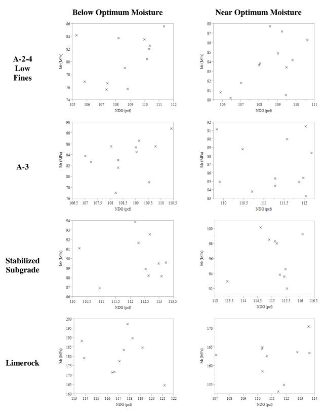
Figure F.5: Scatterplot of laboratory resilient modulus vs. NDG measurements (pcf)
