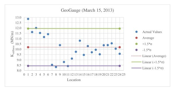
Figure B.22: GeoGauge testing on A-3 at optimum moisture content
