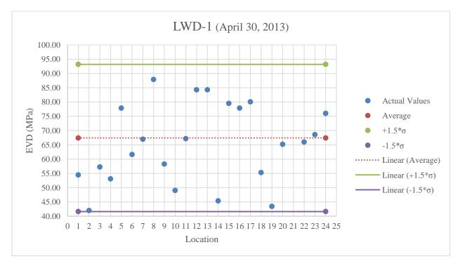
Figure B.30: LWD-1 testing on A-2-4 at optimum moisture content
