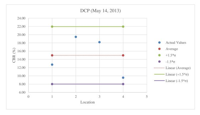
Figure B.18: DCP testing on stabilized subgrade at optimum moisture content
