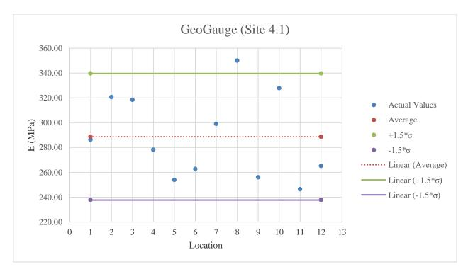
Figure E.31: GeoGauge testing results on stabilized subgrade
