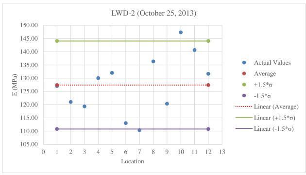
Figure C.23: Plot of LWD-2 values for A-2-4 low fines at 6% less than optimum moisture content
