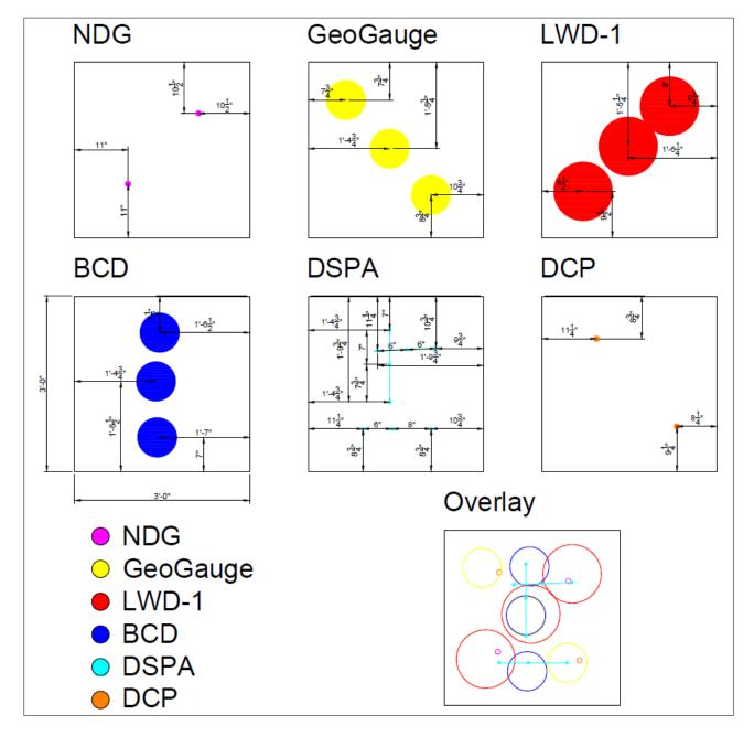
Figure 3.10: Testing device orientation in the test box
