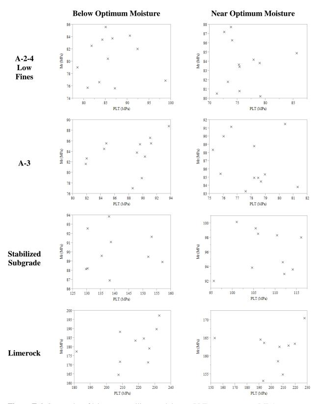
Figure F.6: Scatterplot of laboratory resilient modulus vs. PLT measurements (MPa)
