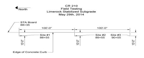
Figure 5.29: Project Site #4 CR-210 - Test location sketch
