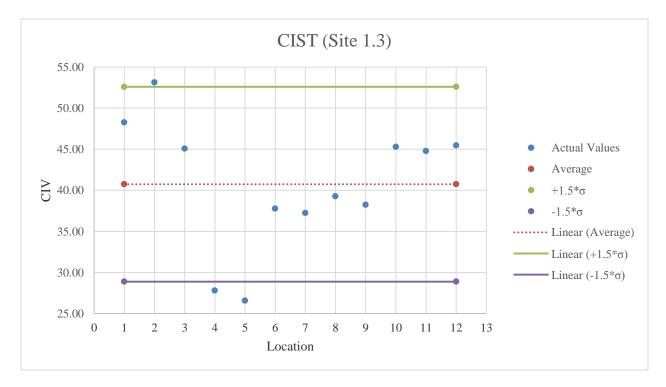
Figure E.12: CIST testing results on GAB material
