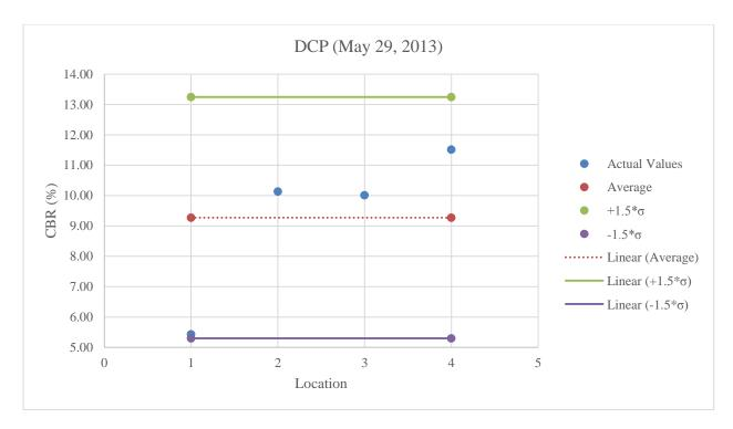
Figure B.21: DCP testing on A-2-4 below optimum moisture content
