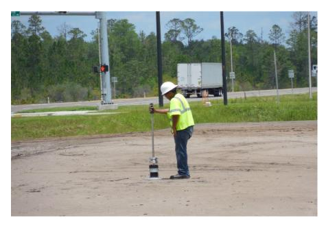
Figure 5.34: Project Site #6 SR-23 A-3 embankment - Photograph of LWD-2 test
