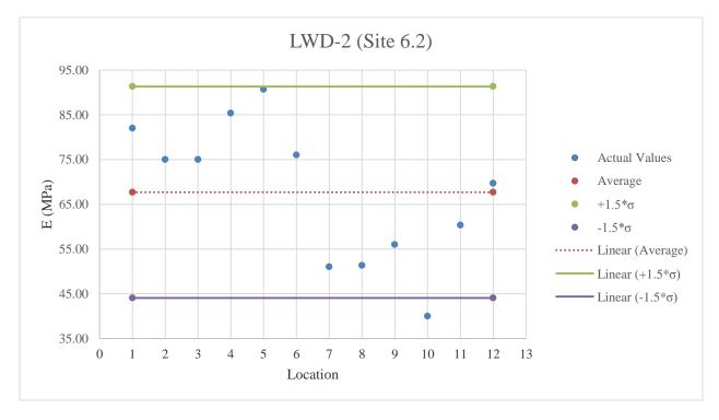
Figure E.58: LWD-2 testing results on A-3 material
