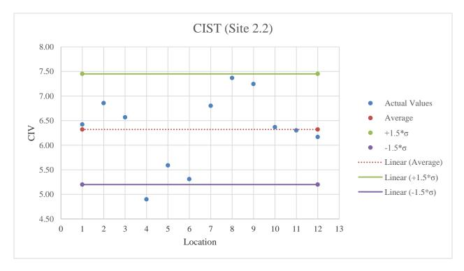
Figure E.18: CIST testing results on A-2-4 material
