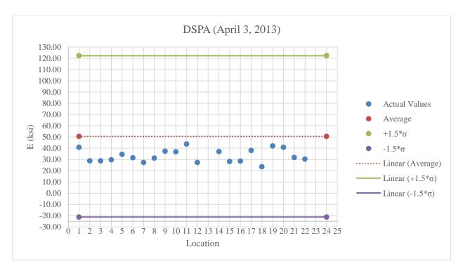
Figure B.9: DSPA testing on A-3 below optimum moisture content
