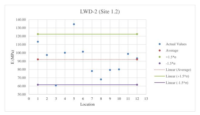
Figure E.5: LWD-2 testing results on GAB material
