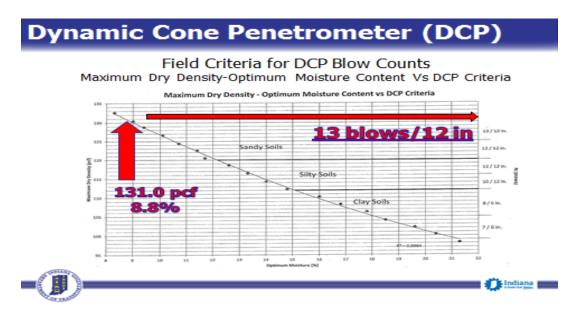
Figure H.3: INDOT Field Criteria for DCP Blow Counts
