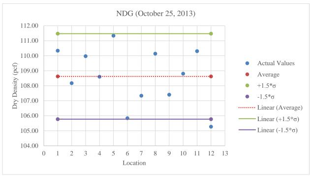
Figure C.27: Plot of NDG values for A-2-4 low fines at 6% less than optimum moisture content
