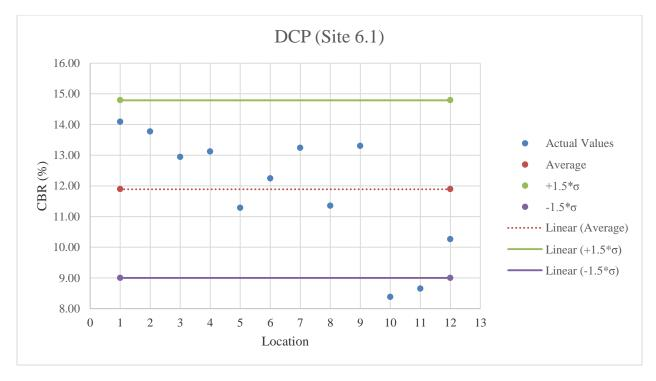
Figure E.56: DCP testing results on A-3 material
