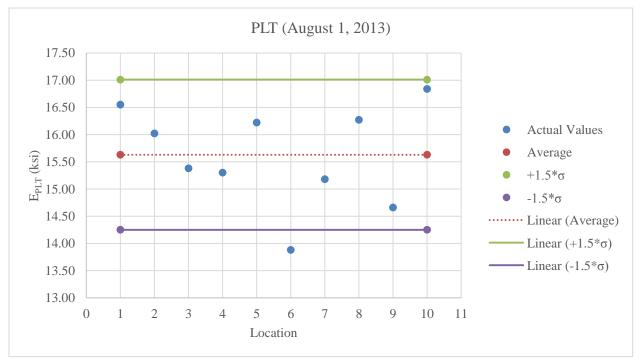
Figure C.50: Plot of PLT values for stabilized subgrade at optimum moisture content
