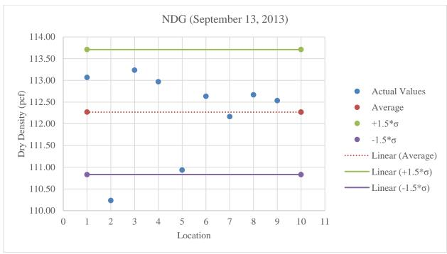
Figure C.55: Plot of NDG values for stabilized subgrade below optimum moisture content
