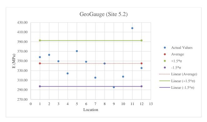
Figure E.47: GeoGauge testing results on limerock material
