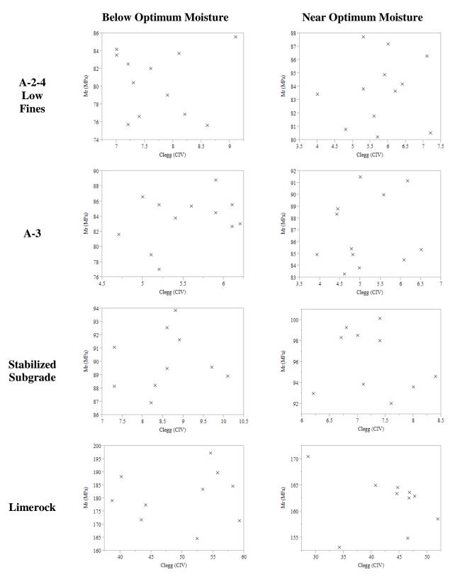
Figure F.1: Scatterplot of laboratory resilient modulus vs. CIST measurements (CIV)
