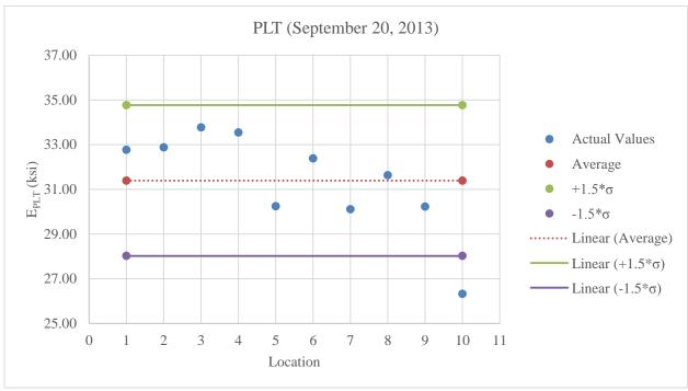
Figure C.43: Plot of PLT vales for limerock at 3% less than optimum moisture content
