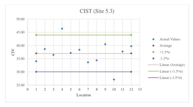
Figure E.52: CIST testing results on limerock material
