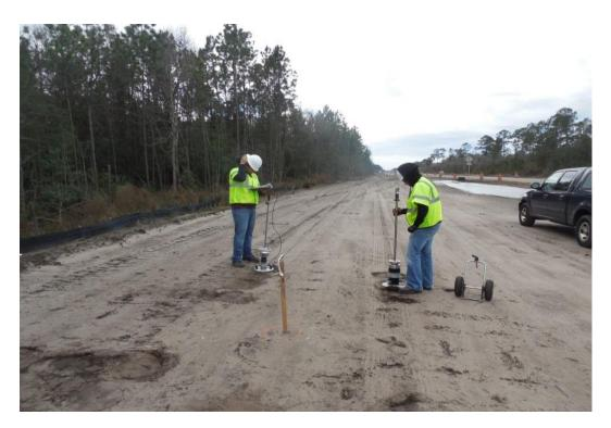
Figure 5.11: Project Site #2 US-301 - Photograph of LWDs by two different manufacturers
