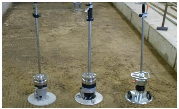
**Figure 3.5:** Photograph of LWD devices in east test pit (From left to right: LWD-P, LWD-2, and LWD-1)
