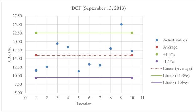
Figure C.53: Plot of DCP values for stabilized subgrade below optimum moisture content
