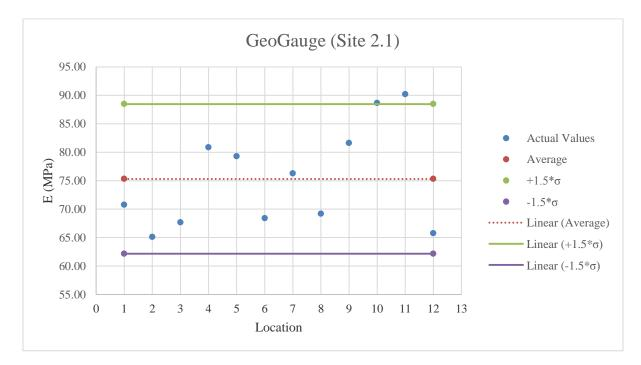
Figure E.14: GeoGauge testing results on A-2-4 material
