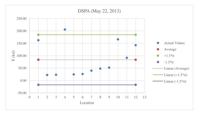
Figure B.14: DSPA testing on stabilized subgrade above optimum moisture content
