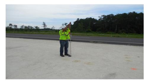
**Figure 5.31:** Project Site #5 SR-23 limerock base - Photograph of DCP (ineffective)
