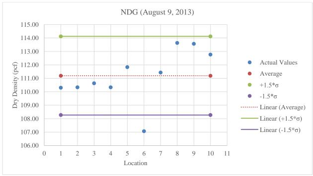
Figure C.34: Plot of NDG values for limerock at optimum moisture content
