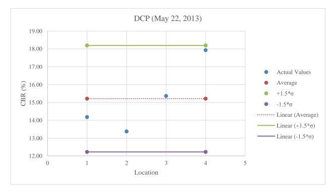
Figure B.20: DCP testing on stabilized subgrade above optimum moisture content
