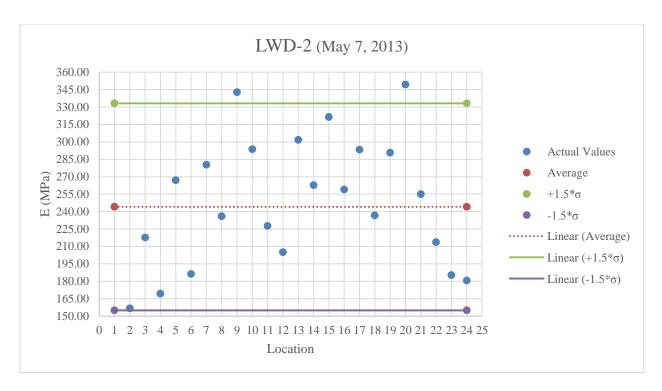
Figure B.37: LWD-2 testing on A-2-4 below optimum moisture content
