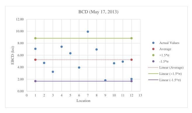
Figure B.5: BCD testing on stabilized subgrade below optimum moisture content
