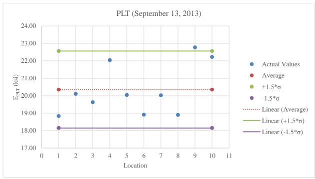
Figure C.57: Plot of PLT values for stabilized subgrade below optimum moisture content
