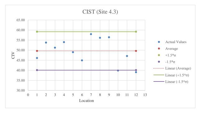
Figure E.40: CIST testing results on stabilized subgrade
