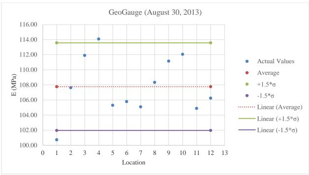
Figure C.9: Plot of GeoGauge values for A-3 at 7% less than optimum moisture content
