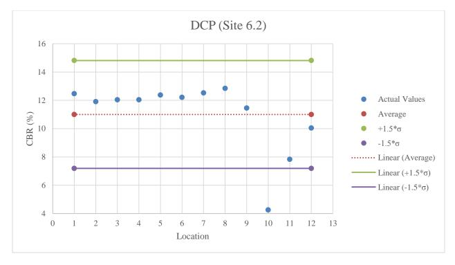
Figure E.60: DCP testing results on A-3 material
