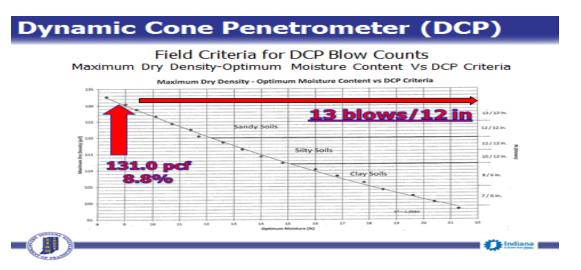
Figure 7.4: INDOT field criteria for DCP blow counts
