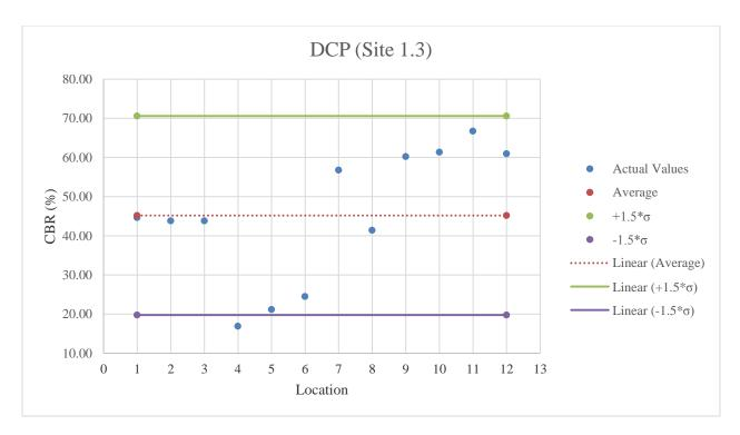
Figure E.11: DCP testing results on GAB material
