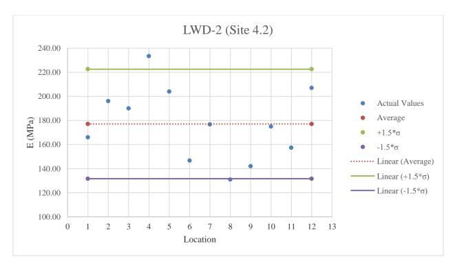
Figure E.35: LWD-2 testing results on stabilized subgrade
