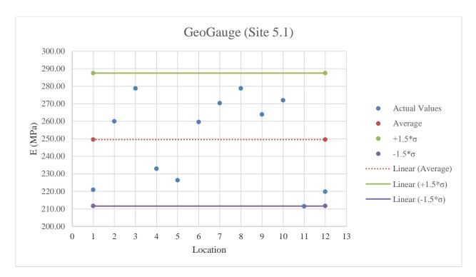
Figure E.43: GeoGauge testing results on limerock material
