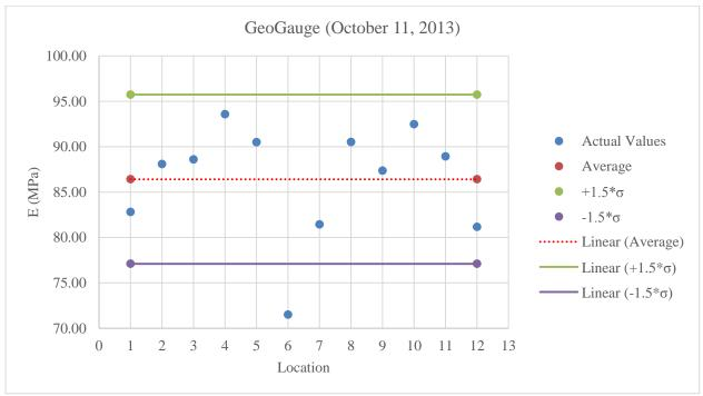
Figure C.16: Plot of GeoGauge values for A-2-4 low fines at optimum moisture content
