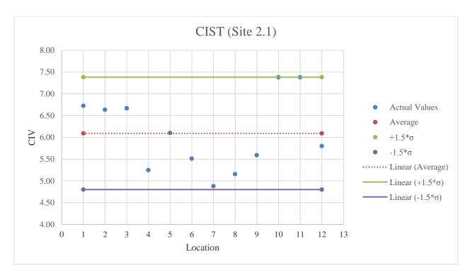
Figure E.15: CIST testing results on A-2-4 material
