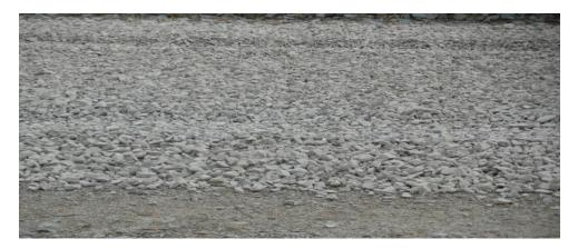
Figure 7.3: Photograph of INDOT #53 aggregate base
