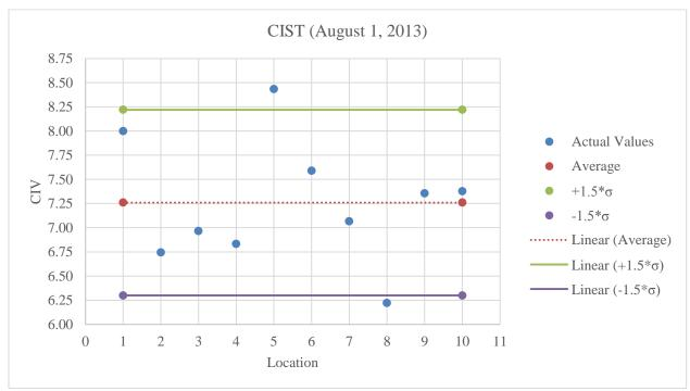
Figure C.47: Plot of CIST values for stabilized subgrade at optimum moisture content
