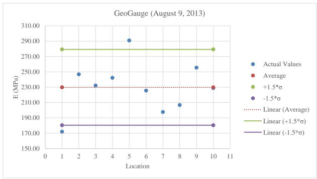
Figure C.31: Plot of GeoGauge values for limerock at optimum moisture content
