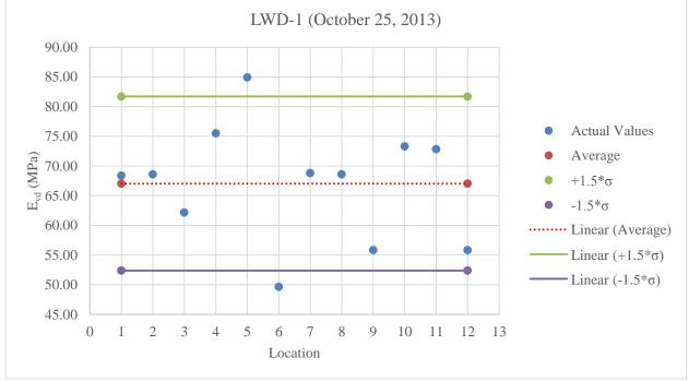
C.4 Results for Devices with A-2-4 Low Fines Material below Optimum Moisture Content
