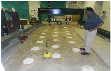
**Figure 4.5:** Photograph of west test pit A-2-4 soil (Locations for 24 PLTs: 12 per moisture percentage. NDG for in-place densities and moistures)
