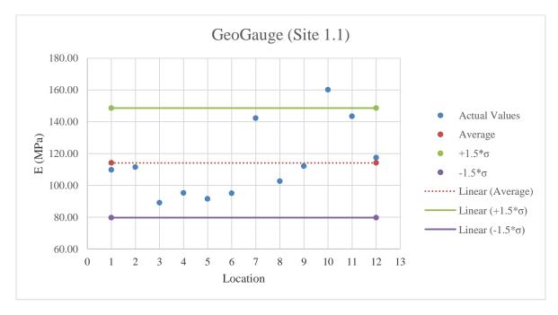
Figure E.2: GeoGauge testing results on GAB material
