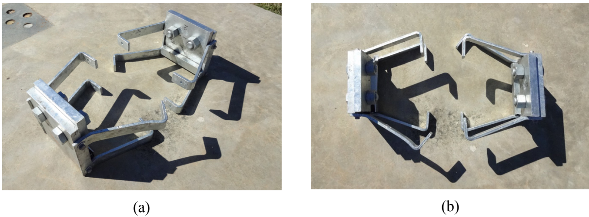
Figure 4.14 Collar components of test article after oblique (25 deg.) 19-mph impact test: (a) Isometric view collar-halves; (b) Overhead view showing U-plate deformations
