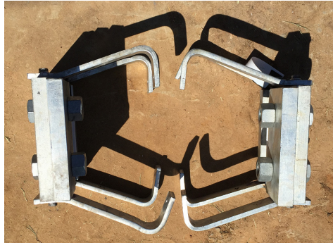
Figure 6.11 Medium-capacity collar components after oblique (25 deg.) 19-mph impact test
