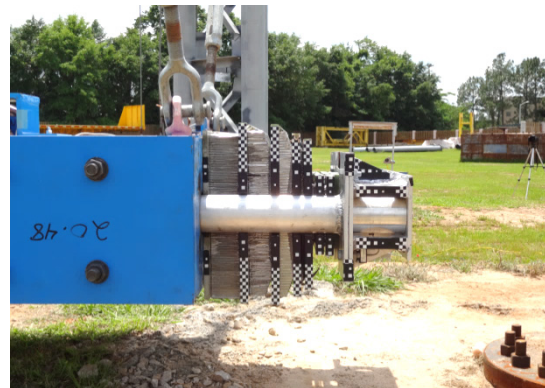
Figure 3.2 Rigid pole pendulum impact testing of surrogate vehicle: (a) Elevation view schematic; (b) Test setup prior to release of surrogate vehicle; (c) Isometric view schematic; (d) Crushable nose after impact test
