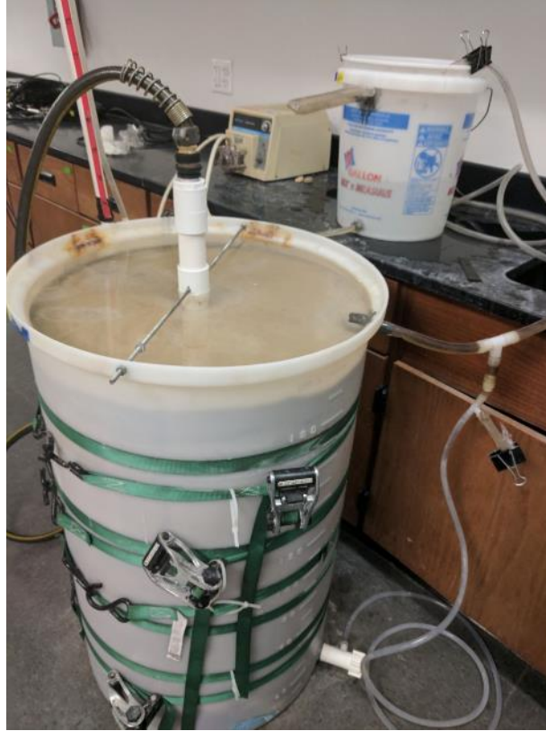
Figure 4.8 Injection test using the PVC prototype
