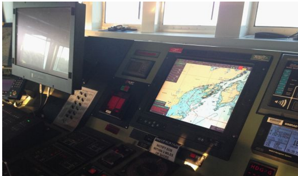
Figure 3.2 ECDIS display on-board a NOAA vessel (Source: http://www.ncep.noaa.gov )
