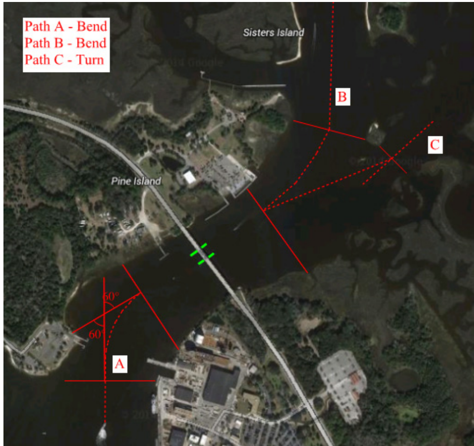
Figure 3.9 Calculation of the bridge location modification factor, R_B (Image adapted from: Google)
