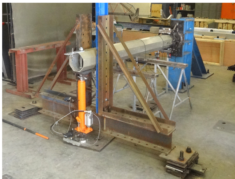
Figure 6.21 Overview of static flexural capacity test with un-epoxied stem
