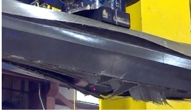
Figure 4.9 Detailed view of FRP condition after failure
