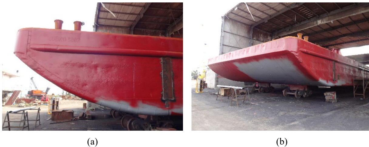
Figure 3.7 Photographs of MOBRO 1202: (a) rake geometry; (b) bow shape
