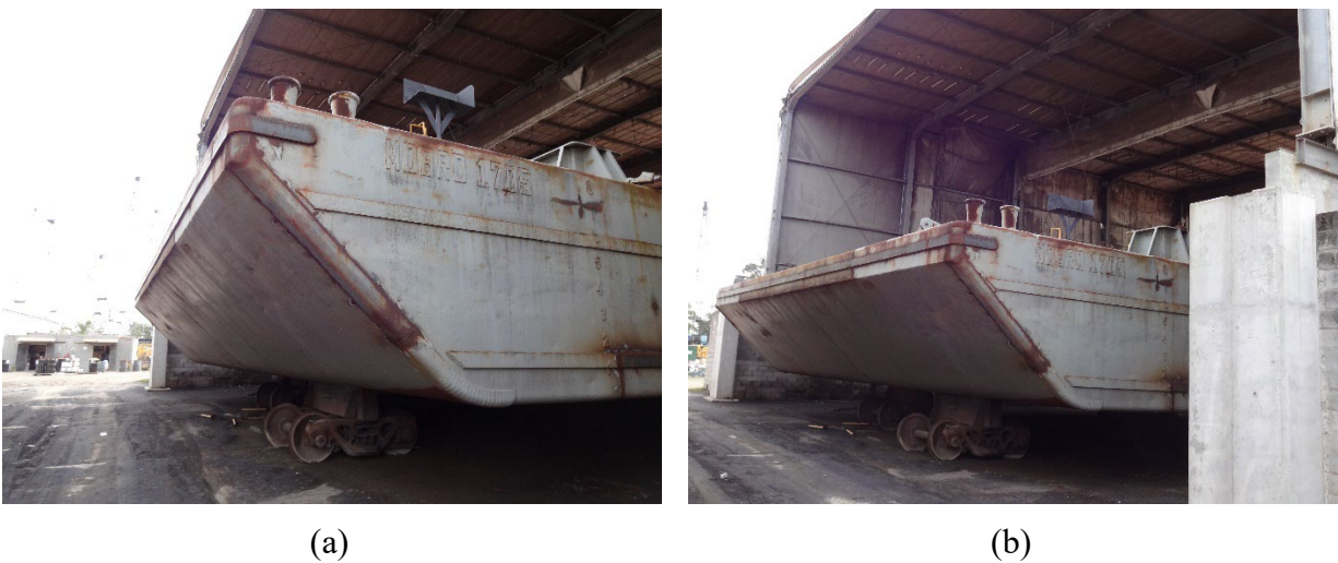
Figure 3.4 Photographs of the bow of MOBRO 1705: (a) rake geometry; (b) bow shape
