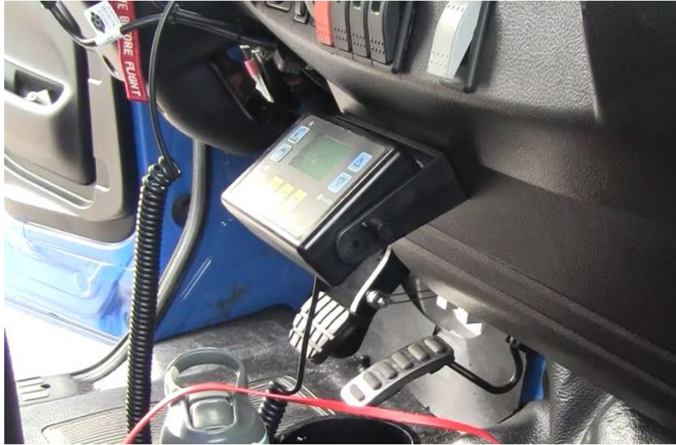
Figure 3-15. Low on the dash are the controls that lower and raise the Scorpion tail and the arrow board on the rear of the follower truck. There is also a port on the Scorpion tail that allows it to be raised and lowered with a plug-in controller (not shown).
