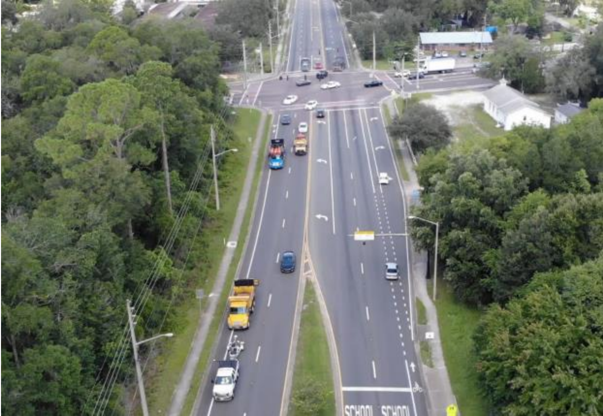
Figure 6-117. ATMA stop too close to intersection caused traffic backup for left-turning traffic at intersection
