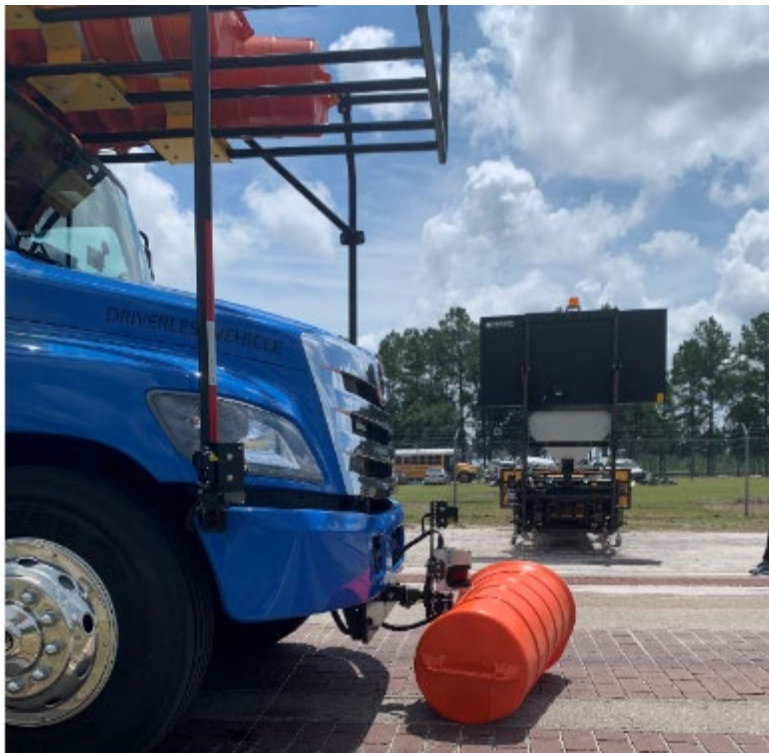
Figure 6-82. External camera view when traffic barrel was struck
