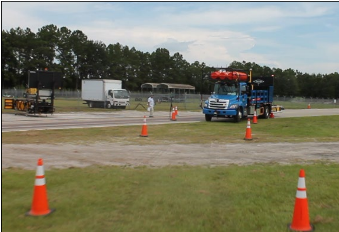
Figure 6-64. External camera view of simple curve test. The follower vehicle hits a cone.
