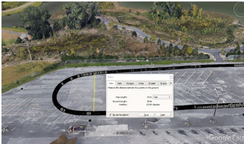
Figure 6-63. Trajectory from log file results that shows two of the successful turns with radius of 45 ft
