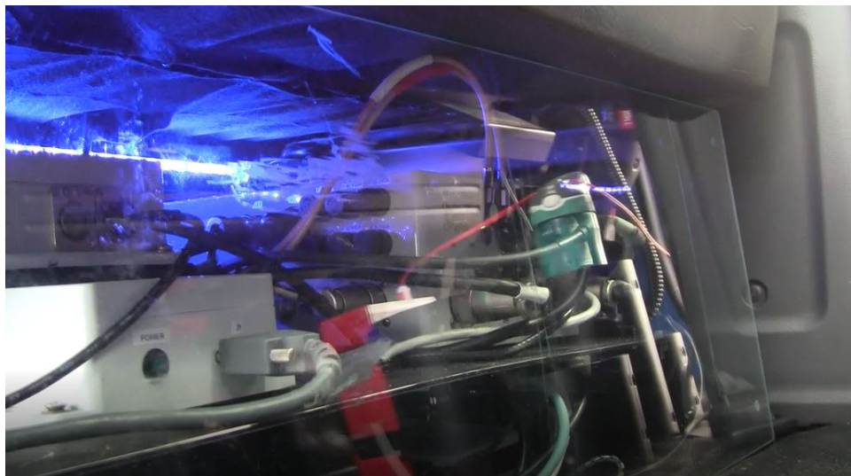
Figure 3-16. Follower truck – Internal controls: Hardware including RS232 hub, gyro, CAN bus hub, video amplifier, and wireless video link are located under the passenger seat. Communications are protected from hacking during operation with military-grade encryption.
