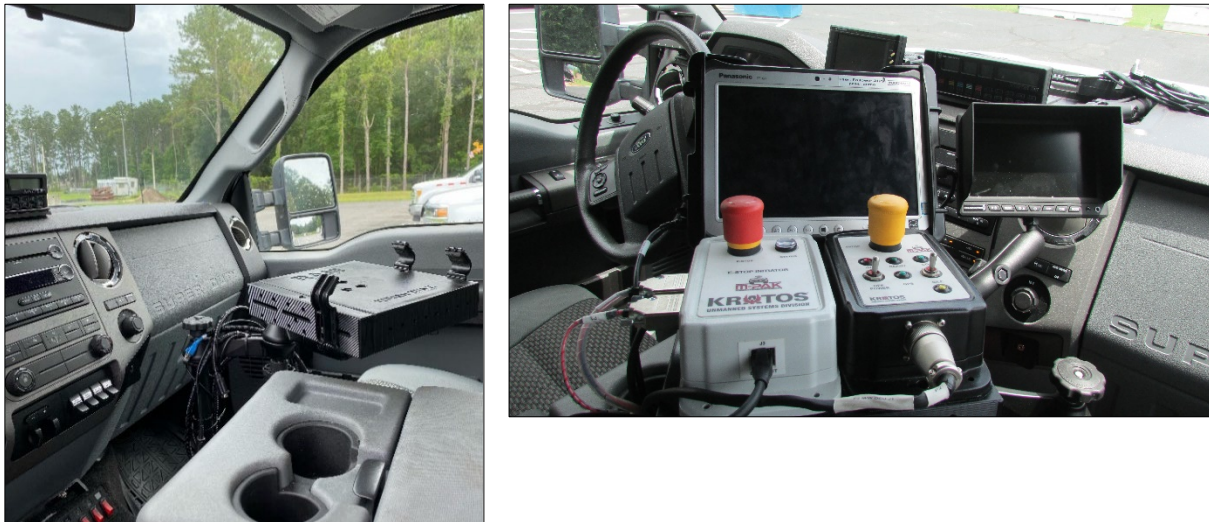
Figure 3-1. Before and after leader kit installation on FDOT F350 leader vehicle center console
