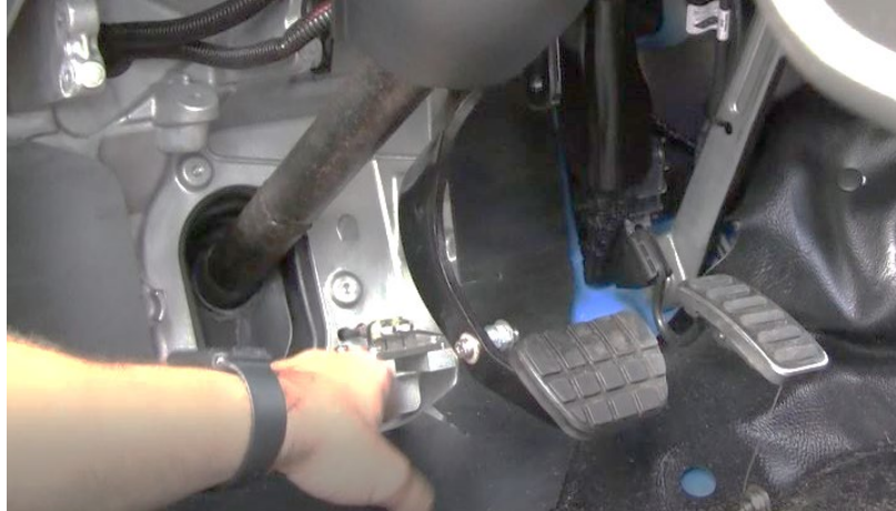
Figure 3-13. Follower truck – Internal controls: The Kratos demonstrator points to the custom cable system that operates the brake and accelerator in the follower vehicle. There are two cable linkages to the brake pedal: one provides a range of motion for normal operations and A-stops; the other one provides full braking during an E-stop.
