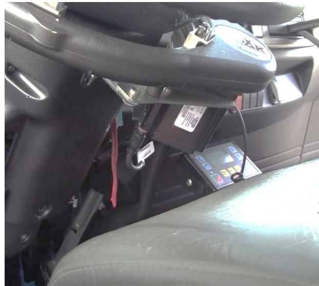
Figure 3-12. Follower truck – Internal controls (left): The steering actuator ring is linked to the steering wheel when the “steering fingers” are mounted on the two steering tabs. When the set screws are tightened, the steering fingers form a secure and tight connection between the steering actuator ring and the steering wheel. Internal controls (right): The steering actuator ring appears in the upper part of the image, with the servo housing at the right. Beneath the servo is the junction box and CAN bus that connects the steering controls to the follower vehicle’s on-board systems control unit (SCU).
