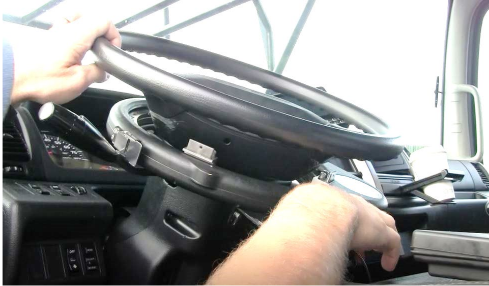
Figure 3-11. Follower truck – Internal controls: Steering in the follower truck is controlled by an actuator ring, seen in the image as a heavy black ring on the steering column below the steering wheel. The silver tab sticking up from the actuator ring is a steering tab. There are two steering tabs on the steering actuator ring.
