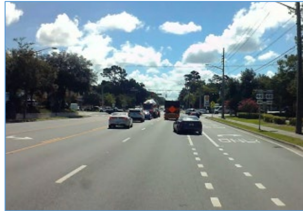
Figure 6-115. Multiple vehicle intrusions in front of ATMA that caused frequent A-stops
