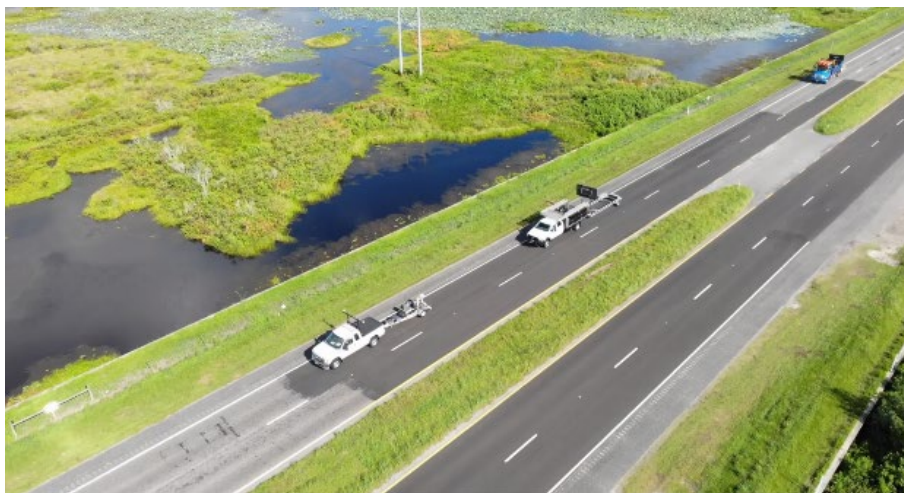
Figure 6-124. US-441 section – Leader: FDOT F350 FWD, middle TMA with attenuator; ATMA follower vehicle
