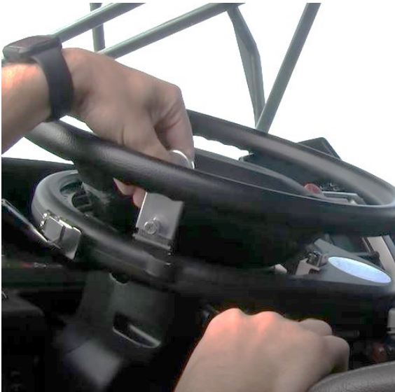
Figure 3-12. Follower truck – Internal controls (left): The steering actuator ring is linked to the steering wheel when the “steering fingers” are mounted on the two steering tabs. When the set screws are tightened, the steering fingers form a secure and tight connection between the steering actuator ring and the steering wheel. Internal controls (right): The steering actuator ring appears in the upper part of the image, with the servo housing at the right. Beneath the servo is the junction box and CAN bus that connects the steering controls to the follower vehicle’s on-board systems control unit (SCU).
