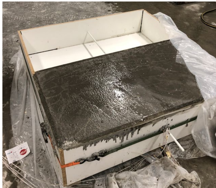
Figure 52: Concrete specimen after placement of the first half
