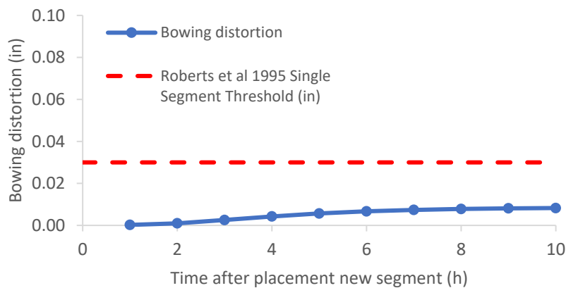
Figure B-38: Simulation 13 - Bowing distortion progression of match-cast segment from time of placement of new segment to 10 hours
