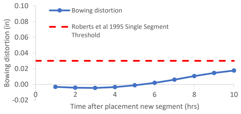
Figure B-437: Simulation 146 - Bowing distortion progression of match-cast segment from time of placement of new segment to 10 hours
