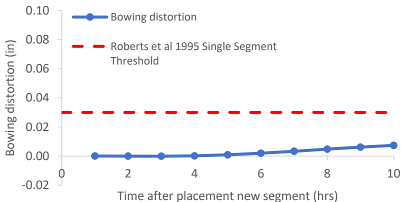
Figure B-119: Simulation 40 - Bowing distortion progression of match-cast segment from time of placement of new segment to 10 hours
