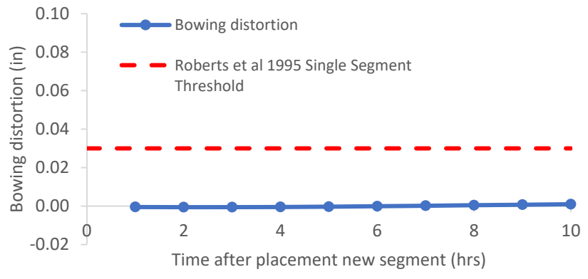
Figure B-386: Simulation 129 - Bowing distortion progression of match-cast segment from time of placement of new segment to 10 hours
