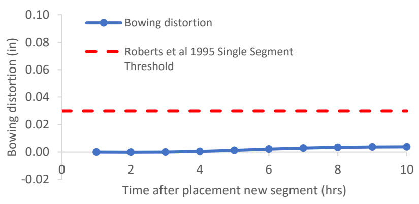
Figure B-362: Simulation 121 - Bowing distortion progression of match-cast segment from time of placement of new segment to 10 hours
