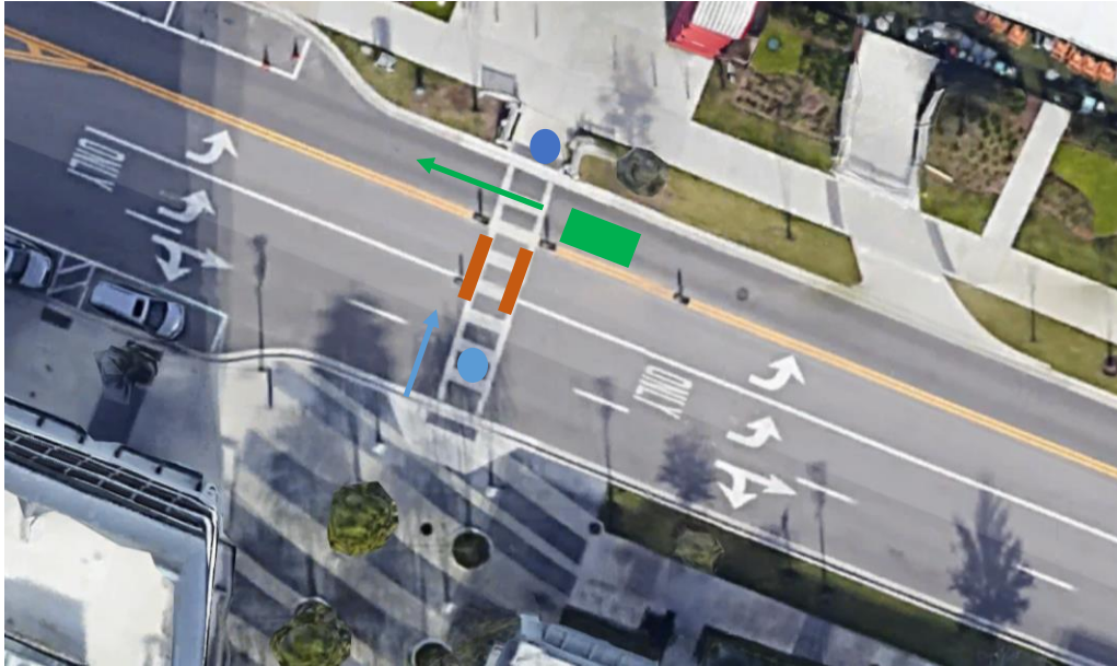
Figure 6-11. AVS did not stop for a slowing pedestrian on the sidewalk and a pedestrian on the crosswalk for the opposing direction.
