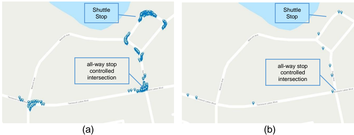
Figure 6-41. Uncomfortable acceleration/deceleration positions near the all-way stop controlled intersection (Zone 3)
