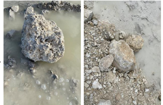
As shown here in a sample taken in the vicinity of the load test, Miami limestone has very high variability as well as a wide range of porosities. From left to right, high variability with high porosity (left) to low porosity (right).
