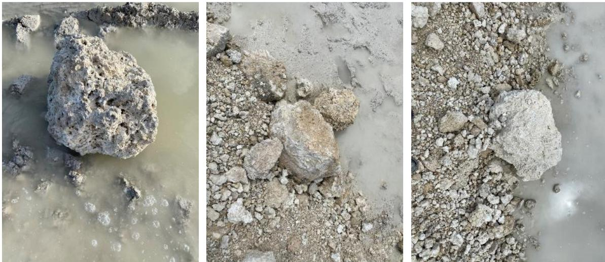
**Figure 5-20 Pictures of rock pieces from tested pit during excavation: high variability with low (middle) and high (left) porosity of Miami limestone**
