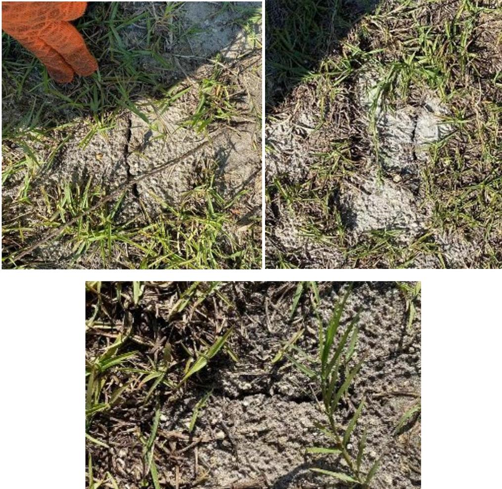
**Figure 7-19 Tension cracks after load test**
