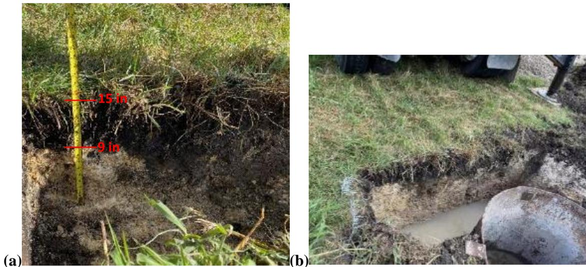
**Figure 6-13 Miami limestone layer: (a) excavated down to 15 in; (b) excavated down to 3 ft.**
