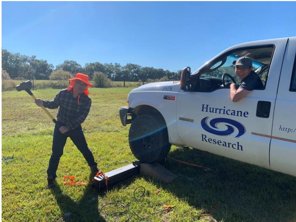
**Figure 4-27 The shear-beam pressed by the vehicle wheel**
