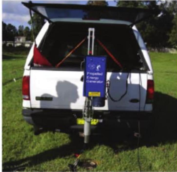
**Figure 4-7 Propelled energy generator (PEG) source**
