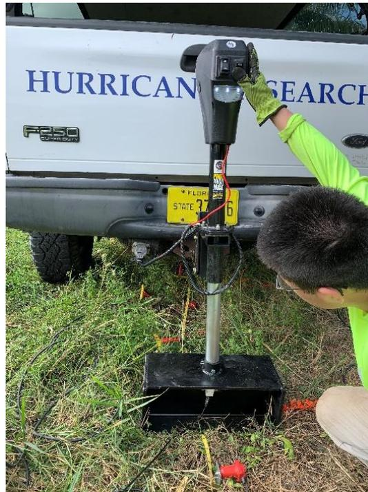
**Figure 4-14 The shear-beam pressed by the hydraulic jack**
