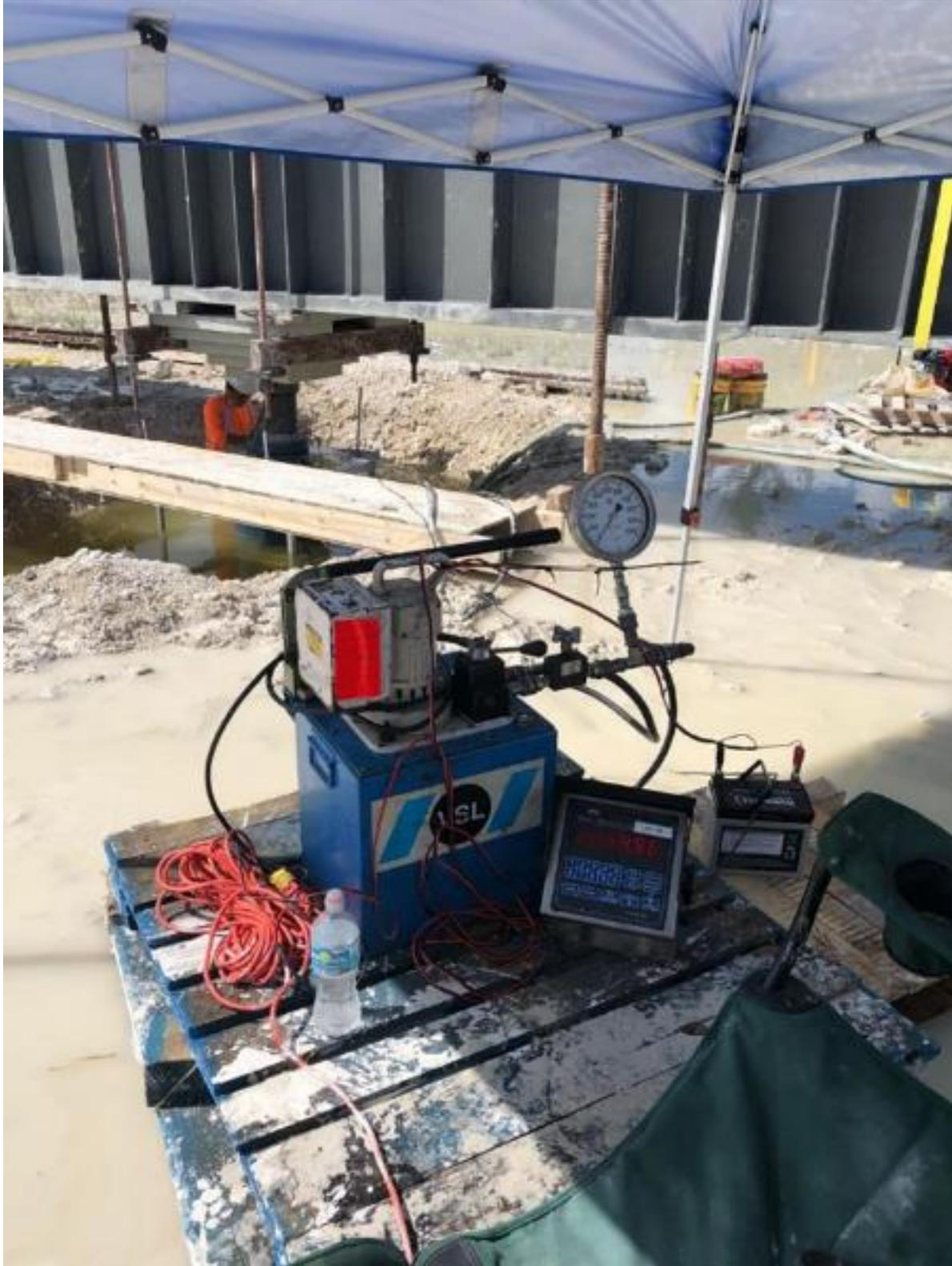
**Figure 5-25 Hydraulic jack and load cell setup**
