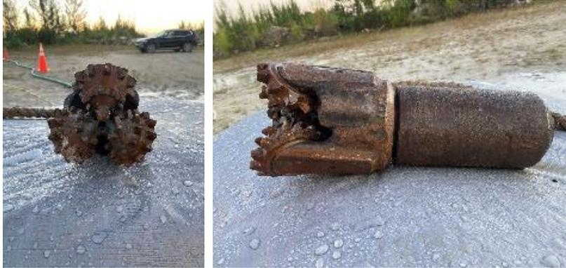
**Figure 5-8 Tricone drill bit**
