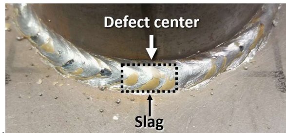
Figure 0-4 – Optical image of the steel pipe-to-plate weld joint with slag over the defect center corresponding to the IR image in Figure 35(c).
