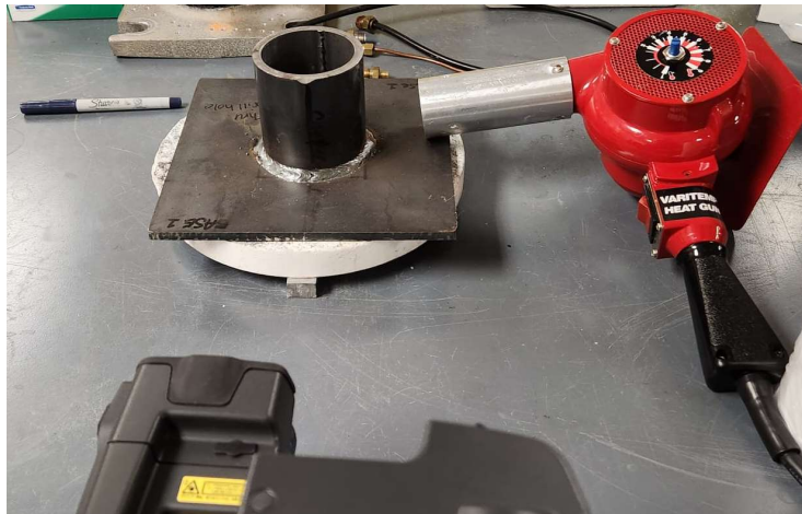
Figure 0-20 – Photography of the trial assembly, showing sample, camera, and heat gun positioning.
