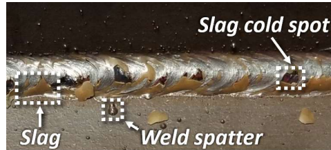
Figure 0-6 – Optical image of the baseline sample steel plate-to-plate weld joint with labels showing examples of slag, cold spots (regions where slag spontaneously removed from the weld during cool-down), and weld spatter.
