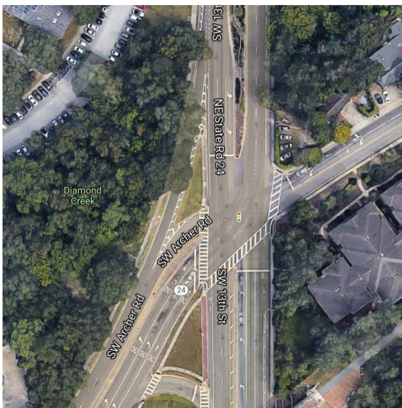
Figure A-6. Layout and lane configuration for the intersection at Archer Rd and 13 th St
