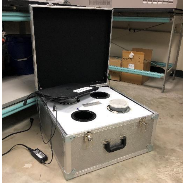
Figure 4-8 Semi-adiabatic temperature test-Calmetrix F-Cal concrete
