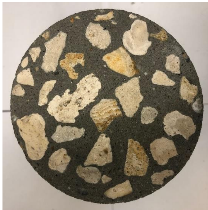
Figure 2-8 Cross-section of standard concrete
