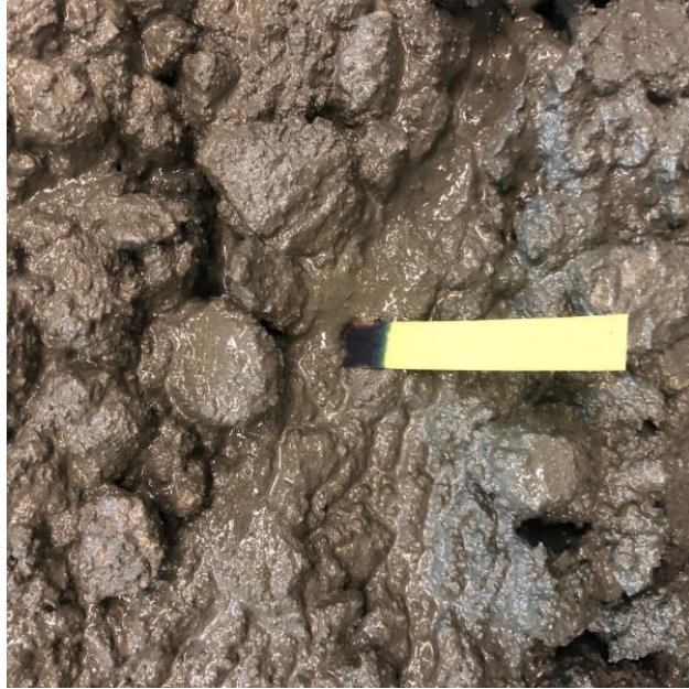
Figure 4-9 Universal indicator paper test on concrete
