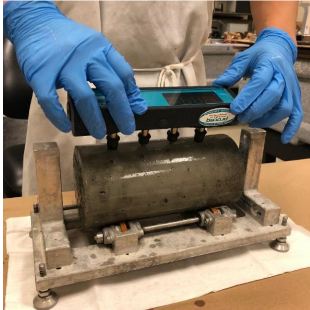
Figure 4-19 Surface resistivity test (Wenner probe array)
