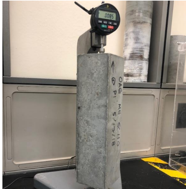
Figure 4-16 The drying shrinkage test apparatus
