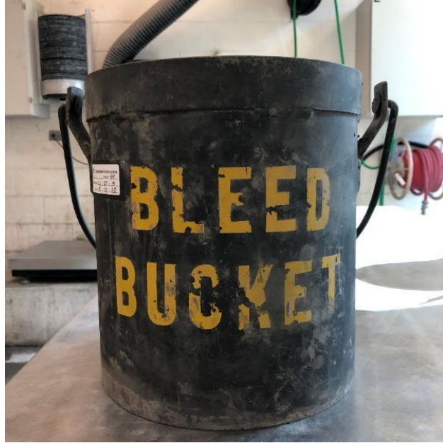
Figure 4-7 Bucket for bleeding water of concrete test
