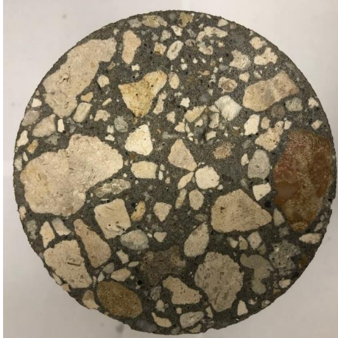
Figure 2-9 Cross-section of concrete with OAG
