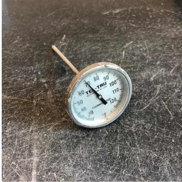
Figure 4-6 Temperature measuring device of fresh concrete test
