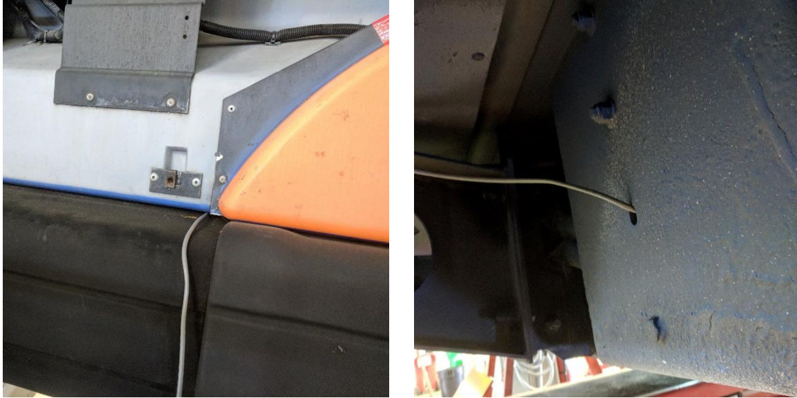
Figure 2-7. (Left) Sensor wire fed through the front bumper of the bus to the front undercarriage. (Right) Port under the front undercarriage where the sensor wires are fed to the battery compartment.
