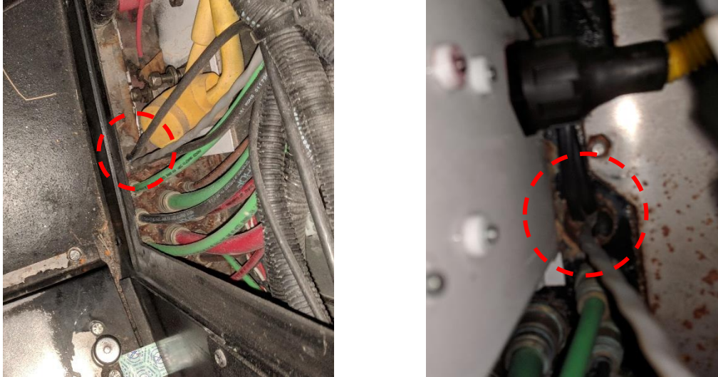
Figure 2-6. (Left) Side panel next to the driver's feet that contains the port to the battery compartment (outlined). (Right) View from the battery compartment of the same port (outlined).
