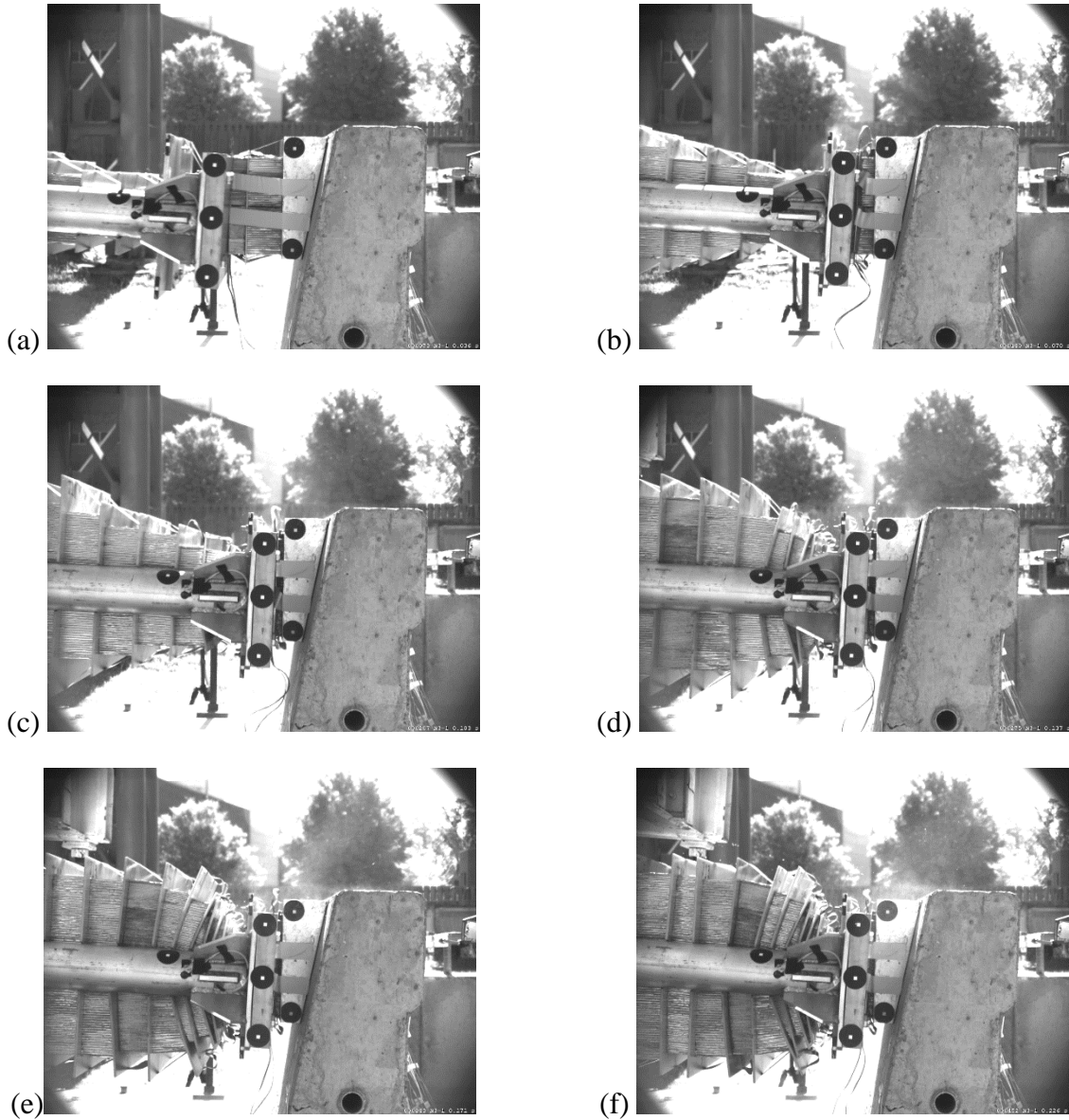
Figure 9-4 High-speed video frames from HSC-1 (R/C EOR test 1) showing crush deformation of aluminum honeycomb: (a) At initial impact; (b) – (c) Intermediate frames; (f) At peak impact force
