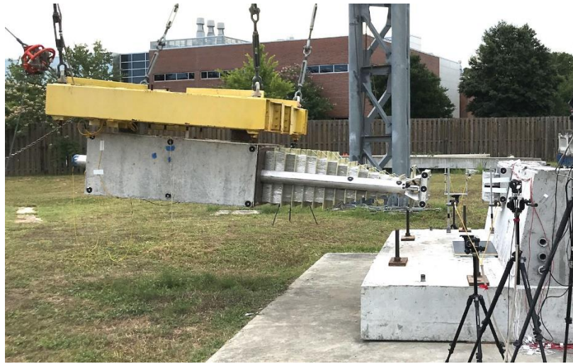
Figure 3-10. FDOT SUT 10000S impactor prior of TL-4 pendulum impact test
