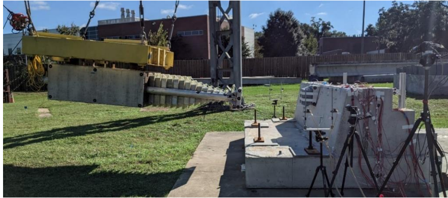
Figure 7-16 Pendulum impactor and impact test specimen prepared and ready for testing
