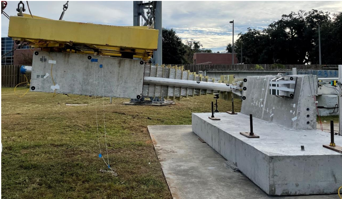
Figure 9-42 GFRP EOR test 2 specimen prepared and ready for pendulum impact testing (with instrumentation in place)
