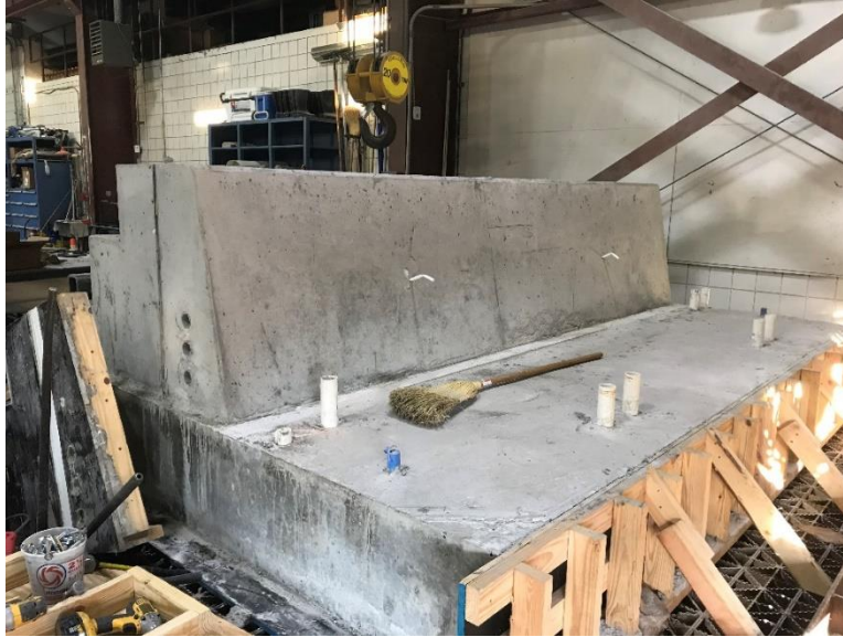
Figure 7-6 Formed R/C test specimen 1
