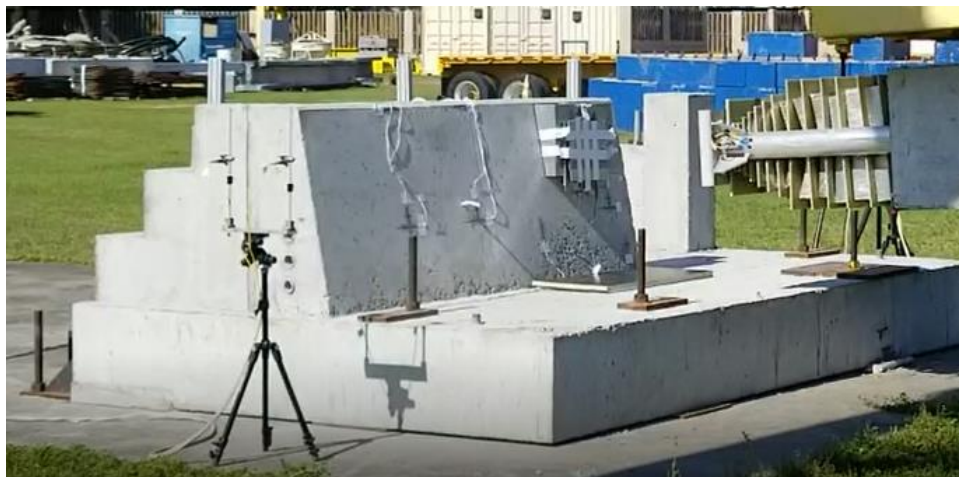
Figure 9-6 R/C EOR test 1 specimen after completion of impact test
