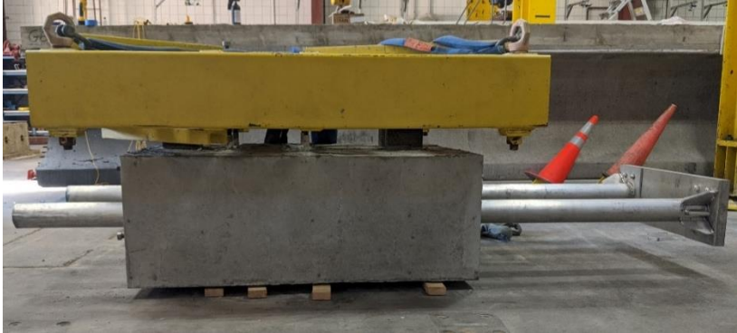
Figure 3-9. FDOT SUT 10000S impactor (without aluminum honeycomb cartridges installed)
