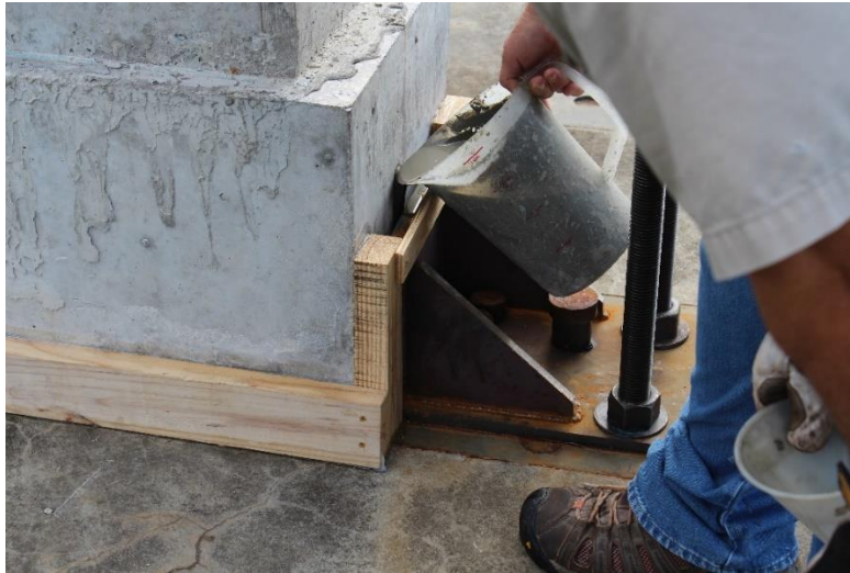
Figure 7-14 Placing grout between test specimen and reaction element (steel slide stopper) as a secondary reaction system to prevent specimen from sliding during impact testing
