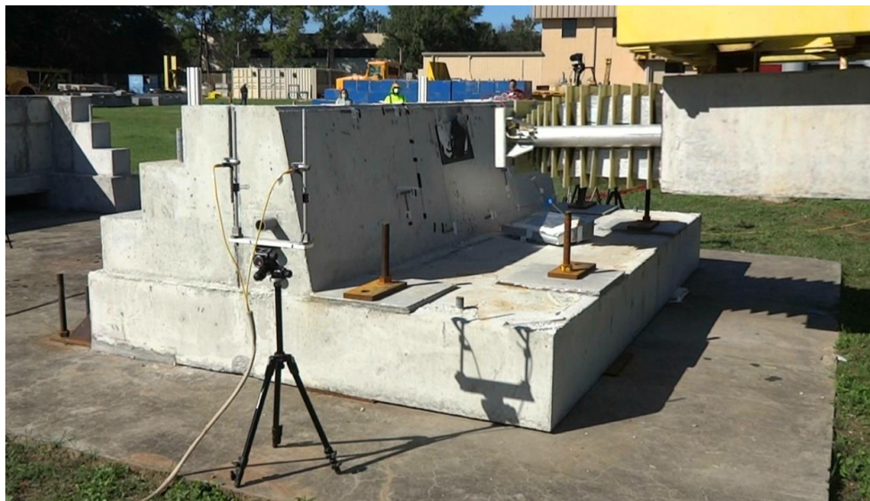
Figure 8-4 R/C COR 1 test specimen after completion of impact test
