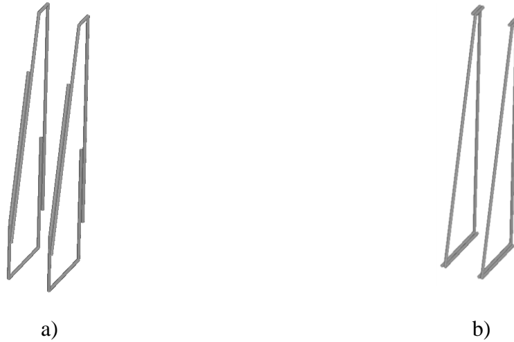
Figure 6-6. Rebar models for COR test specimens: a) Steel transverse bars; b) GFRP transverse bars
