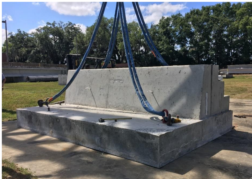
Figure 7-9 Impact test specimen in position on pendulum foundation
