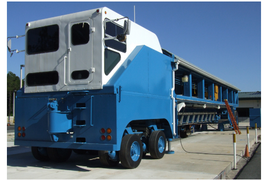
The heavy vehicle simulator allows accelerated testing of pavement samples by applying the equivalent of 29,000 vehicle passes in a 24-hour period.
