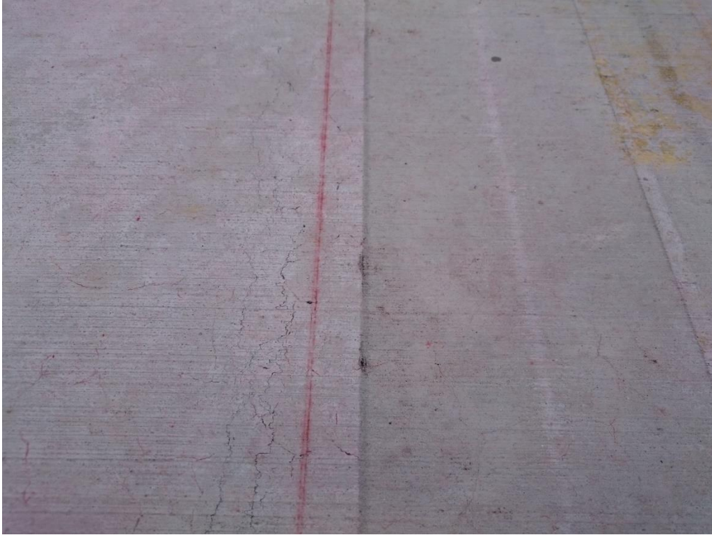
Figure 5-25. Surface of standard-mix slab after HVS loading.
