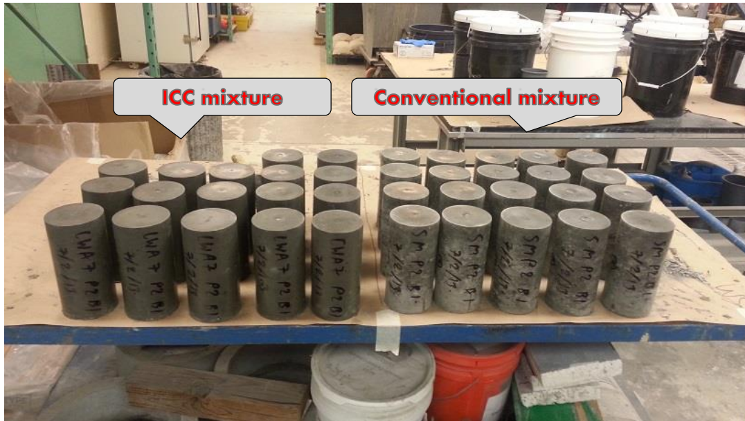
Figure 4-10. Concrete cylinder specimens just after removing from molds.
