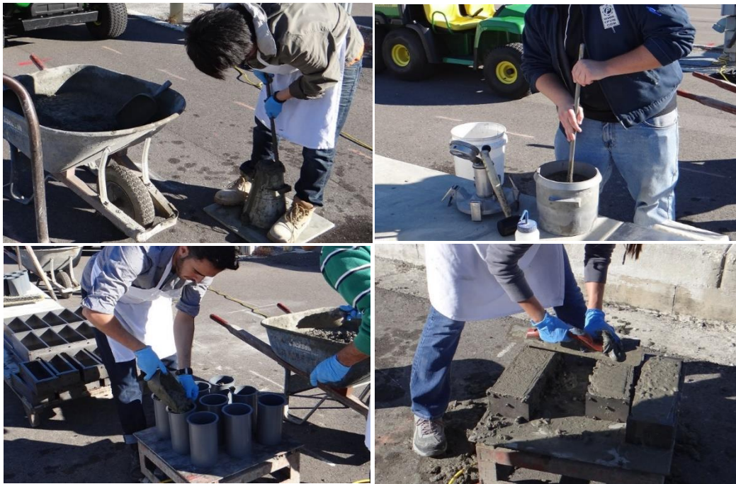
Figure 5-2. Fresh concrete properties testing and samples making.
