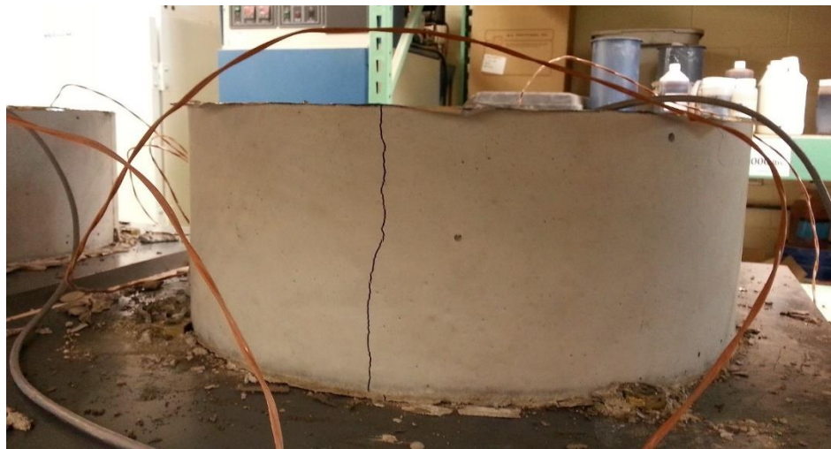
Figure 4-21. Crack on a concrete ring specimen.
