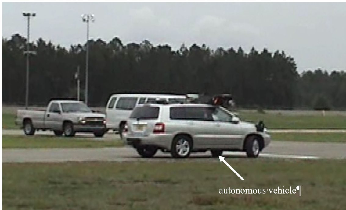
Figure 3-6: Autonomous vehicle at four-way-stop intersection.
