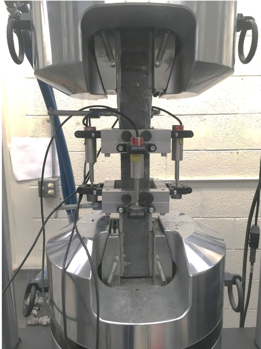
Figure 48: Image of tensile testing setup including c-clamps
