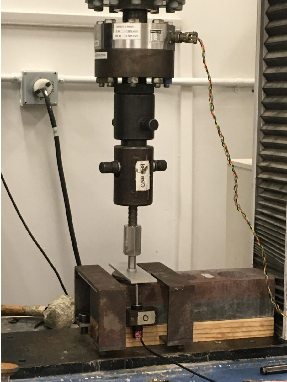
Figure 84: Pull-off testing setup
