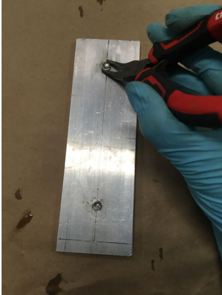
Figure 105: Gauge points with epoxy are placed in template notches
