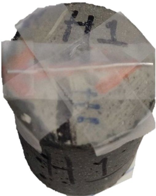
Figure 224: The aluminum strip held by tapes placed on the double-headed arrow signifying the direction of the magnetic scan
