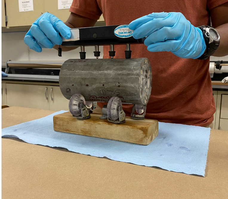
Figure 152: Surface resistivity test set up
