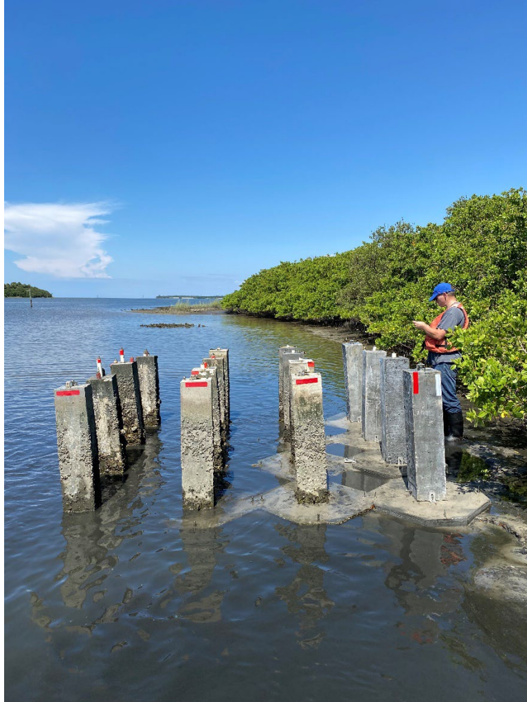
Figure 201: UHPC samples placed at Seahorse Key
