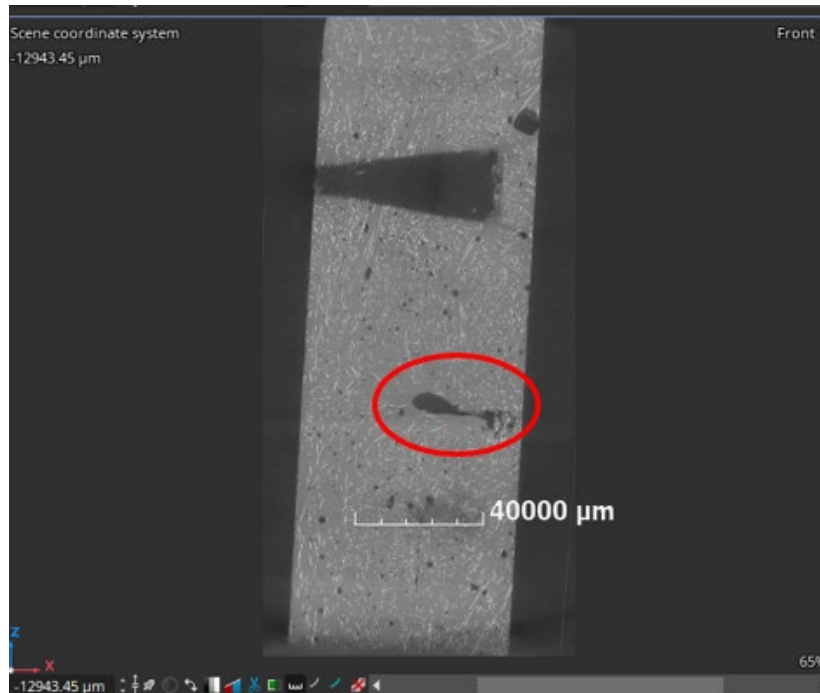
Figure 99: 2-D view (front) of large air void at location where concrete was rodded from Figure 96
