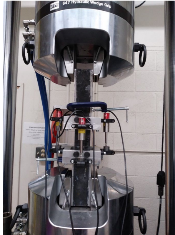
Figure 15: Tensile test before gripping with the C-clamps attached
