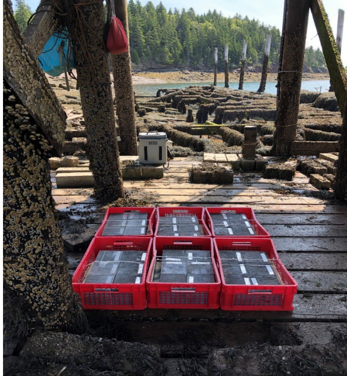
Figure 202: UHPC samples placed at Treat Island
