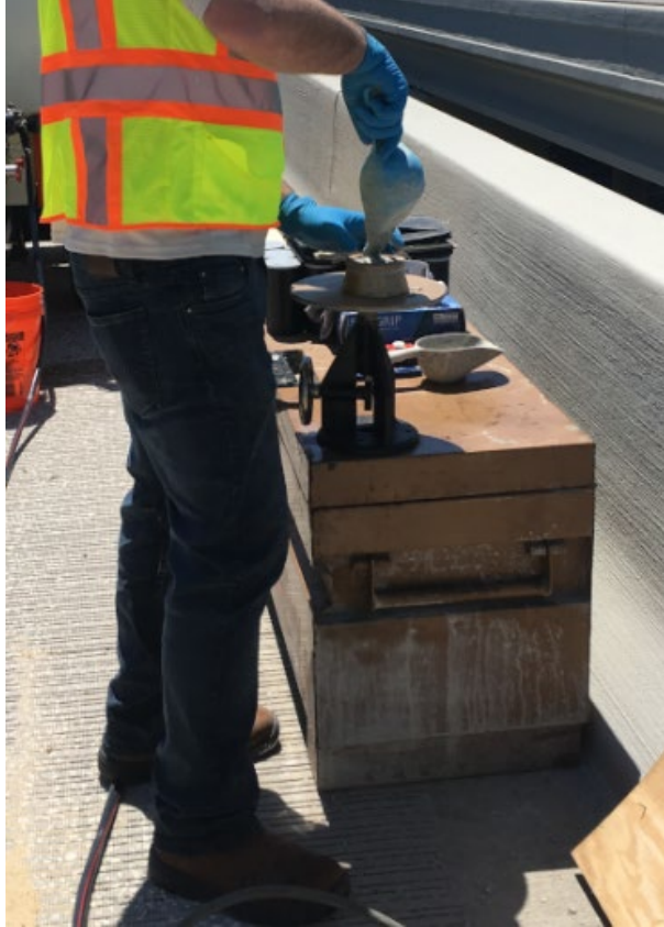
Figure 2: Filling the mold with UHPC
