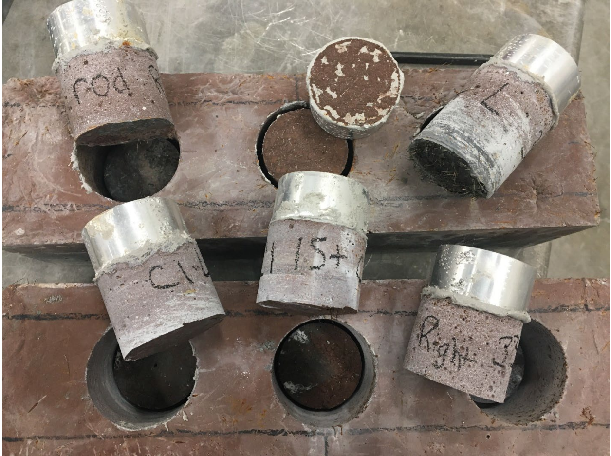
Figure 86: Concrete cores after testing
