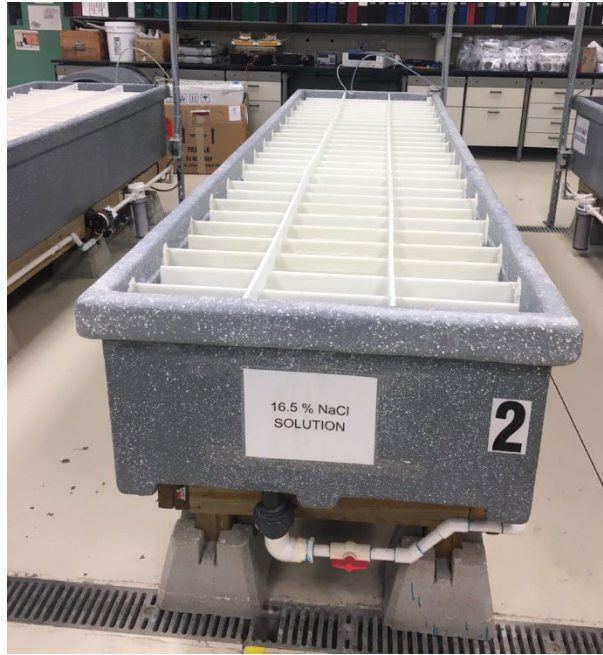
Figure 155: Sodium chloride tank at FDOT
