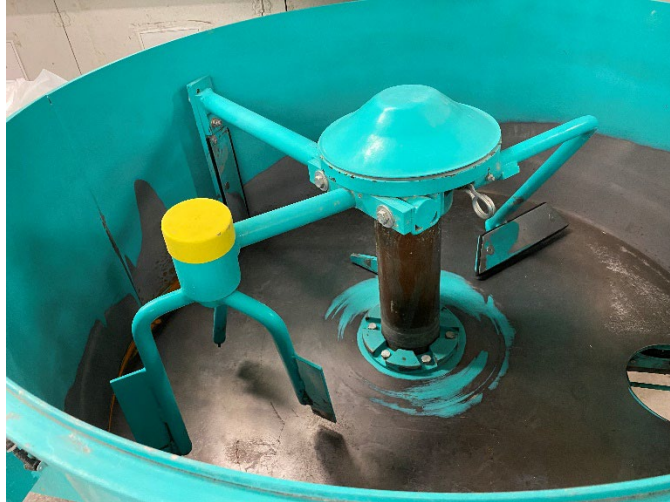
Figure 146: IMER Mortarman mixer for UHPC batches up to 4.0 ft 3
