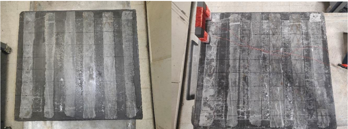
Figure 218: (a) The UHPC slab that is used for the orientation test, the stripes show the approximate preferred orientation of the steel fiber alignment. (b) shows the specimen with the magnet sensor on it taking incremental measurements to measure the orientation. The black marker lines are visible and were used to measure the inductance in the perpendicular direction to the striped direction
