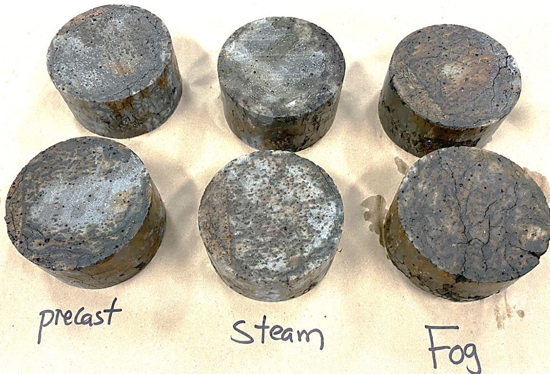
Figure 163: Mix 15 ksi samples with 1.5% of steel fibers at the end of 10 days of RCM testing
