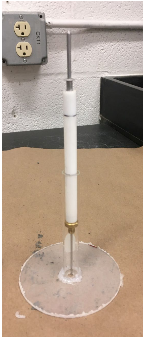
Figure 83: Vicat needle used to test concrete and elephant skin stiffness
