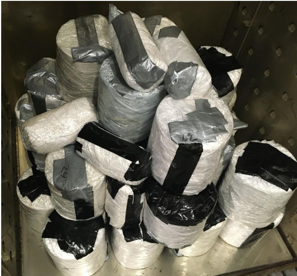
Figure 73: Specimens wrapped for steam treatment
