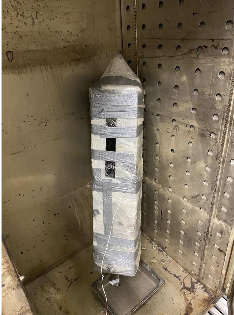
Figure 197: Column specimen during steam curing
