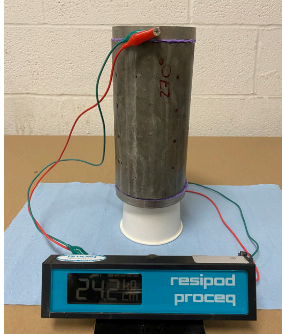
Figure 153: Bulk resistivity test set up
