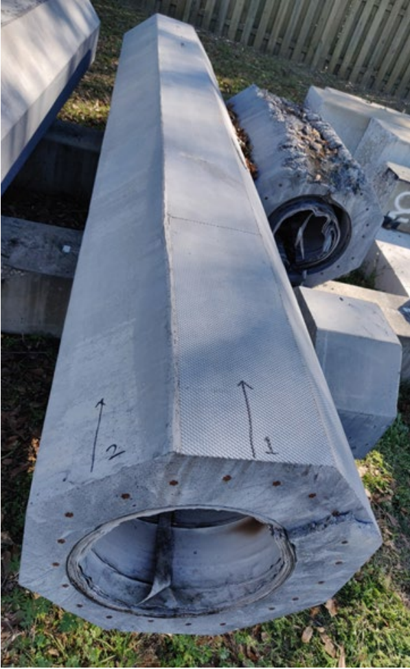
Figure 231: Longitudinal view of the octagonal pile scanned
