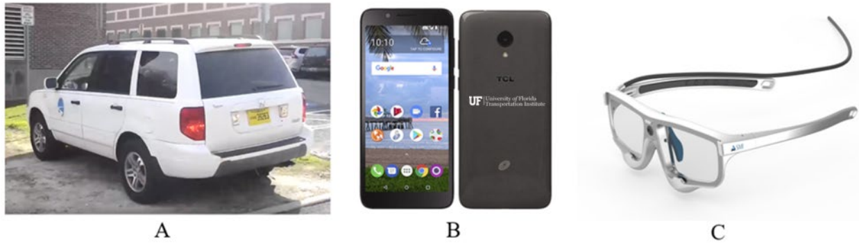
Figure 5 Apparatus and equipment used in the study: A) UFTI instrumented vehicle (2004 Honda Pilot), B) UFTI's smartphone - Alcatel TCL android phone (Model: A502DL), and C) SMI ETG 2 head-mounted glasses.
