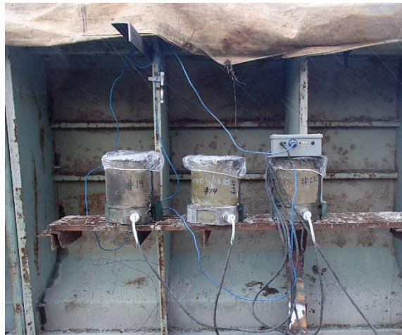
Figure 3-24 Match-cure system used for mockup cylinder samples
