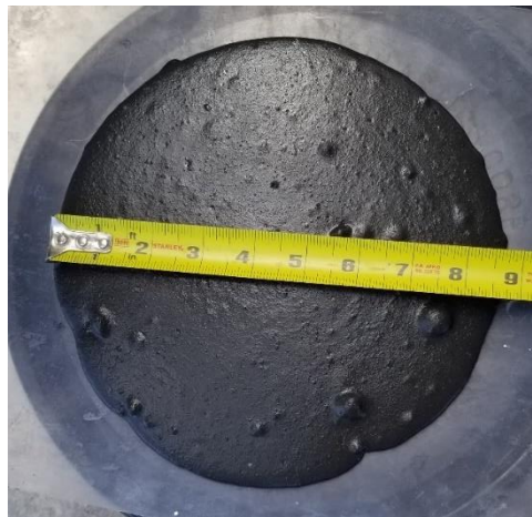
Figure 2-6 Spread test on UHPC without fibers (Photo credit: Torres)
