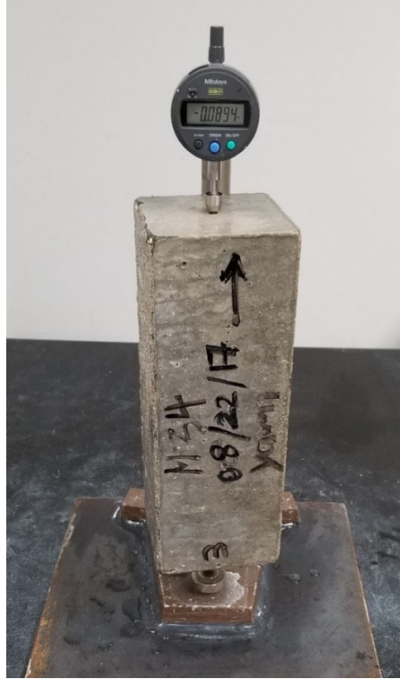
Figure 8-7: Concrete prism in length comparator
