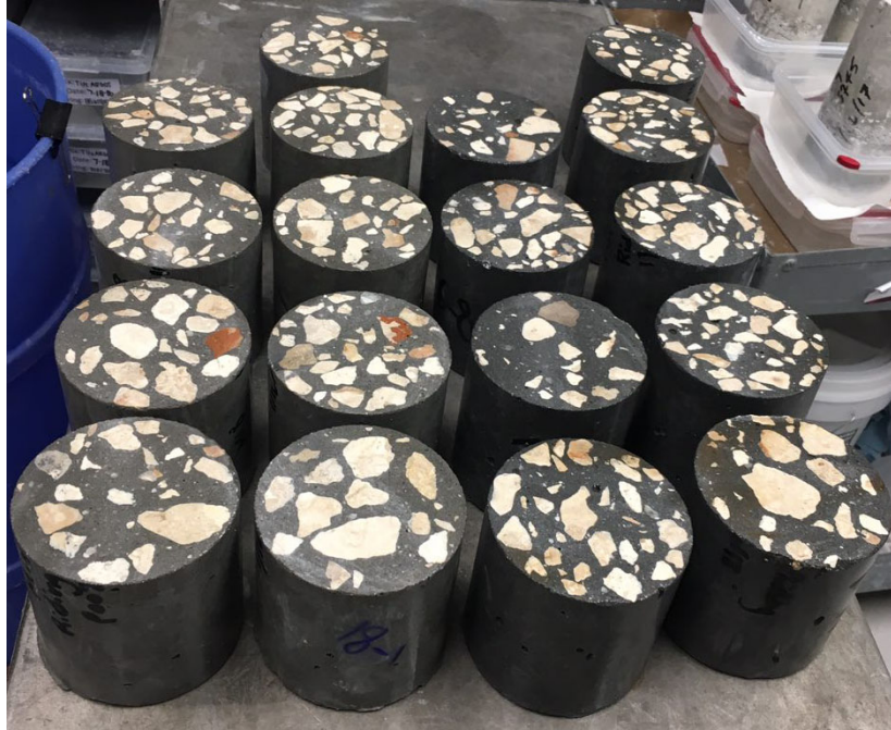
Figure 6-2: Bulk diffusion samples during storage at 23 \pm 2^\circ\text{C} and 50% RH
