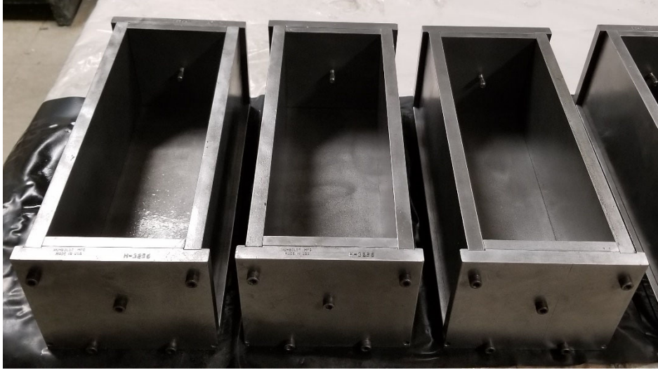
Figure 8-1: Prism molds assembled and ready for use
