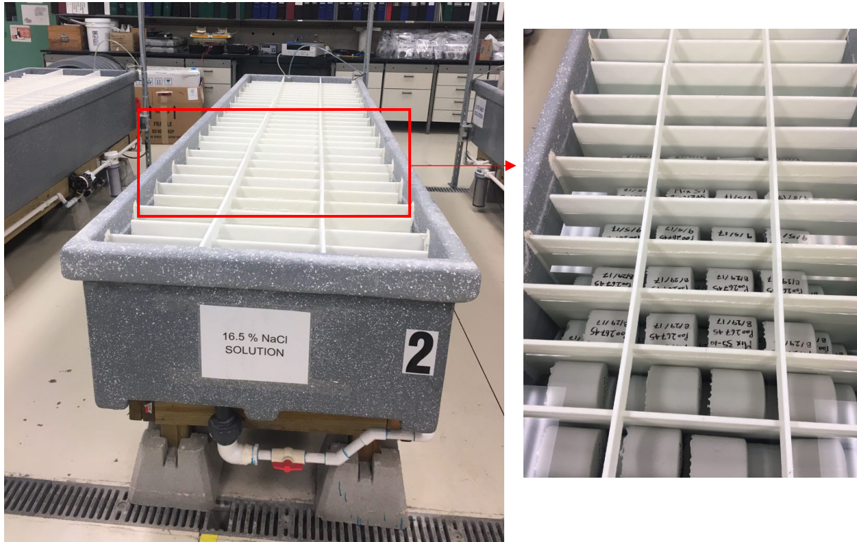
Figure 6-3: Tank containing 16.5% NaCl solution and bulk diffusion samples
