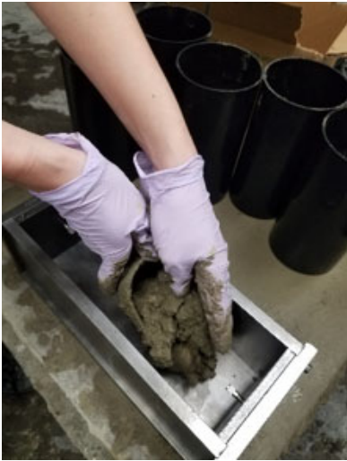
Figure 8-2: Concrete placement in mold
