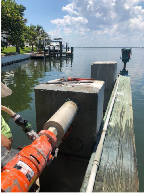
Figure 7-3: Getting core from the piles
