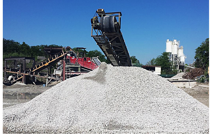
Crushed concrete at a recycling facility in Gainesville.
