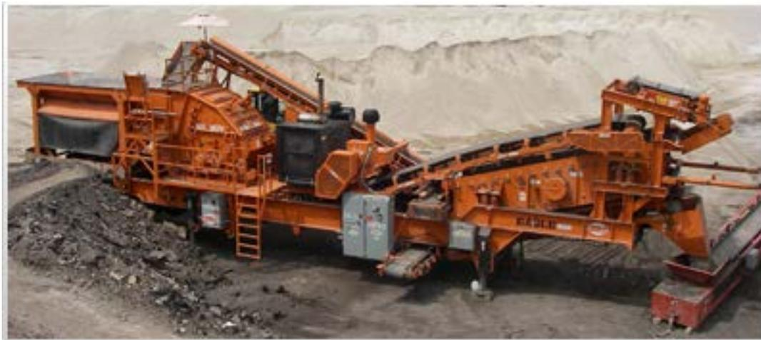
**Figure 18:** Crush-It portable concrete crusher
