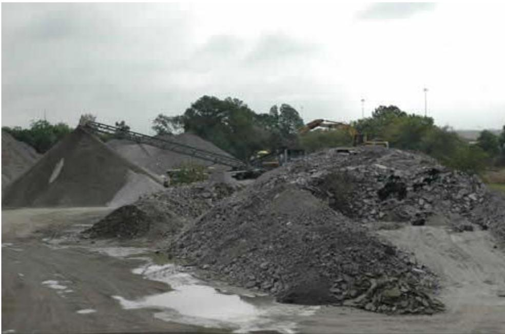
**Figure 19:** Recycled aggregate stockpile at Transcor Recycling<sup>2</sup>
