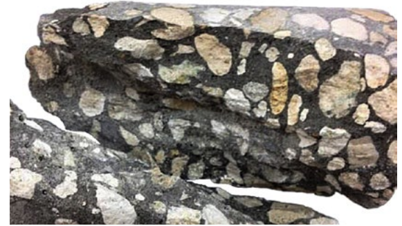
This concrete sample shows how aggregate is distributed in concrete. The whitish areas are Brooksville limestone.
