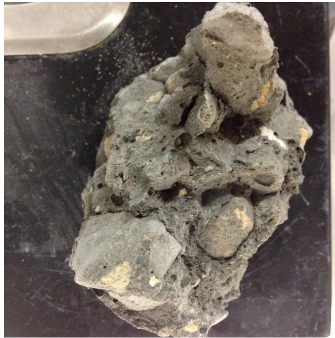
Figure 7.8 Class II mixture with Perry aggregate, 3-day failure cone
