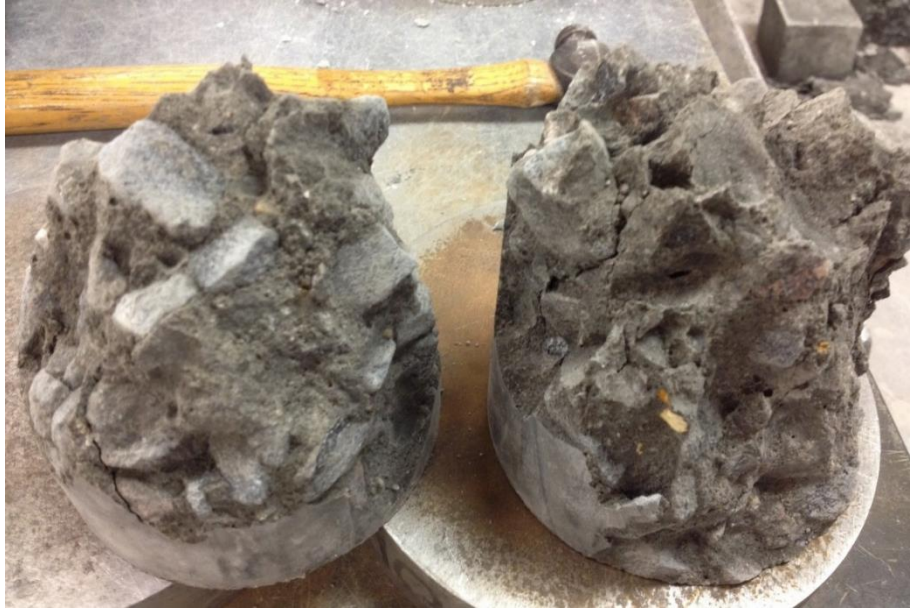
Figure 7.10 Class II mixture with granite aggregate, 3-day failure cones
