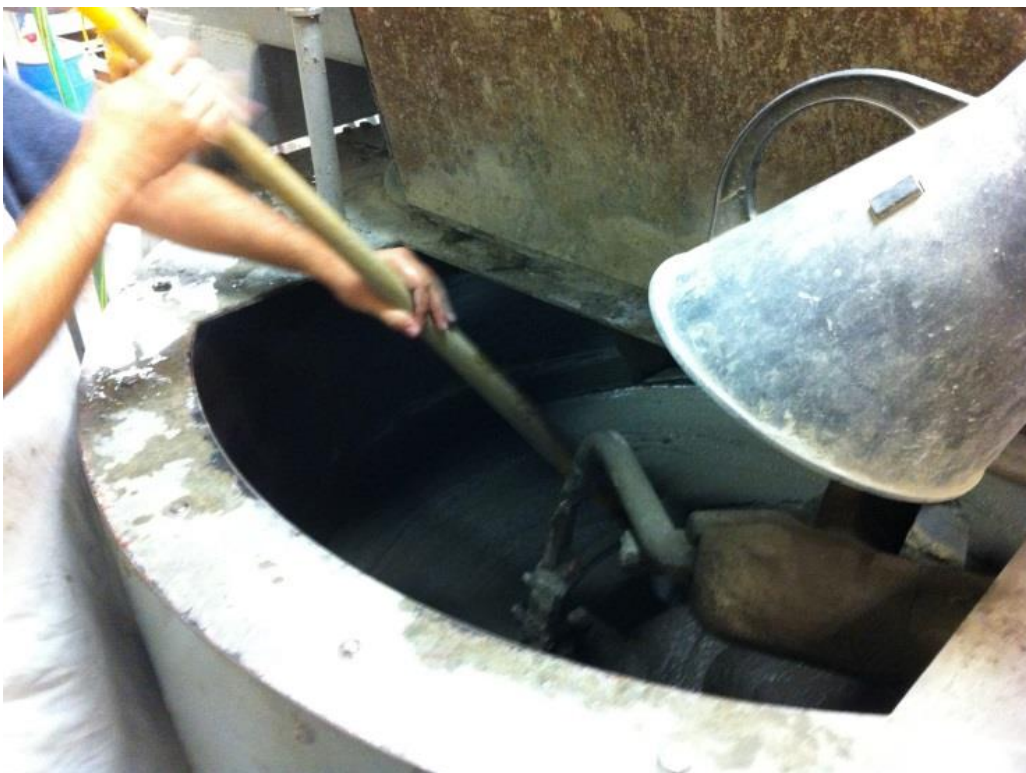
Figure 6.4 Butter mix being applied to the sides of pan mixer
