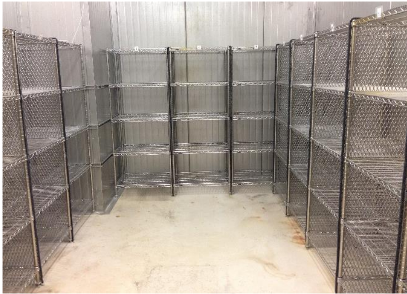
Figure 6.10 Moist curing chamber at FDOT
