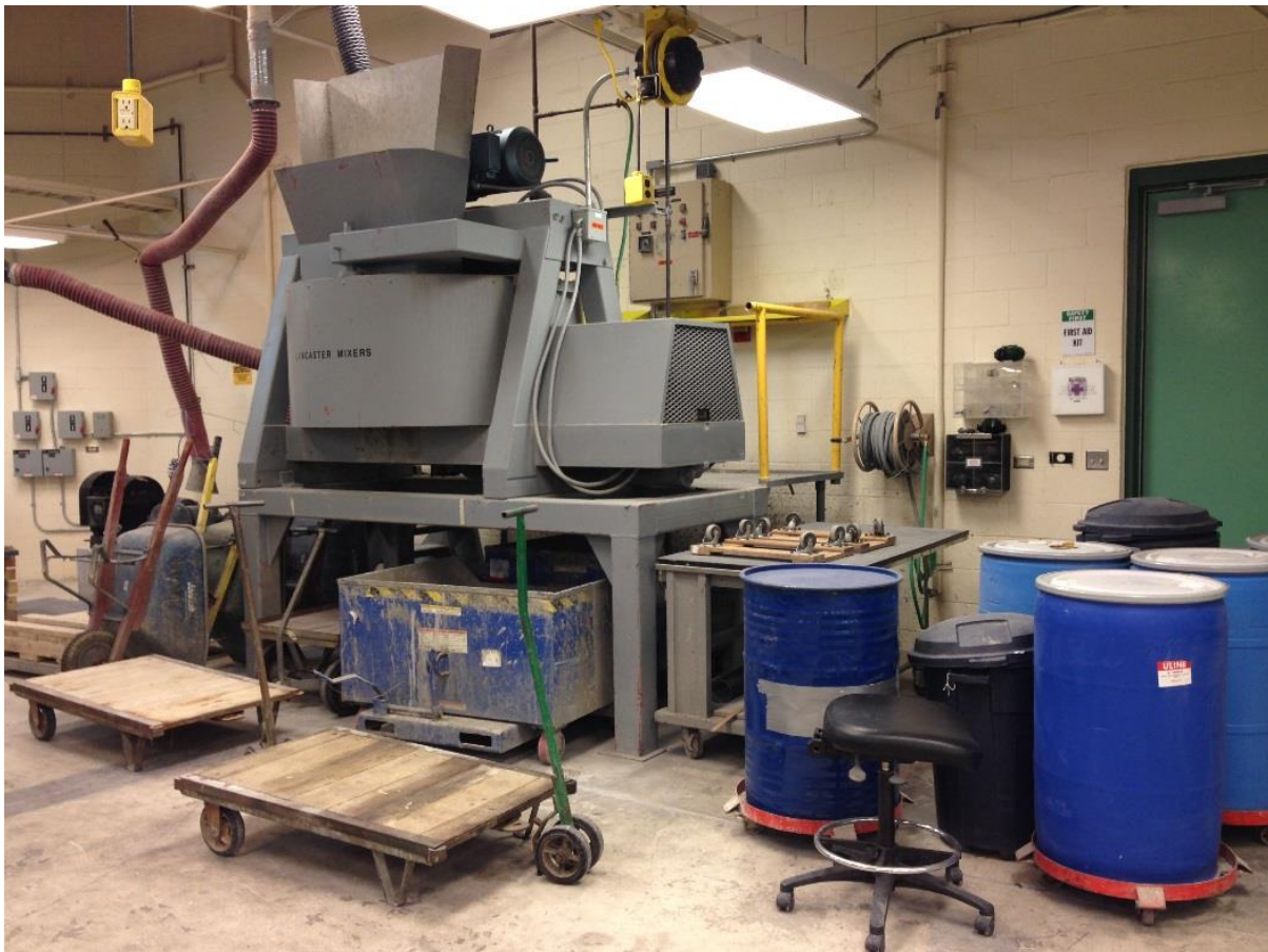
Figure 6.5 Lancaster rotary pan mixer with bins underneath
