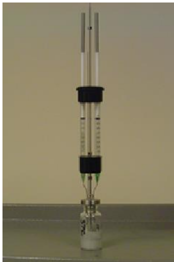
Figure 5.2 Mixing cell and ampoule used for internal mixing procedure
