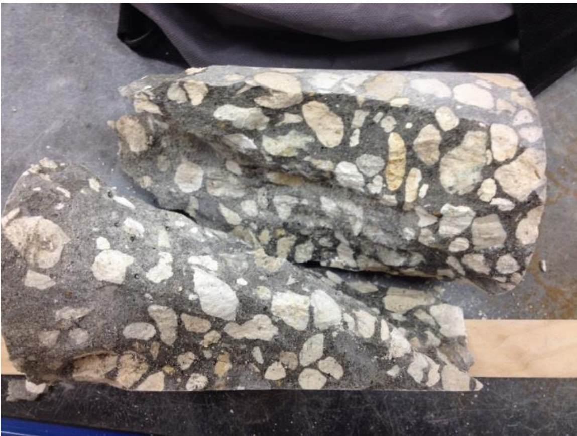
Figure 7.7 Class II mixture with Brooksville aggregate, 91-day fracture plane
