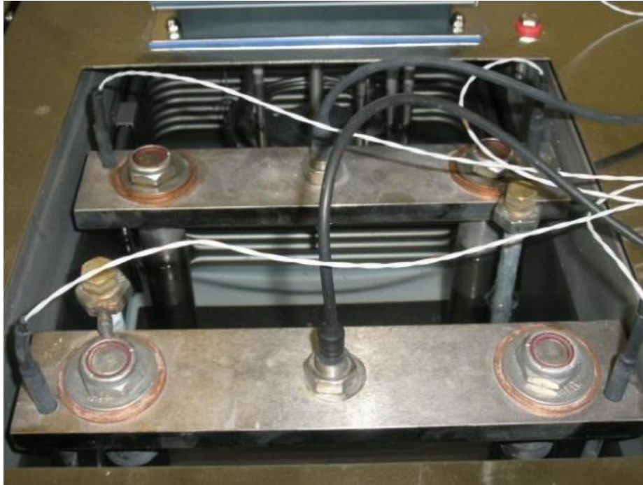
Figure A.5 Water bath reservoir with INVAR frames in place (FDOT system)
