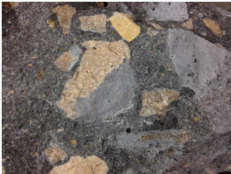
Figure 7.9 Class VI mixture with Perry aggregate, 56-day fracture plane
