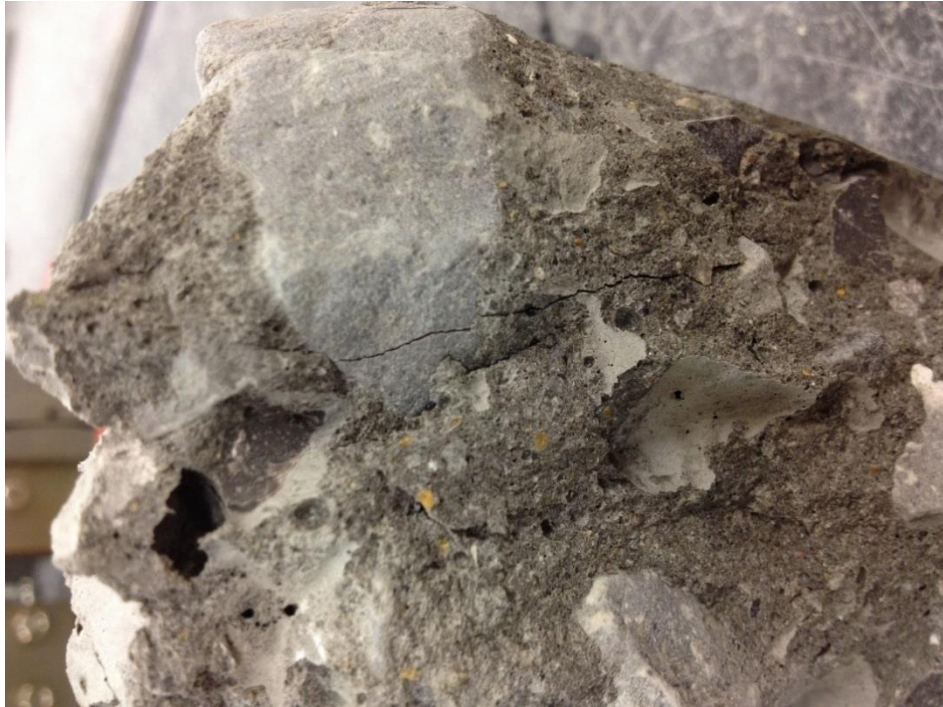
Figure 7.12 Class VI mixture with granite aggregate, 56-day fracture plane
