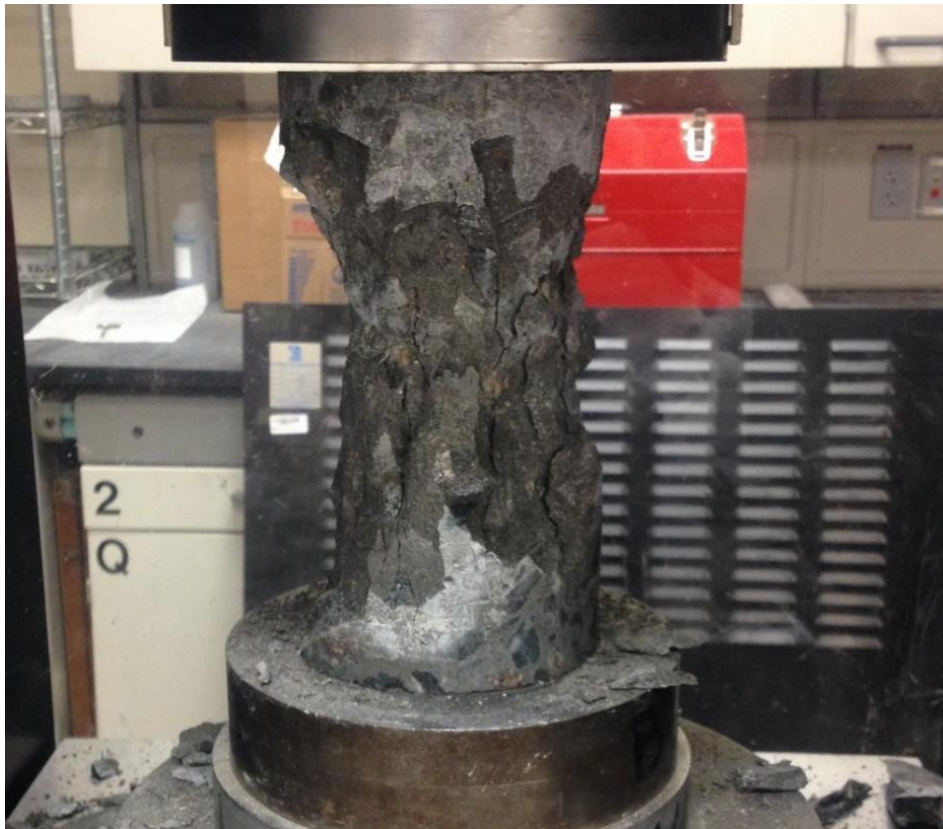
Figure 7.13 Class VI mixture with granite aggregate, 91-day cylinder failure
