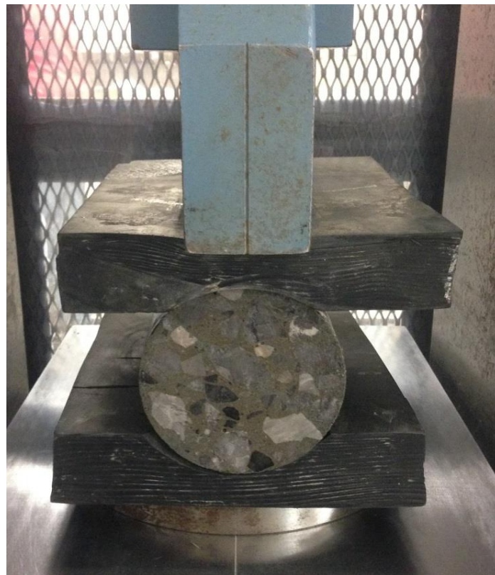
Figure 8.2 Specimen prepared for horizontal orientation for rebound numbers
