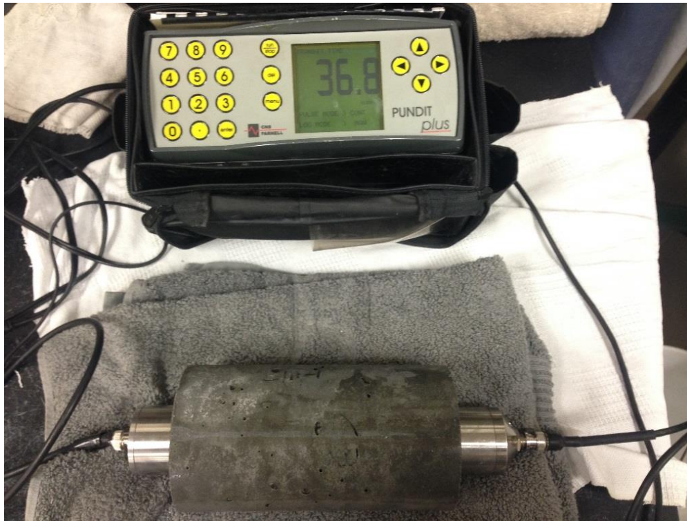
Figure 8.7 Pulse velocity recording transit time on cast specimen
