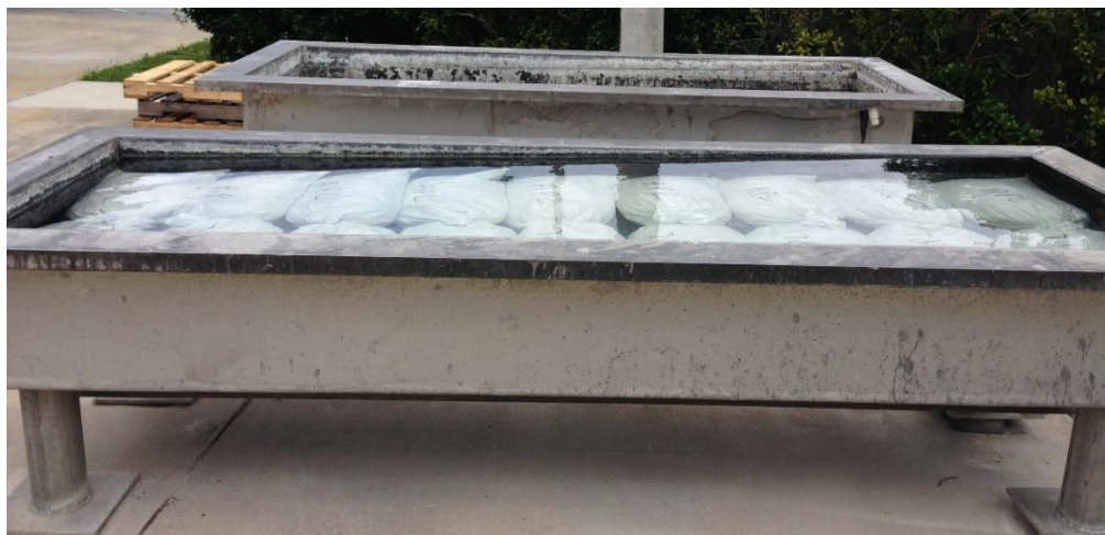
Figure 6.1 Coarse aggregate soaking in tanks at FDOT State Materials Office
