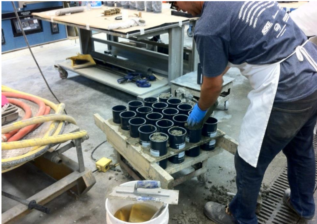
Figure 6.7 Placement of concrete in cast specimens
