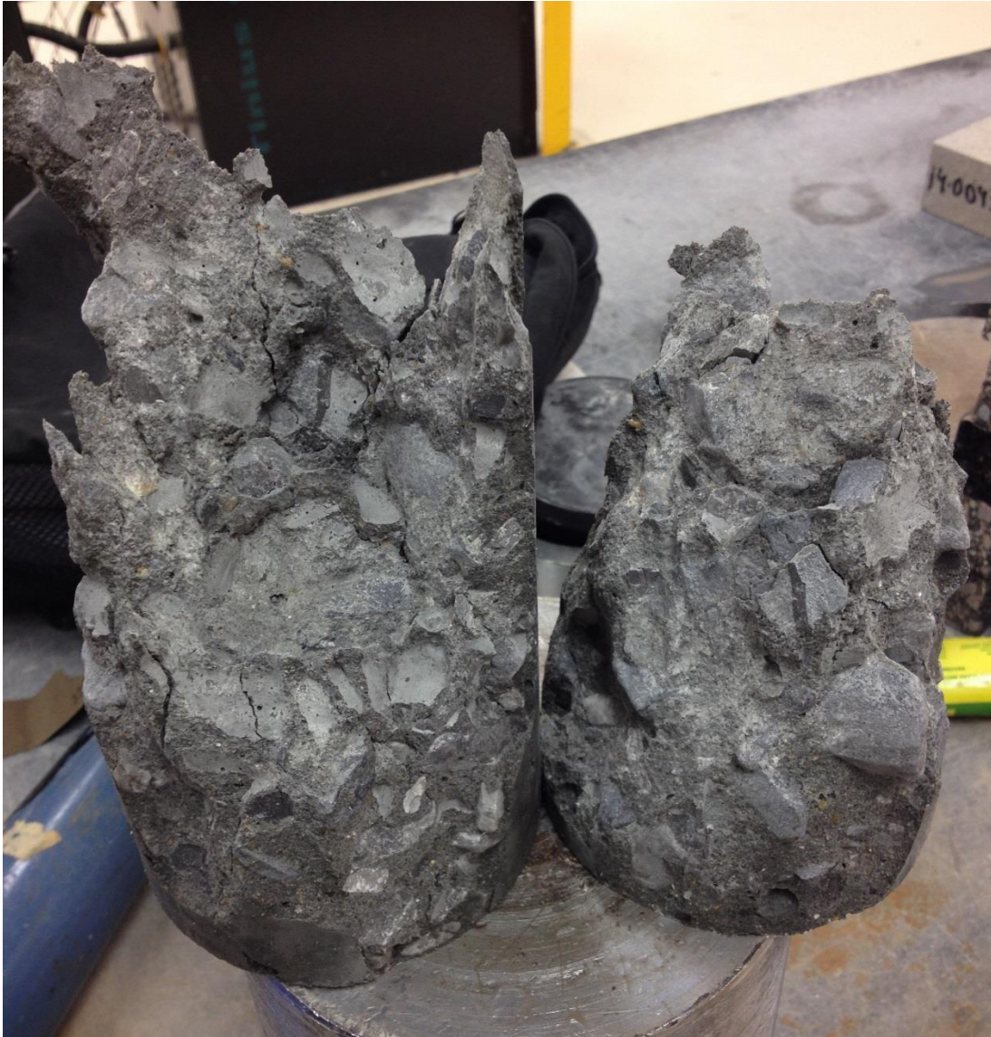
Figure 7.14 Class VI mixture with Calera aggregate, 14-day cylinder failure
