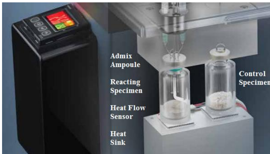
Figure 5.1 Internal view of TAM Air isothermal conduction calorimeter
