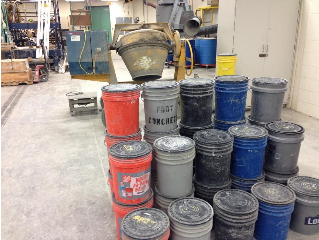
Figure 6.3 Trial mixes batched and ready for mixing
