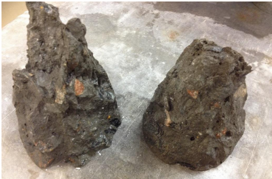
Figure 7.11 Class VI mixture with granite aggregate, 3-day failure cones
