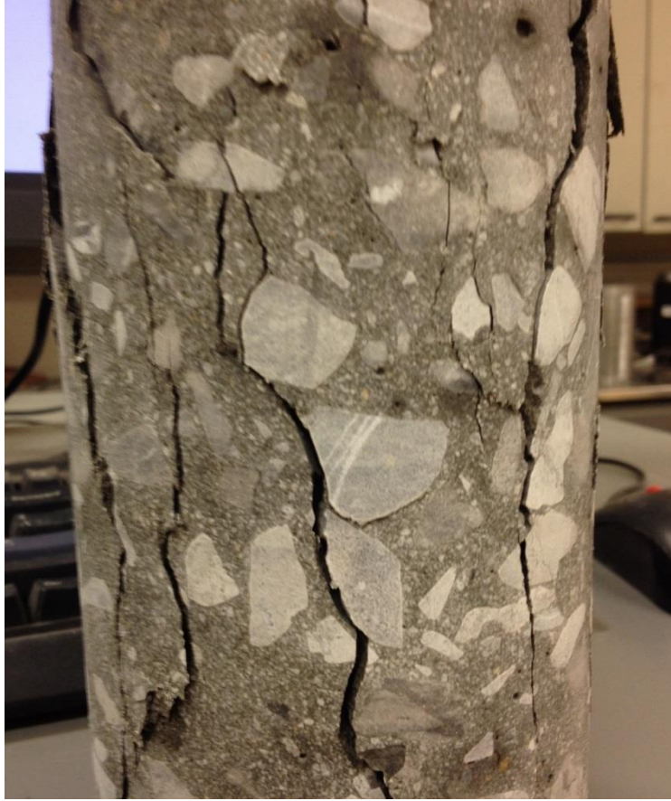
Figure 7.15 Class VI mixture with Calera aggregate, 14-day core failure
