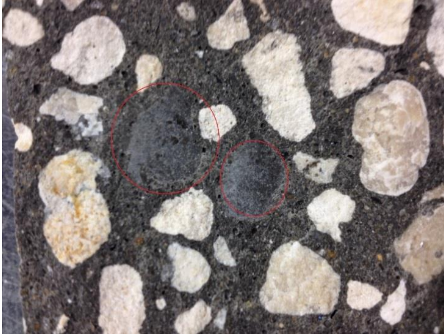
Figure 7.6 Class VI mixture with Brooksville aggregate, 7-day fracture plane
