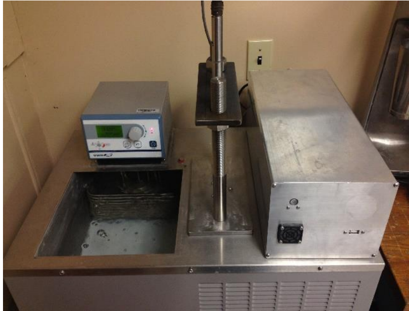
Figure A.1 Thermal Bath used for AASHTO T336.
