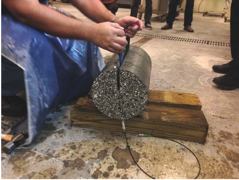
Figure 0-14. Prying technique used for sensor removal.
