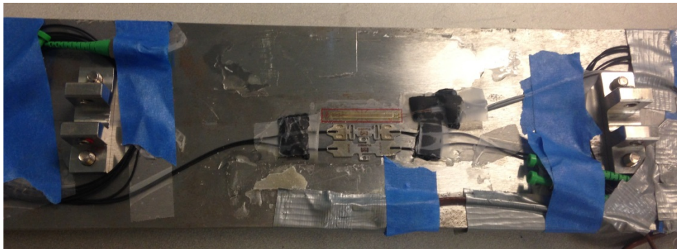
Figure 0-17. Sensor layout before installation of os3610.
