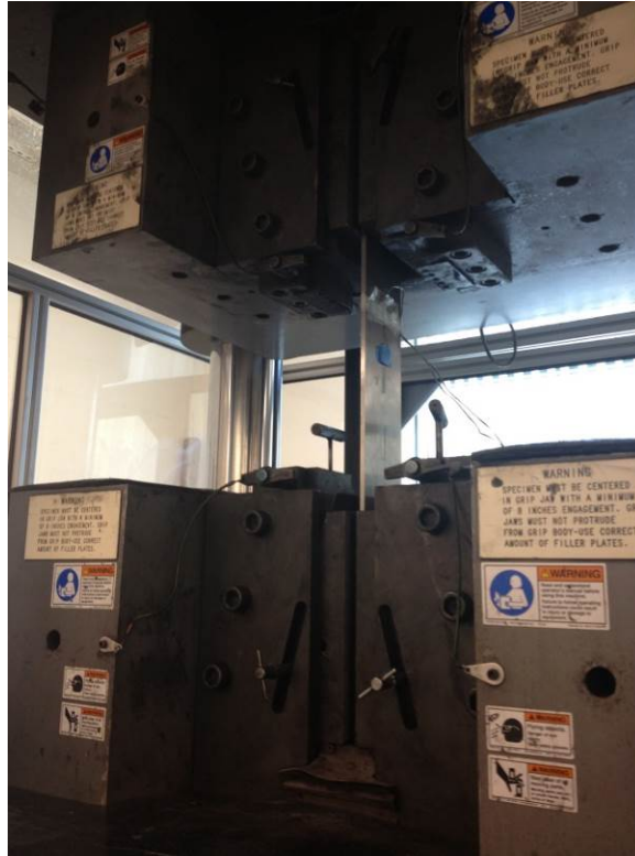
Figure 0-19. Instron UTM being used for steel plate tension test.
