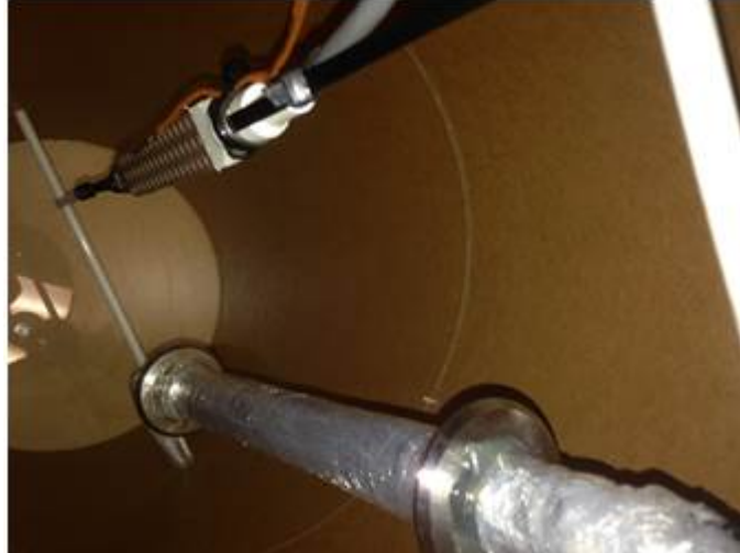
Figure 0-5. Sensor layout for formwork of the concrete cylinder specimen.
