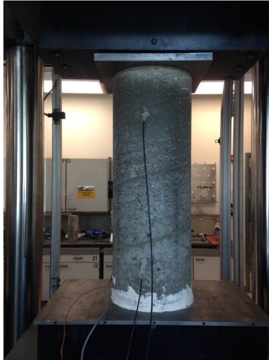
Figure 0-7. Instron UTM being used for concrete cylinder compression test.
