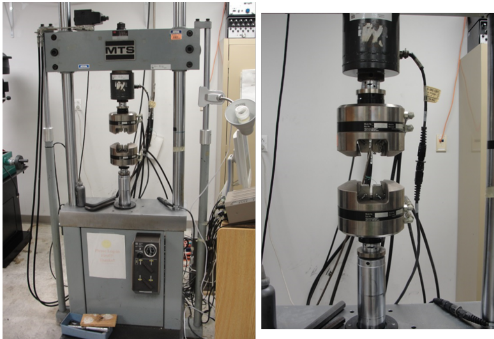
Figure 5-5. MTS 470 with hydraulic grips.
