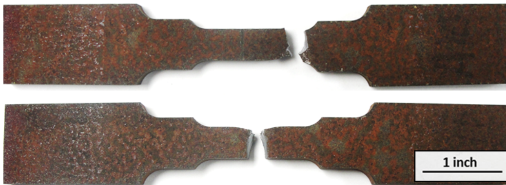
Figure 5-12. Fatigue specimen that fractured (top) near the shoulder and (bottom) at the plasma notch.
