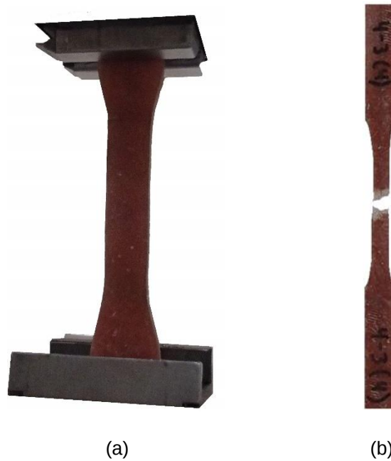
Figure 157—(a) GFRP coupon tension test setup (b) typical failure mode of test coupon
