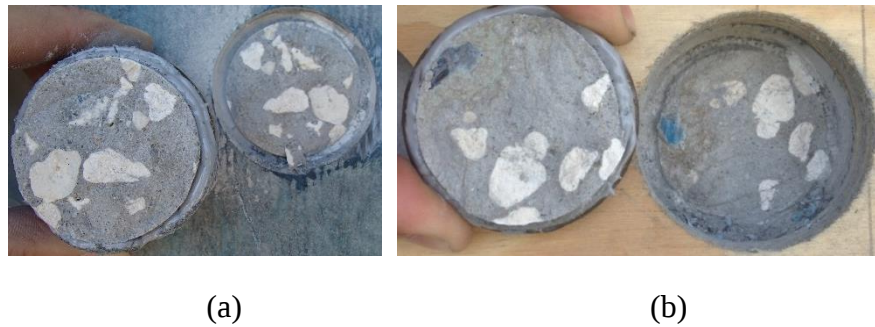
Figure 75—(a) Typical cohesive failure mode (b) typical mixed failure mode
