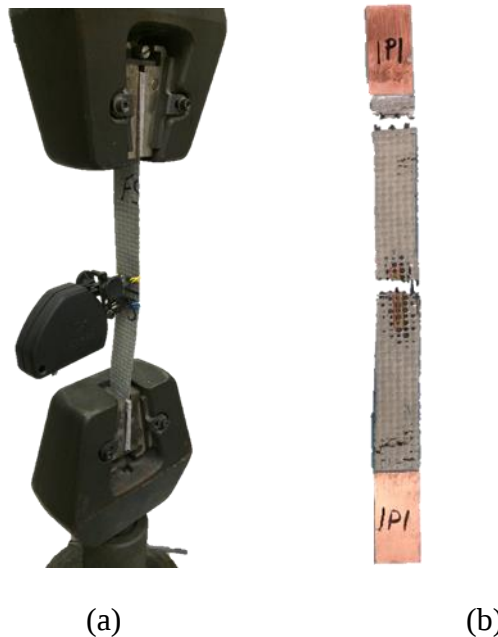
Figure 100—(a) CFRP coupon tension test setup (b) typical failure mode of test coupon
