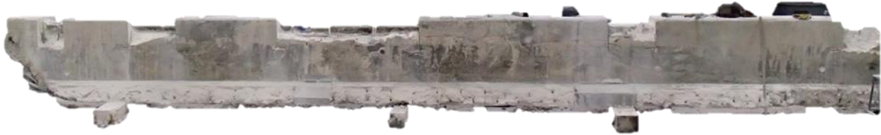
Figure 119—Test girder in inverted position
