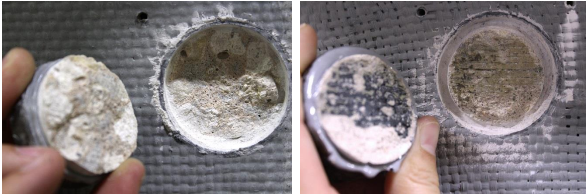
Figure 102—Failure mode: (a) cohesive and (b) adhesive
