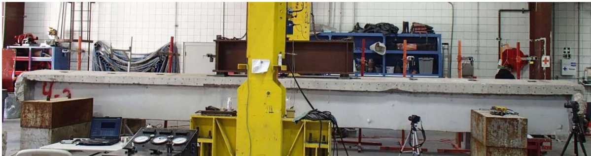
Figure 167—Girder loaded in test frame
