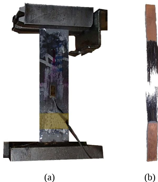
Figure 149—(a) CFRP coupon tension test setup (b) typical failure mode of test coupon
