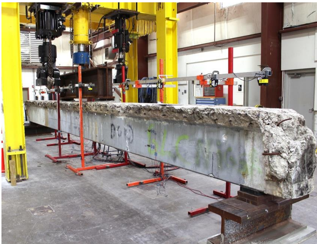
Figure 110—Girder loaded in test frame
