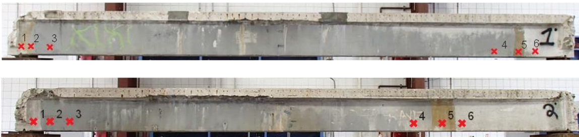
Figure 93—Approximate coring locations for \text{Cl}^- penetration profile cores on each girder
