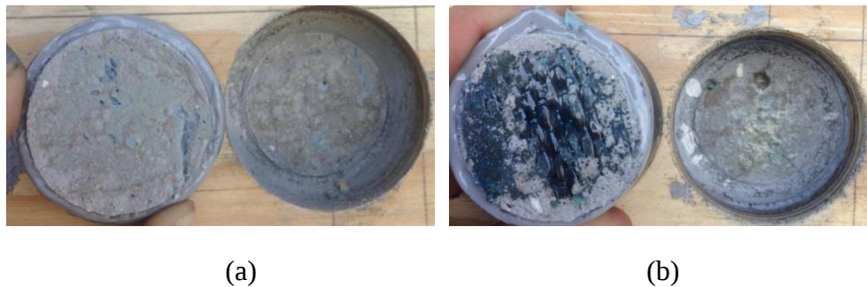
Figure 76—(a) Typical adhesive failure mode (system with putty) (b) typical adhesive failure mode (system without putty)
