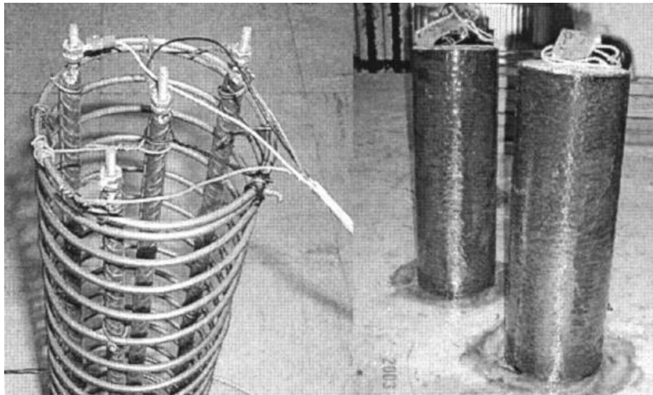
Figure 265—Small-scale columns (Bae and Belarbi, 2009): reinforcement cage used for small-scale RC columns (left) and small scale RC columns after CFRP sheet wrapping
