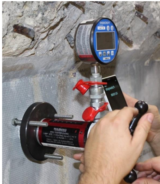
Figure 101—Direct pull-off test setup
