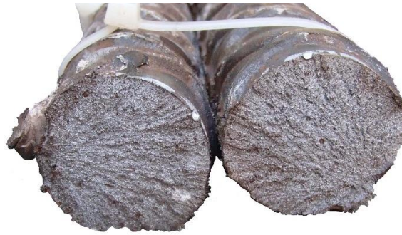
Figure 146—Typical hackle pattern pointing to the origin of fracture surface, which in this case is the spot weld
