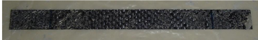
Figure 262—CFRP sample with most of its debonding at the concrete-epoxy interface
