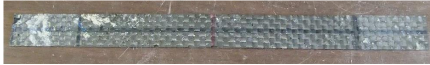
Figure 261—CFRP sample with most of debonding at the CFRP-epoxy interface
