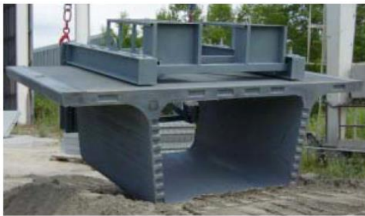
Figure 2.10 (a) General view of PS34 overpass (Resplendino 2008); (b) full-scale mock-up of a precast segment, with the scheme of extracted samples (AFGC recommendation 2013).
