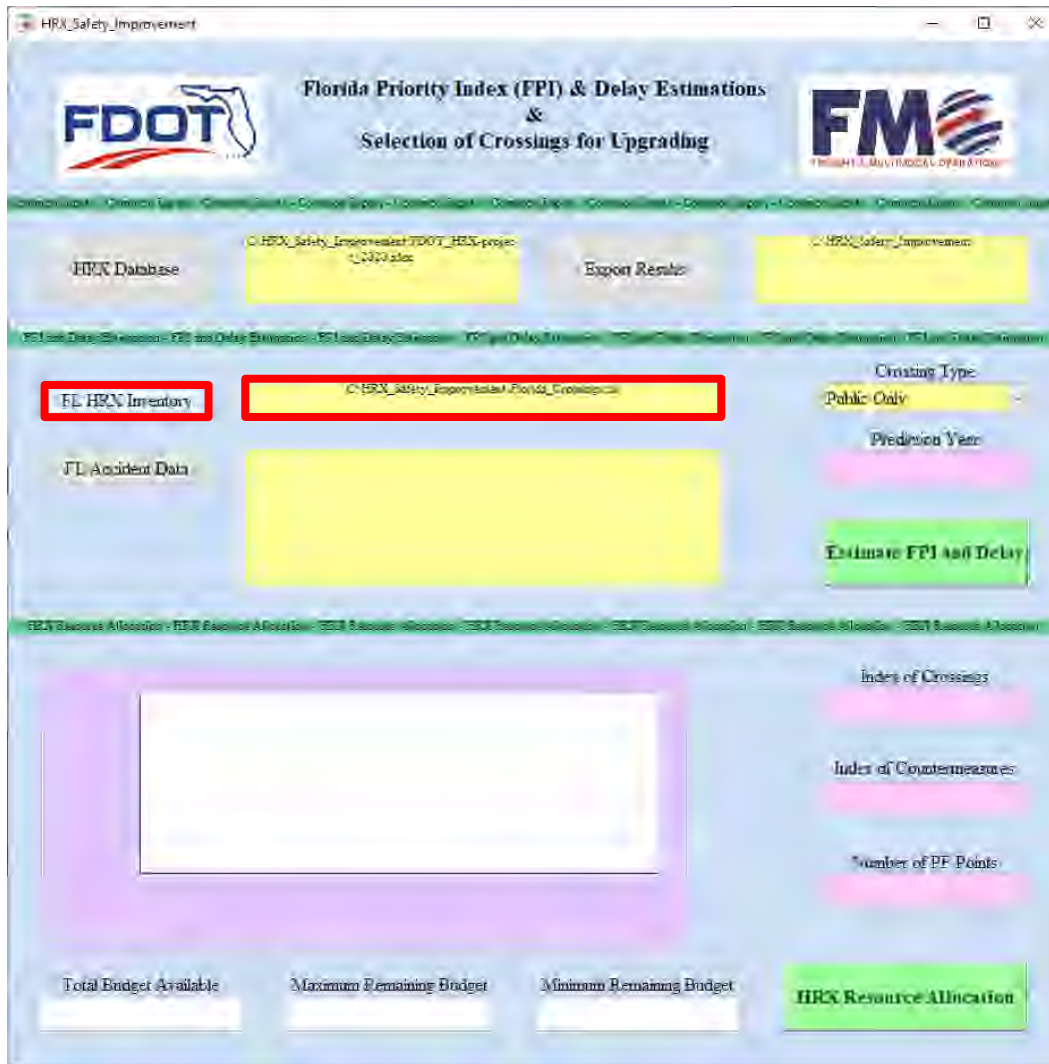
Figure 89 Loading the crossing inventory data.
