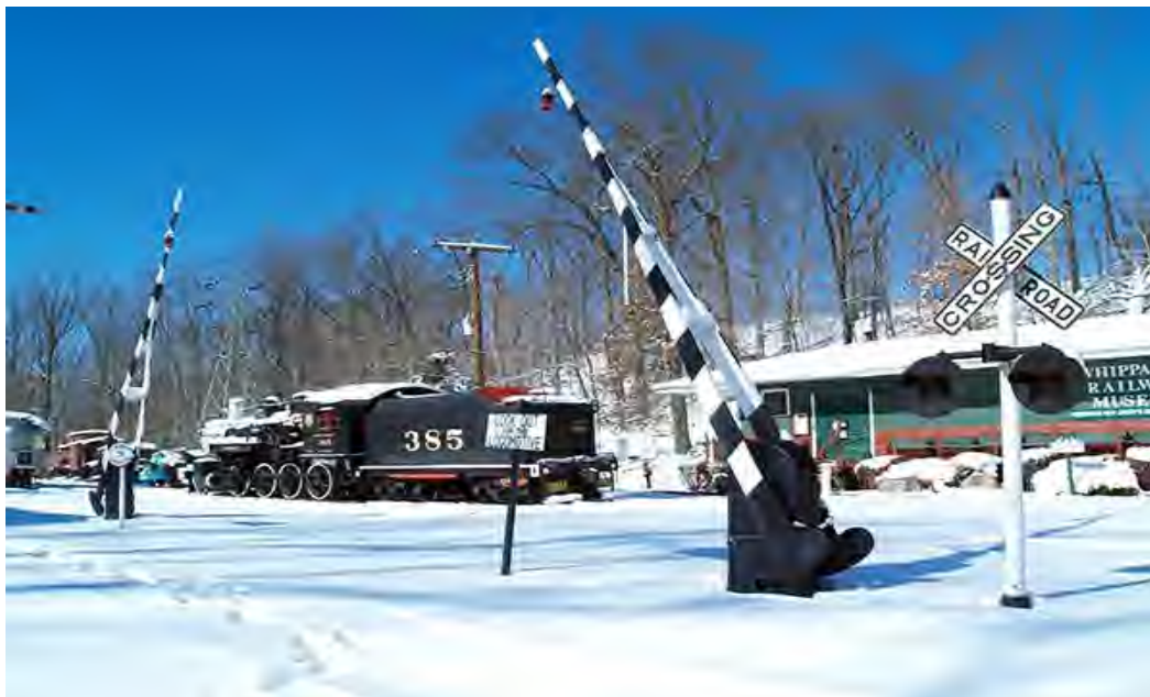
Figure 39 An example of basic gates. Source: Whippany Railway Museum. (2020). Railroad Crossing Gates & Signals
