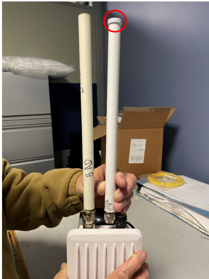
Figure 2.2 Antenna Design Changes Made by the Vendor
