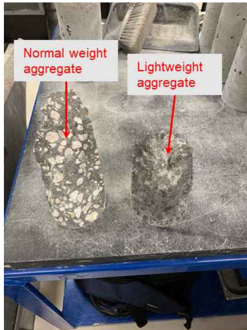
Figure 9 Illustration of normal-weight and lightweight aggregates in cylinders
