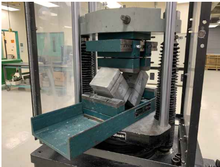
Figure 15 Failure of concrete beam in tension
