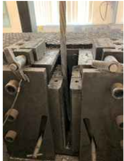
(c) seating the end of the specimen in the grip
