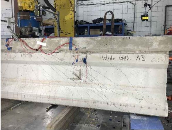
Figure 10-26 Flexure-shear failure of Girder A3_1
