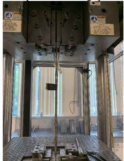
(f) failure of the specimen close to the grip
