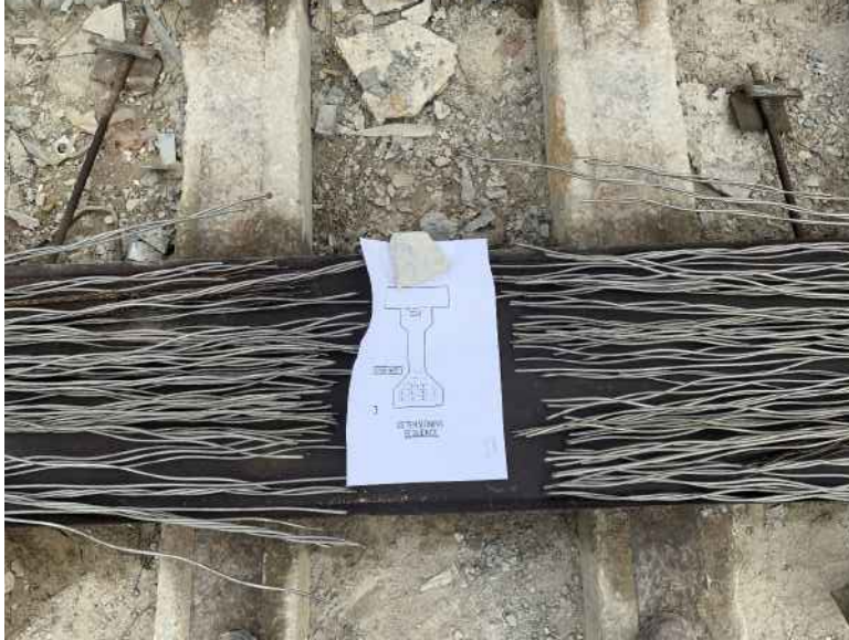
Figure 4-27 Twist of HSS strands after cut
