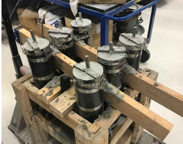
Figure 3-8 Six HSSS specimens prepared for bond strength test
