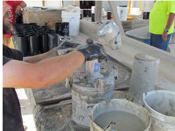
Figure 4-11 Concrete air content test
