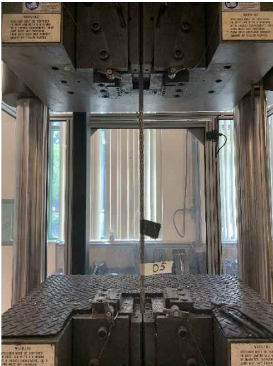
(d) preload to align the strand and seat the ends in the grips
