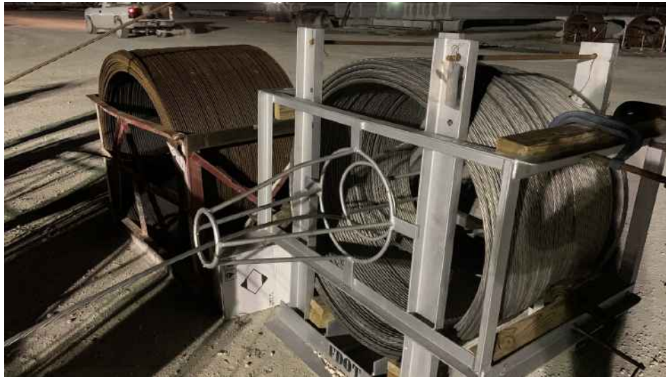
Figure 1-3 Comparison of surface layer of carbon steel spool (left) and stainless steel spool (right)
