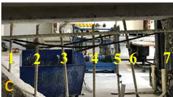
Figure 10-19 Concrete crushing and rupture of GFRP for Girder A2_1
