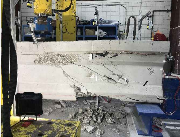
Figure 10-31 Web shear failure of Girder B3_1
