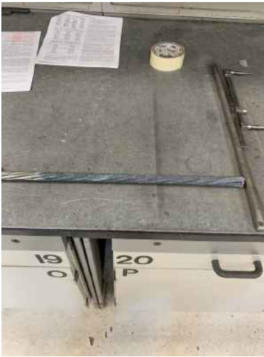
(a) coating end of a specimen with epoxy
