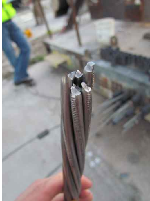
Figure 4-18 Notching effect of grips on fractured HSSS strands
