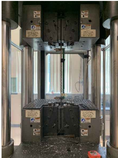
(e) attached extensometer to measure strain up to 1% elongation
