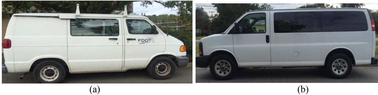
Figure 3.4 Test Vehicles Used with Axle Spacing of (a) 9.04 ft and (b) 11.19 ft
