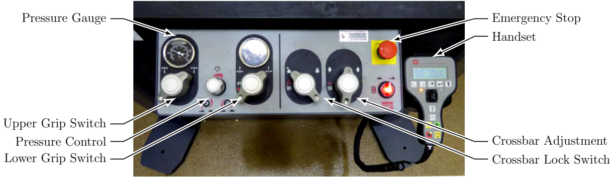
Figure 4.15: MTS load frame control panel
