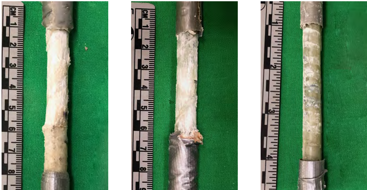
(a) Type-A (b) Type-B (c) Type-C Figure 5.19: Bond failure at rebar interface of all rebar types after 365 day of exposure to 60 °C saltwater
