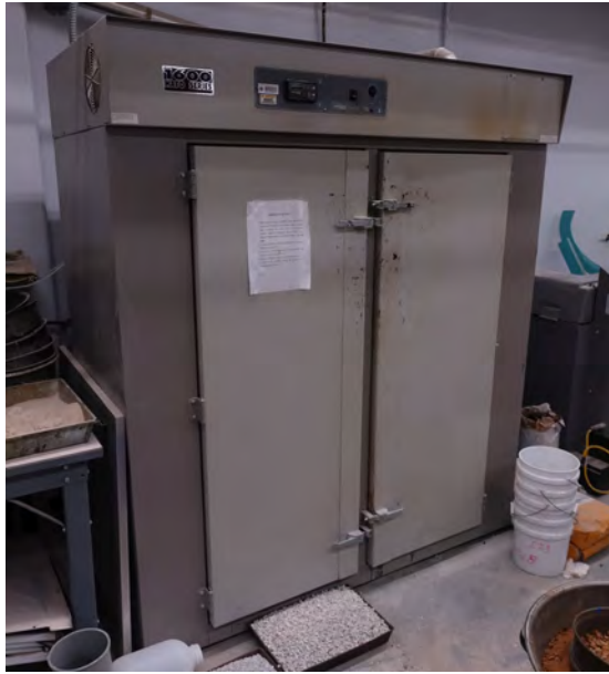
Figure 4.8: Drying oven VWR Scientific Products Oven Model 1690
