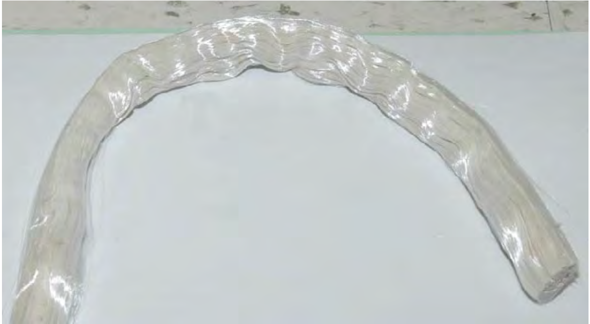
Figure 2.7: Bare fibers of bent section after removing the resin
