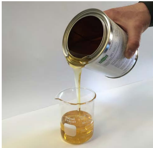
Figure 2.1: Thermosetting polymeric resin used for GFRP rebars
