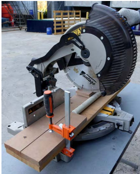
Figure 4.3: Miter saw used to cut raw materials to specimen length
