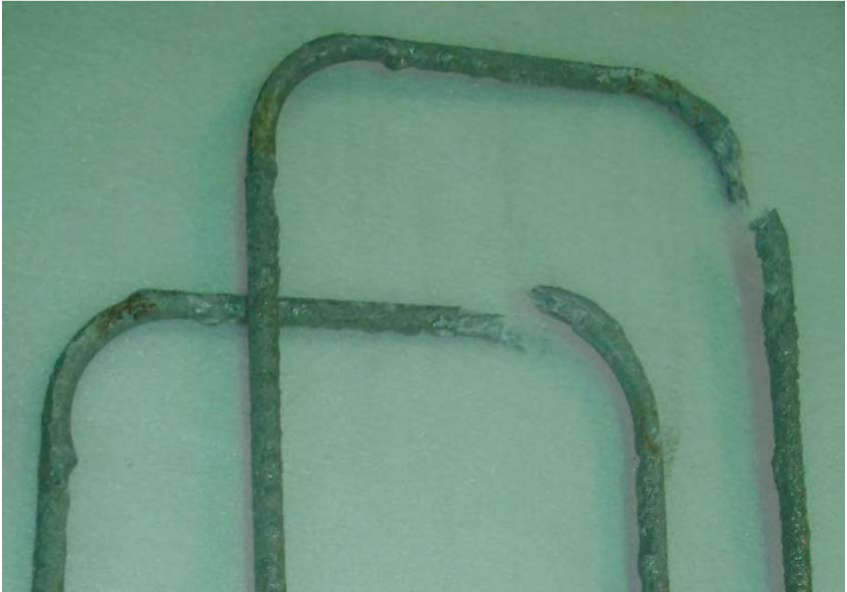
Figure 2.9: Typical failure of FRP stirrups Ahmed et al. (2010)
