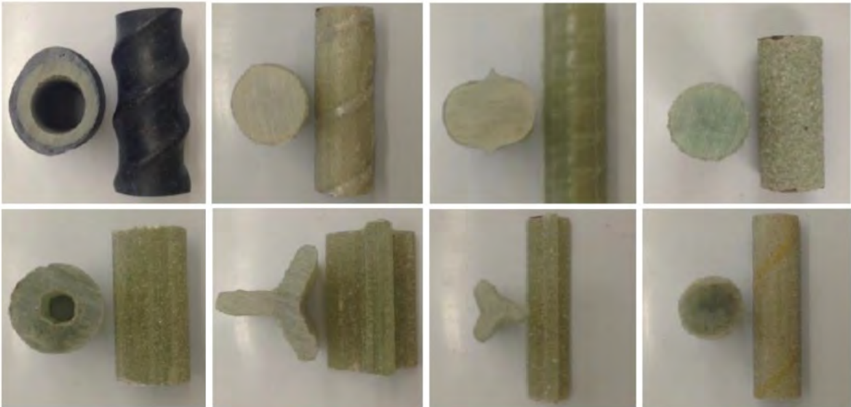
Figure 2.5: GFRP bars with different cross-sectional shapes, reprinted with permission from Claire (2015)
