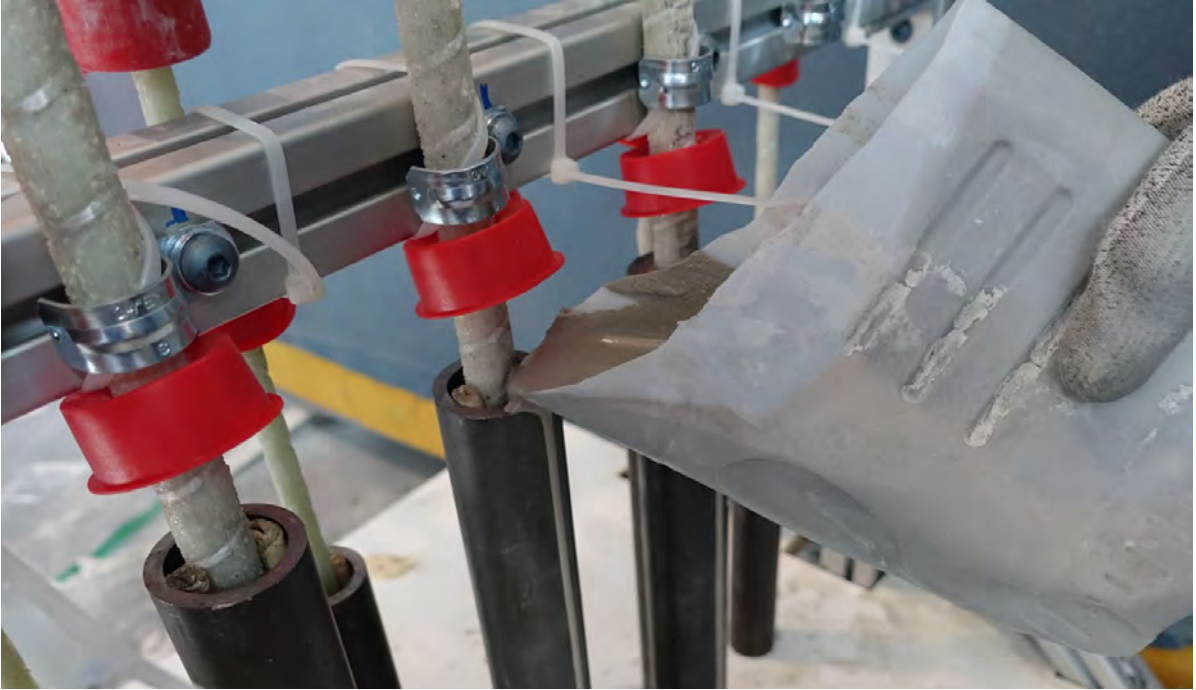
Figure 4.38: Potting of the anchors for tensile test specimens
