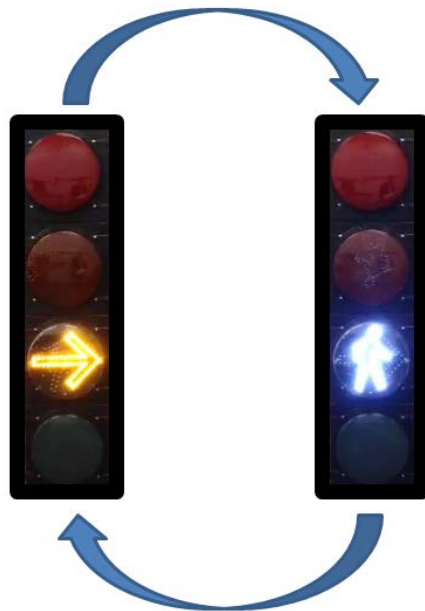
Figure 1. The Flashing Turn Signal Head with Pedestrian Indication (FPI).
